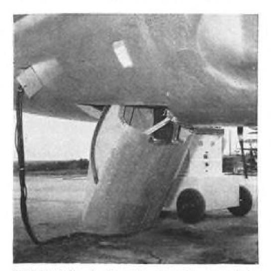
SPEED brake is close to ground, cannot be used during taxiing, takeoff, or landing.
