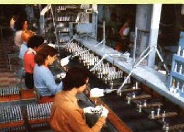
FINAL INSPECTION of the completed aircraft spark plug includes visual inspection, resistance test, high-voltage bomb test and final X-ray. After checking the gap size for extreme accuracy, the spark plug is dated for factory records.
