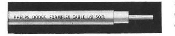
A semi-flexible cable with tubular copper inner conductor, foamed polyethylene dielectric and commercially pure aluminum outer conductor.
