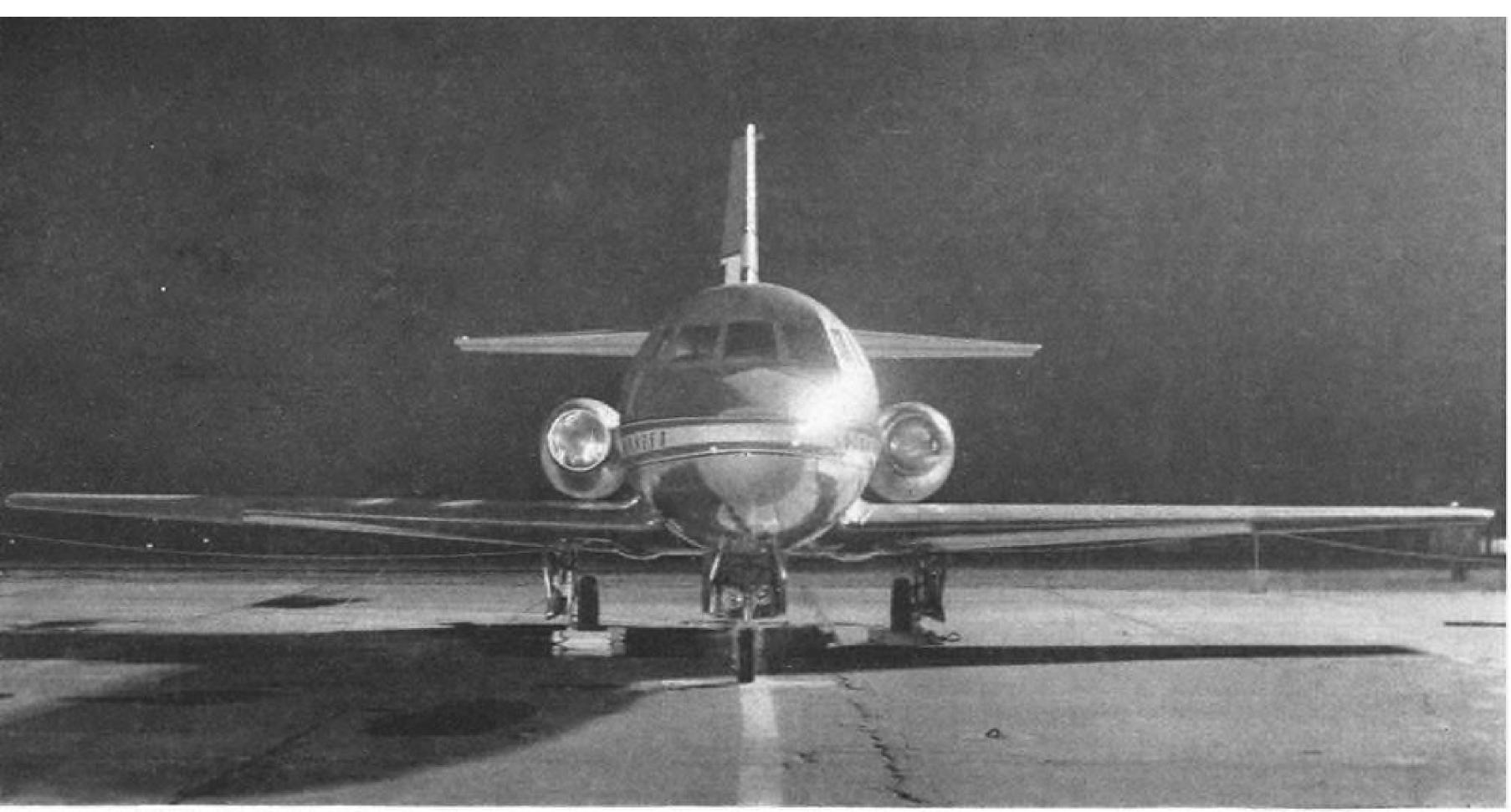
LOCKHEED CL-329 JetStar ground visibility runs 40 ft. ahead of nose. Tread is 10 ft. 9 in.; wheel base is 20 ft. 9 in.
