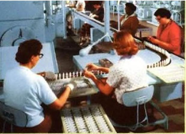
FINAL ASSEMBLY where the insulator assembly is mated to the shell. Starting with a resistance check of the insulator, the finished aircraft spark plug begins to take shape. After the shell components are in place, they are crimped, welded and brazed to form a leakproof unit. This unit must then pass a 1,000 p.s.i. air test.
