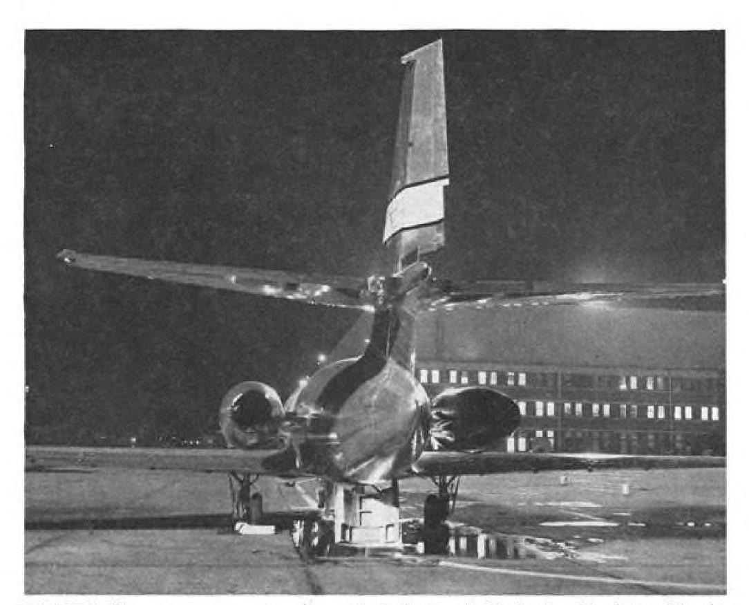
ENTIRE JetStar empennage rotates fore and aft for longitudinal trim. Total travel is nine degrees of stabilizer angle. Speed brake serves as access door to rear compartment.
