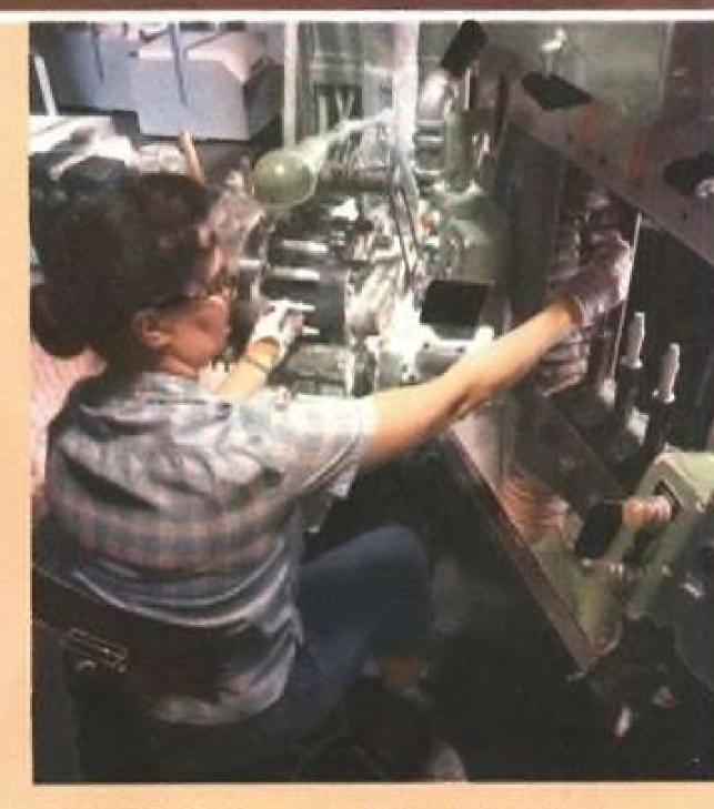
RUBBER MOLDS automatically form insulator blanks with precise accuracy through modern compression methods. After molding, the blanks are precision ground to insure uniformity in length and contour. This method is typical of AC's uncompromising accuracy.
