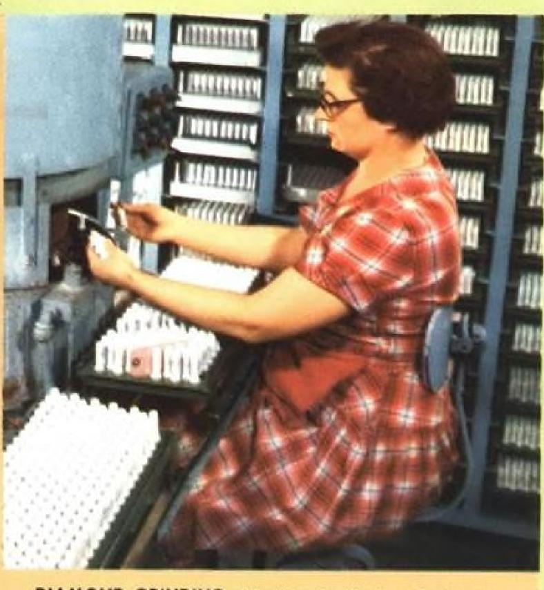
DIAMOND GRINDING of insulator shoulder is confined to extremely close tolerances. This final precision operation insures perfect matching of insulator and the spark plug shell.
