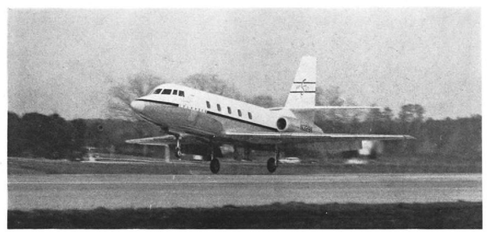
SECOND JetStar prototype is about to touch down. Flaps are full-span slotted type. Drag chute can be used if necessary.
