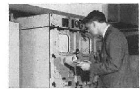
Engineer at Ford Instrument Co. checks out fire control computer developed and built by Ford for the U.S. Navy's Bureau of Ordnance.
