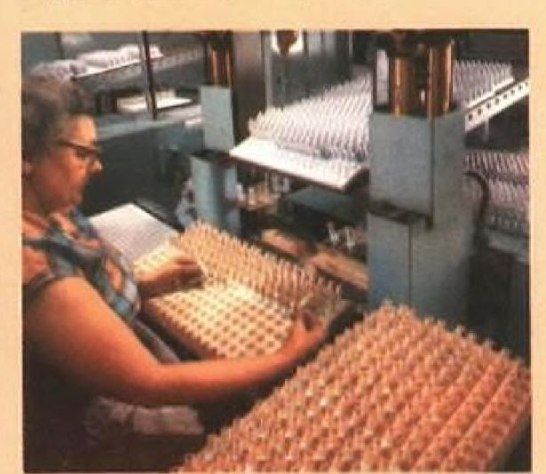
FINISH GLAZE is applied to the insulator barrel and sealing surface prior to final firing. Glazing provides super-smooth surface which minimizes barrel contamination throughout its lifetime.
