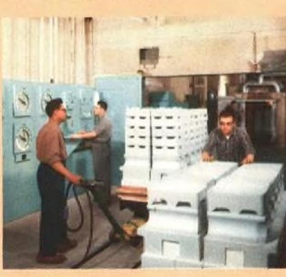
KILN CONTROL PANEL accurately measures both time and temperatures for the all-important insulator blank firing and glazing processes from four stations in the automated high-temperature kiln.
