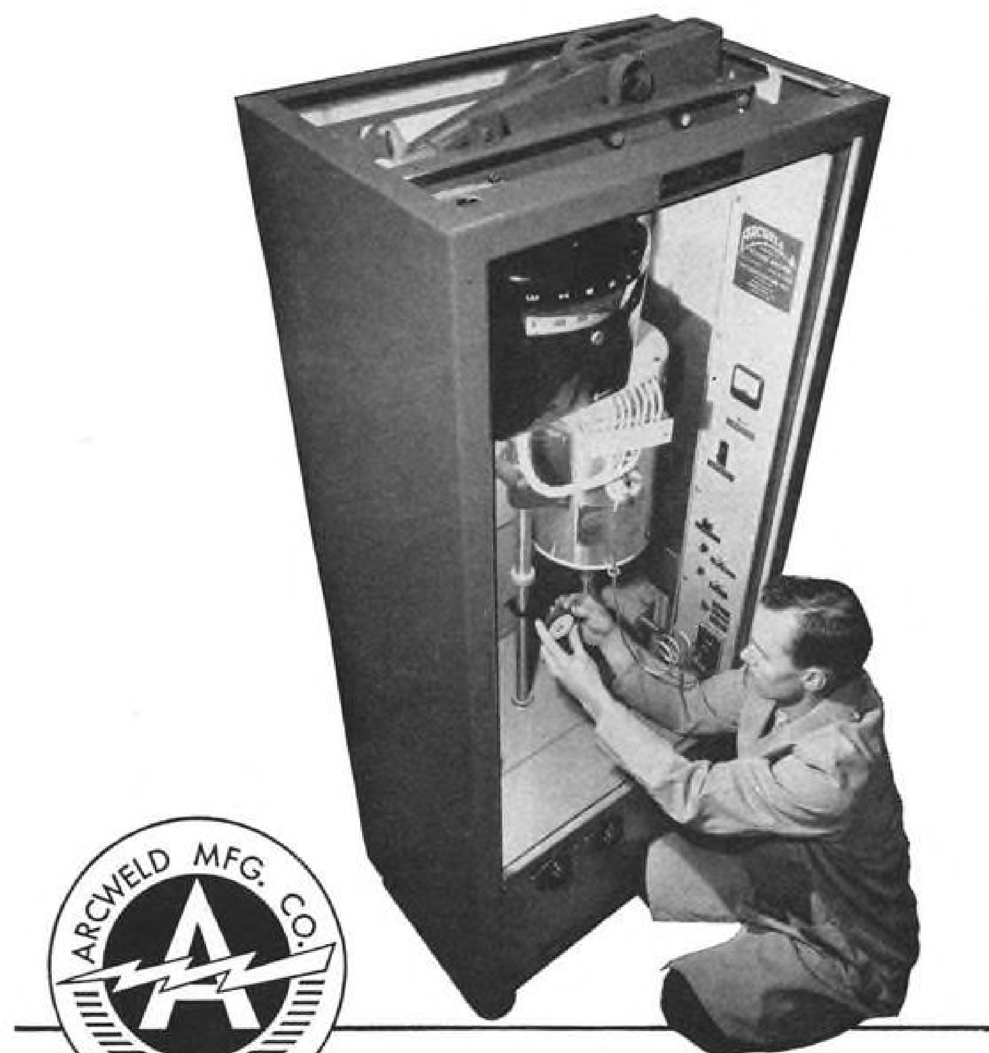
M-3 Arcweld Creep Rupture Tester, custom designed for labs which test smaller size specimens or use lighter loads.
