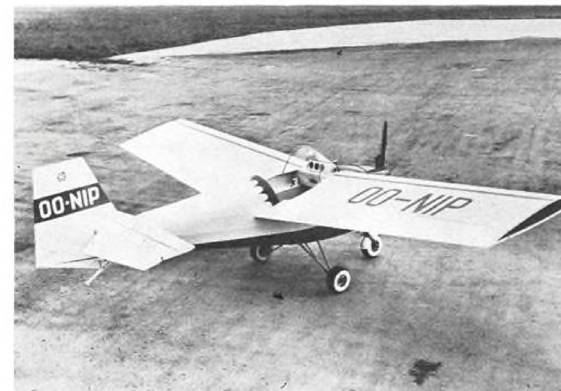
TIPSY NIPPER shoulder-wing layout yields minimum fuselage cross section (left). Portion of wing is hinged to form step (right).
