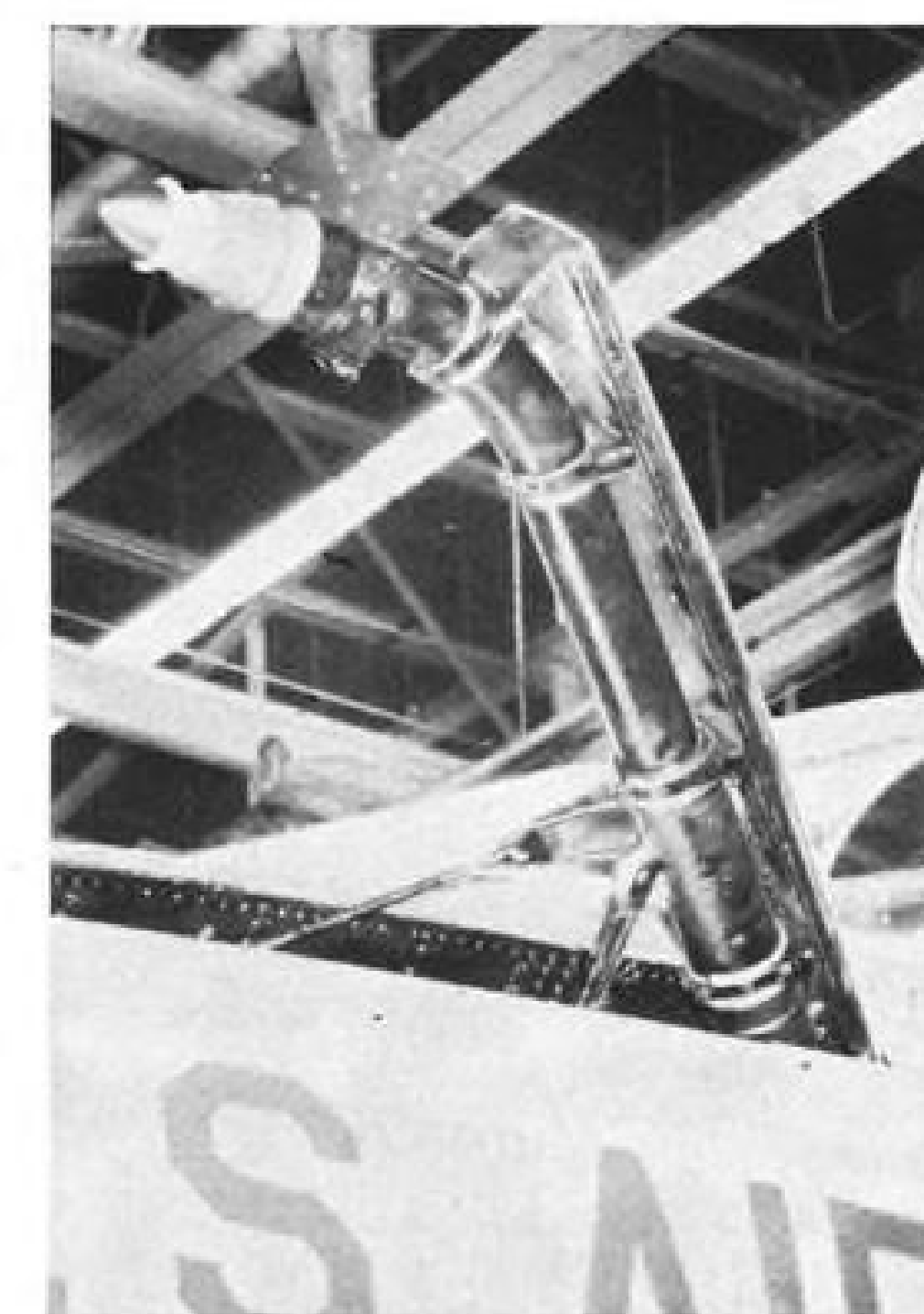
REFUELING PROBE on port side of Thunderchief's nose is shown fully extended. Fairing, door enclose probe when retracted.
