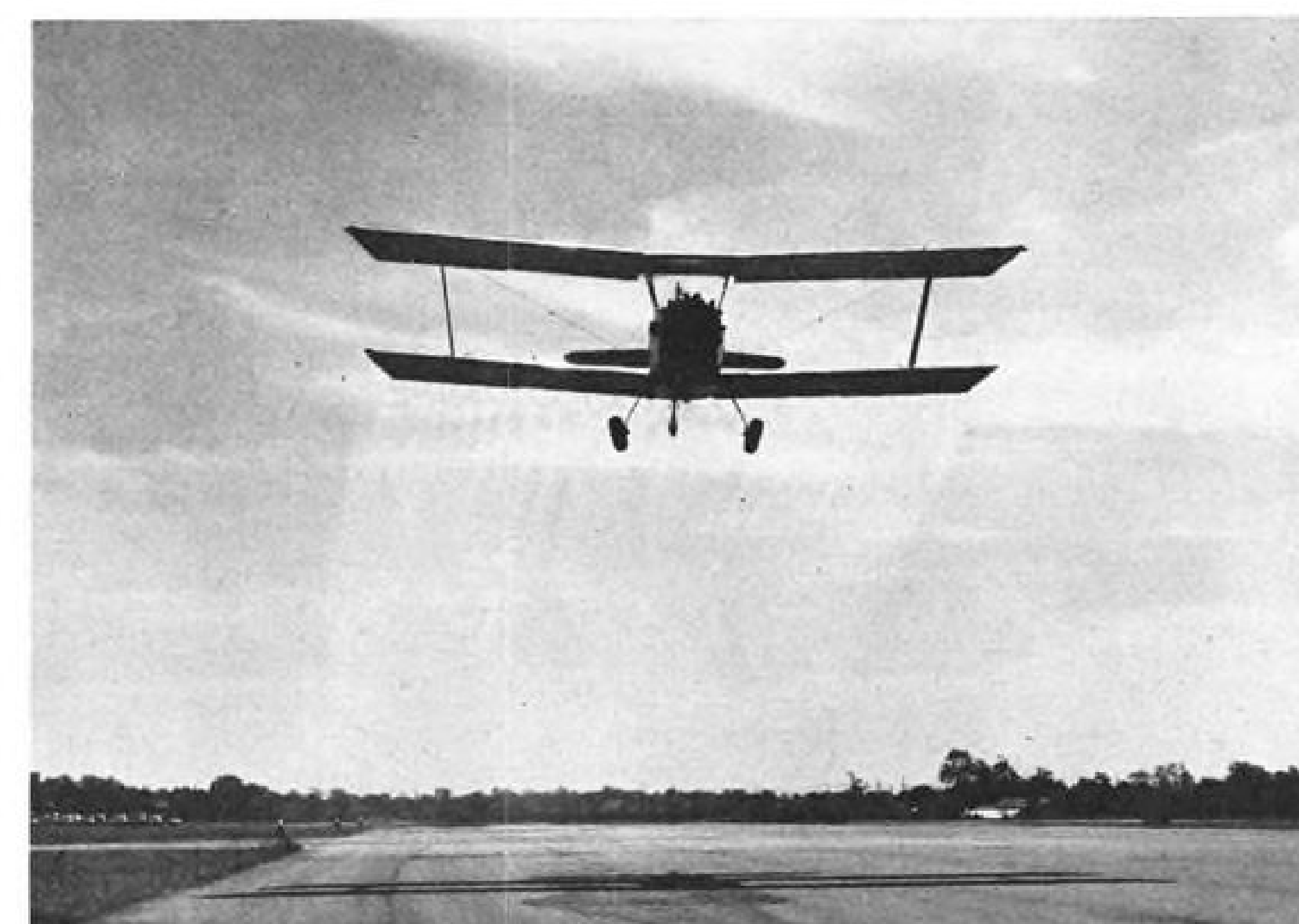
TOTAL wing area of 326 sq. ft., four ailerons, add to Ag-Cat control.
