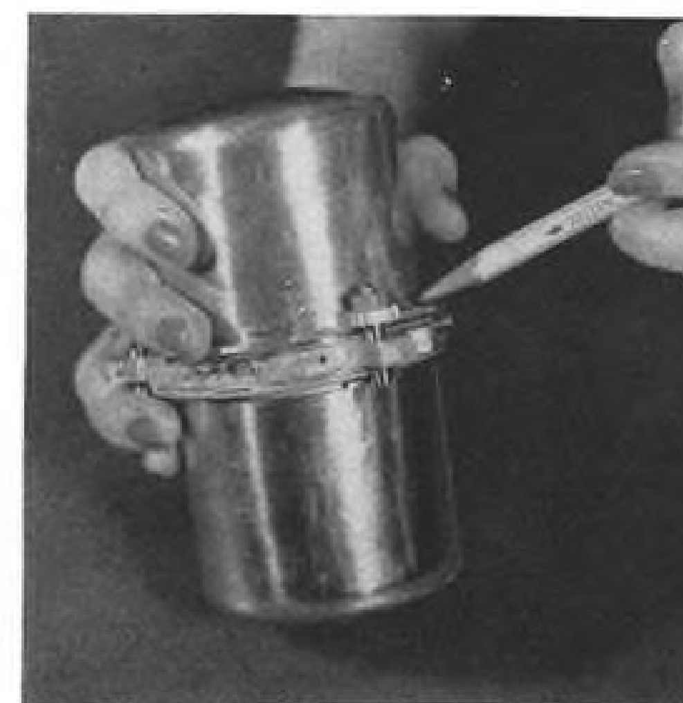
TITAN gyro, two-degree-of-freedom device, is fully-floated, uses wire suspension.
