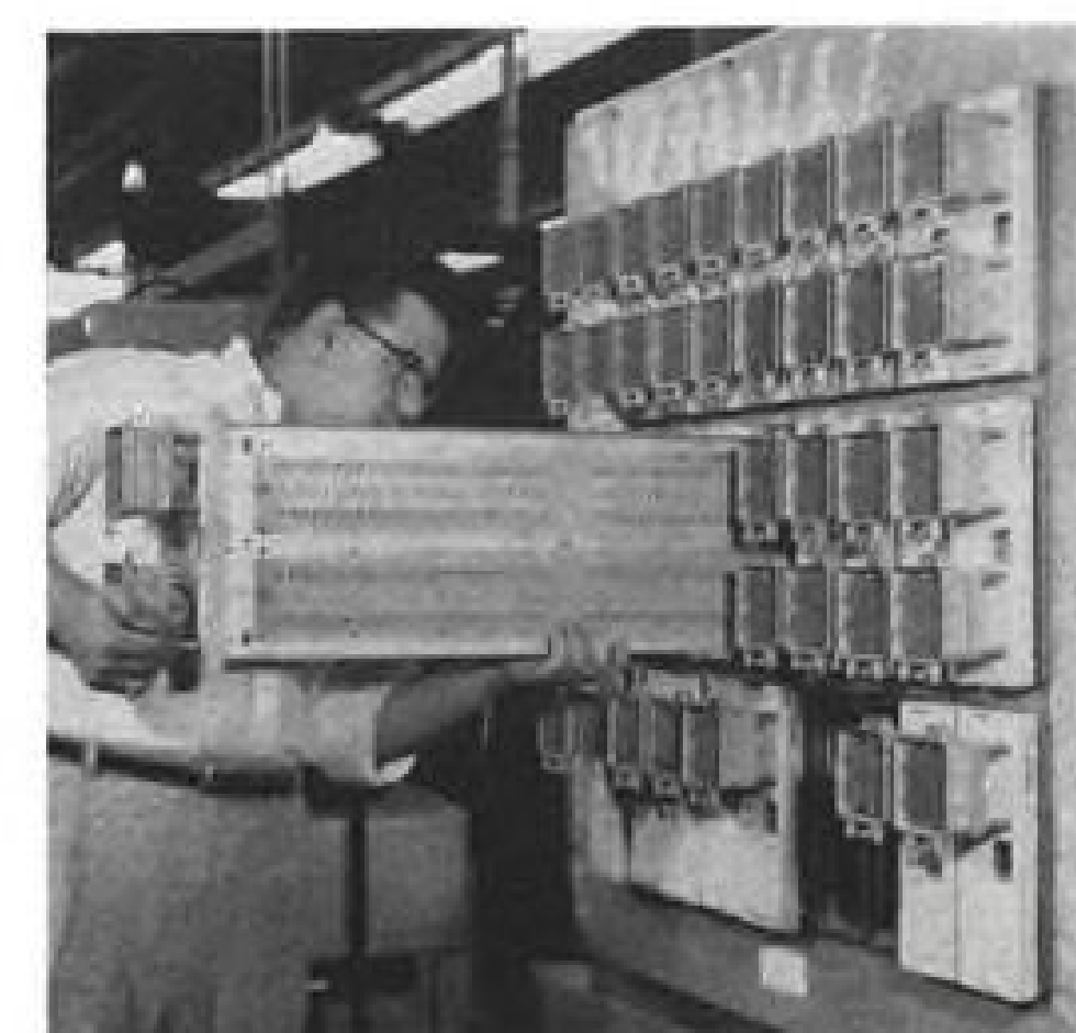
EVERY component of the 40,000 used in Titan guidance system must pass severe environmental tests (left). Weight reduction of Titan guidance computers will result from sandwich construction (lower right) which is one-quarter size of equivalent unit.
