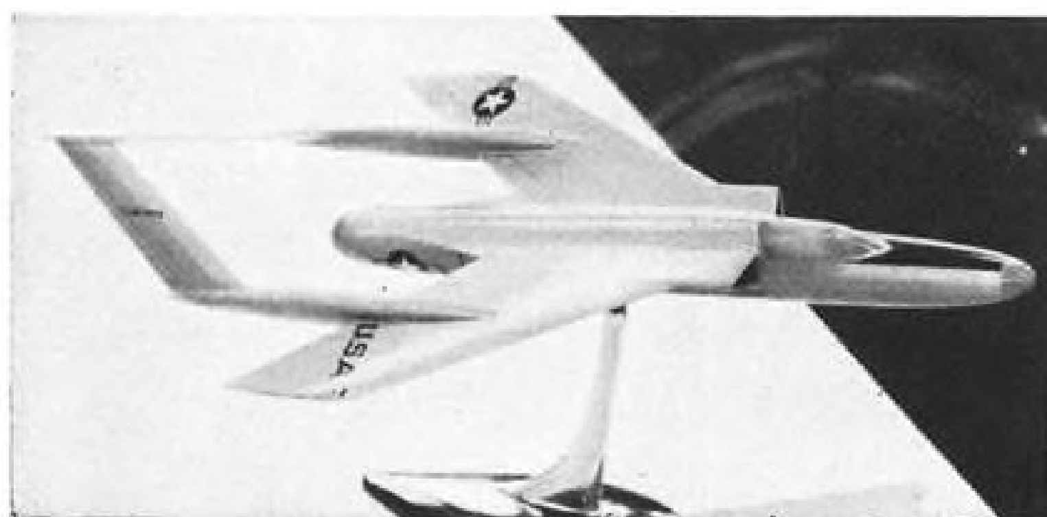
REPUBLIC XF-103 wind tunnel model shows basic delta-wing layout, turbo-ramjet underbelly intake and large tail for high-speed stability.
