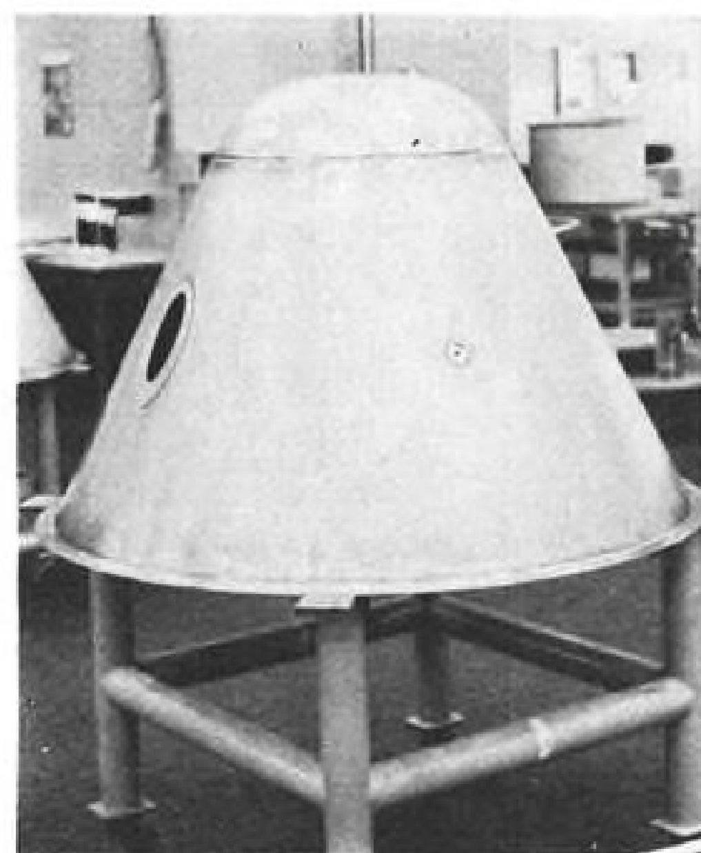
NOSE CONE (above) and afterbody (left) for Thor and Atlas re-entry vehicles were displayed at Republic (AW May 5, p. 29). Nose cone is blunt, copper-based, heat-absorbing structure. Cone liner inside extends below heat shield. Afterbody is hidden from view inside missile until after separation.
