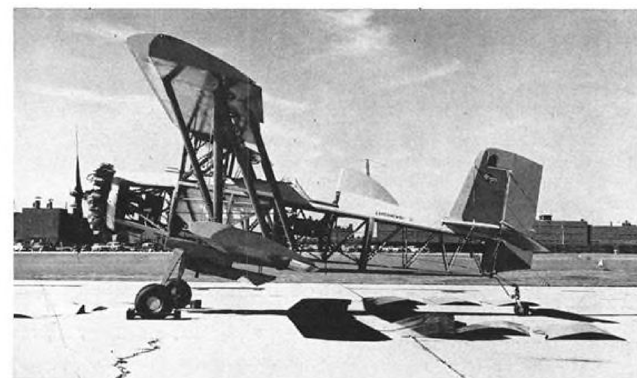
METAL panels can be quickly stripped for inspection of basic structure.
