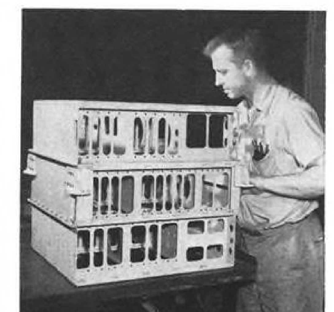
WEIGHT-SAVING magnesium frame for Titan computer, built from extrusions.
