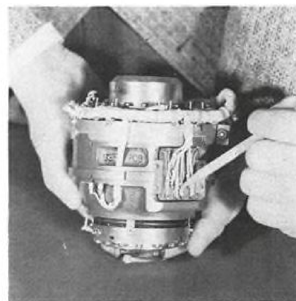
ACCELEROMETER is relatively simple, low-cost device; may employ vibrating reed.
