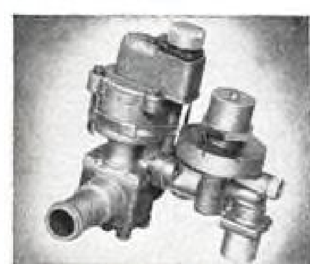
Hot air shut-off and pressure regulator; temperatures to 815°F; inlet pressure to 250 p.s.i.; outlet pressure range from 5-30 p.s.i.g. \pm 1/2 p.s.i.
