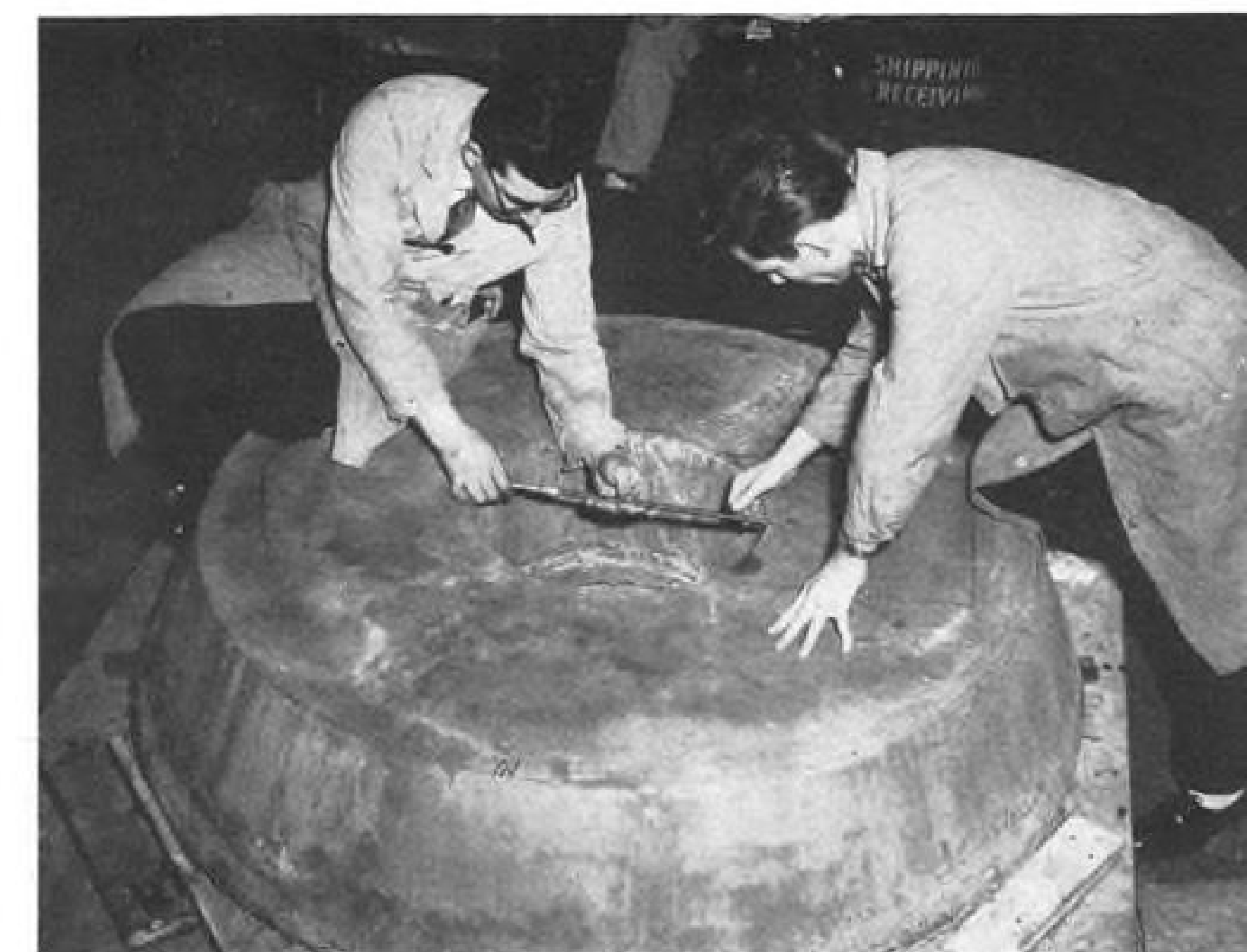
CONCENTRIC rings (left) were cut from large beryllium ingot (right) by Avco experimental manufacturing group as part of its effort to develop fabricating techniques for making beryllium nose cones. Avco is working on research and development of the Titan nose cone.
