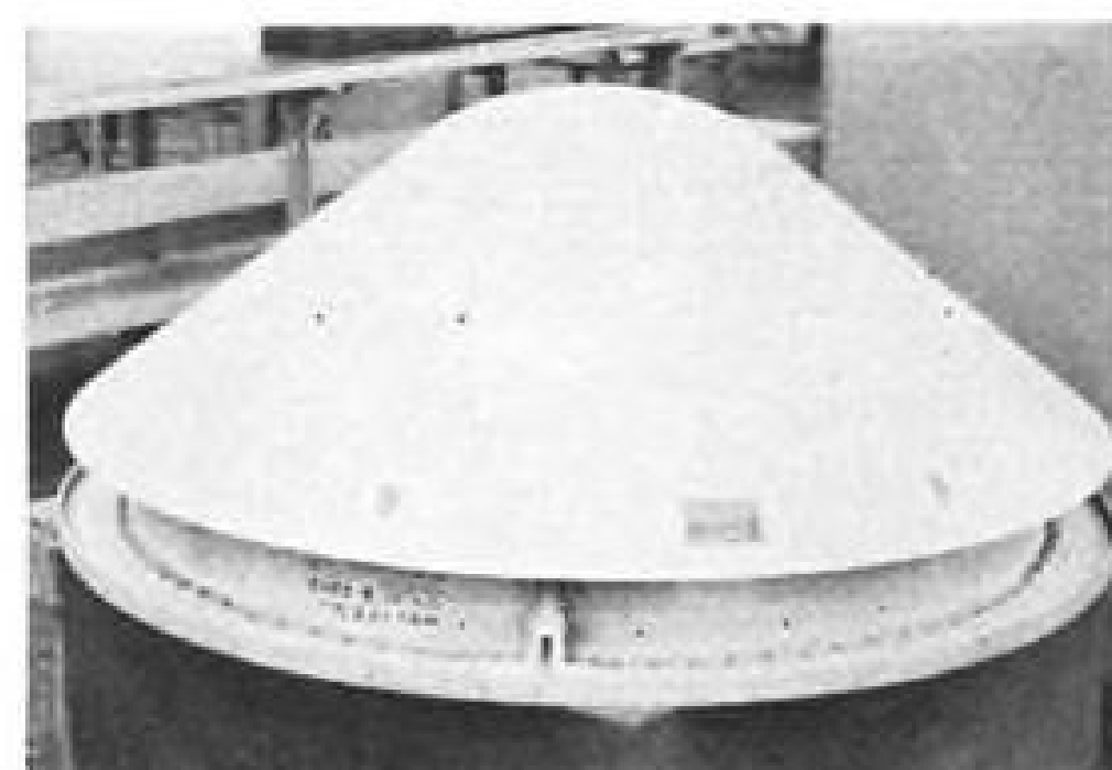
NOSE CONE (above) and afterbody (left) for Thor and Atlas re-entry vehicles were displayed at Republic (AW May 5, p. 29). Nose cone is blunt, copper-based, heat-absorbing structure. Cone liner inside extends below heat shield. Afterbody is hidden from view inside missile until after separation.
