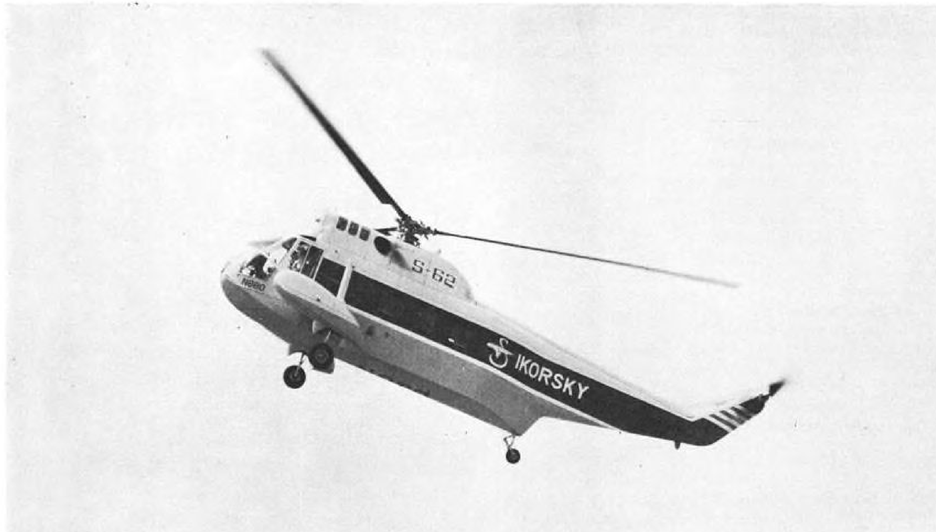
FIRST SIKORSKY S-62 amphibious helicopter is powered by a single General Electric T58 gas turbine engine rated at 1,050 shp.
