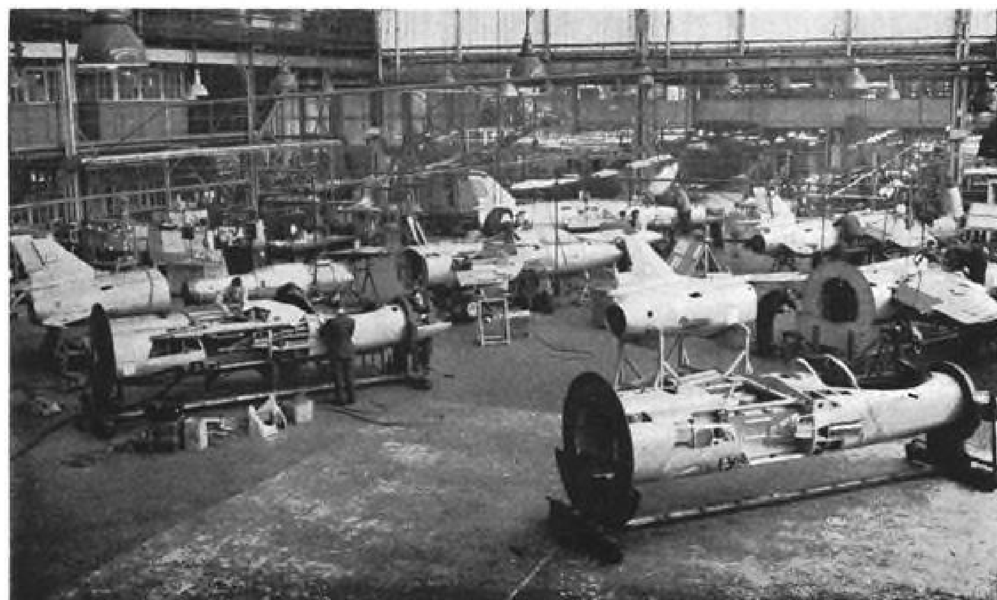
MOST of Folland Gnat can be reached from ground in final assembly at Hamble, Hampshire. In earlier assembly stages, entire front and center fuselage are rotated in jig for access.
