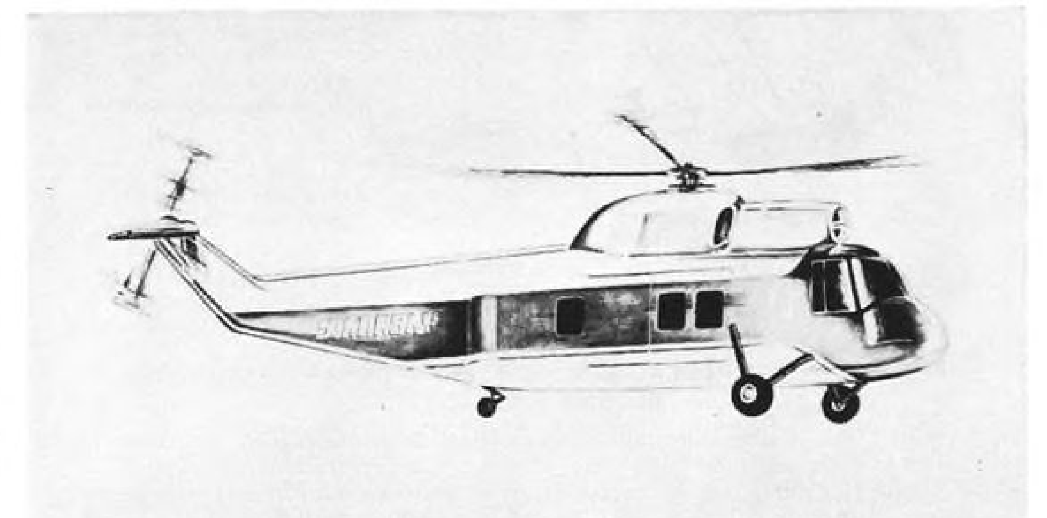
THREE fixed-wheel land version of Sikorsky S-62 would be designed for air transportability.
