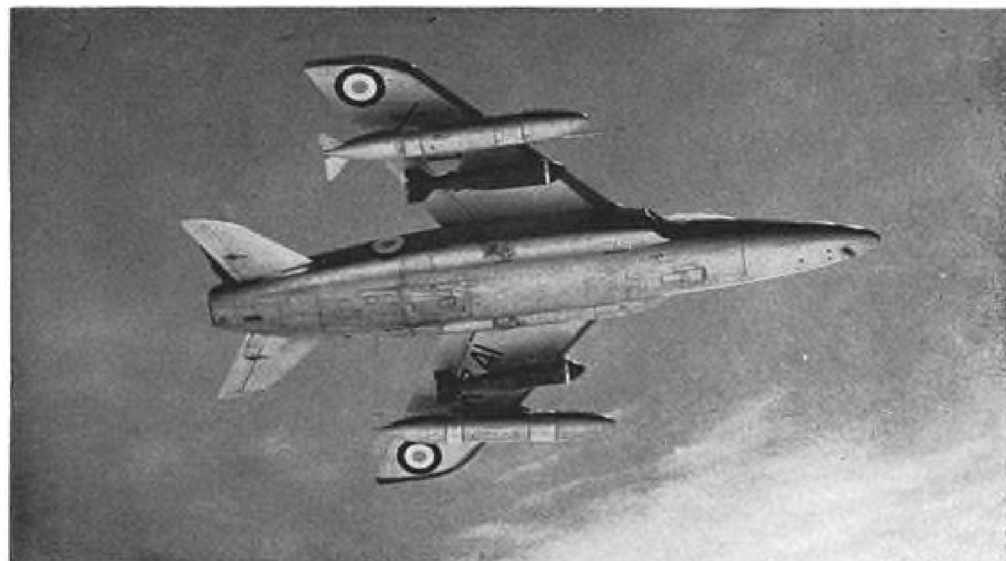
FOLLAND Gnat XK.741, used by Ministry of Supply for flight development, is carrying two 500 lb. bombs and two 66 gal. drop tanks. Tanks have proved buffet-free to Mach 1.
