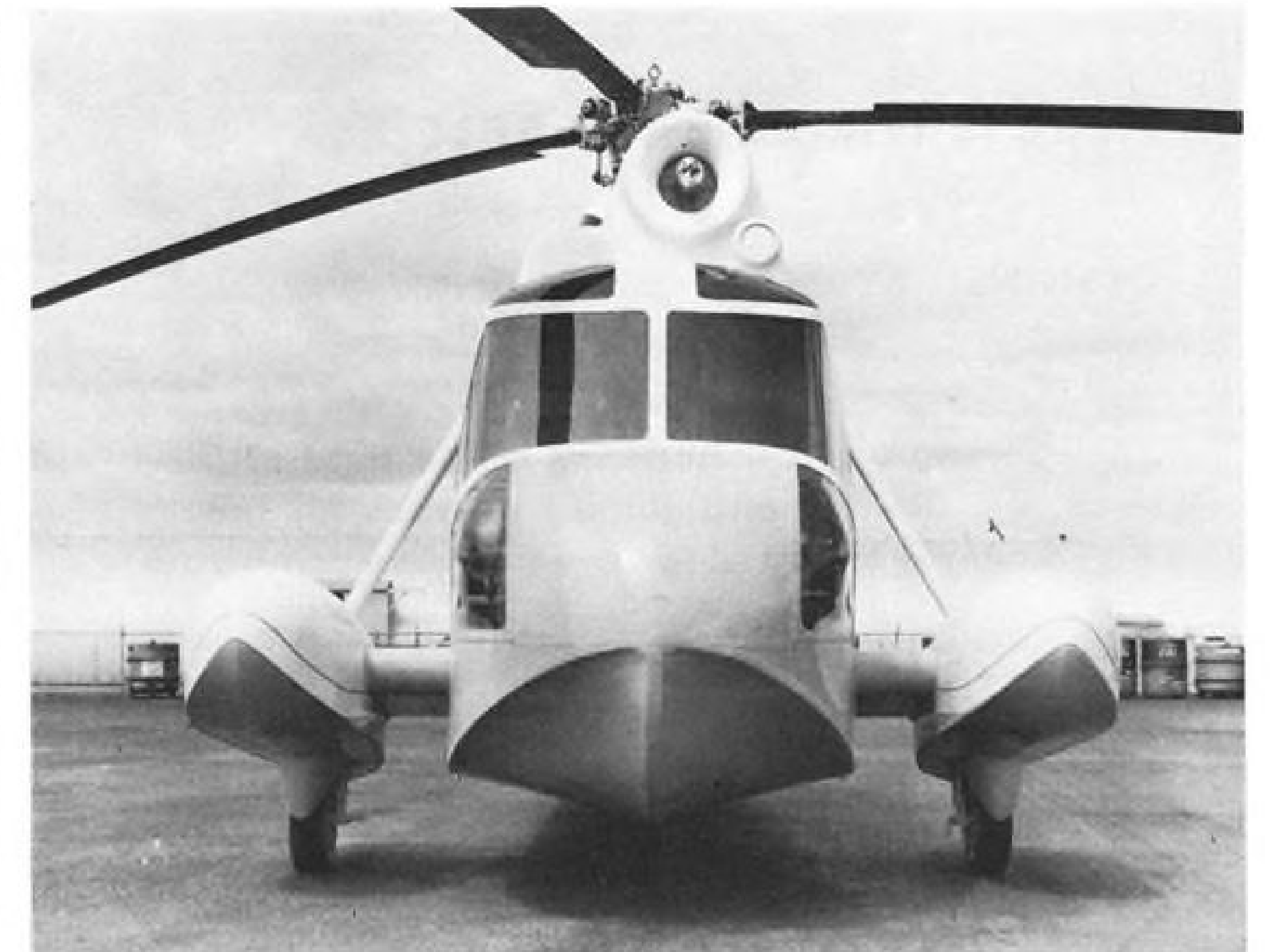
V-BOTTOM of S-62 fuselage is designed to cushion impact when settling on water. It also directs spray outward and down. Floats house landing gear and resist pitching and rolling.
