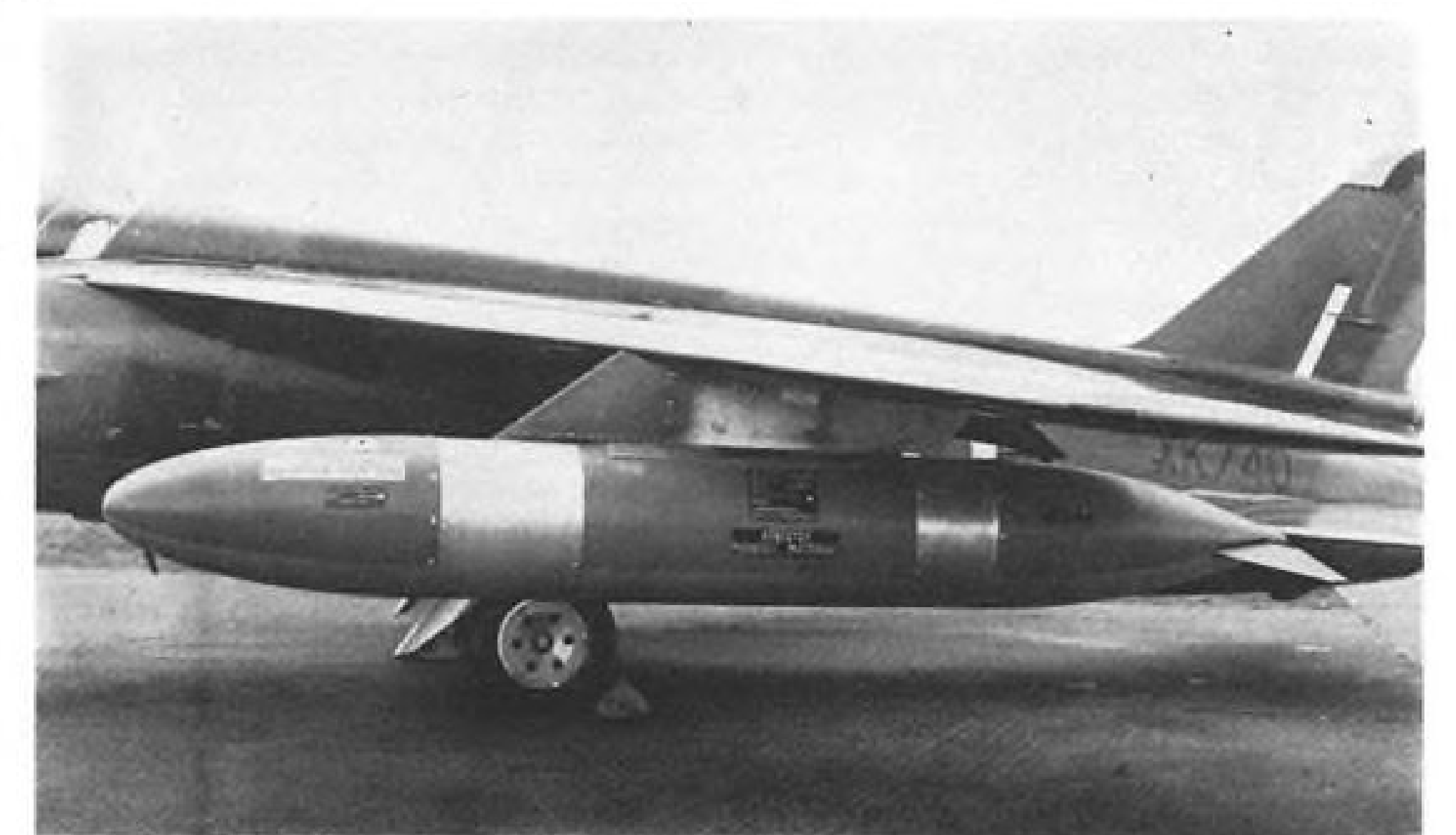
DROP tank above will be used on all production Folland Gnats. Tank is a conversion of an original Bristol 50 gal. asbestos phenolic tank. The inserted metal sections raise its capacity to 66 gallons.
