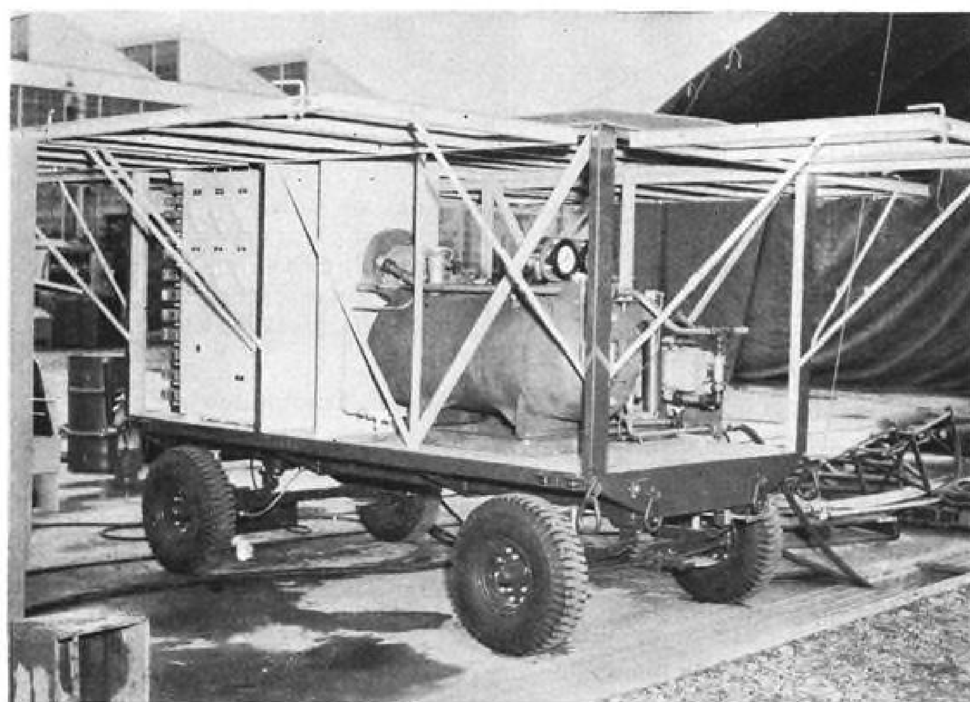
HYDRAULIC power unit supplies power for erecting Thor and for moving unbilical mast.
