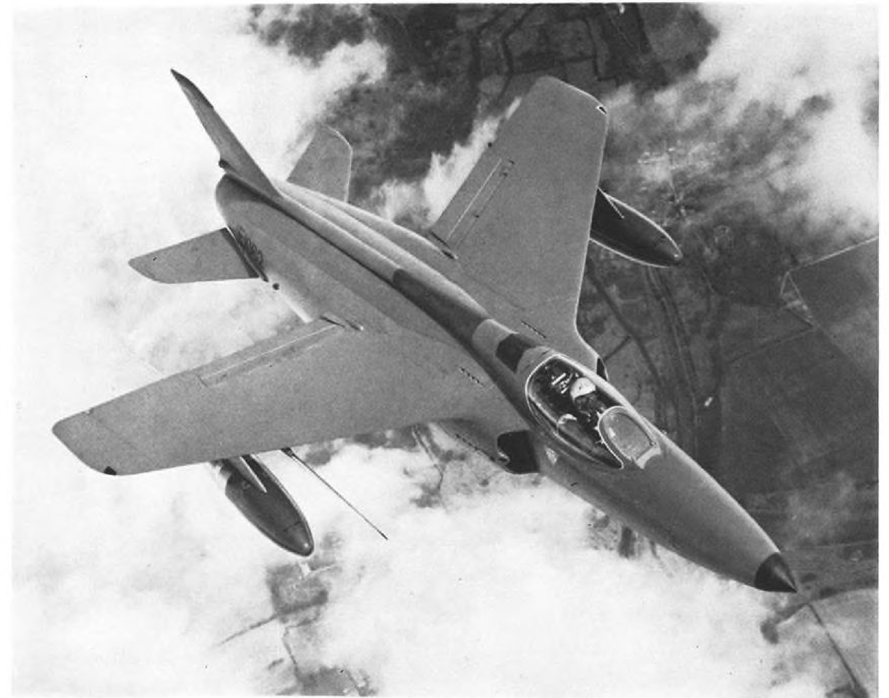
PRODUCTION model of Folland Mk.1 Gnat is earmarked for India. Fighter, powered by Bristol Orpheus 701 turbojet (4,850 lb. thrust), has dielectric nose cone containing radar, and two dielectric panels in dorsal spine for radio compass loop (fore) and sense aerials (aft).
