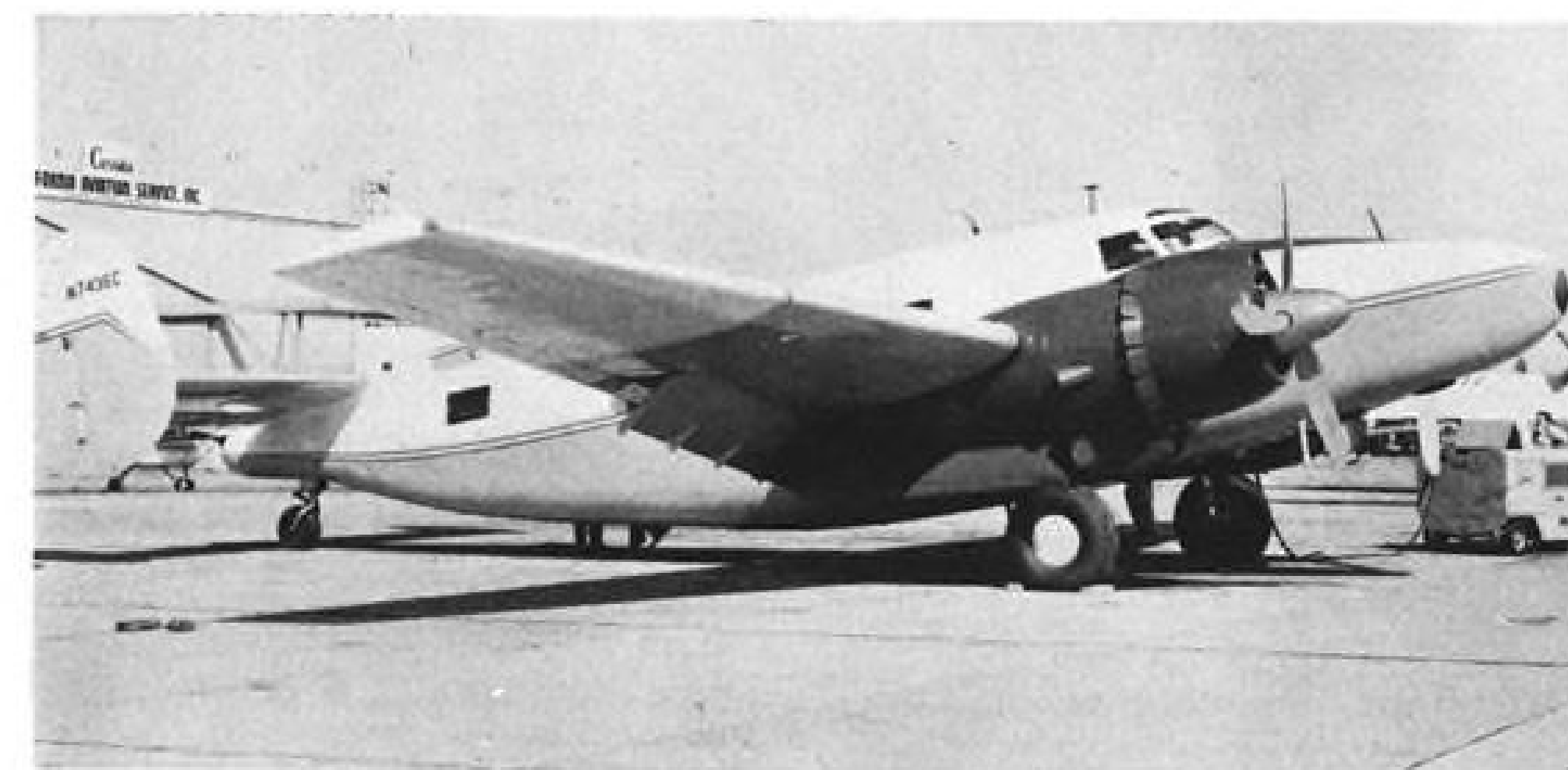
PROTOTYPE Centaurus, World War II patrol bomber modified for executive transport, has extended nose to provide space for radar installation. Formerly PV-2 Harpoon, aircraft can be pressurized if desired, cruises at 280 mph. at 10,000 ft., has 2,000-mi.-plus range.
