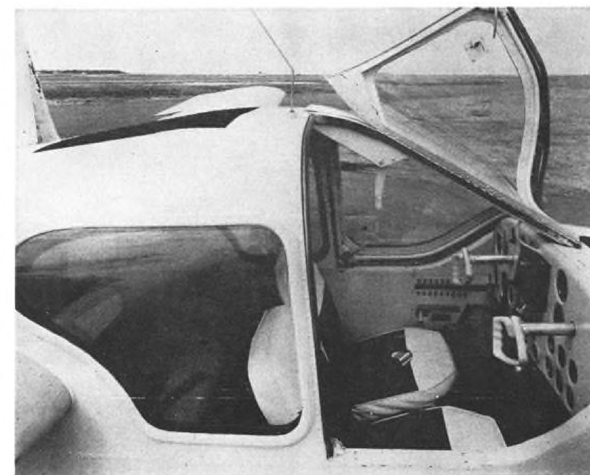
HINGED and watertight windshield folds over from either side; bow accessories are within easy reach. Cabin is 47 in. high, 44.5 in. wide and 62.5 in. long.
