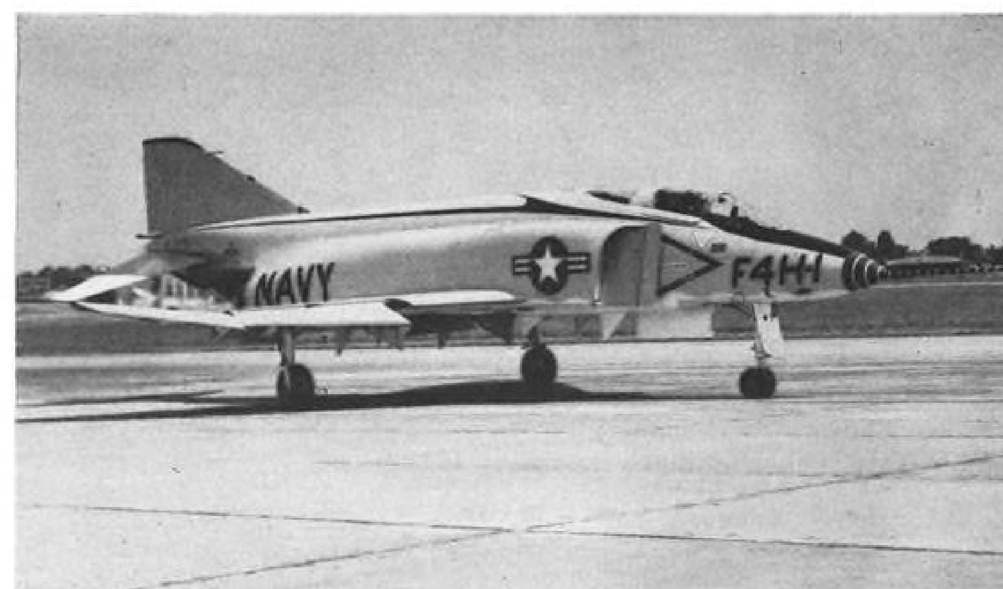
SPARROW III missile, geometry control inlet hinge can be seen in this F4H-1 runway view.
