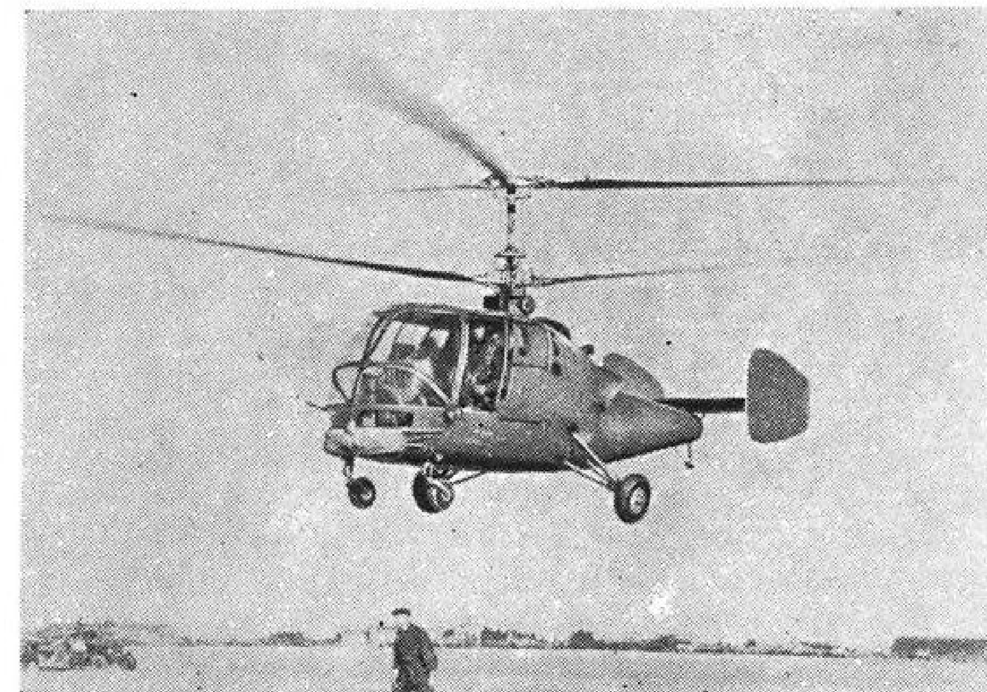
COAXIAL Kamov Ka-15 helicopter is powered by 255 hp. engine, has top speed of 93 mph.
