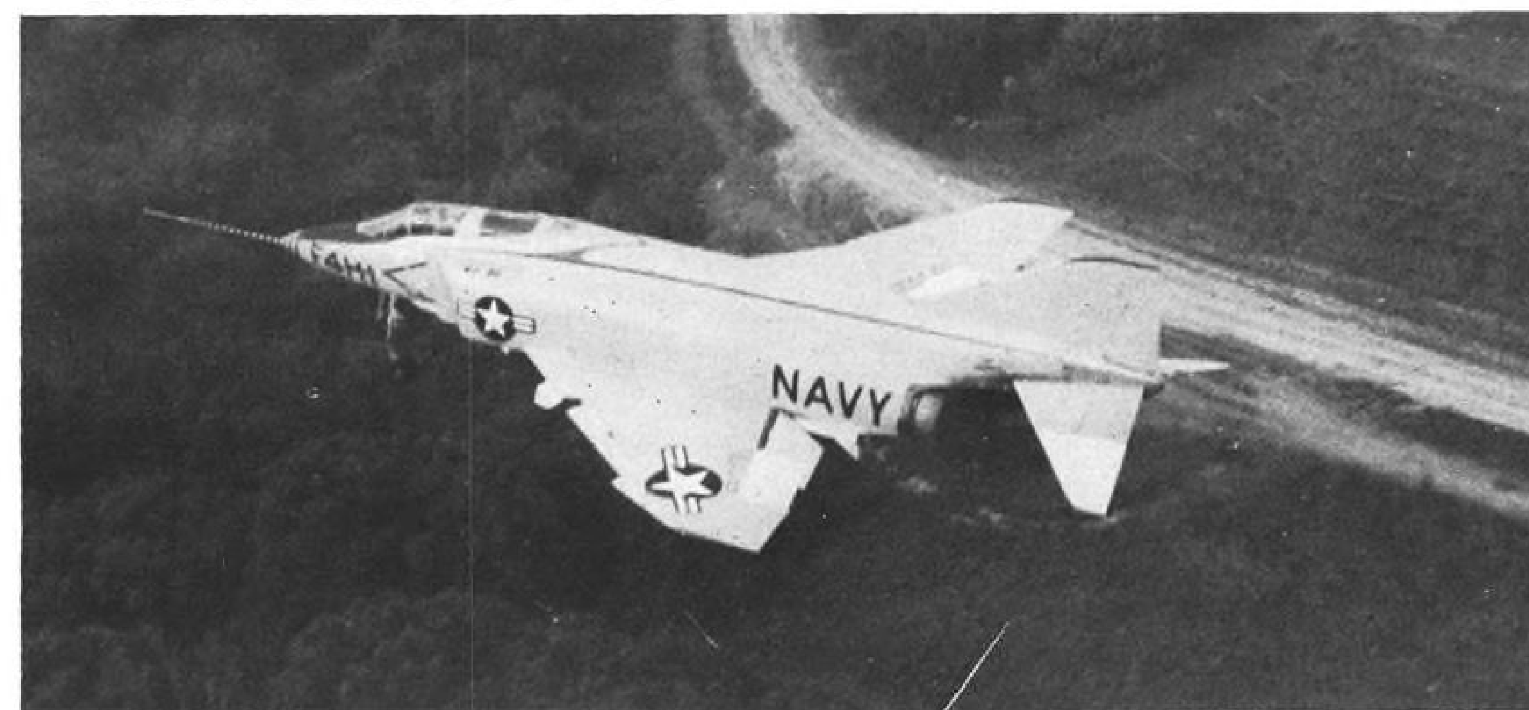
FLIGHT view of McDonnell F4H-1 shows aircraft in traffic pattern, gear and flaps down. Note extended droop in horizontal tail.
