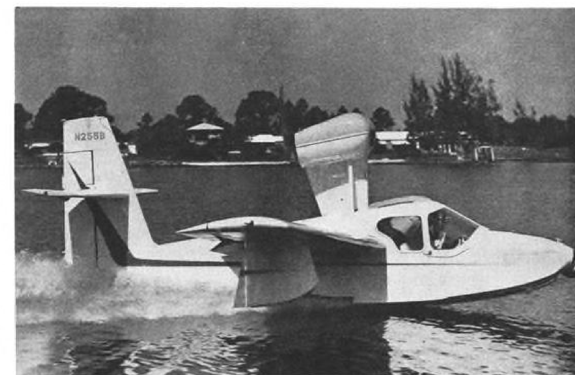
AMPHIBIAN'S float bumpers and wing tips are plastic; nosewheel acts as buffer.
