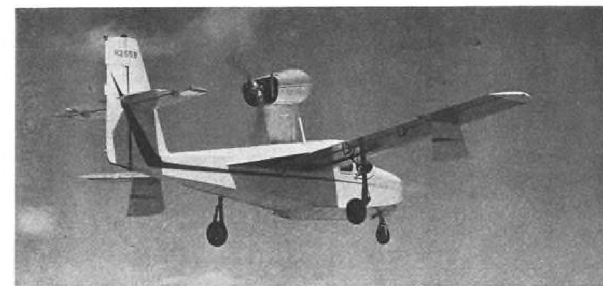
C-2 gear, with long oleo travel, is weldment of 4130 steel; tread is 11 ft. 2 in.
