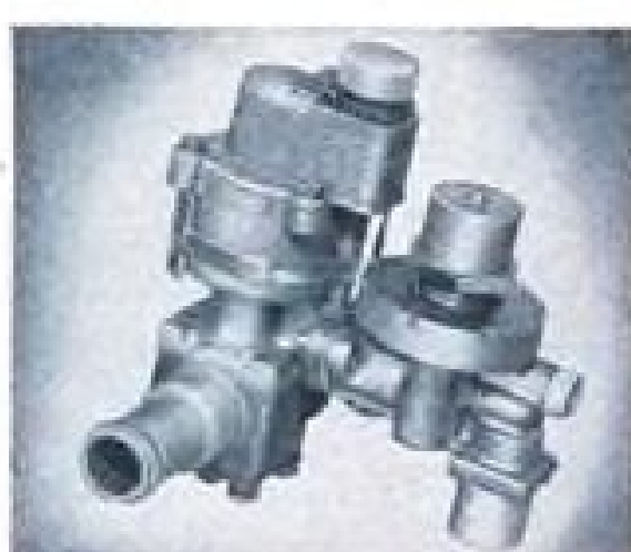
Hot air shut-off and pressure regulator; temperatures to 815°F; inlet pressure to 250 p.s.i.; outlet pressure range from 5-30 p.s.i.g. ±1/2 p.s.i.
