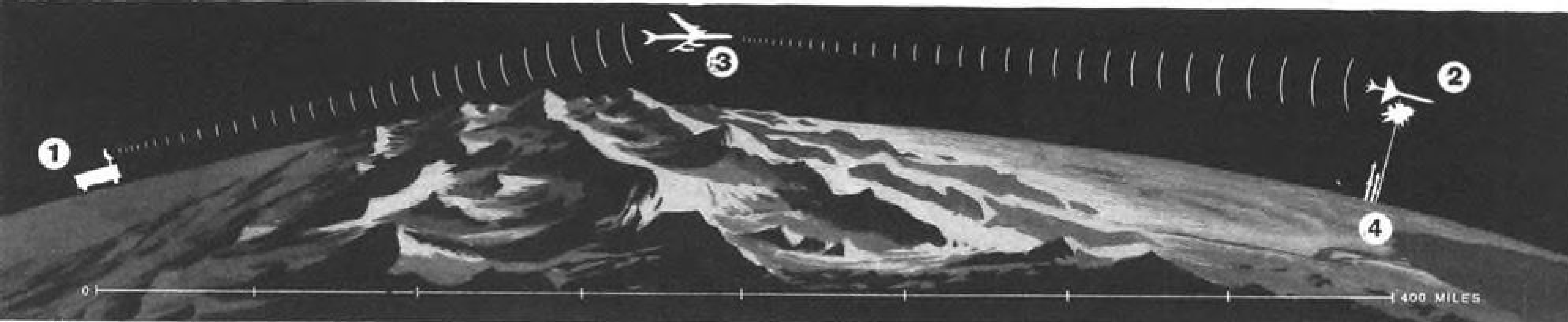
GREAT RANGE of Sperry microwave command guidance system is shown in diagram. Ground station (1) controls target drone (2) either directly
