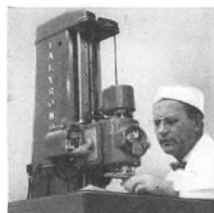
The Talyrond, a super-accurate measuring device, is used by Barden as a development tool; as a standard for correlation of other quality control instrumentation; as a gage for ultra-precise bearing parts. It measures roundness and waviness to five millionths of an inch.
