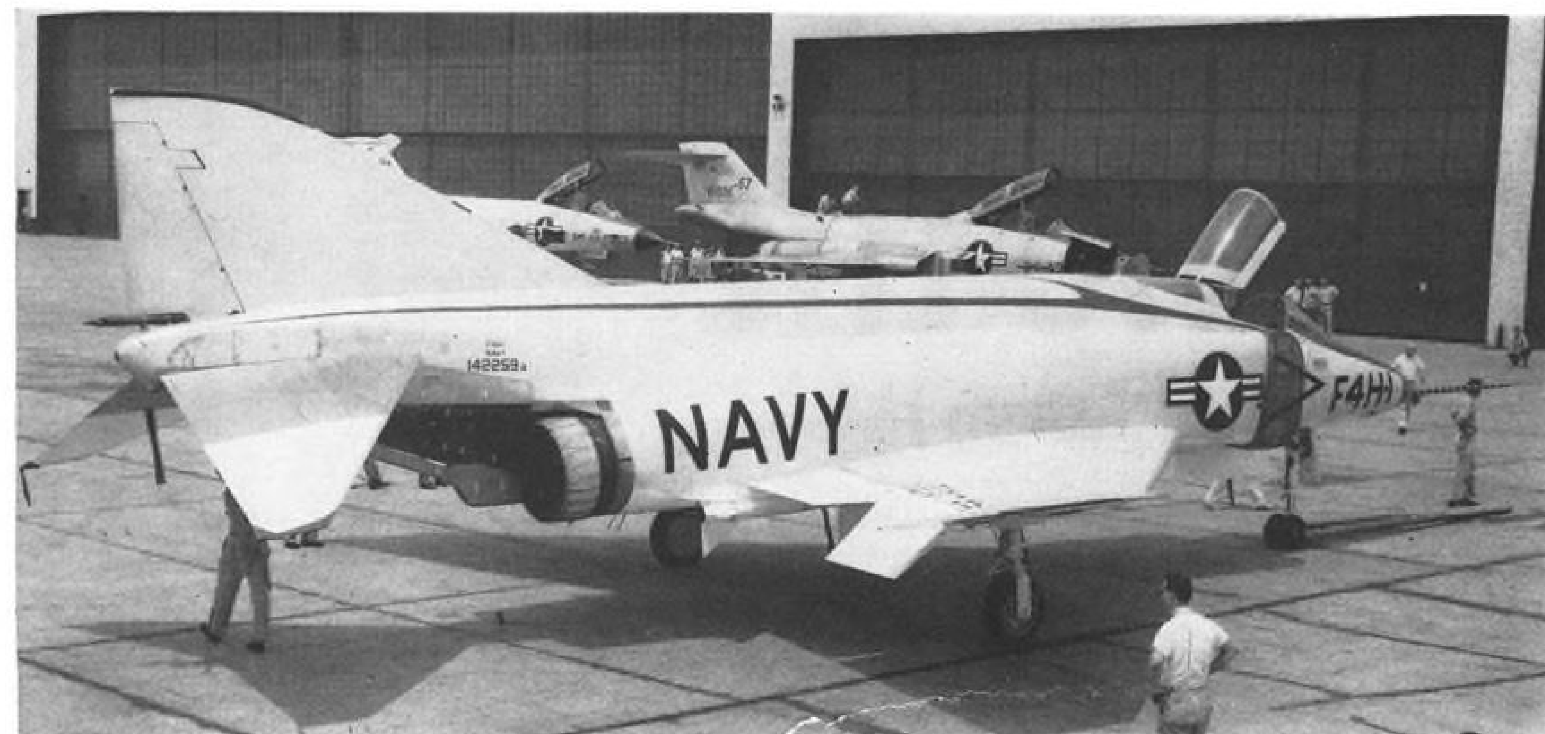
HOW F4H-1, which has an engine mounting layout similar to the USAF F-101, differs from the USAF airplane is indicated below. F4H-1 has enlarged vertical tail for improved high speed control, and horizontal tail has negative dihedral. Check inlets also differ. Parabrake for F4H-1 is in tail cone.
