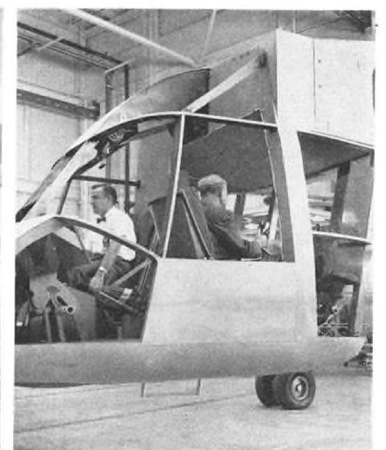
PILOT'S SEAT SWIVELS 180 deg. to provide him with optimum view while flying S-60 or manipulating crane's hoist. Separate sets of controls are provided for either operation. In the seat swiveled rearward is Sikorsky engineering manager Michael E. Gluhareff.
