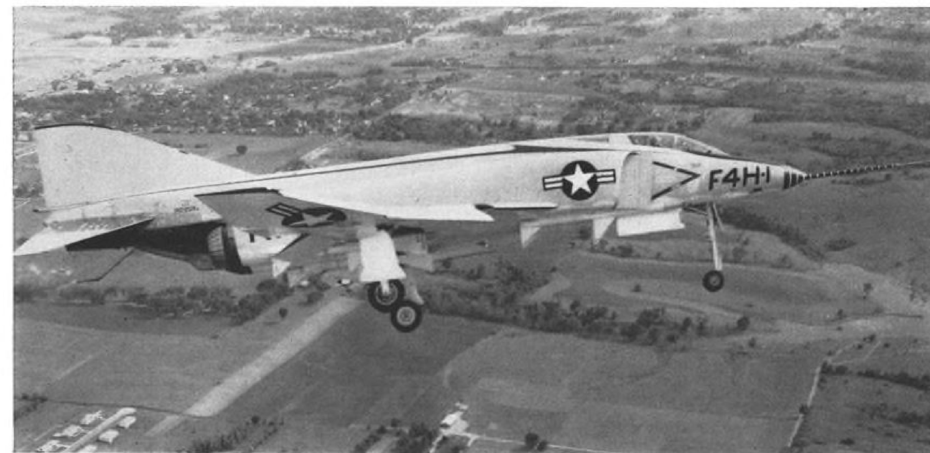
HOW F4H-1, which has an engine mounting layout similar to the USAF F-101, differs from the USAF airplane is indicated below. F4H-1 has enlarged vertical tail for improved high speed control, and horizontal tail has negative dihedral. Check inlets also differ. Parabrake for F4H-1 is in tail cone.
