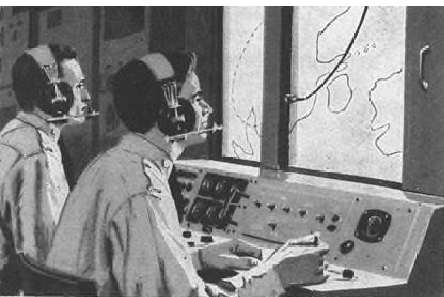
GROUND CONTROL of target drone centers in air-portable van. Men at console maintain control through flight instruments. Path of drone is traced automatically on plotting board at right.
