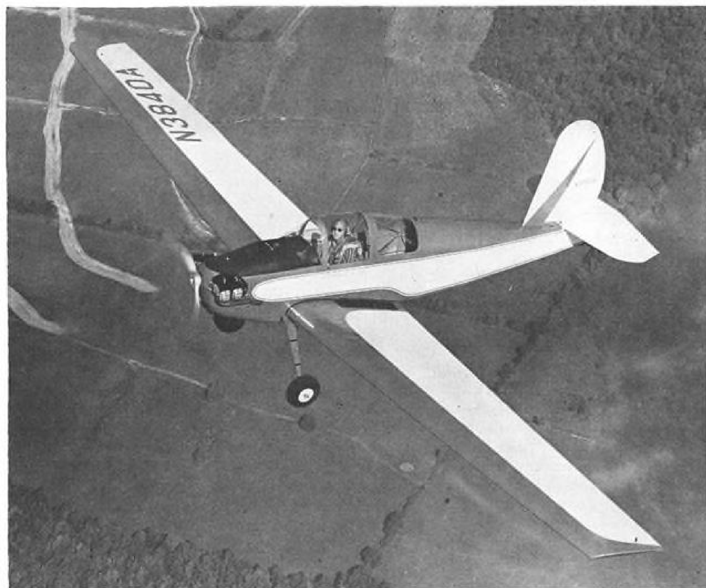
EXPERIMENTAL Schweizer 1-30 has Continental A65-12 engine generating 65 hp.
