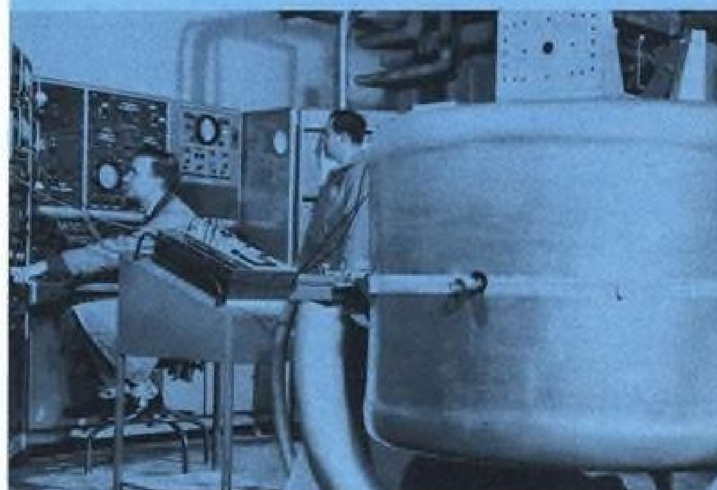
Vibration testing of missile component. Such tests duplicate inflight environments that components undergo when missiles are fired.
