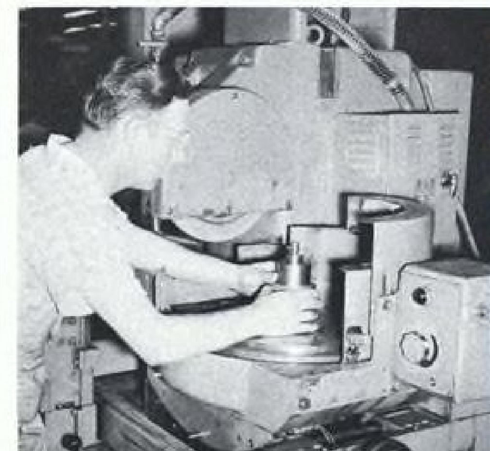
Technician grinds gyro part to a length within 20 millionths of an inch—typical of tolerances being met in missile work at Ford Instrument.
