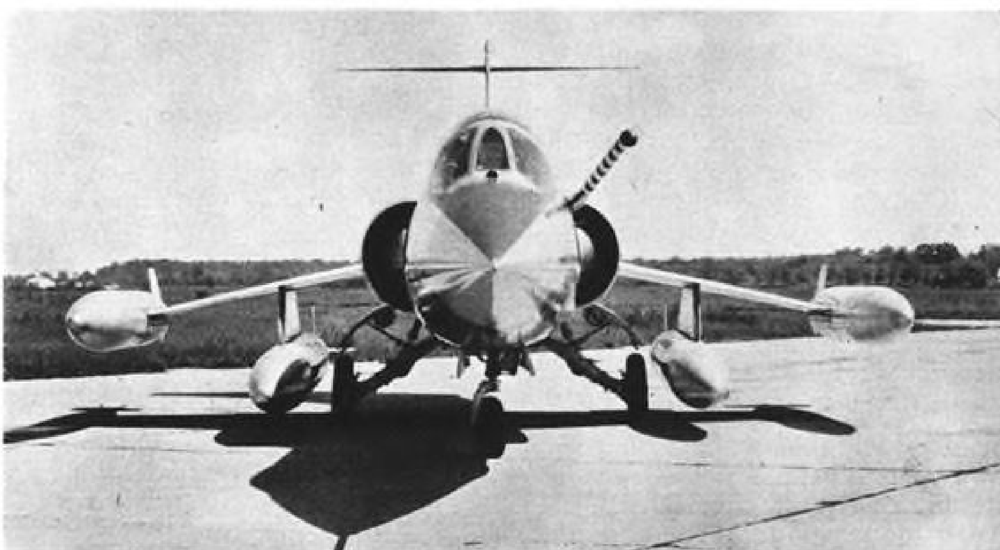
F-104's standard external fuel stores are 195-gal. pylon tanks and 170-gal. wingtip tanks.
