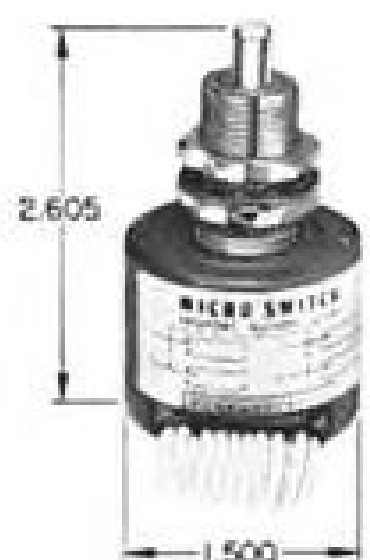
A 4-pole DT assembly with four SPDT "SM" basic switches sealed in enclosure only 1 1/2" diameter.
