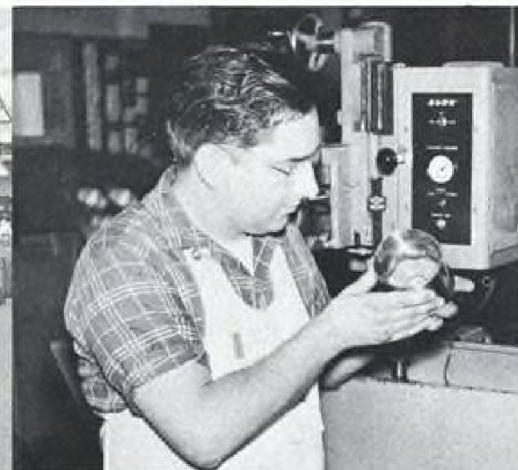
A special machine is used to mill irregular internal contours by an "electrical discharge" method, with extreme dimensional accuracy.
