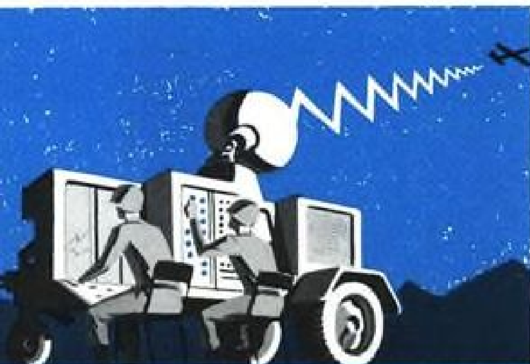
Drone control. Battlefield surveillance aircraft are remotely controlled by Ford Instrument system (radar, transmitting, computing and plotting equipment).
