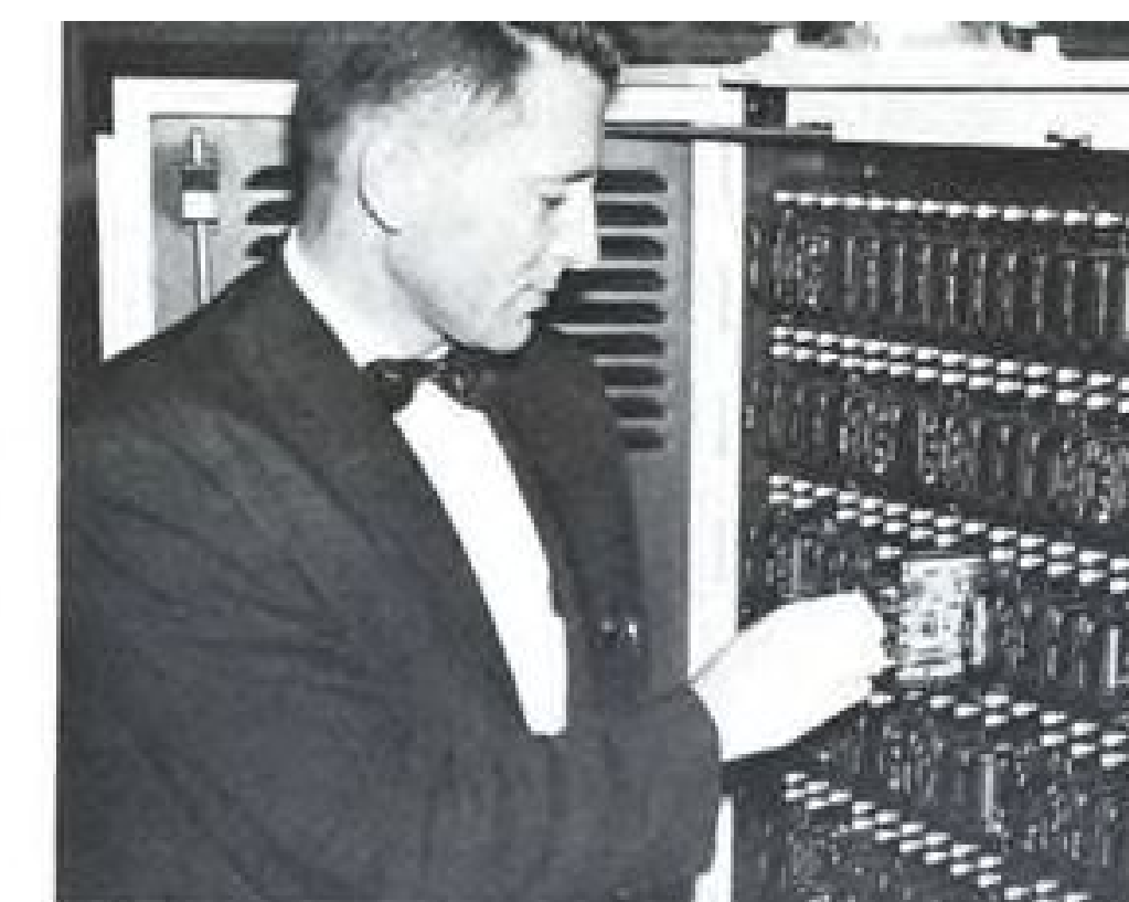
Launching and control order computers for TARTAR Missiles. Electronic and electromechanical portions of this all-transistorized modular computer are shown at left and right.
