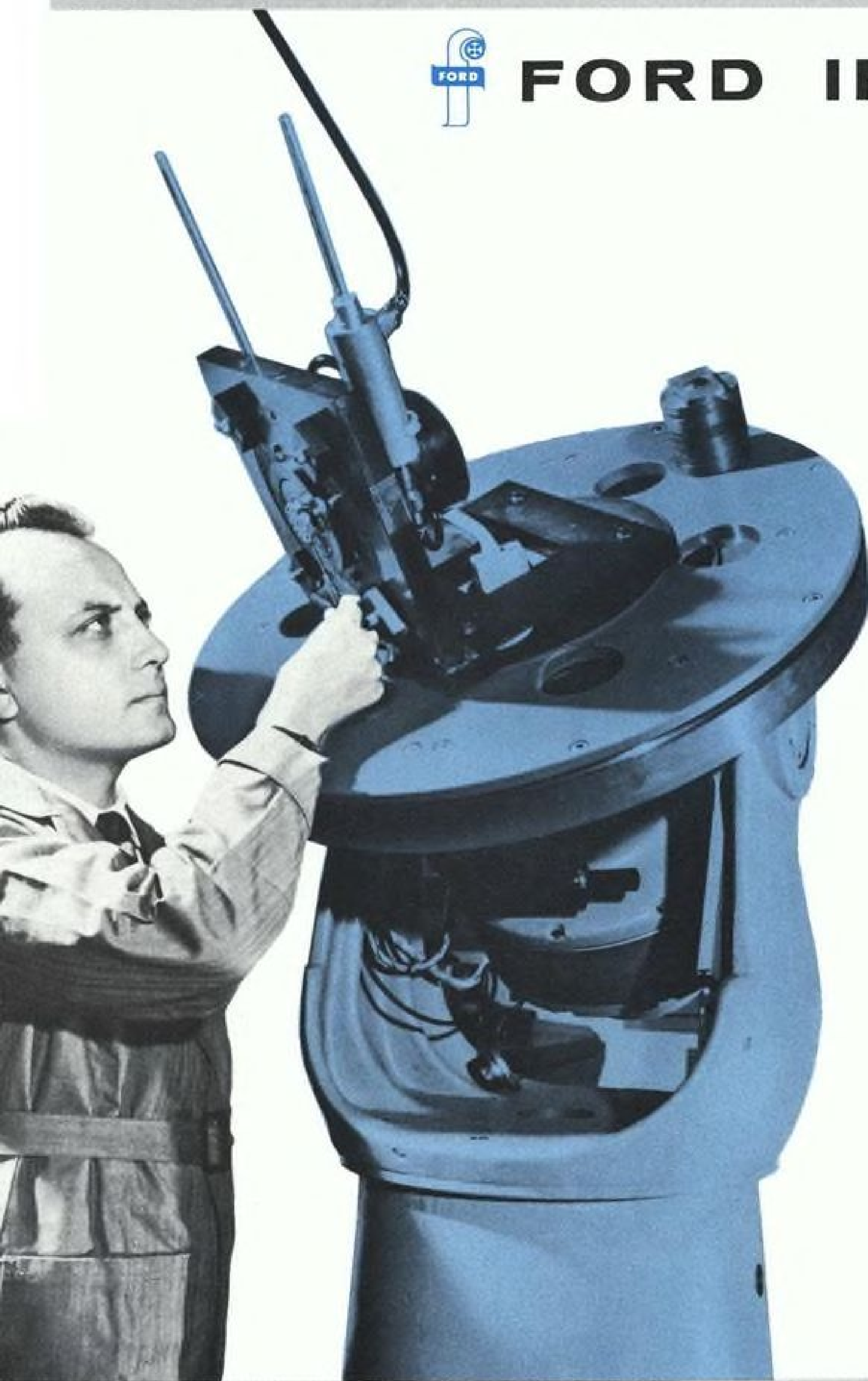
Equatorial test stand, built by Ford Instrument for its own laboratory facilities, is used for conducting basic drift error research. This type of unit can also be built to contractor order.
