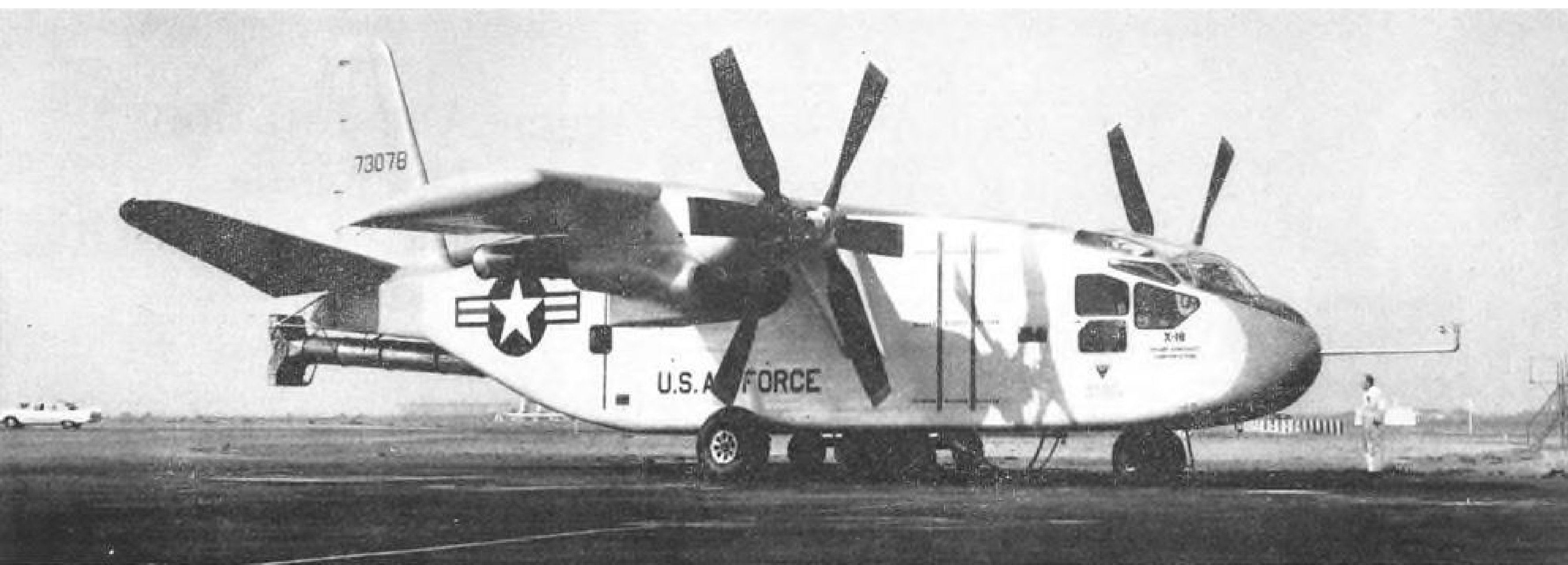
WING of Hiller X-18 vertical takeoff and landing aircraft is in position for horizontal flight; engines are two Allison T40 turboprops, producing 5,535 eshp. each. Engine in aft section is 3,400-lb. thrust Westinghouse J34 turbojet, used for pitch control.
