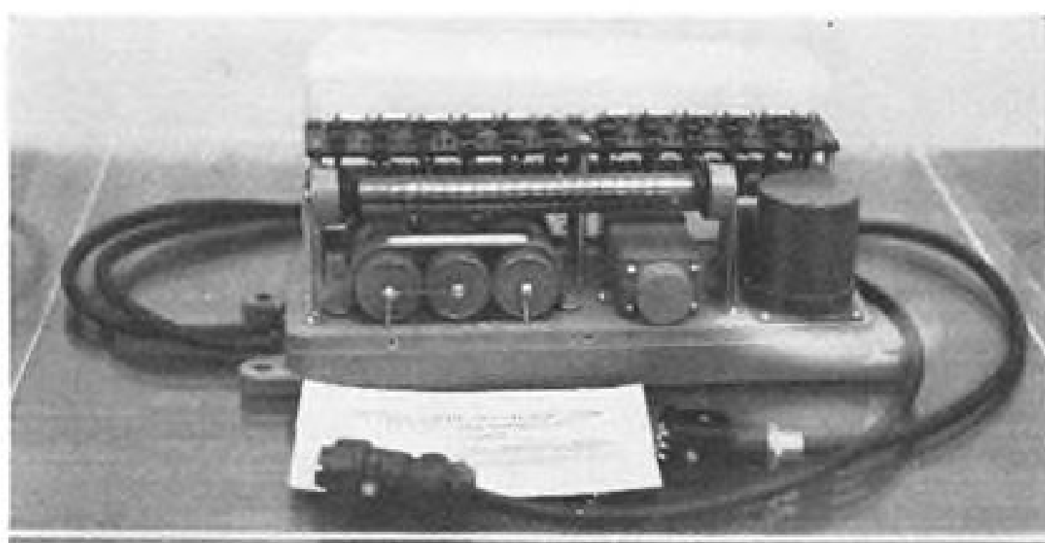
INSTRUMENT for probing composition of cosmic rays (above) permits measurement of atomic nuclei within the charge. Device to measure radiation (right) is connected to a silicon solar battery (circular instrument at far right).
