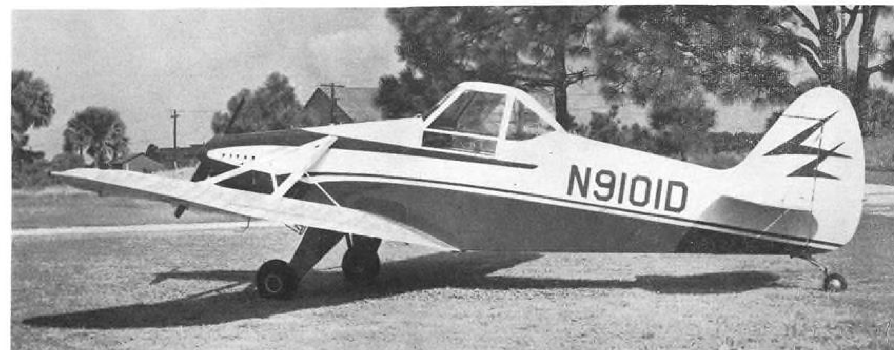
HIGH COCKPIT provides good visibility over sloping nose. Pawnee uses numerous Piper standard components to ease maintenance.
