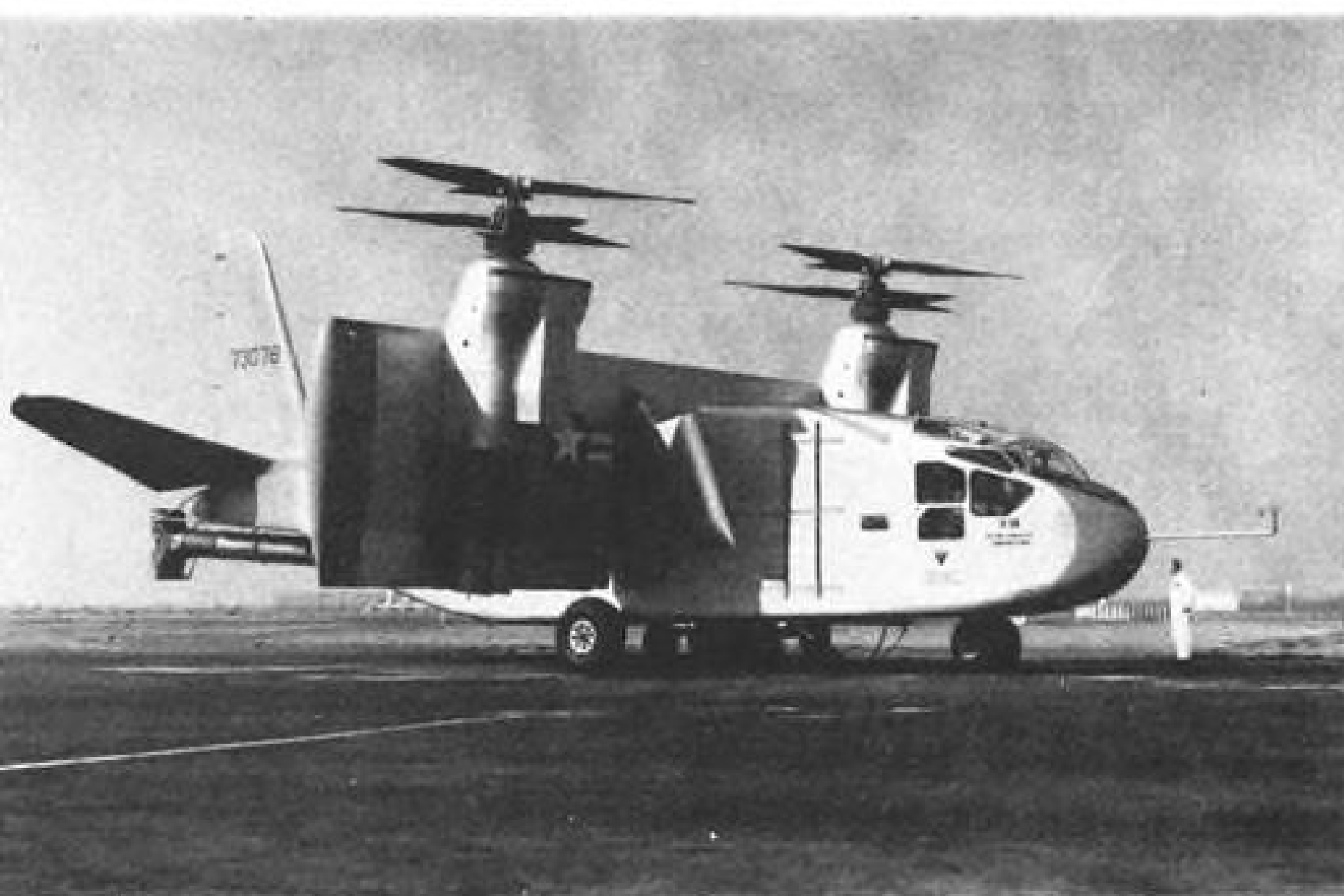
NOSE AND TAIL sections are adapted from Fairchild C-123 transport; note horizontal stabilizer dihedral. Propellers are dual-rotating Curtiss-Wright turboelectric unit from Navy Pogo VTOL program.
