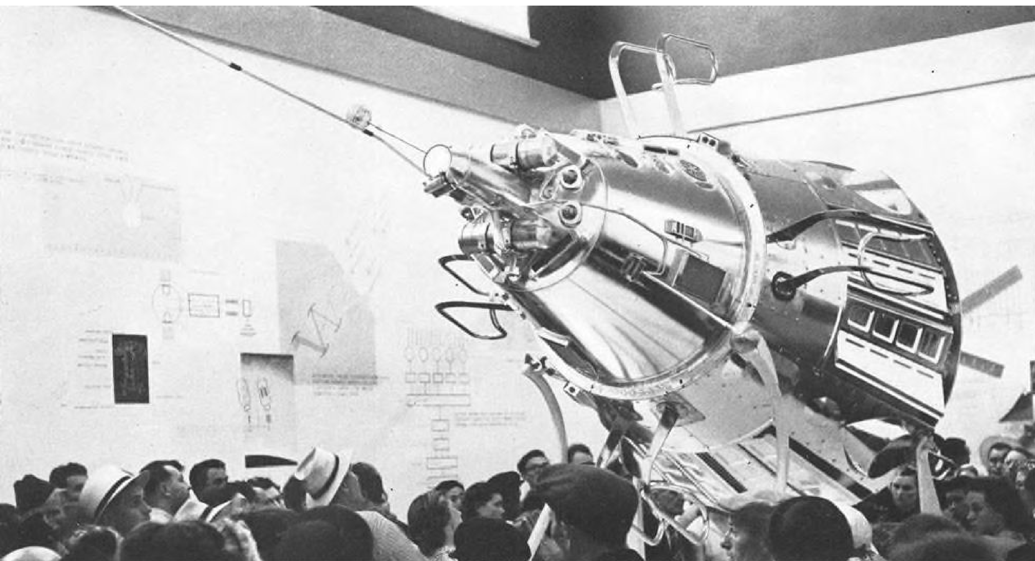
DOORS near conical base of Sputnik III, shown on industrial display at Moscow, swing outward or lie flat to change radiation coefficient and control internal temperatures. Ball microphones measure positive ion concentration. Large bent hooks in front are for telemetry use.
