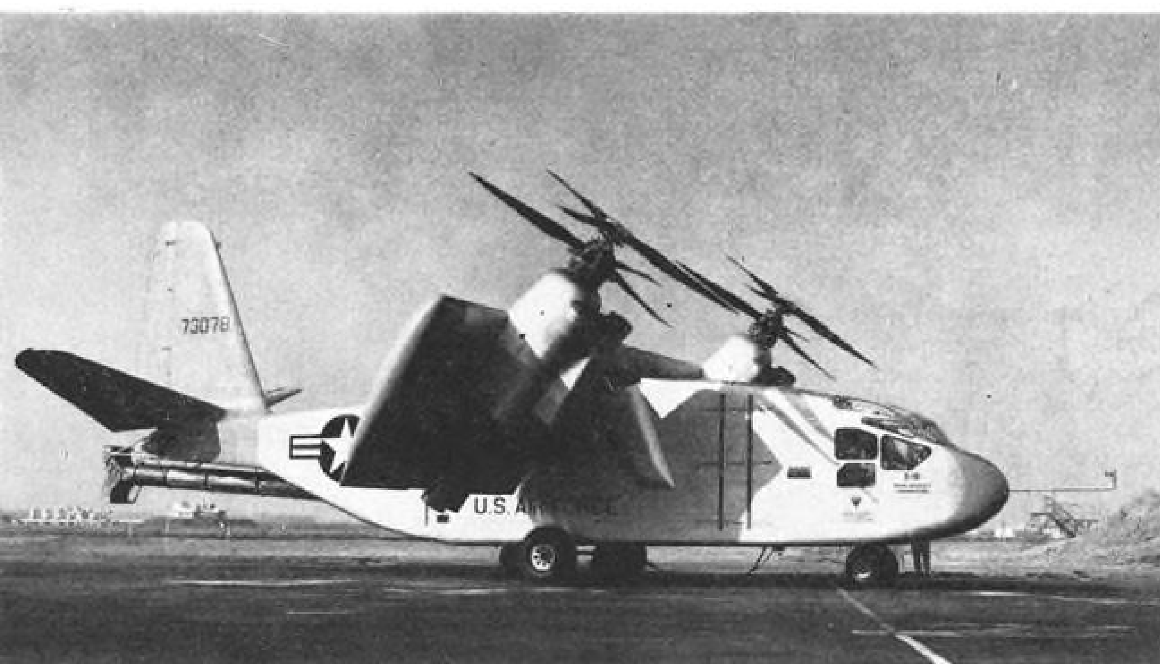
X-18 WING is in short takeoff and landing configuration. Company said the aircraft can clear a 50 ft. obstacle in 500 ft. with moderate overload in STOL uses.
