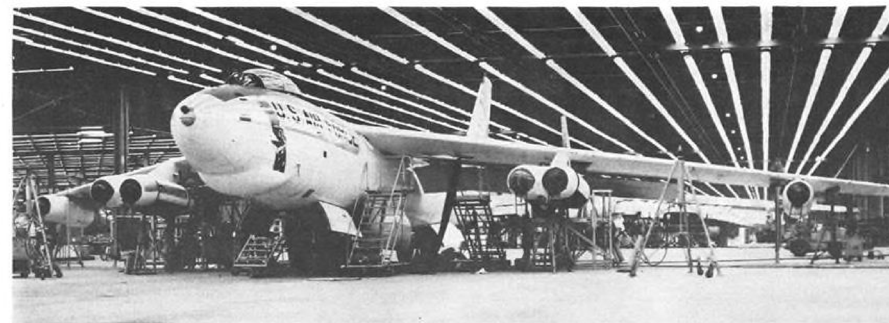
BOEING B-47 jet bomber is jacked up and optically aligned at Oklahoma Air Materiel Area hangar at Tinker Air Force Base, so that the wing is within 1/30,000th of an inch of its original configuration. The wing then is clamped in this position during the Project Milk Bottle modification program, to ensure that it will be in the proper placement when the modification kit is installed and the wing is reconnected to the fuselage. Modification shop is nearly a mile long.
