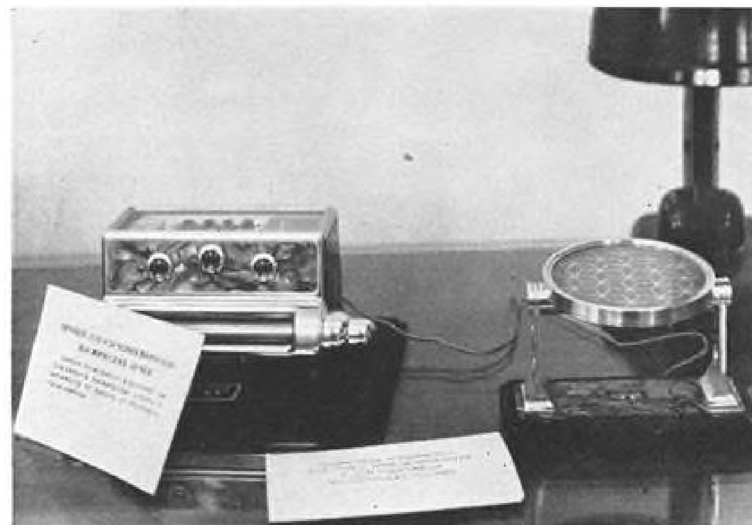
INSTRUMENT for probing composition of cosmic rays (above) permits measurement of atomic nuclei within the charge. Device to measure radiation (right) is connected to a silicon solar battery (circular instrument at far right).
