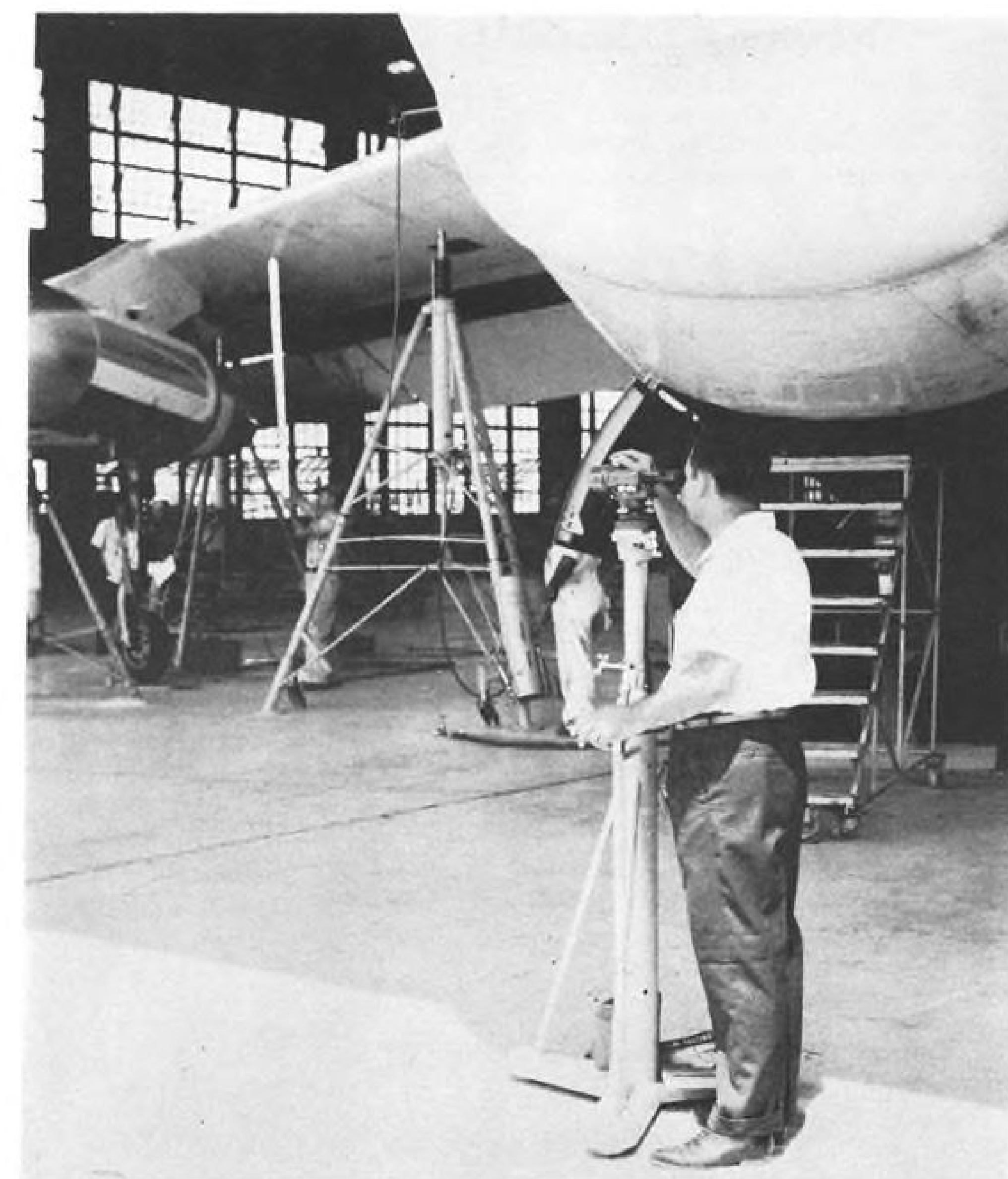
BALANCING the aircraft to high tolerances is part of preparation for the Project Milk Bottle modification program. Tinker's Ernest L. Rolland (above) uses optical device to check hydraulic jack positions. Modification kits were designed by Boeing Airplane Co. About 1,800 B-47s have been modified.
