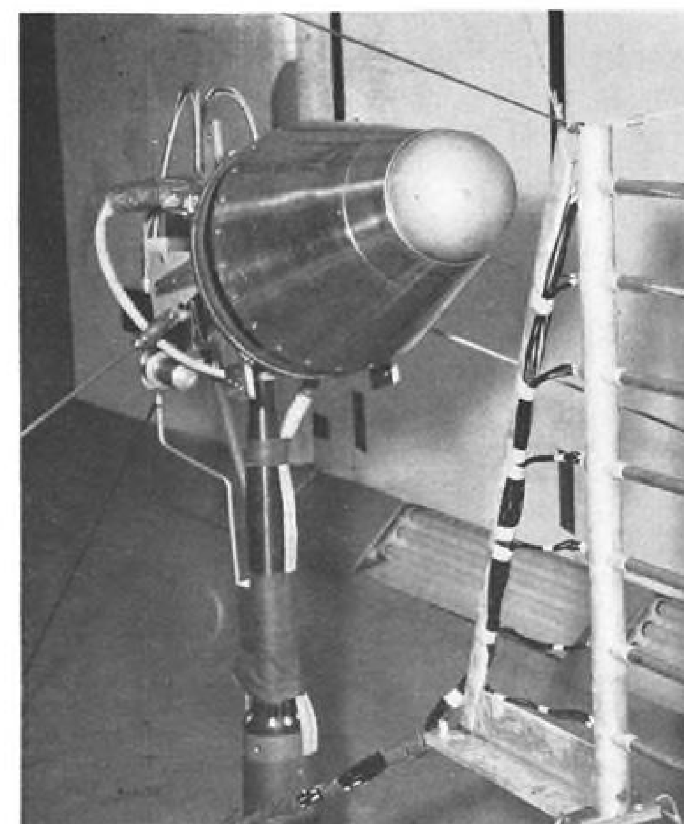
TOTAL impact pressure port on Q-Ball (left) is positioned directly into relative wind to pick off q at the stagnation point. Schlieren photo (right) shows Q-Ball at 16 deg. angle of attack at Mach 6.8; note slight secondary shock wave along lower edge of lip.
