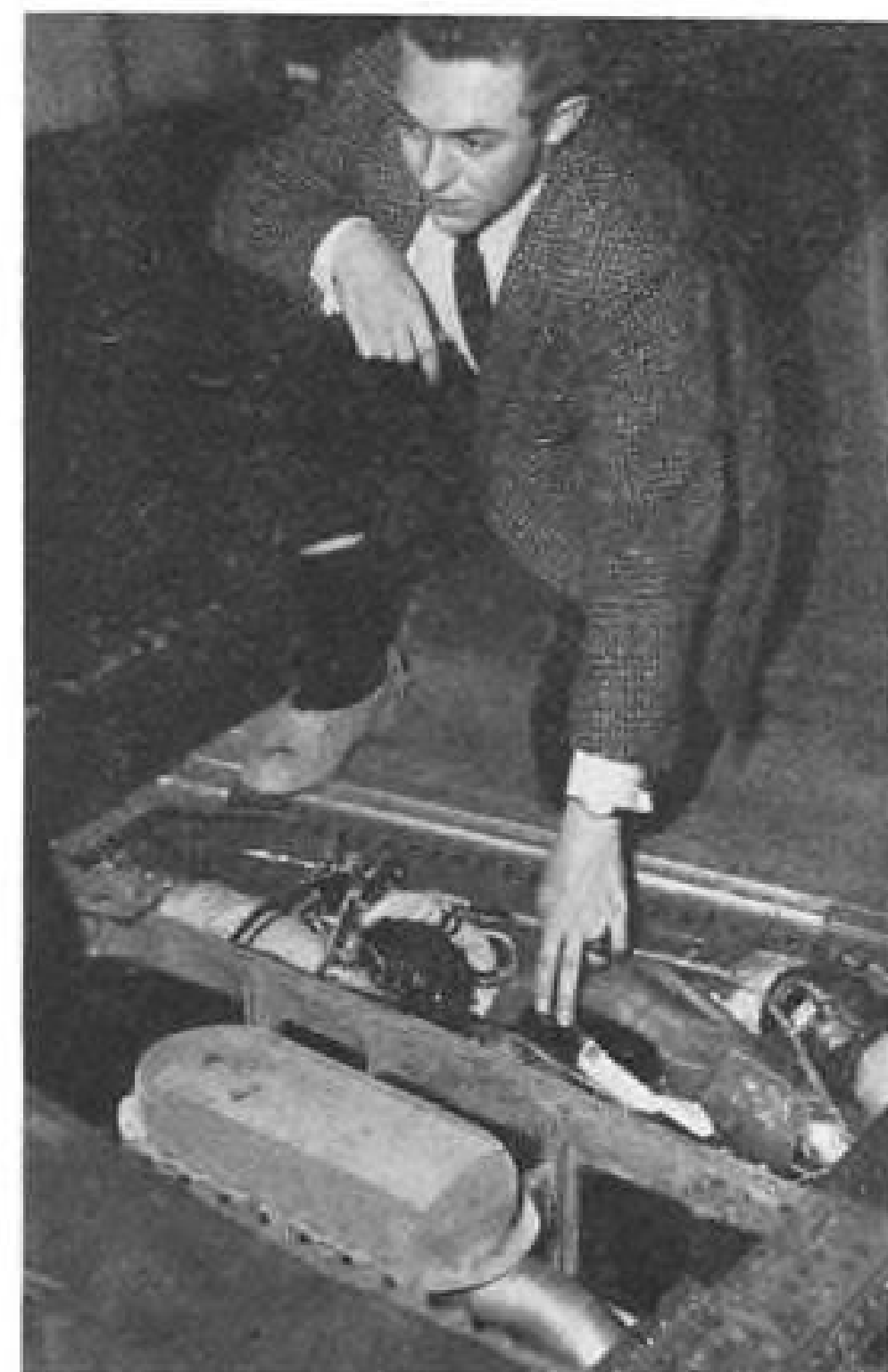
REMOVAL of upper wing panel over inboard engine exposes water boiler of B-58 air conditioning system.
