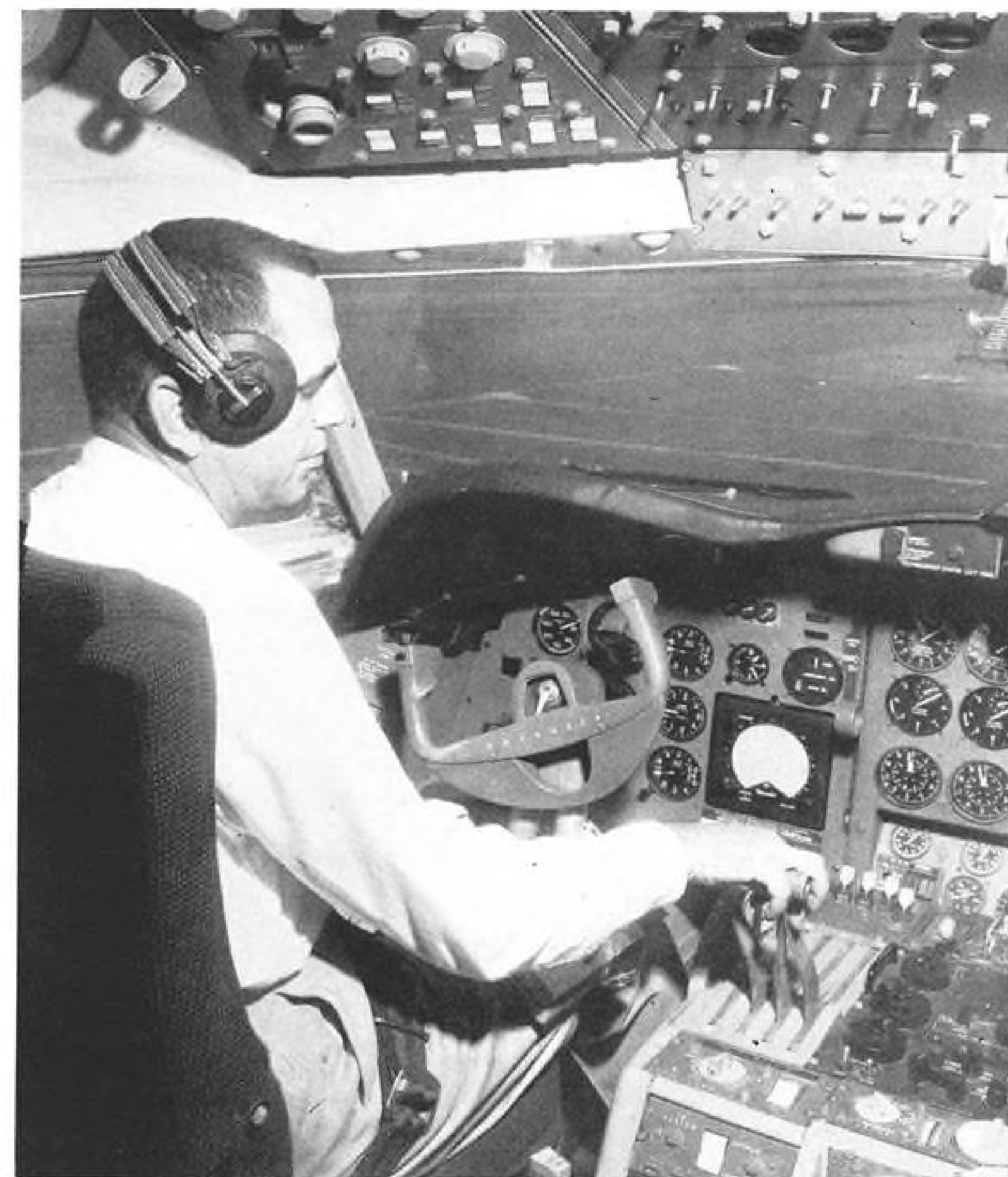
PRESTART checklist is run through in Electra cockpit by Aviation Week evaluation pilot Richard Sweeney. Instrument at right of pilot's panel is a radar scope.
