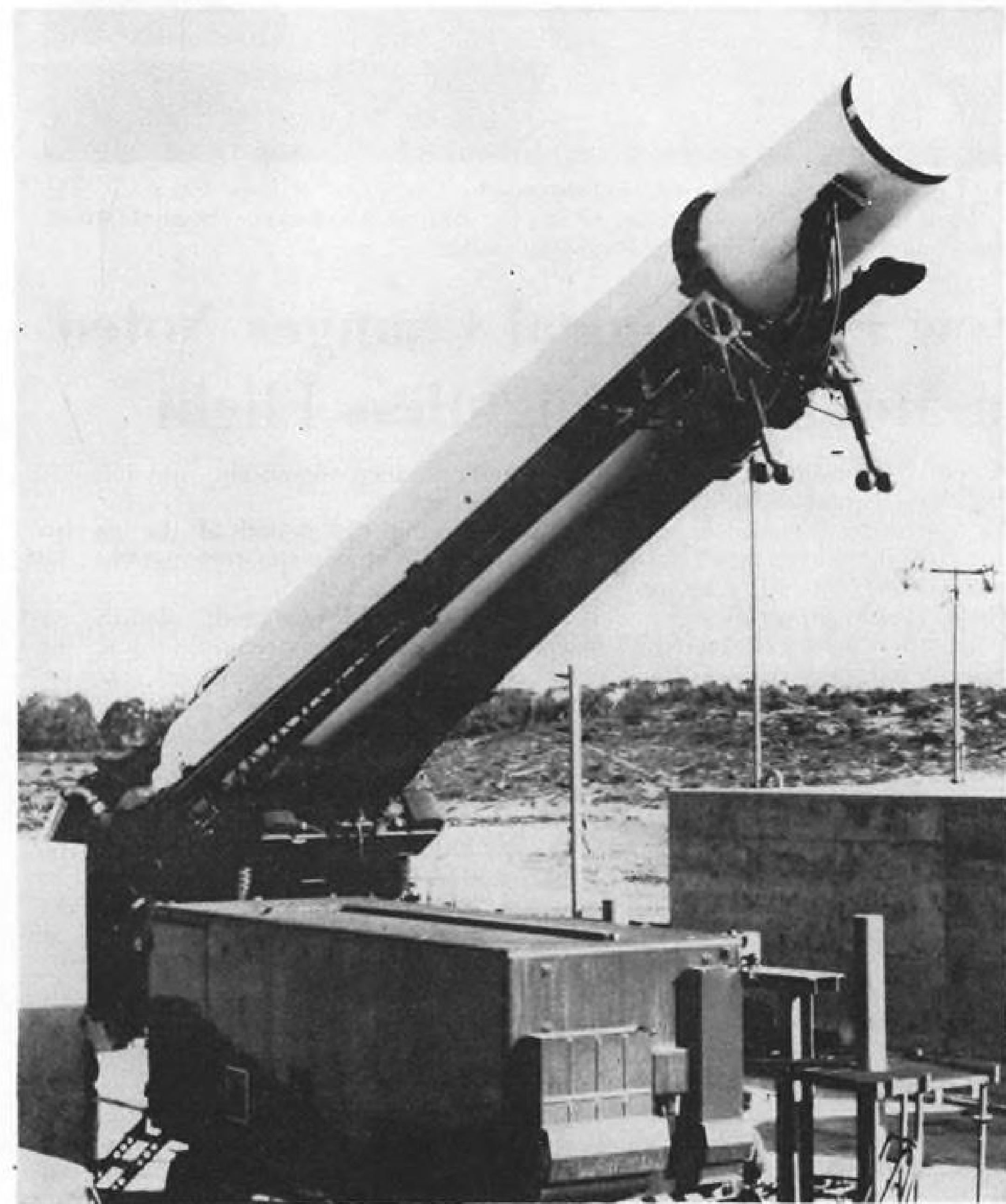
THOR intermediate range ballistic missile is raised half way to its launch position by a transporter erector in preparation for firing from Vandenberg AFB launch site.
