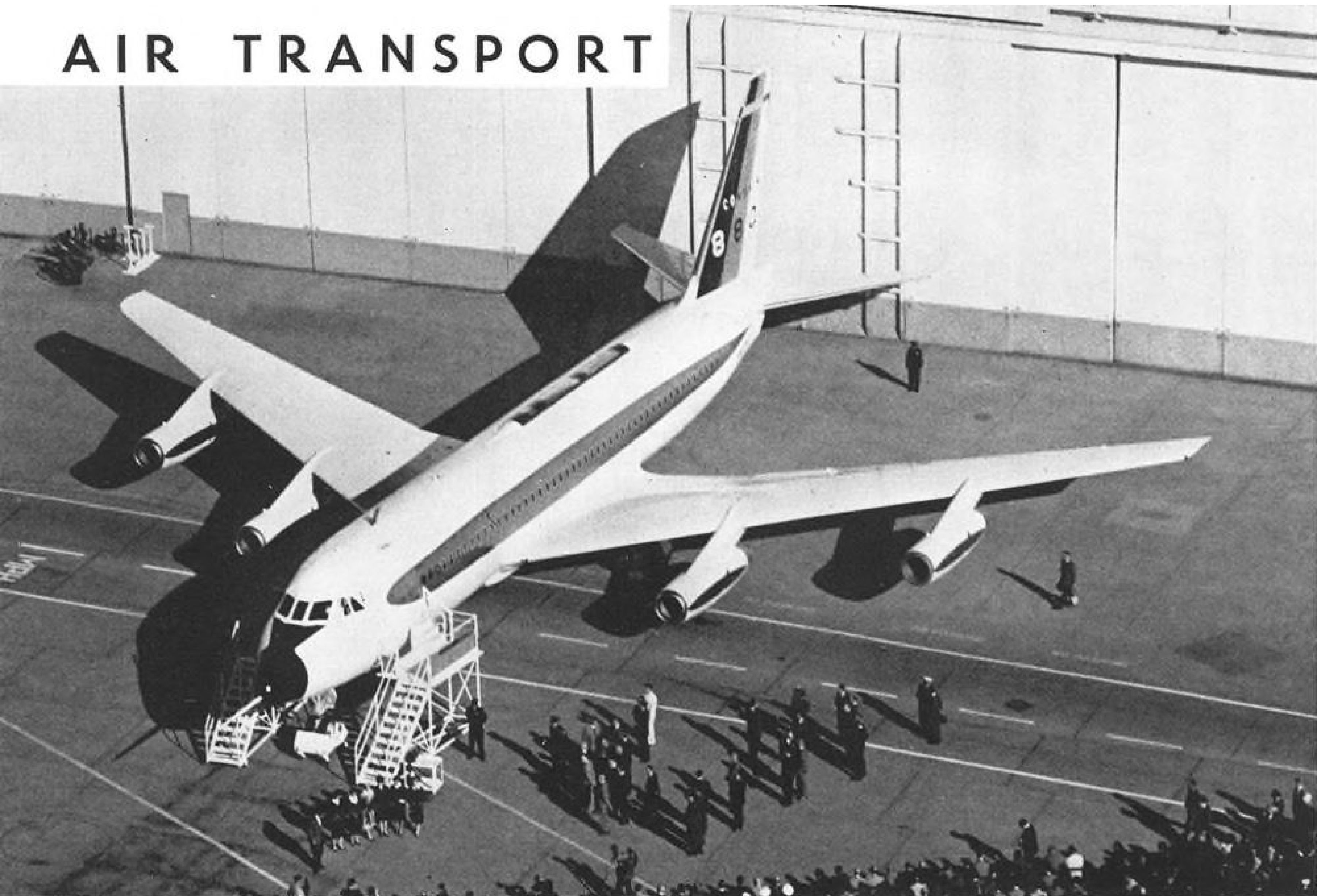
ANTENNAS are flush-mounted in semi-circular housing on top of Convair 880 jet transport fuselage. Engine sound suppressors and reversers are scheduled to be installed soon.
