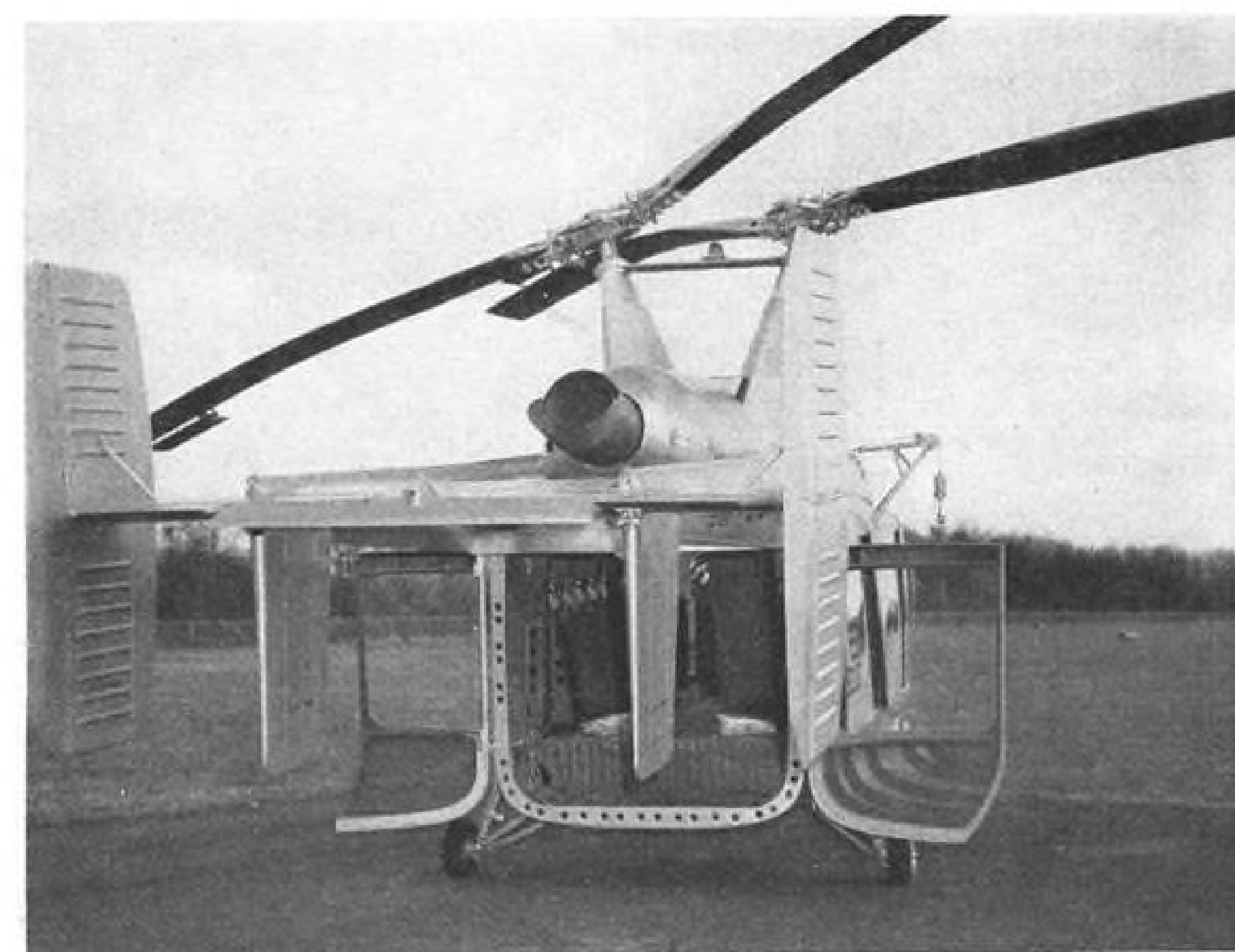
EXTERNAL MOUNTING of T53 turbine permits full use of fuselage internal area for payload and entrance is eased by fitting clamshell doors (shown open, above). H-43B has approximately twice the cubic capacity of previous piston-engine H-43A/HOK-1, its cabin measuring approximately 63 in. wide x 46 in. high x 103 in. long. Varied personnel loading accommodations (below) permit carrying up to seven passengers plus pilot.
