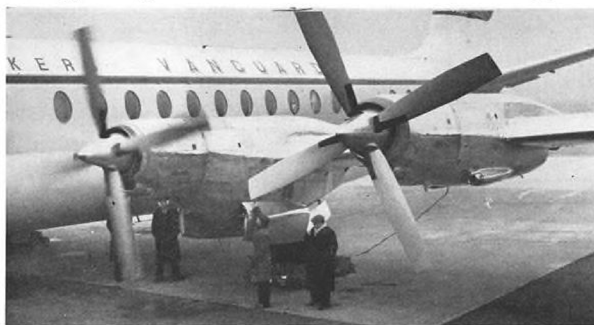
VANGUARD utilizes de Havilland propellers on its four Rolls-Royce Tyne engines. Scoop on outboard nacelle ducts ram air into heat exchanger for leading edge anti-icing.
