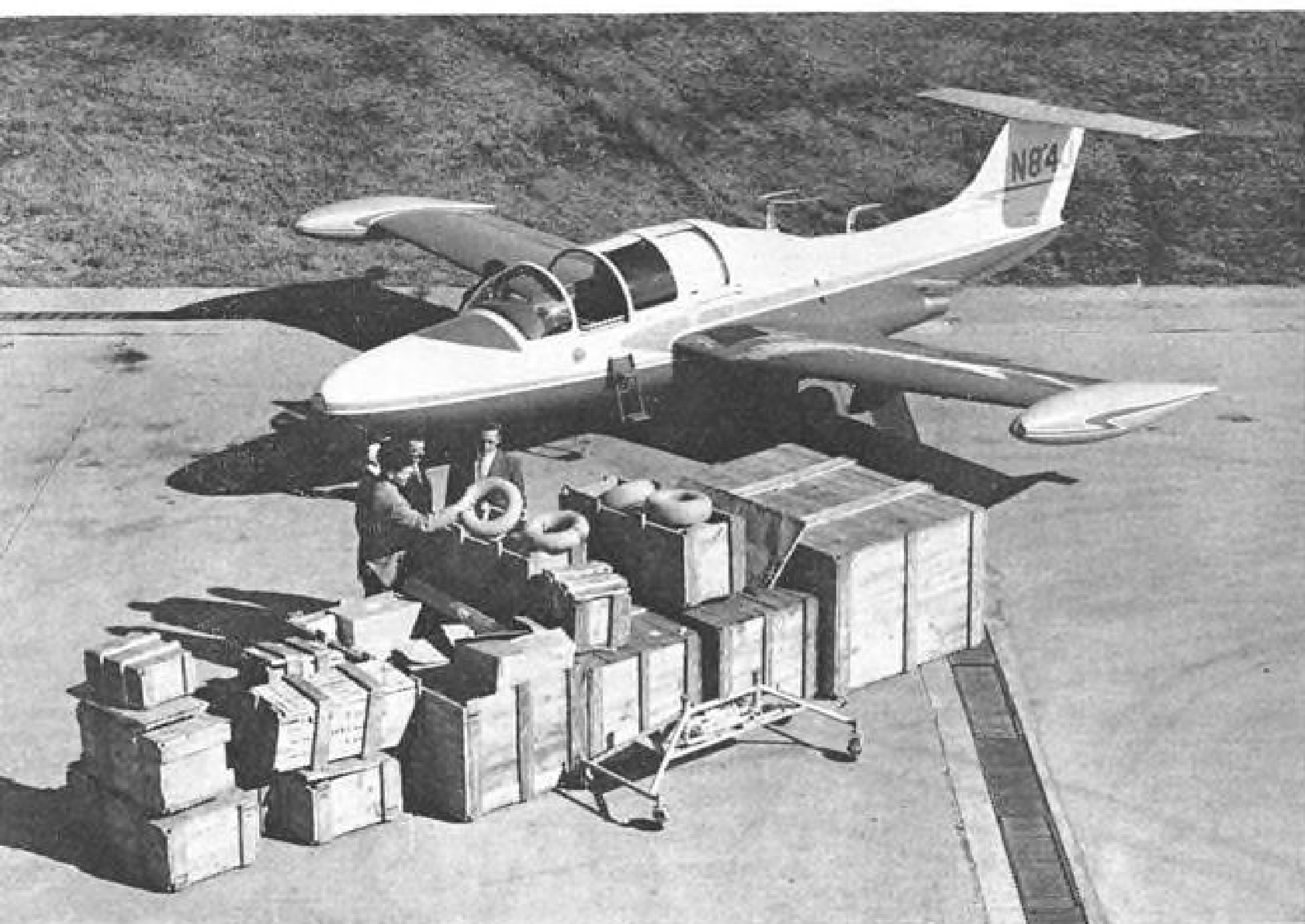
CRATED ground handling equipment, tools and spares are included in the basic price of the MS 760. Items include dollies, rigging fixtures, slings, tow bar, hoists, extra tires and tubes, wrenches, etc. Beech stocks engines and spare parts.
