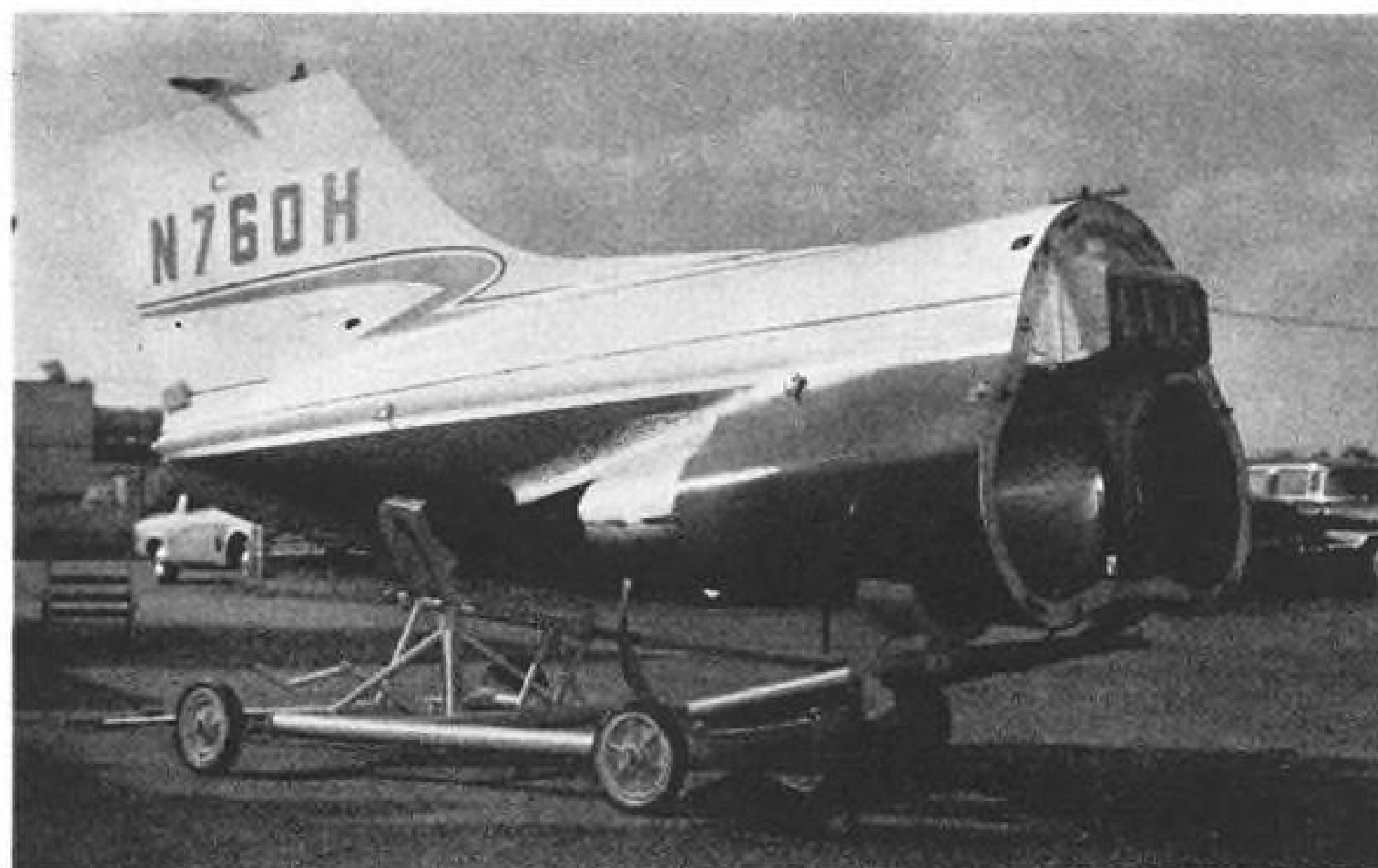
REAR fuselage of the MS 760 is demounted by removing six bolts. Work time to detach tail is approximately 15 min. Demounting exposes complete engine installation.
