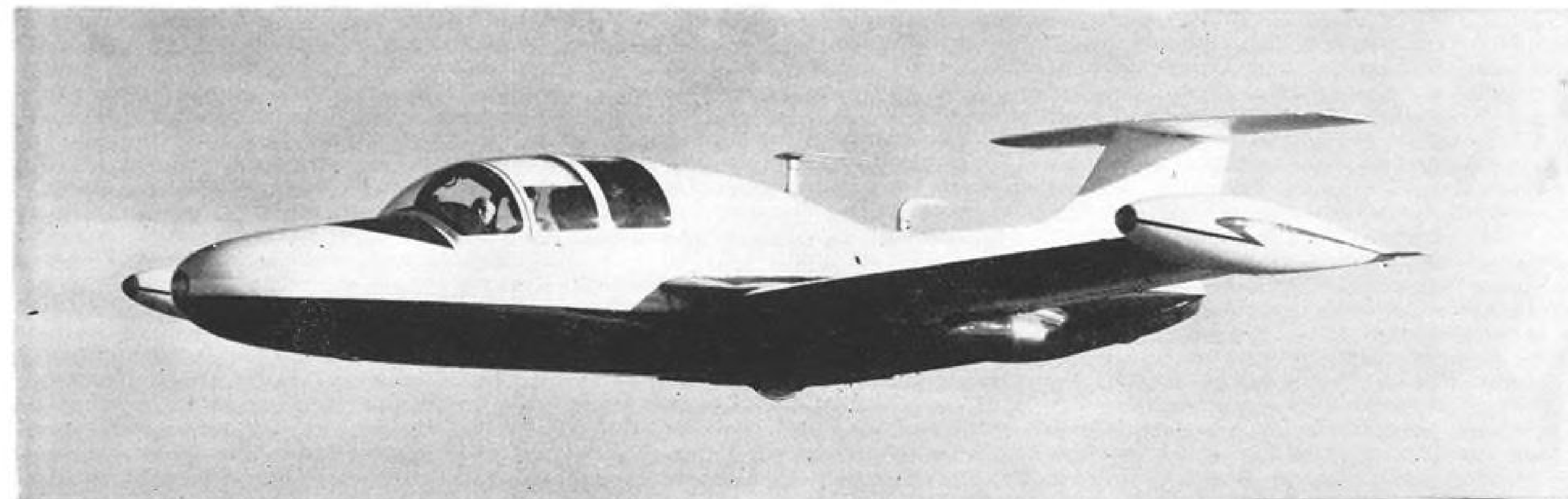
BEECH marketed MS 760 400-mph.-plus twin-jet has a span of 33 ft. 3 in. Length is 32 ft. 11 in. Wing area is 193.9 sq. ft. Four place, with tip tanks full, wing loading is 39.8 lb./sq./ft. Maximum gross weight is 7,500 lb. Maximum range is 820 naut. mi.
