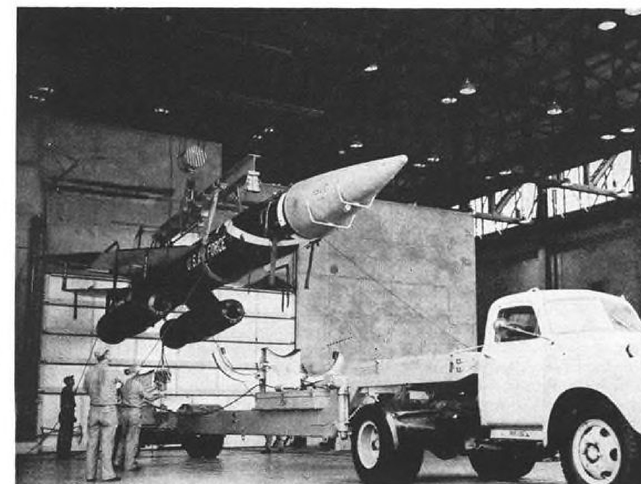
IM-99A MISSILE will be followed by Super Bomarc IM-99B which will have a range of 400 mi. and speed of Mach 3.5. Missile is loaded on transporter (bottom).
