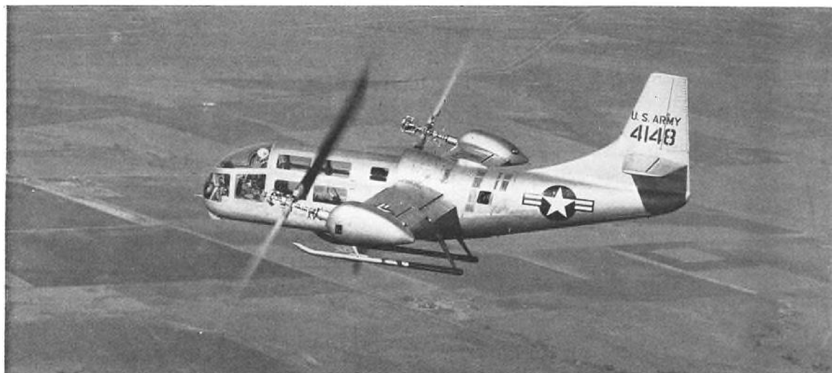
ROTOR MASTS on Bell XV-3 convertiplane are in about 85 deg. position for full forward airplane flight configuration.
