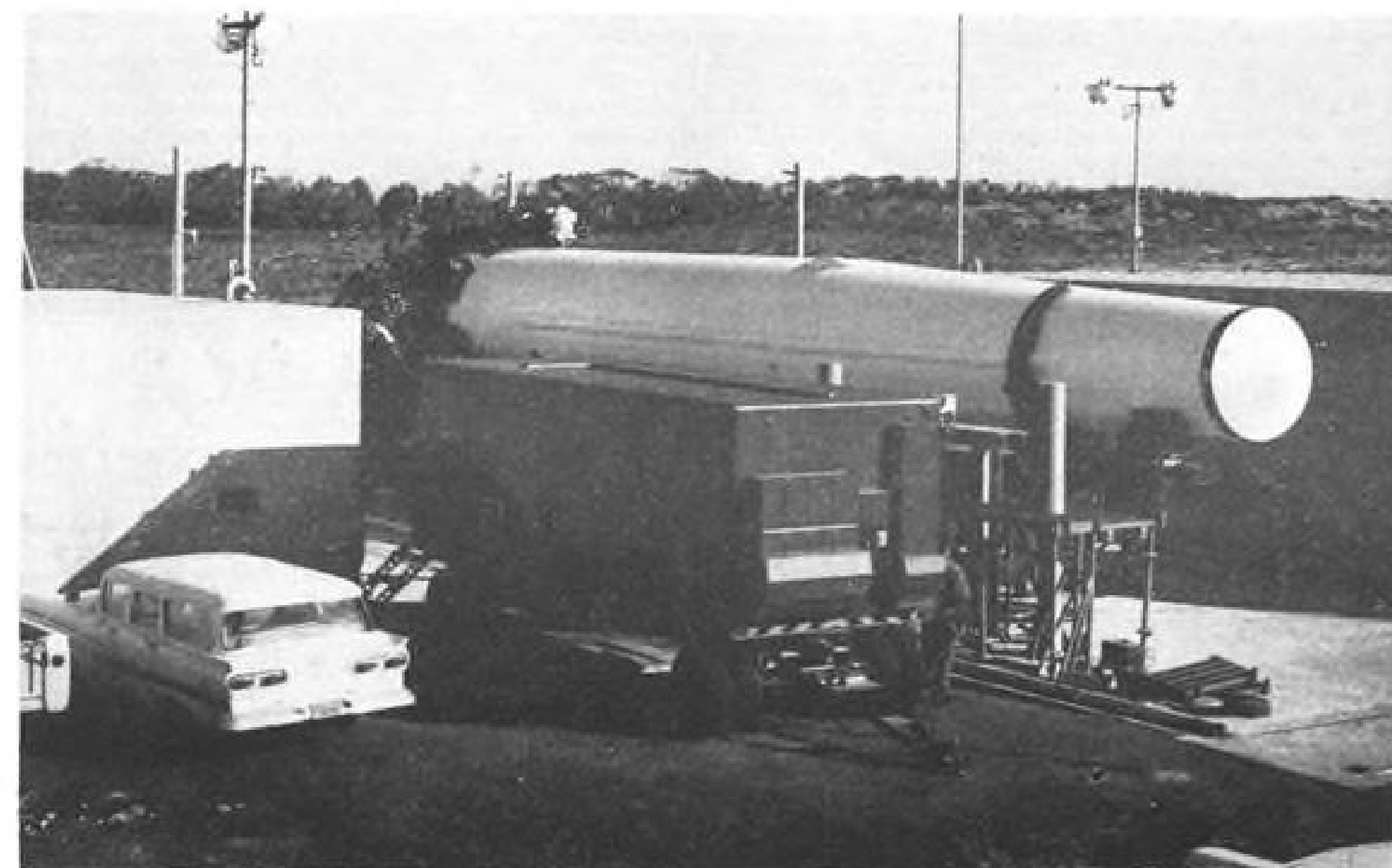
USAF's Thor intermediate range ballistic missile is partially enclosed in portable shelter (above). Front wall of cover slides to one side; main structure is rolled back to expose the missile. Below, the Douglas Thor is ready to be erected to the firing position.
