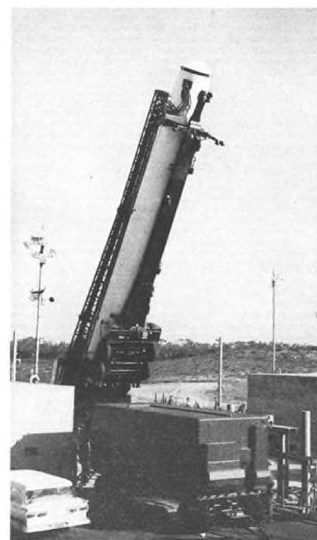
Transporter-erector elevates Thor to firing position. Missile is automatically elevated to vertical for the launching.
