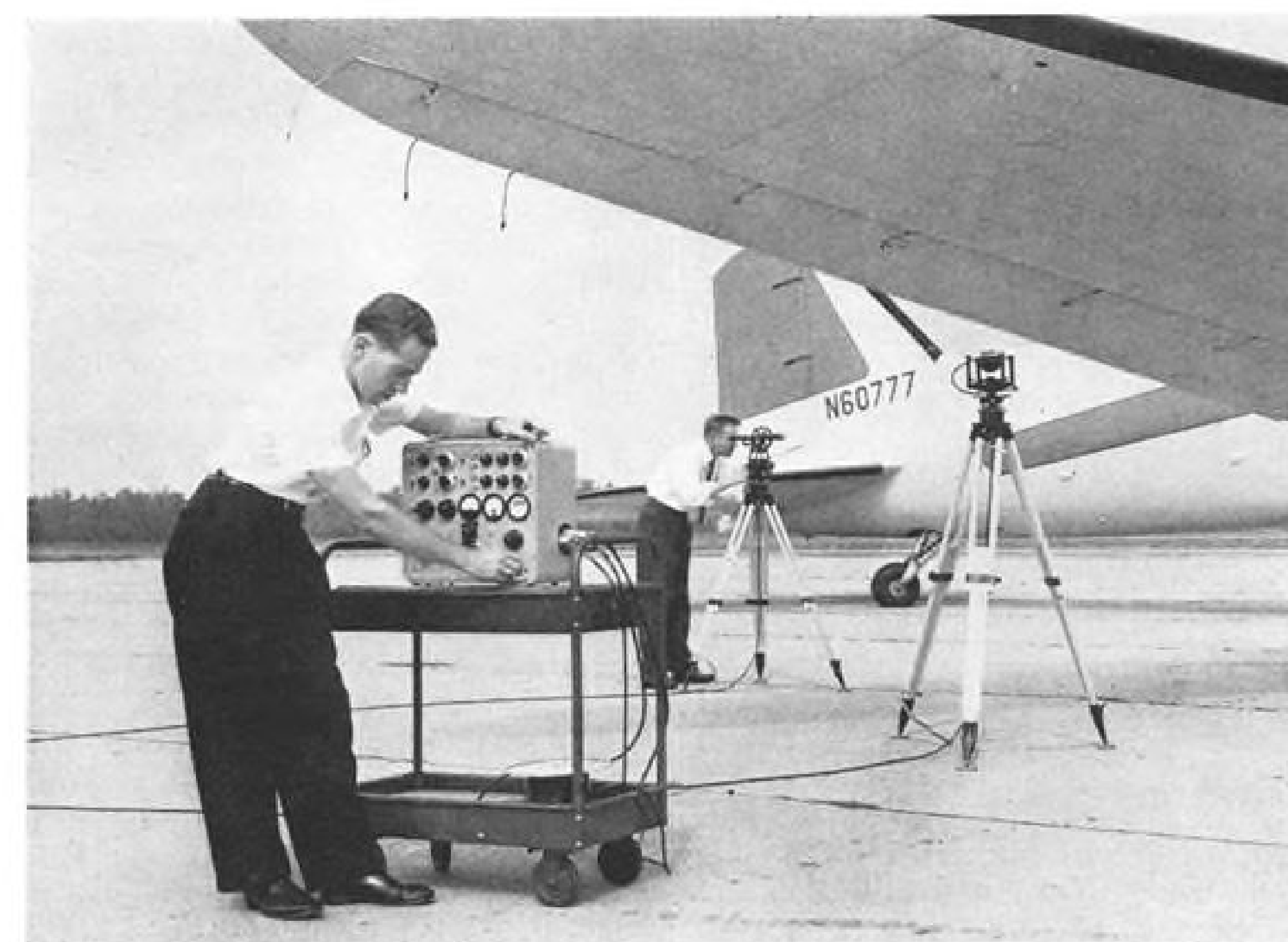
FLUX valve (direction-sensing device) is mounted on surveyor's tripod at right.
