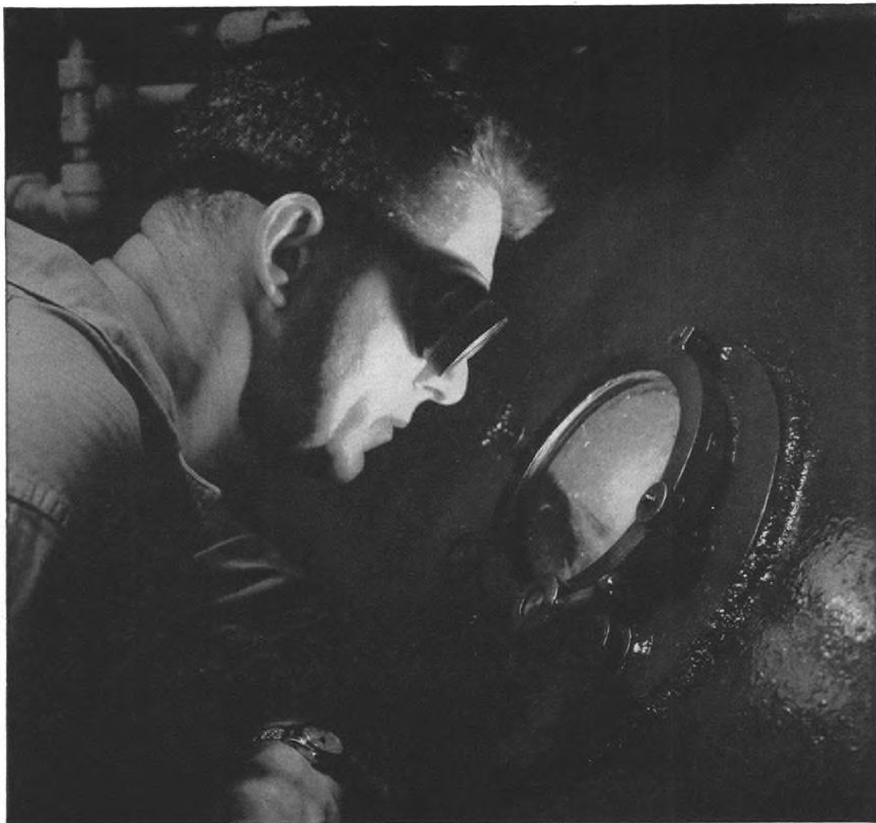
Technician viewing melt under a vacuum of approximately one-millionth of atmospheric pressure.
