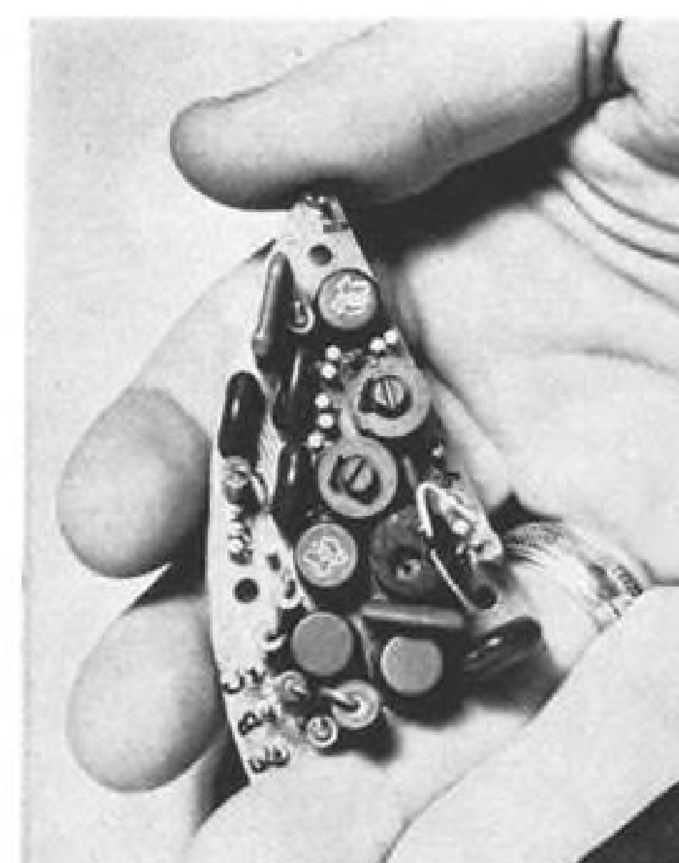
ONE of 10 transistorized amplifiers which mount directly onto gimbals of the Sperry gyro stabilized platform.
