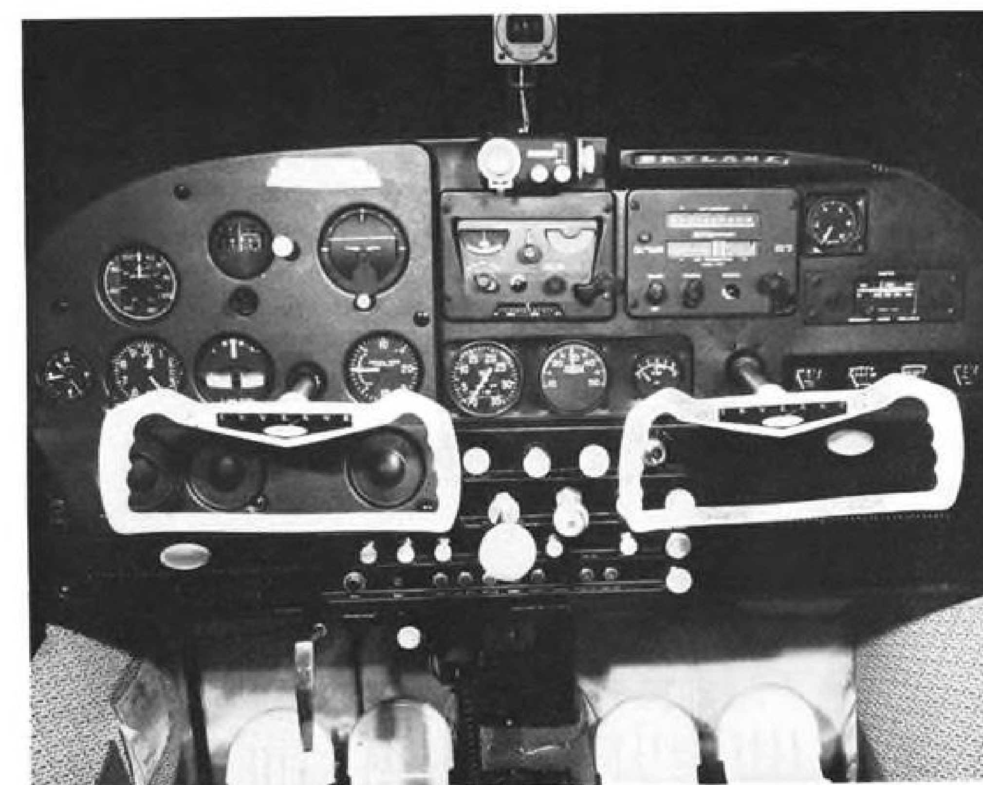
INSTRUMENT PANEL has instruments regrouped; Tactair Levelair is mounted top center.
