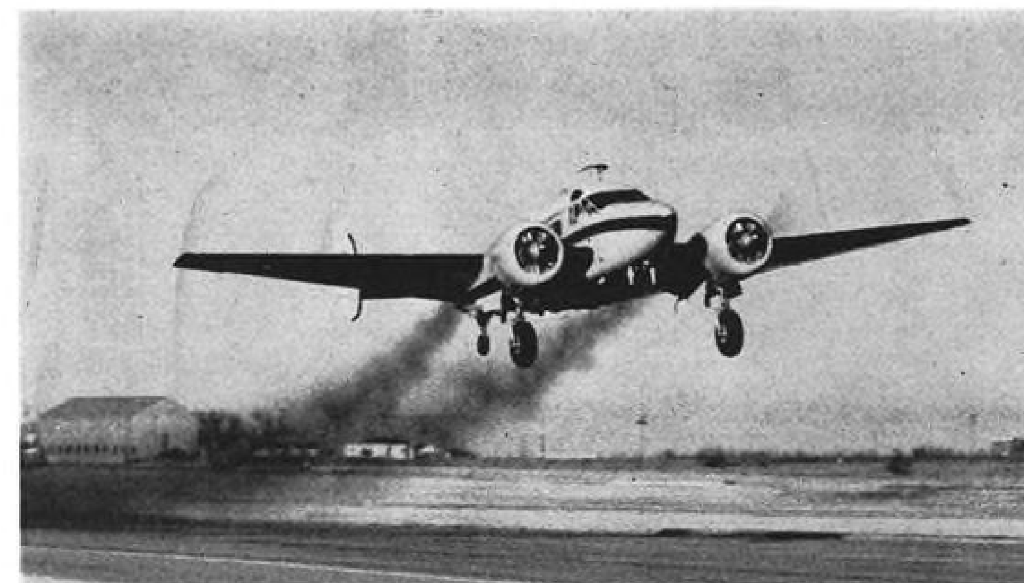
JATO ROCKETS boost Super 18 twin-engine climb rate nearly 600 fpm.; by 500 fpm. on one engine with airplane at full gross weight.
