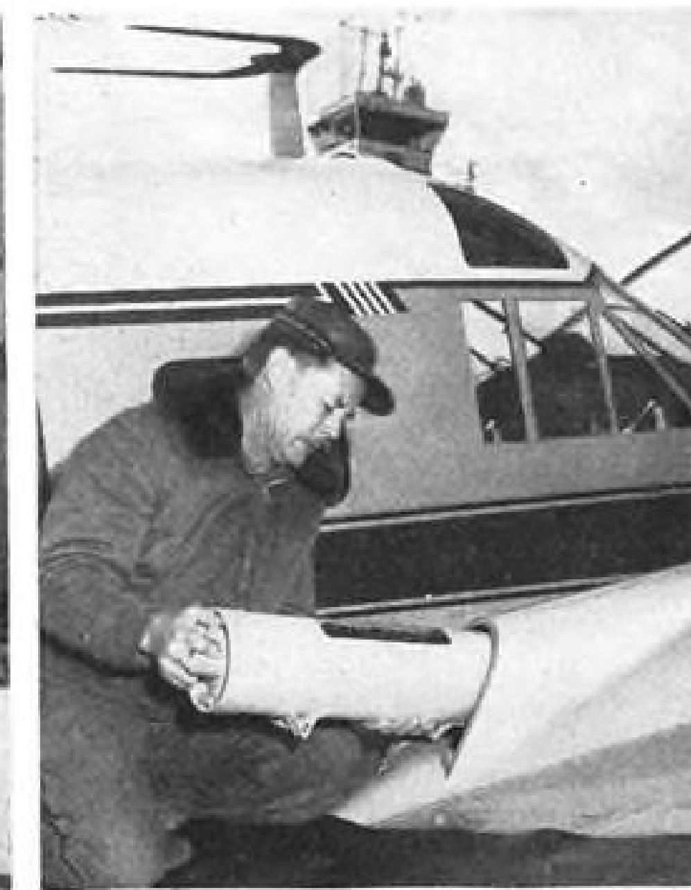
ONE SWITCH (left) fires both rockets at once. Motor is placed in engine nacelle (right).
