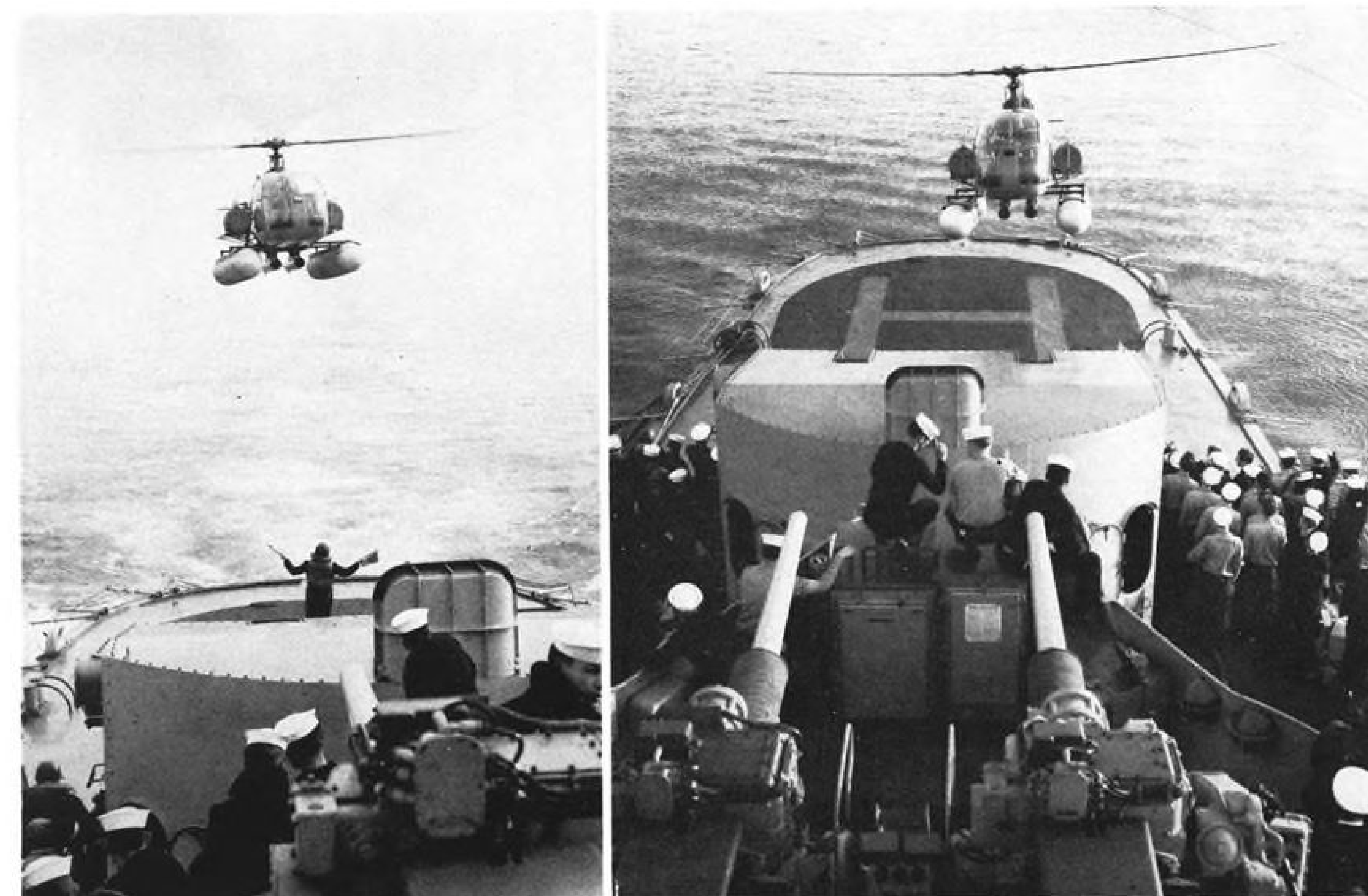
ACOUSTIC-SEEKING torpedoes are slung between floats of Republic Alouette (left), shown taking off; aircraft is landing on fantail at right.
