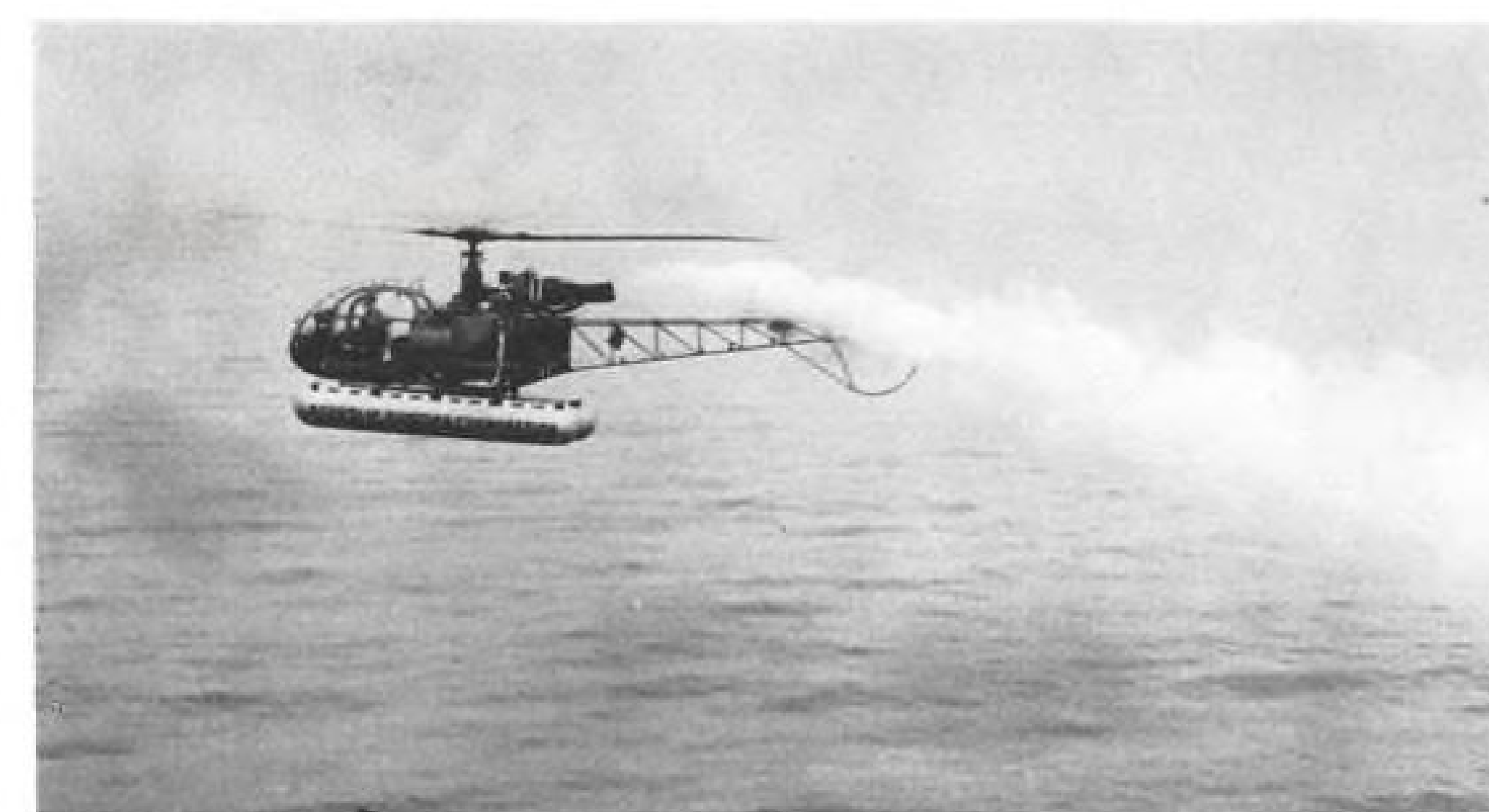
REPUBLIC Alouette's smoke-laying capability is attained by pumping chemicals directly into the tailpipe. Navy is testing materials to make the smoke opaque to radar.
