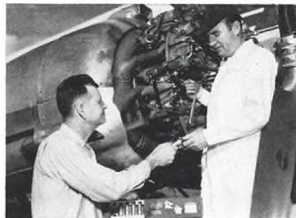
Robert Eakle (L), Assistant Foreman Accessory Shop, and Lead Mechanic John Brennan (R) installing AC-271's in FAL plane.
