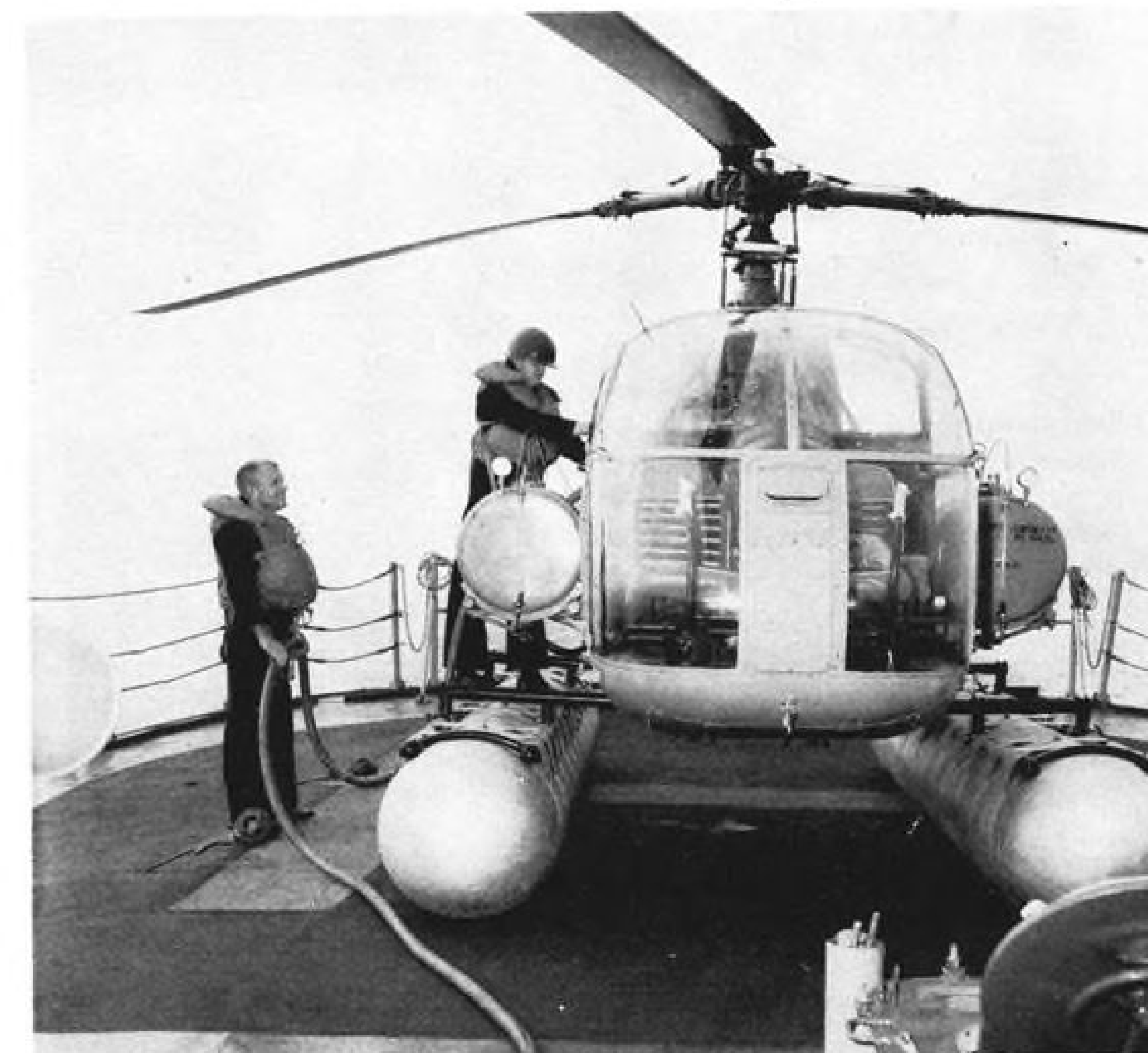
CERTIFIED for diesel fuel operation, Alouette II is fueled by hydrant from ship's bunkers.
