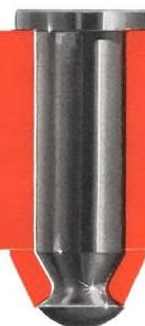
NOSE CONE SPLICE JOINTS ARE FASTENED WITH HS67 PINS, TYPE 431 STAINLESS STEEL, HEAT TREATED TO 125,000 PSI MINIMUM SHEAR. THE HS60M COLLARS ARE R MONEL.
