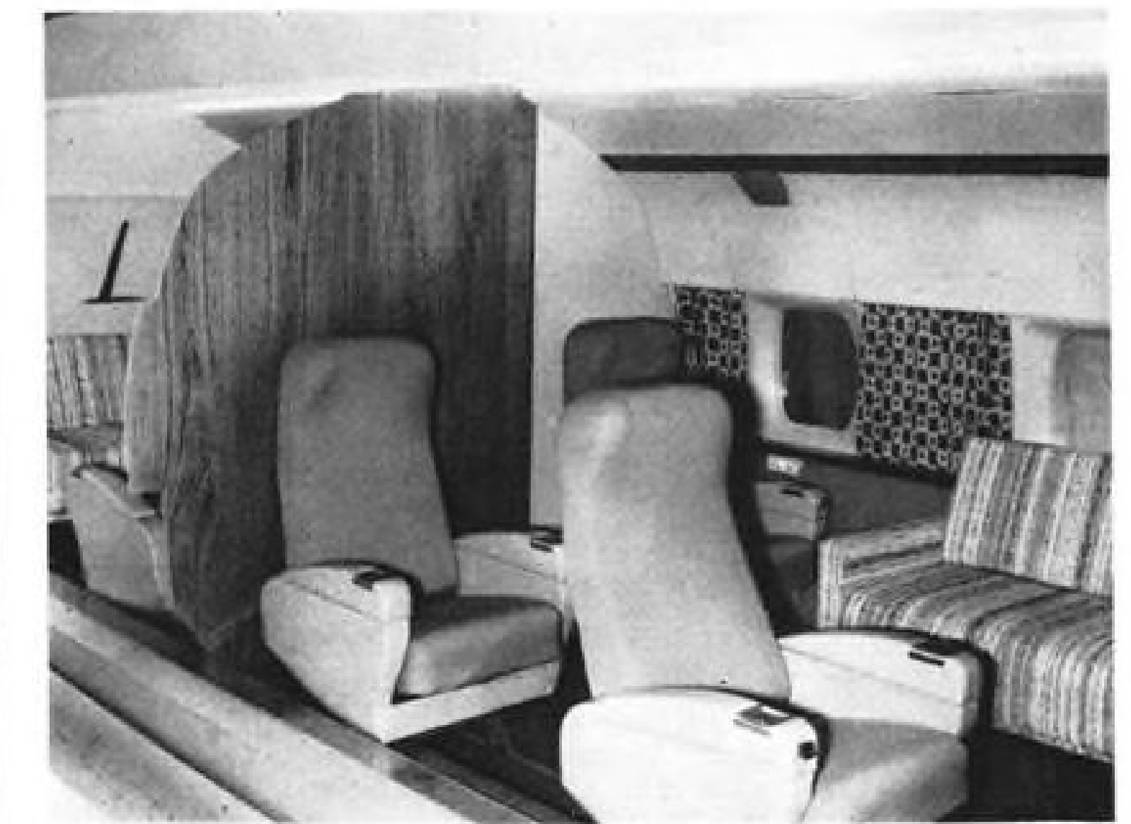
Model 119 is pressurized with bleed air from Westinghouse J34 turbojet engines; later, Pratt & Whitney JT12 engines will be installed. Configuration at left shows six of 12 litters. Another arrangement (right) includes use of divans and fore and aft seating.
