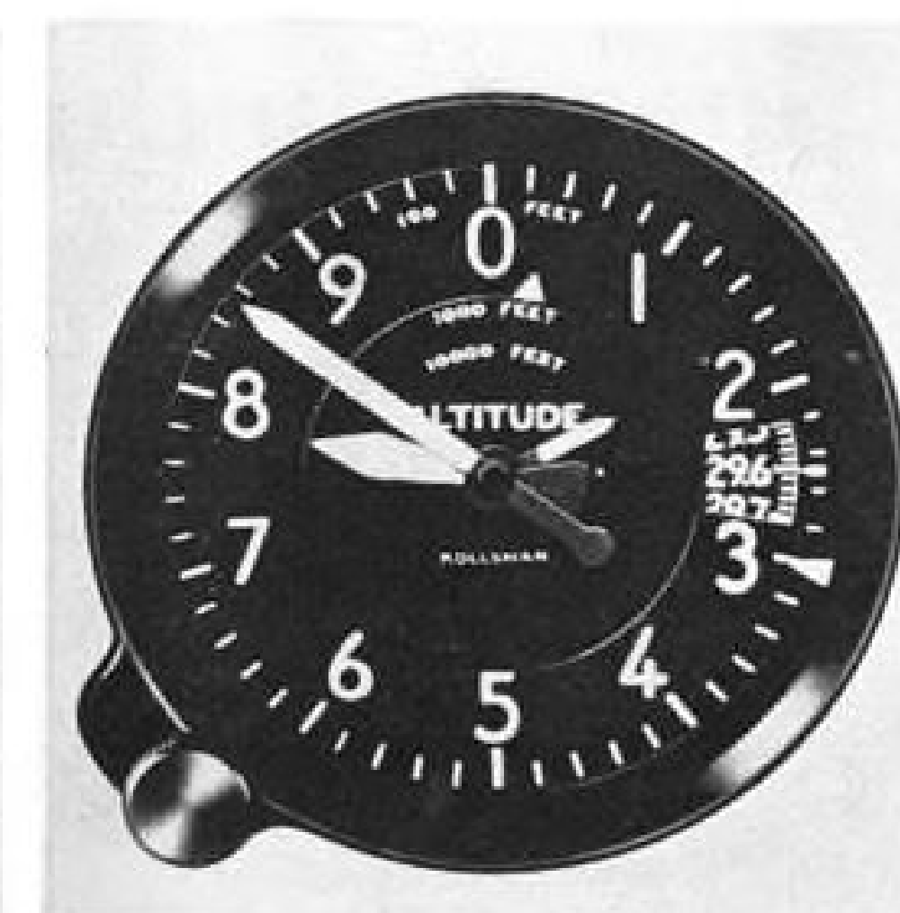
DRUM-POINTER altimeter (left) is a new presentation introduced on the Lockheed Electra and the Boeing 707-120 and due to be production equipment in Douglas DC-8s and Convair 880s. This altimeter could be misread in 1,000-ft. increments but is considered easier to read than the three-handed altimeter (right) which could be misread by 10,000-ft.
