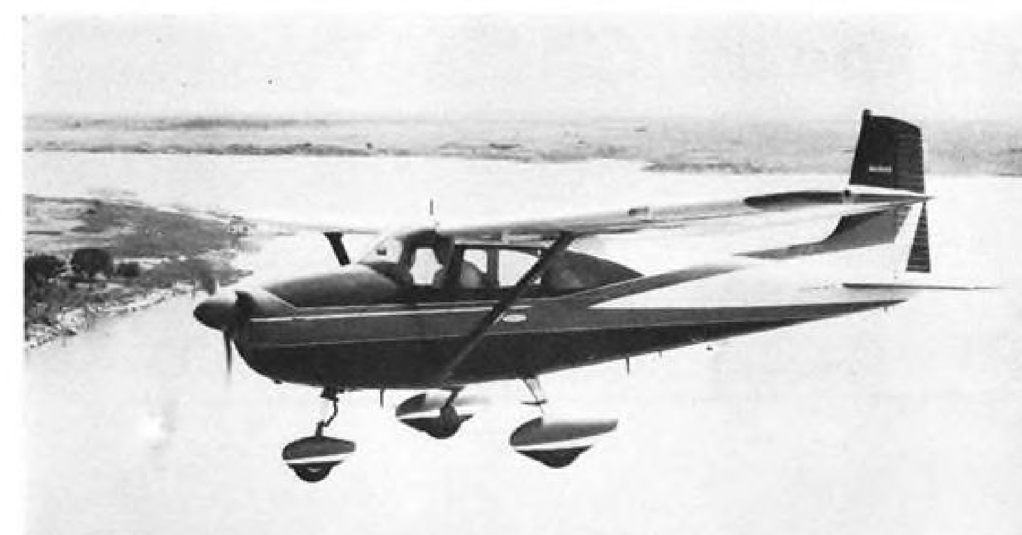
CLEANED-UP COWL in 1959 Cessna Skylane, priced at $17,095, boosts speed two miles-per-hour. Cowl features streamlined nose cap.
