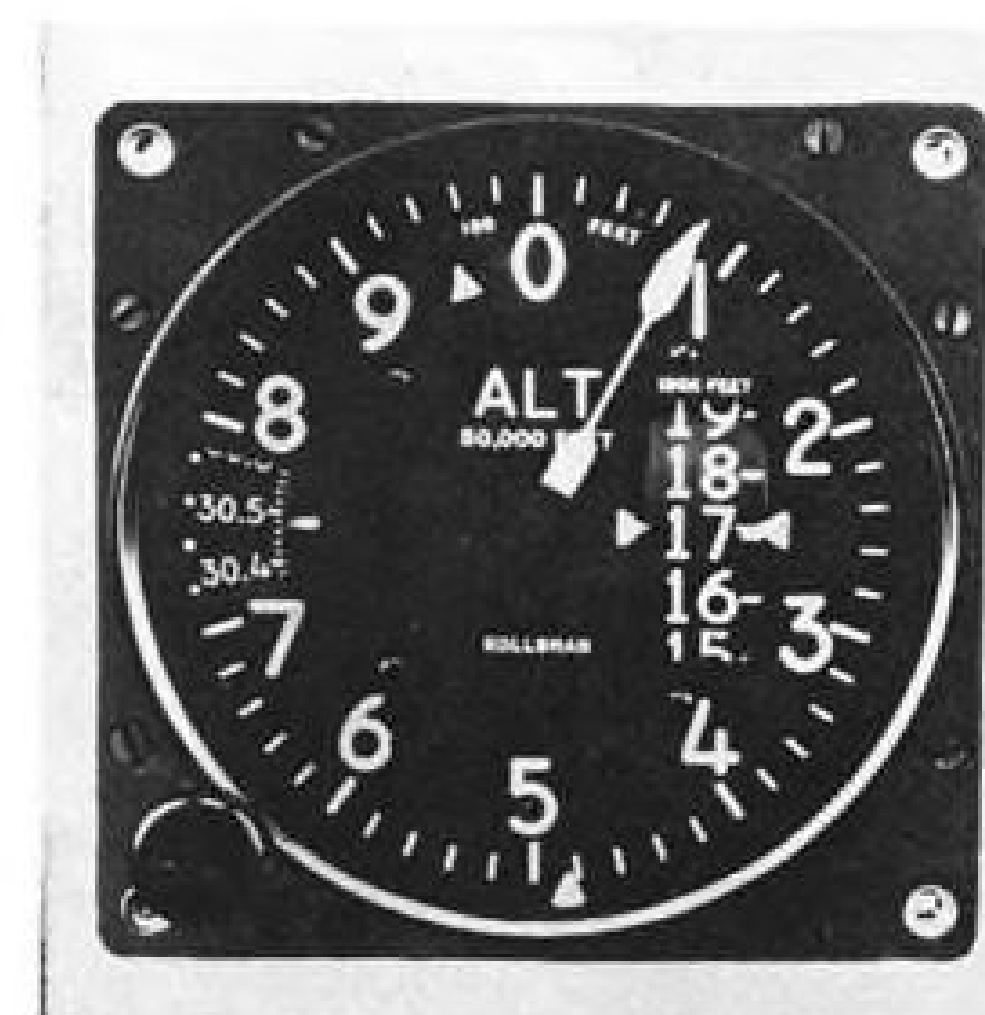
DRUM-POINTER altimeter (left) is a new presentation introduced on the Lockheed Electra and the Boeing 707-120 and due to be production equipment in Douglas DC-8s and Convair 880s. This altimeter could be misread in 1,000-ft. increments but is considered easier to read than the three-handed altimeter (right) which could be misread by 10,000-ft.
