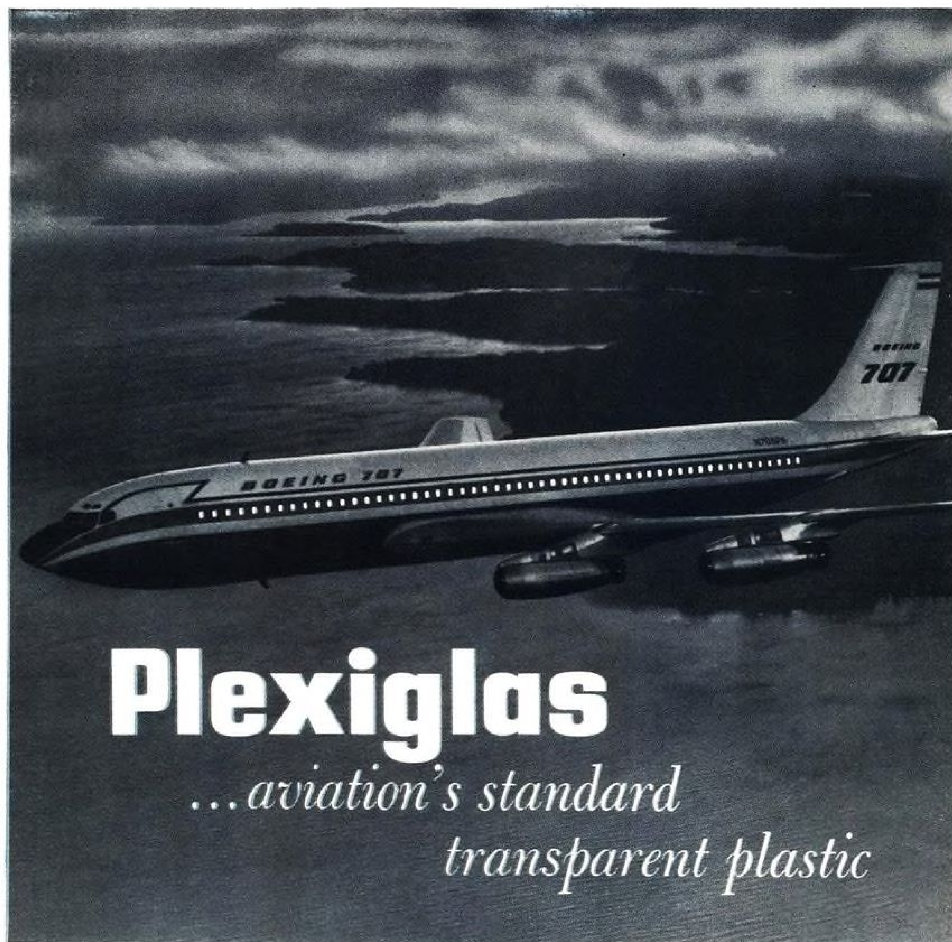
Boeing 707's 98 windows are triple-glazed with PLEXIGLAS. Outer and middle panels are made of stretched PLEXIGLAS 55.
