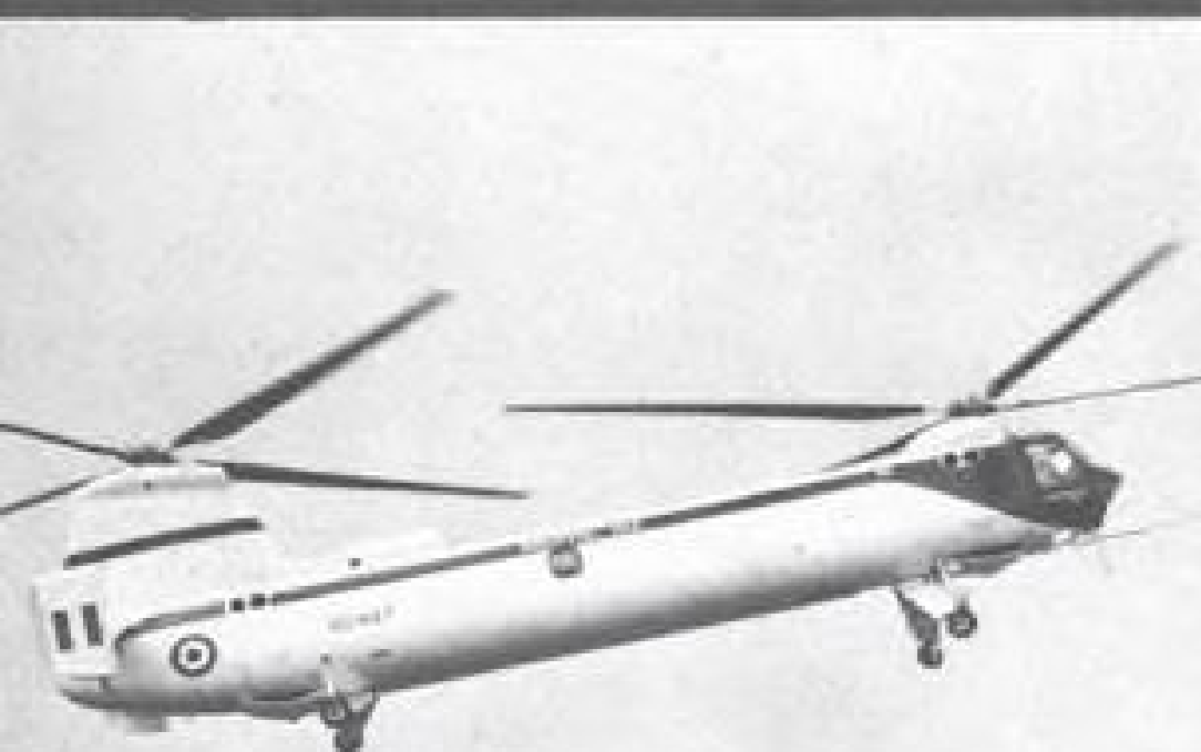
Bristol 192. Royal Air Force Helicopter with two Napier Gazelle free turbines.
