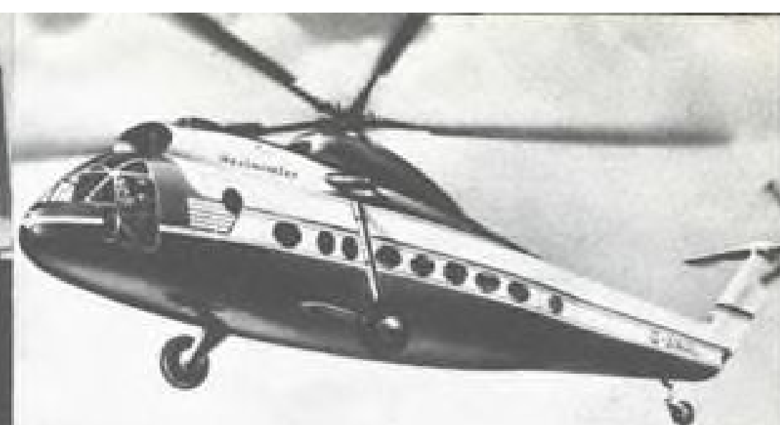
Westland Westminster—helicopter carries 6 tons of cargo or 46 passengers . . . powered by two Napier Eland engines.
