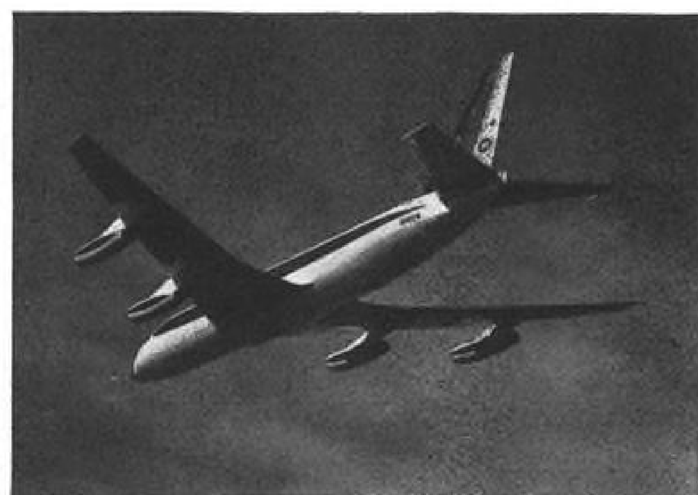
Intercontinental version (not yet built) of the Convair 880 will have 4,210 mi. range. The four General Electric CJ-805-3 turboprop engines are commercial versions of military J79. Engines are fitted with daisy-type sound suppressors with thrust reversers planned.
