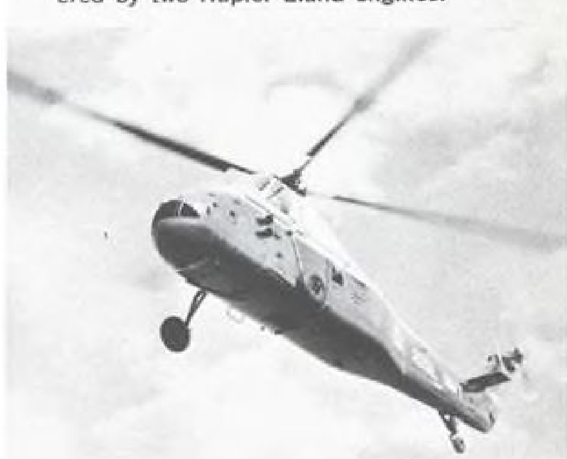
Westland Westminster—helicopter carries 6 tons of cargo or 46 passengers . . . powered by two Napier Eland engines.
