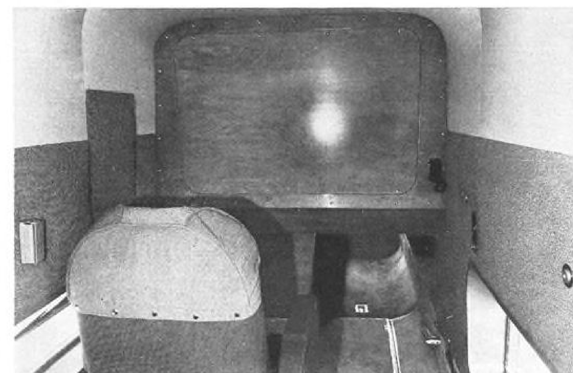
REAR WING SPAR carry-through shown here covered by wood paneling, cuts into cabin space, but LeTourneau accepts the penalty in order to retain the strength originally designed into the wing structure.
