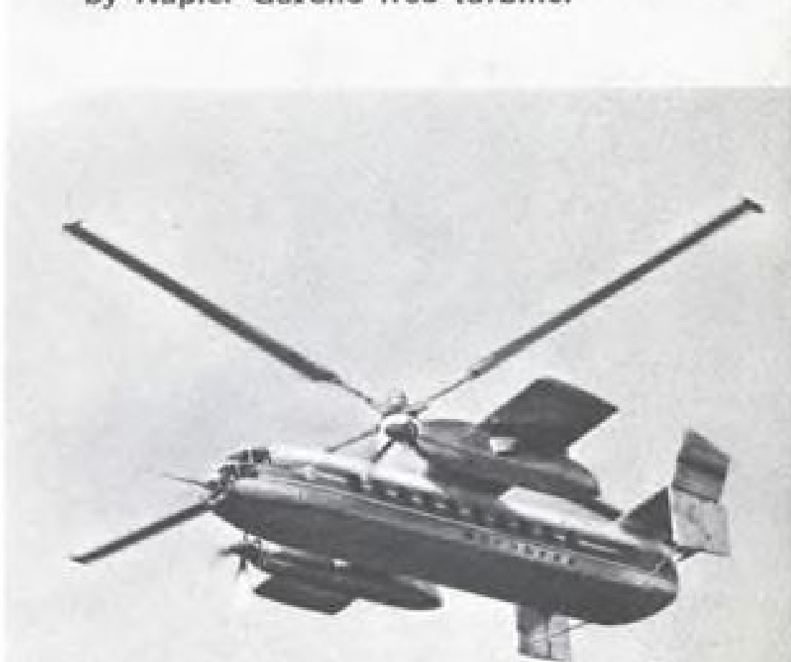
Westland Wessex . . . helicopter powered by Napier Gazelle free turbine.
