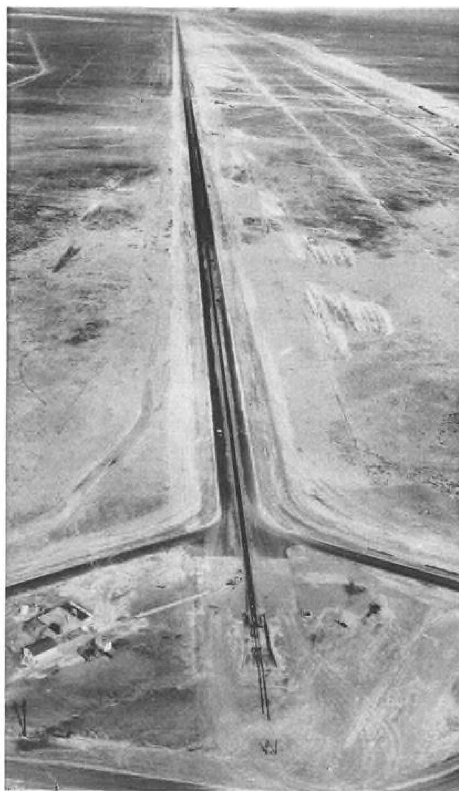
AERIAL view of I-beam test sled shows vehicle hitting the water brake. Triangular shaped scoop mounted below the sled (lower photo) picks up water in the trough and throws it out on both sides and behind the sled, thus bringing it to a stop.
