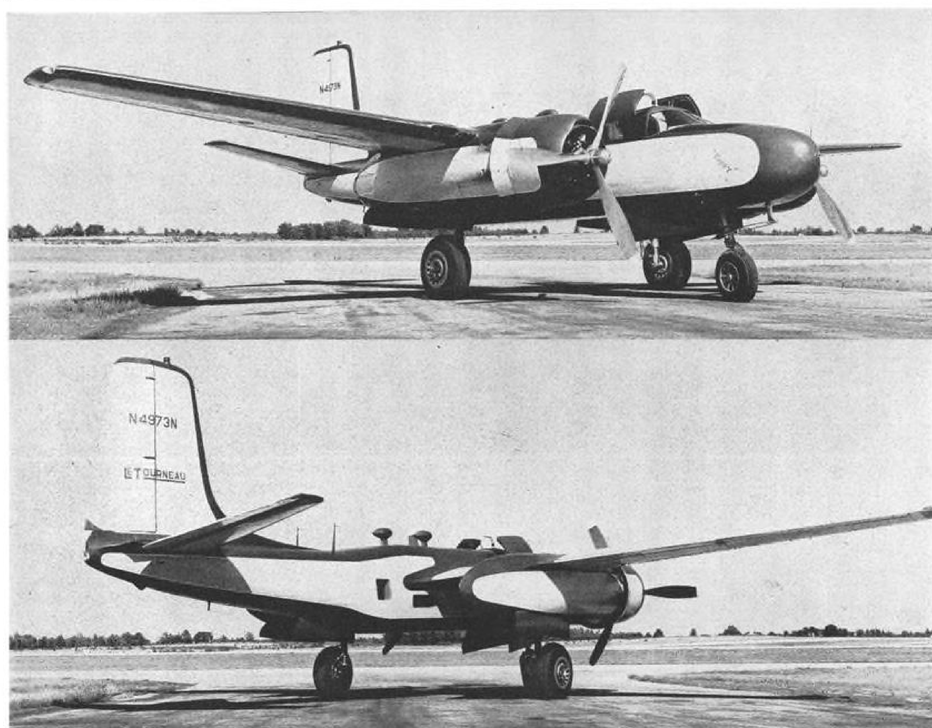
B-26 CONVERTED for executive use by R. G. LeTourneau, Inc. Note in front view insulated metal roof that has been installed in the cockpit hatch cover to protect the pilot. The conversion has a narrow cabin window under the wing (see rear view) and a square window aft of the wing which also serves as an escape hatch.
