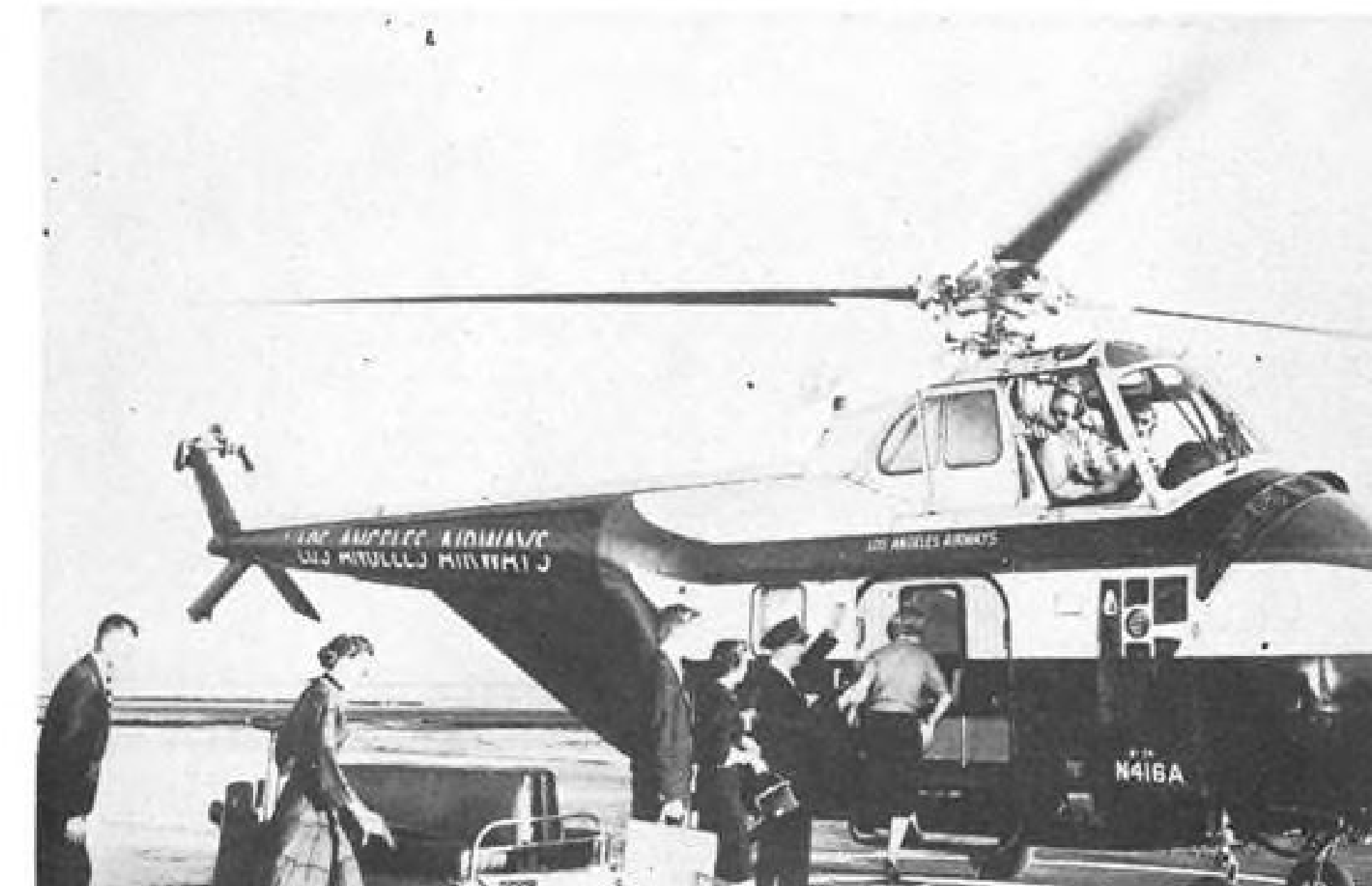
SIKORSKY S-55 takes off from Long Beach Municipal Airport (above). During passenger loading (below), the helicopter's rotor rpm. is maintained but blades are in flat pitch, producing minimum downwash disturbance to the passengers. Company-installed seats fold against wall, making helicopter convertible from passenger to cargo carrier in 3 min.
