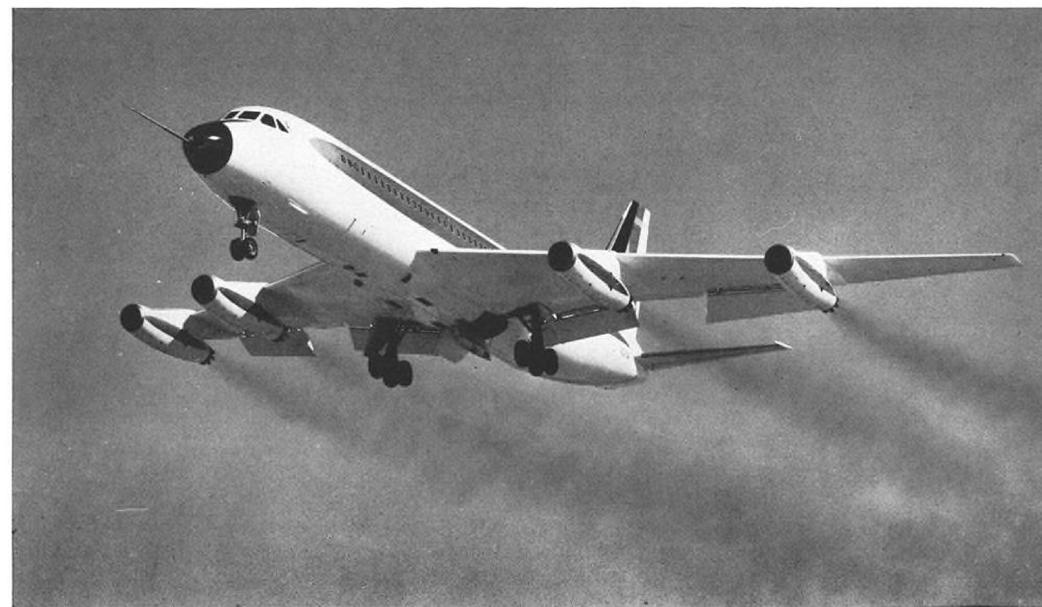
Transport, shown in "dirty" configuration, uses fuel at the rate of 12,000 lb./hr. to maintain top cruise speed of Mach .89.
