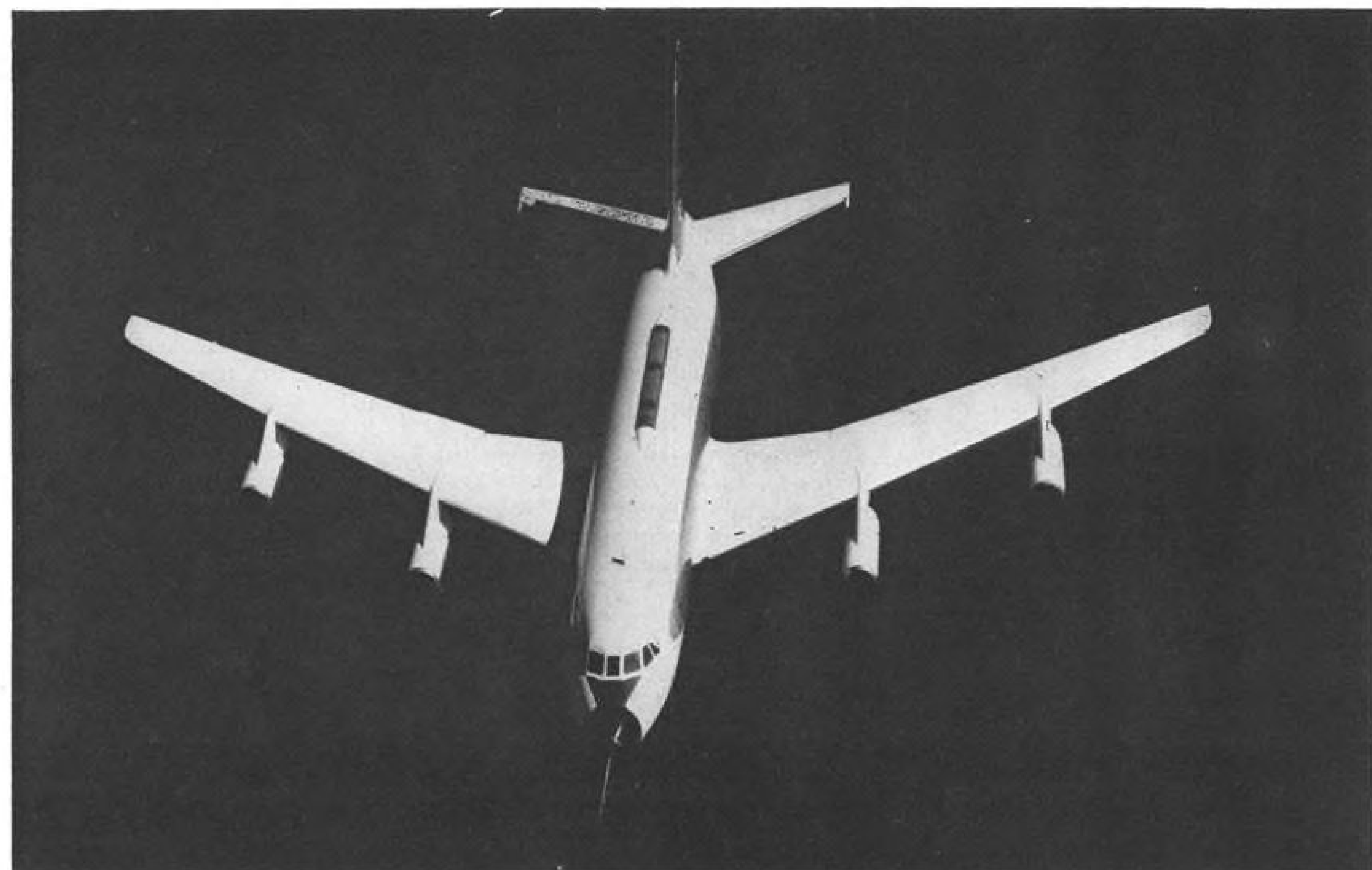
Intercontinental version (not yet built) of the Convair 880 will have 4,210 mi. range. The four General Electric CJ-805-3 turboprop engines are commercial versions of military J79. Engines are fitted with daisy-type sound suppressors with thrust reversers planned.
