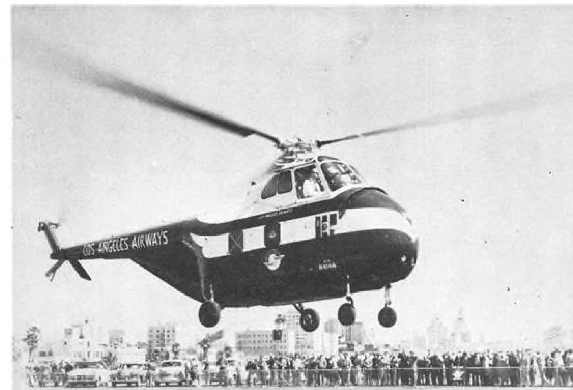
SIKORSKY S-55 takes off from Long Beach Municipal Airport (above). During passenger loading (below), the helicopter's rotor rpm. is maintained but blades are in flat pitch, producing minimum downwash disturbance to the passengers. Company-installed seats fold against wall, making helicopter convertible from passenger to cargo carrier in 3 min.
