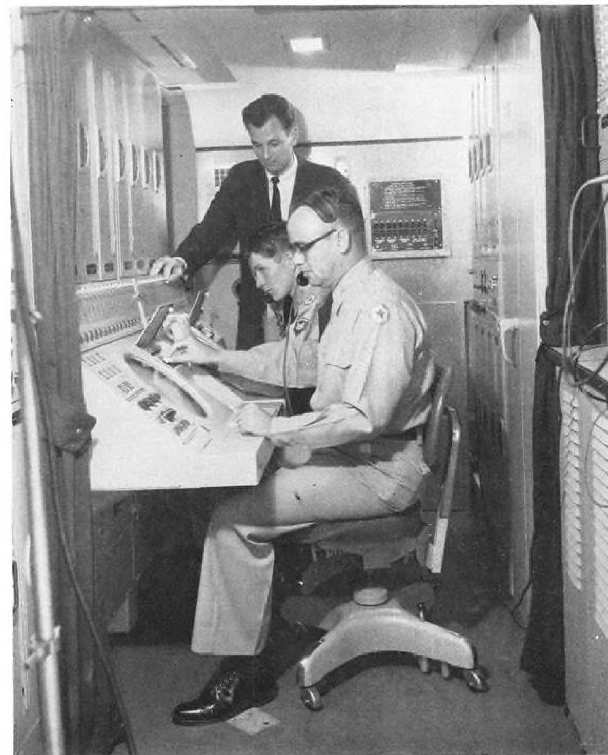
AIR BATTLES can be monitored and targets assigned to missile batteries from controls at tactical display screen of Hughes Aircraft Co.'s air defense system's command center. System is being produced under a $30 million Army contract.
