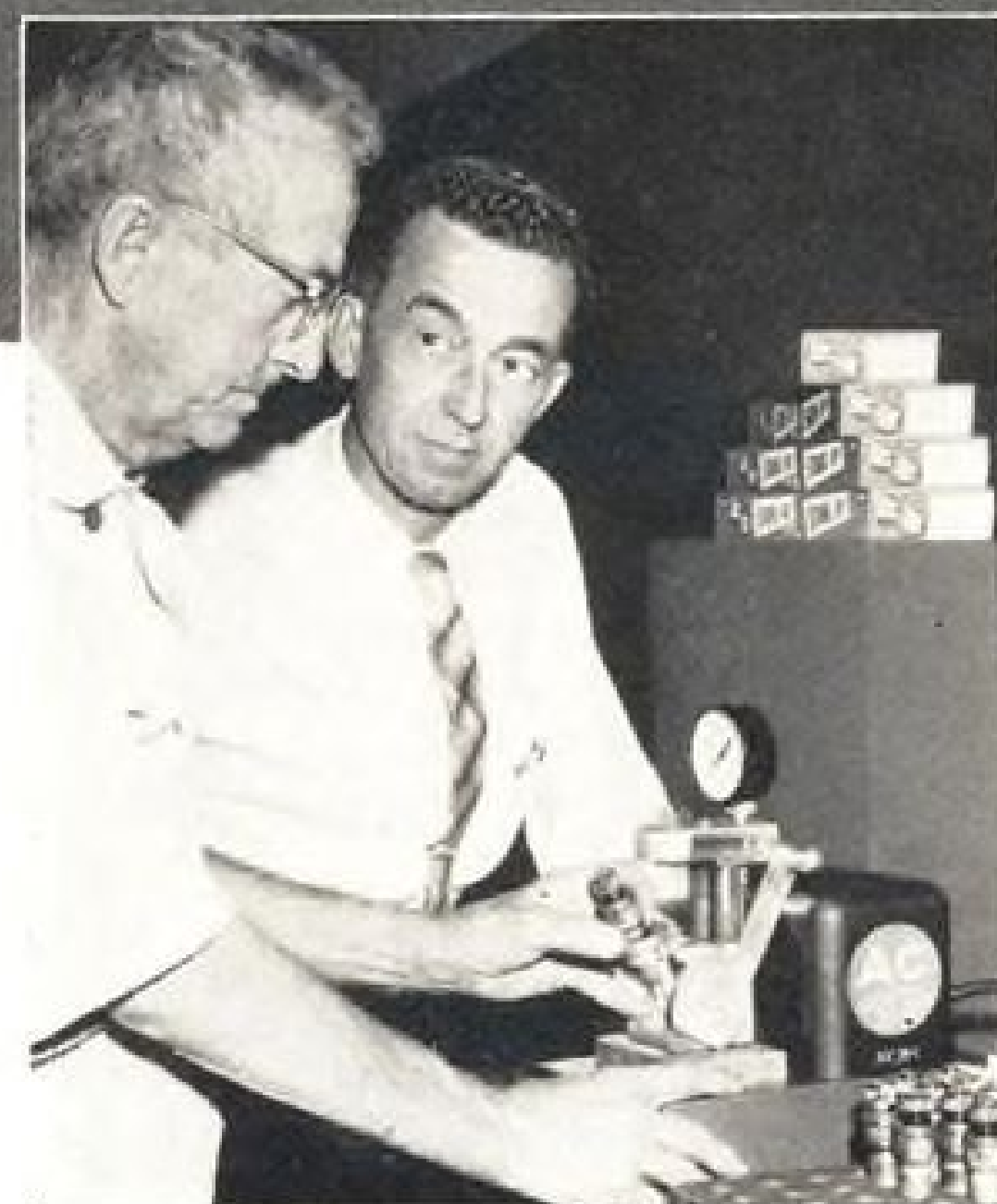
General Foreman Al Jespersen watches Aviation Mechanic Frank Neal "bomb-test" the AC 271 Spark Plug. Frank prefers the combination of AC 271 and 275 spark plugs to power Western's P & W R2800-CB Engines "... they are easier to clean, provide greater scavenging area which keeps plugs burning cleaner, longer."
