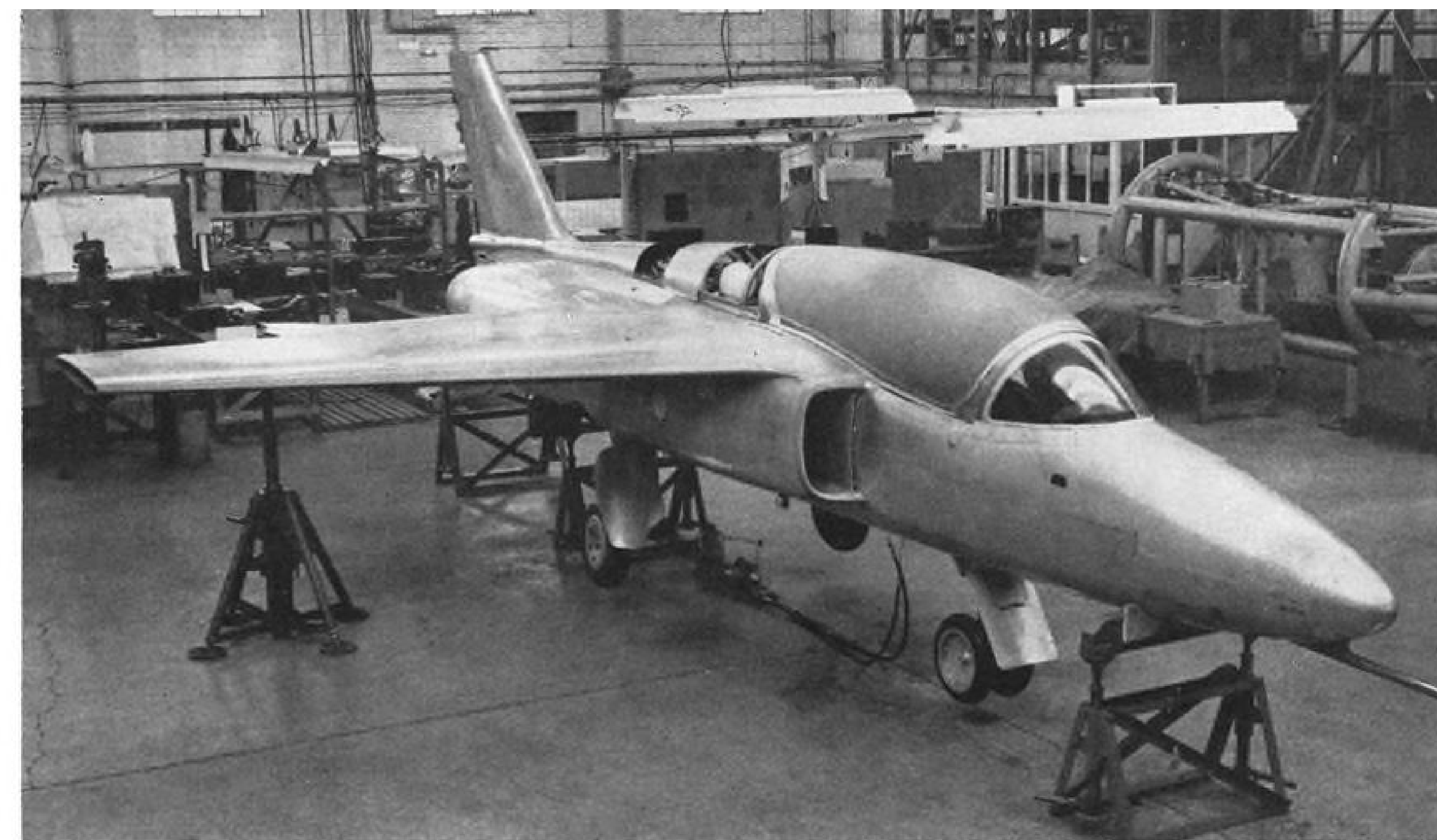
LARGE canopy and lengthened nose differentiate Gnat trainer from standard Mk. 1 fighter. Fuselage was lengthened 9 in.
