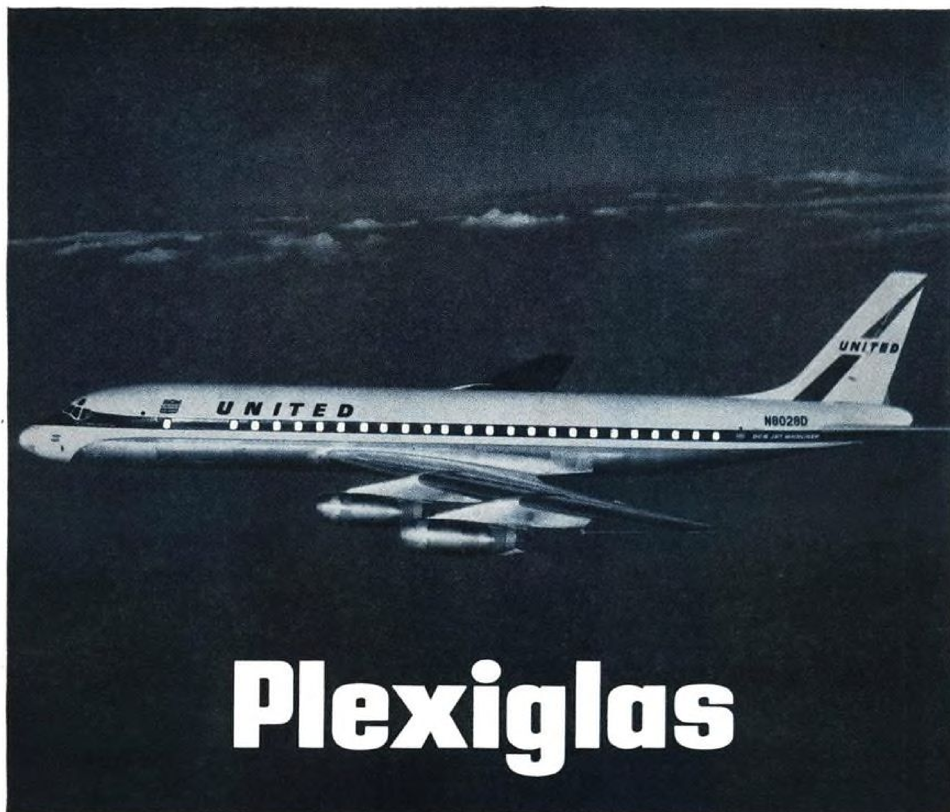
Douglas DC-8 jet transport of United Air Lines has windows measuring approximately 17" x 21", double-glazed and triple-glazed with PLEXIGLAS acrylic plastic. Outer panels are stretched PLEXIGLAS 55.
