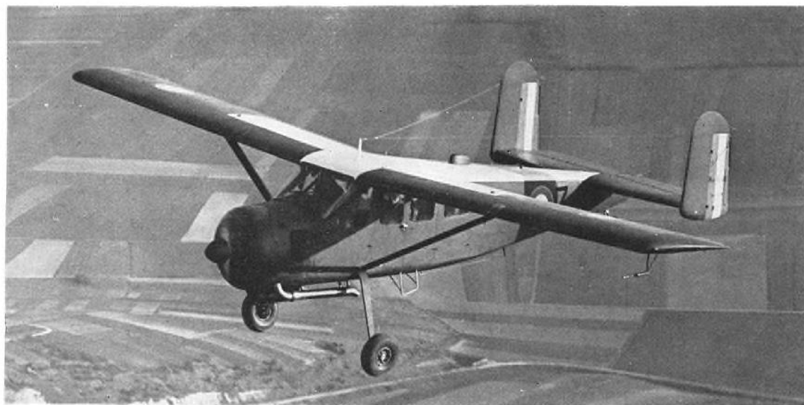
MH-1521 Broussard has a span of 45 ft. and length of 28.2 ft. Wing area is 274 sq. ft. Payload of 1,655 lb. can be hauled 745 mi.
