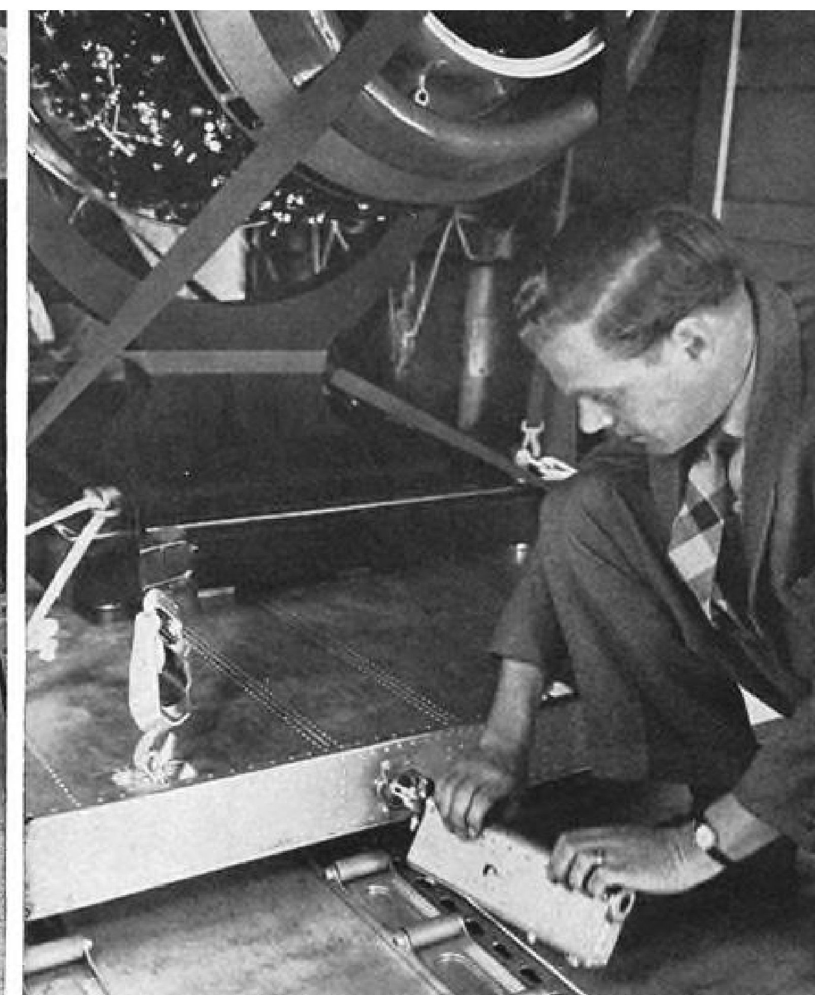
TRUCK HEIGHT loading floor speeds cargo operation (left); at right, palletized freight is secured to floor by locking pieces.
