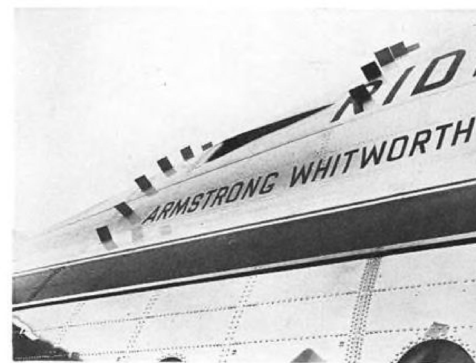
VORTEX generators (left) are installed on cockpit blister to help eliminate buffeting at rear. At right is AW 650 cockpit layout.
