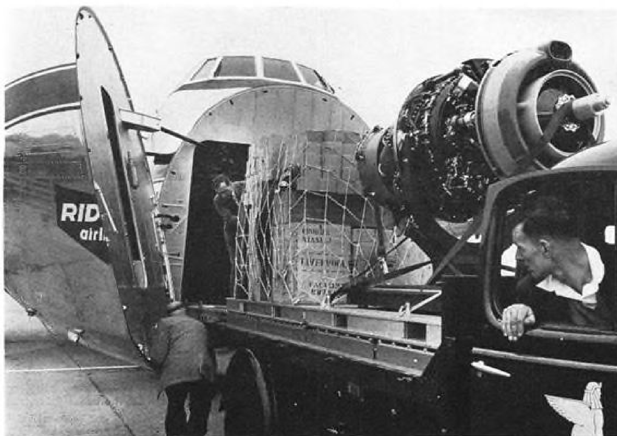
TWO MEN can load palletized freight in a short time, aided by roller strips on flooring.
