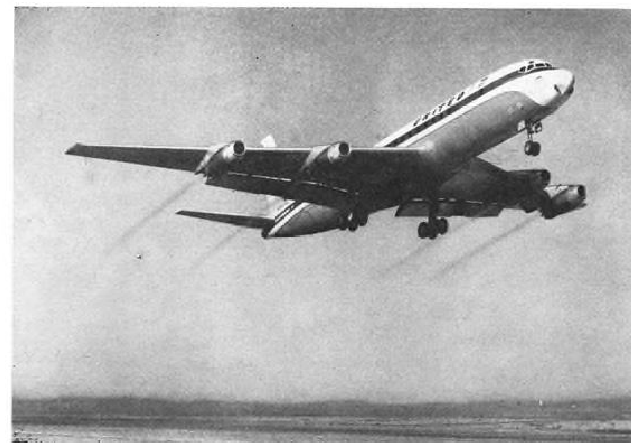
DOUGLAS DC-8 jet transport, in United Air Lines markings, makes takeoff for another in a series of flight tests. United has 40 DC-8s on order at a cost of $225 million. Aircraft's four P&W J57 turbojet engines provide total thrust of more than 40,000 lb.
