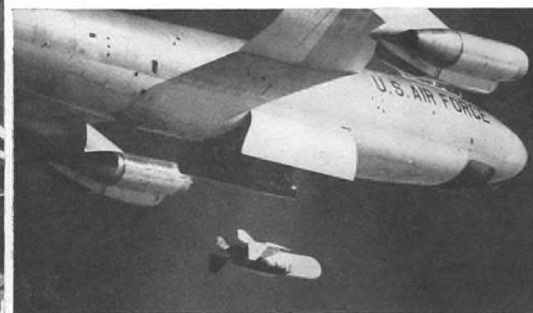
McDONNELL'S GAM-72 DECOY MISSILE, powered by General Electric's J85, will give the U.S. one of today's most effective diversionary weapons. The GAM-72 is shown above being air dropped from a B-47 during flight test.
