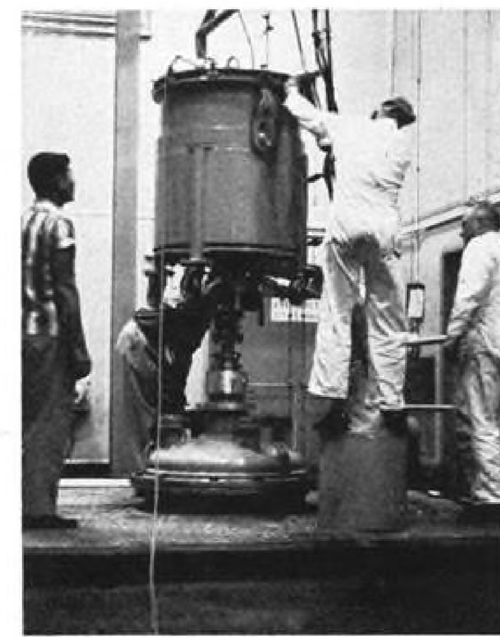
Technicians place casting can on top of the de-aerating valve and contents are dumped into the rocket case below.
