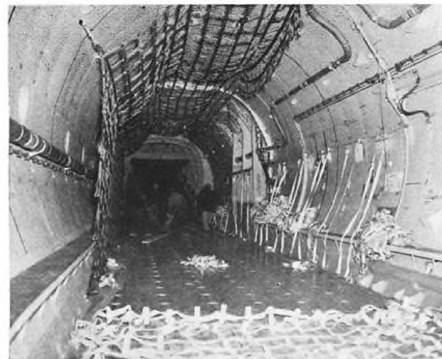
PALLETS are pushed manually into C-133A (left) by backing a conveyor-equipped flatbed trailer to the horizontal ramp. Lightweight roller conveyors are being installed in C-133A floor in background at right. Nylon straps form a cage which restrains palletized cargo.
