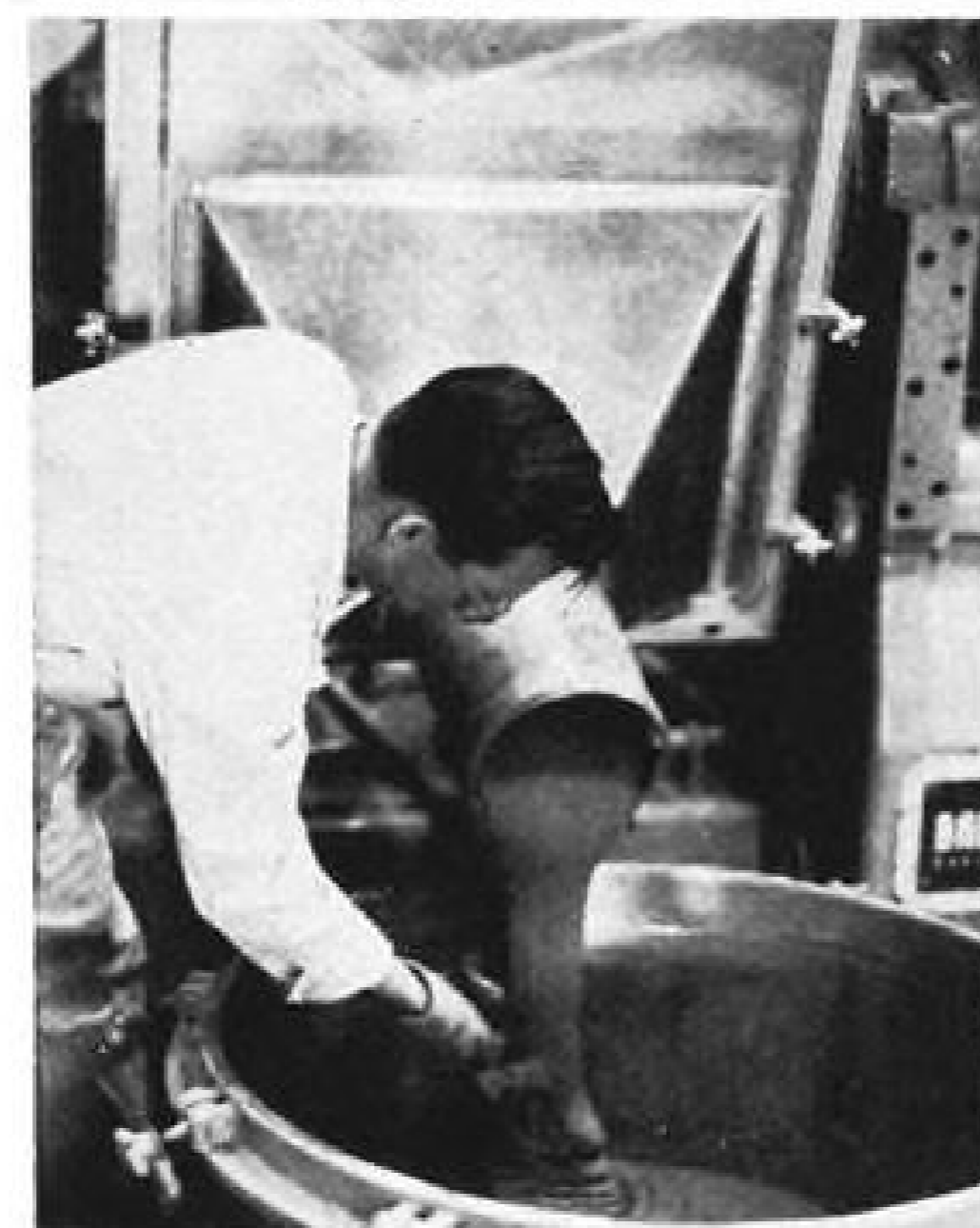
Quality and consistency of propellant is checked as it is poured into casting can.
