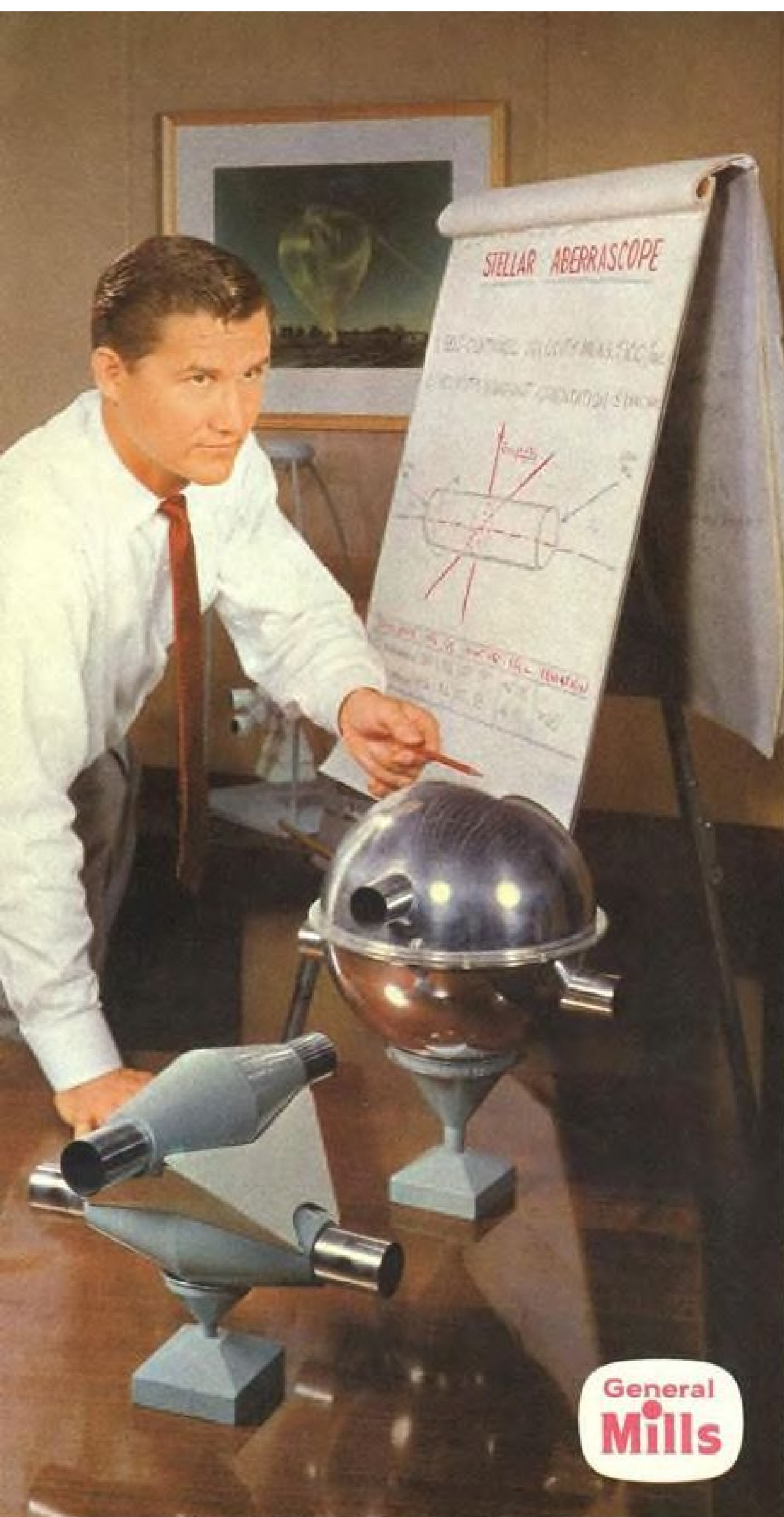
This is our R. L. Lillestrand, Project Engineer. Here he examines a model of his Stellar Aberrascopes, a multiple star tracking device which is expected to provide the measurement of space vehicle velocities to accuracies of the order of
