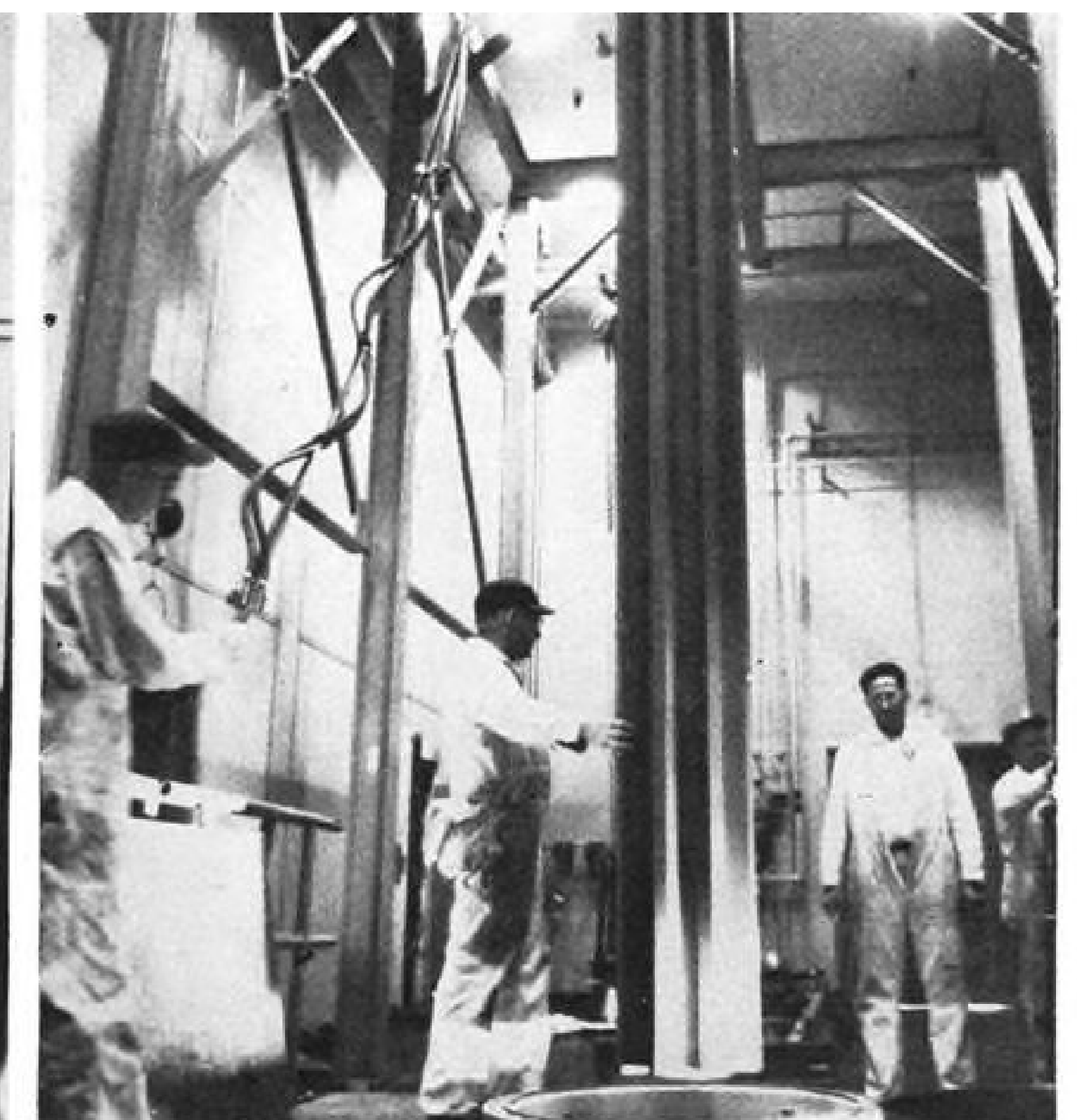
Rocket case is lowered into casting bell (left) in preparation for pouring; motor is cured in bell for 72 hr. at 170F after final pour. At right, star-shaped mandrel is poised for insertion into the case. Mandrel is coated with Teflon, which acts as a lubricant.
