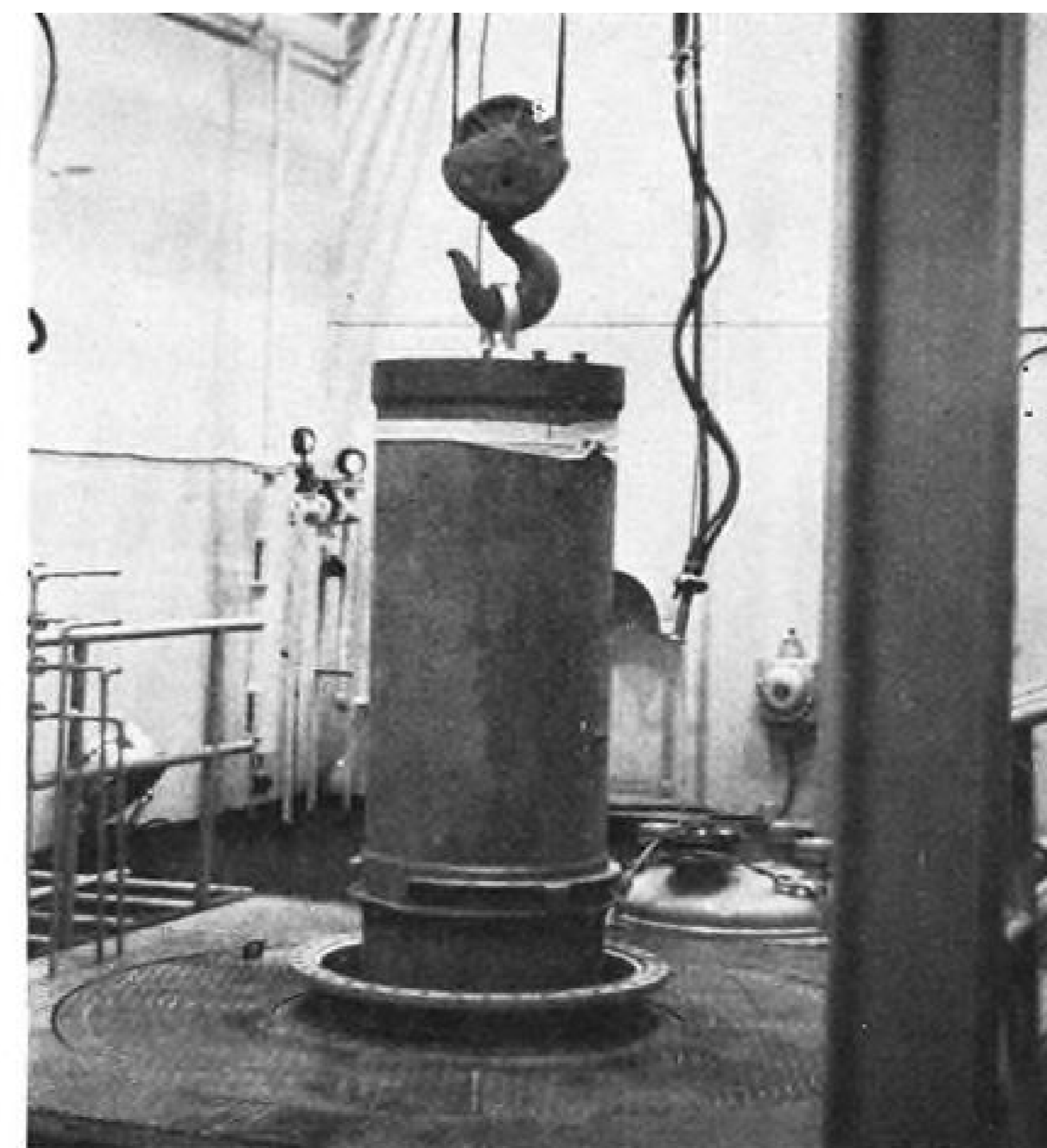
Rocket case is lowered into casting bell (left) in preparation for pouring; motor is cured in bell for 72 hr. at 170F after final pour. At right, star-shaped mandrel is poised for insertion into the case. Mandrel is coated with Teflon, which acts as a lubricant.
