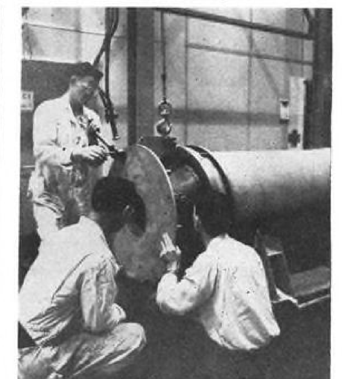
Aft head is placed in assembly to vulcanize rubber-based insulation to inside (left). At center, the rocket motor has been removed from casting bell for application of the nozzle assembly. Special jig (right) is used to align aft head assembly to rocket case.
