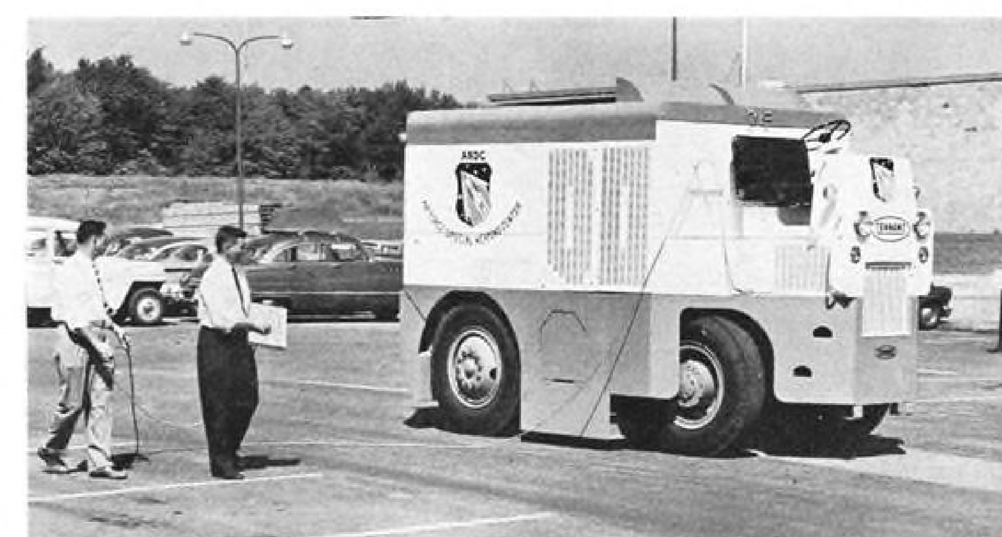
REMOTE control capability of decontamination sweeper is demonstrated with electrically connected control panel. Vehicle will be radio controlled.
