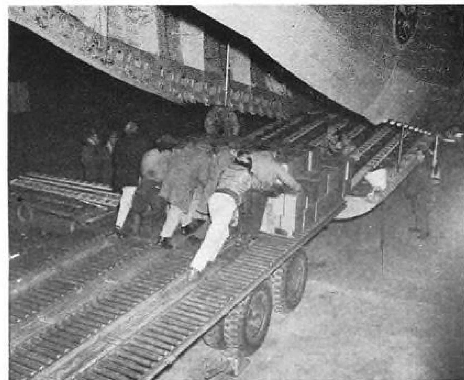
PALLETS are pushed manually into C-133A (left) by backing a conveyor-equipped flatbed trailer to the horizontal ramp. Lightweight roller conveyors are being installed in C-133A floor in background at right. Nylon straps form a cage which restrains palletized cargo.
