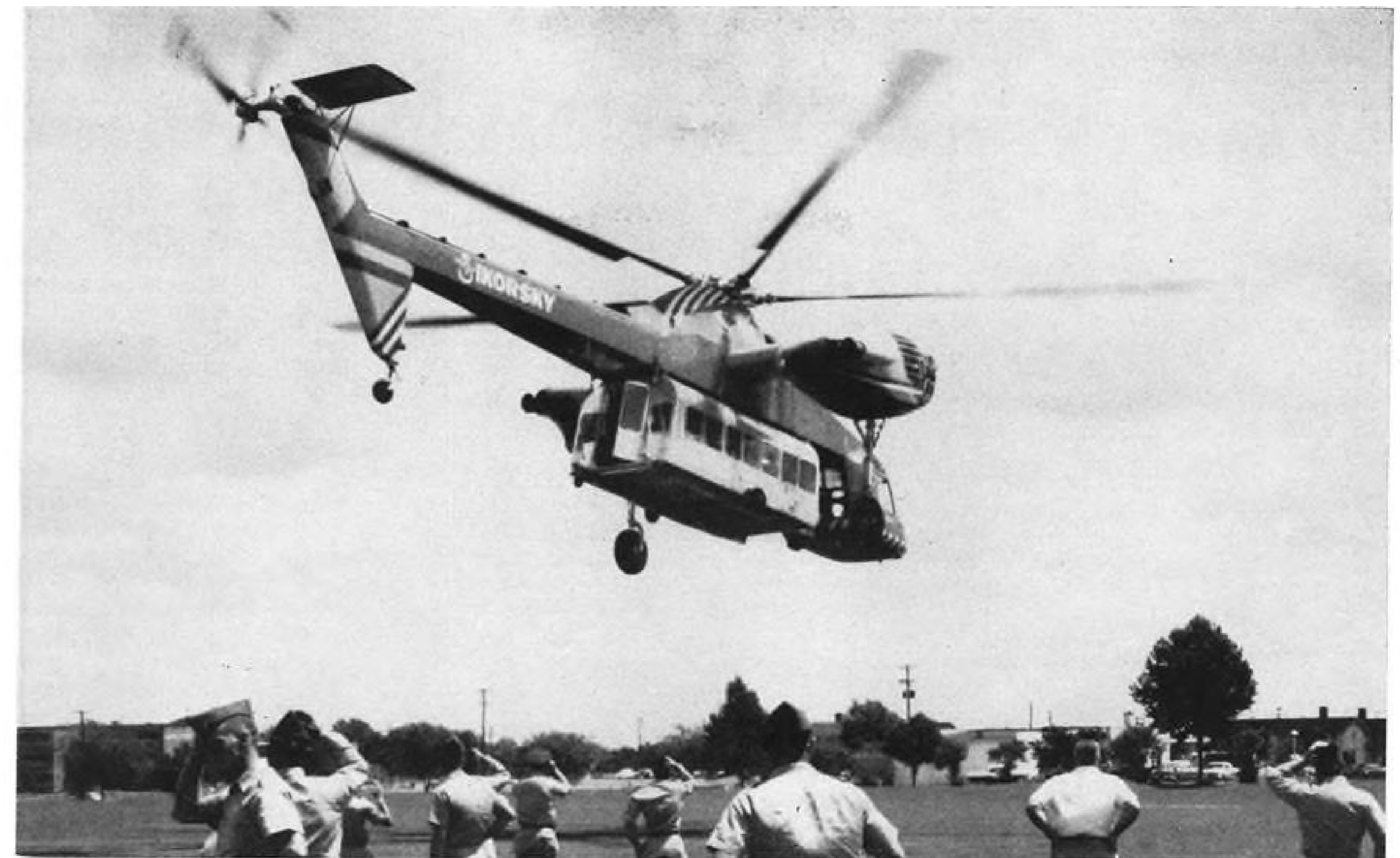
Sikorsky S-60 Carries Detachable Passenger Pod
