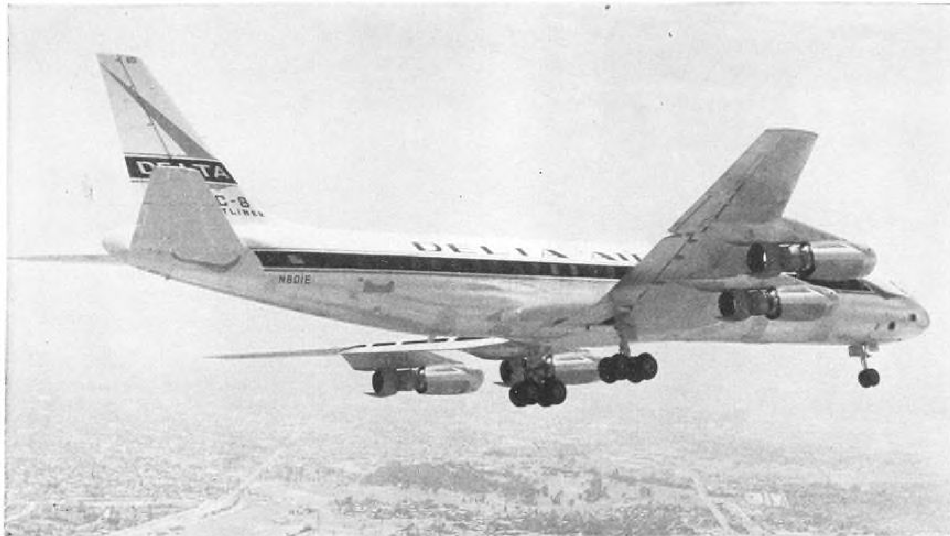
EJECTORS which are part of Douglas DC-8 sound suppressor units are extended on this Delta Air Lines transport in traffic pattern. Ejector cuts sound and increases takeoff thrust to offset loss caused by tailpipe daisy-type nozzles (AW Nov. 17, p. 91).
