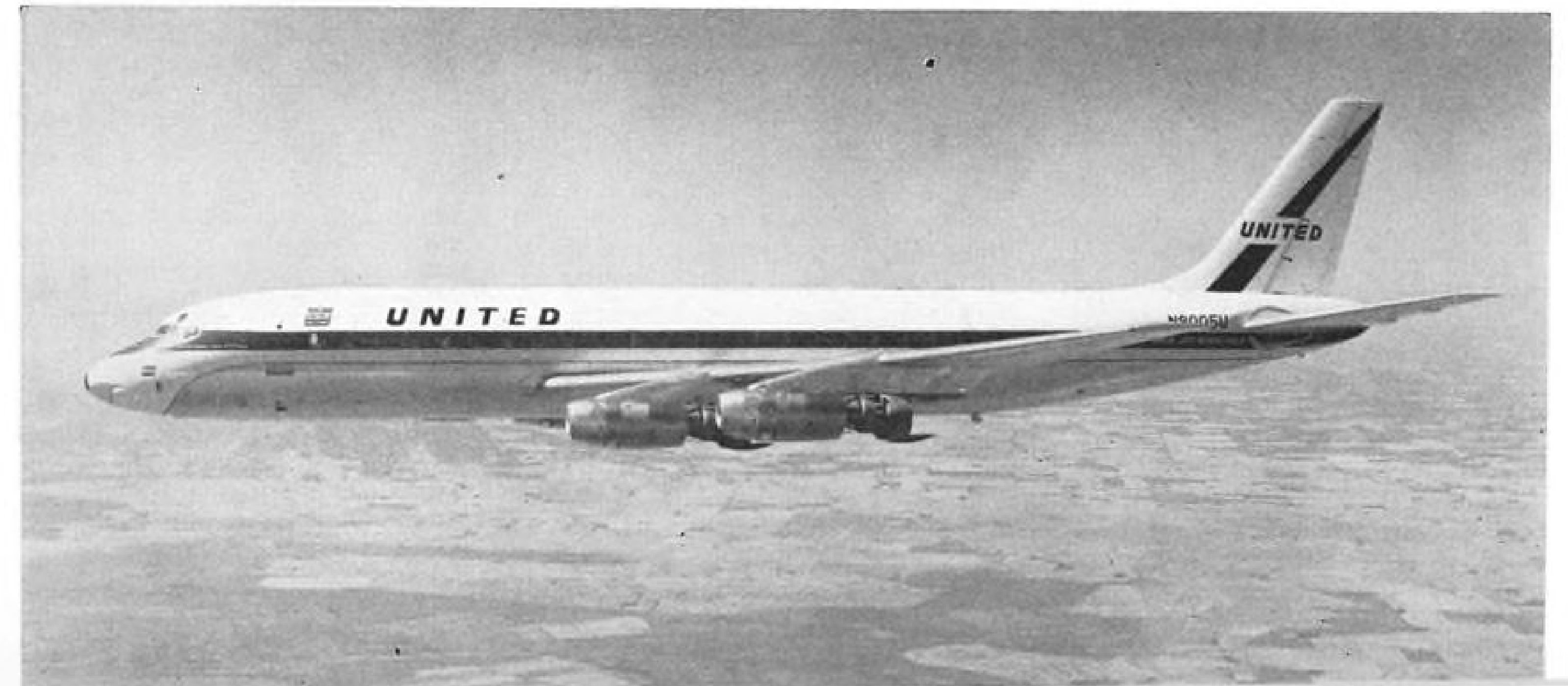
SIDE VIEW of United's DC-8 emphasizes ejector in extended position. Unit has clamshell doors which can be closed for thrust reversing action during landings. N8005U is powered by four Pratt & Whitney JT3C-6 engines rated at 13,000 lb. thrust each.
