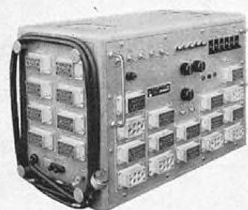
3. PORTABLE MAINTENANCE JUNCTION BOX allows functional equipment groups of complex radar sets to be interconnected on a maintenance bench. The mobile box provides accurate testing for comprehensive subsystems.
