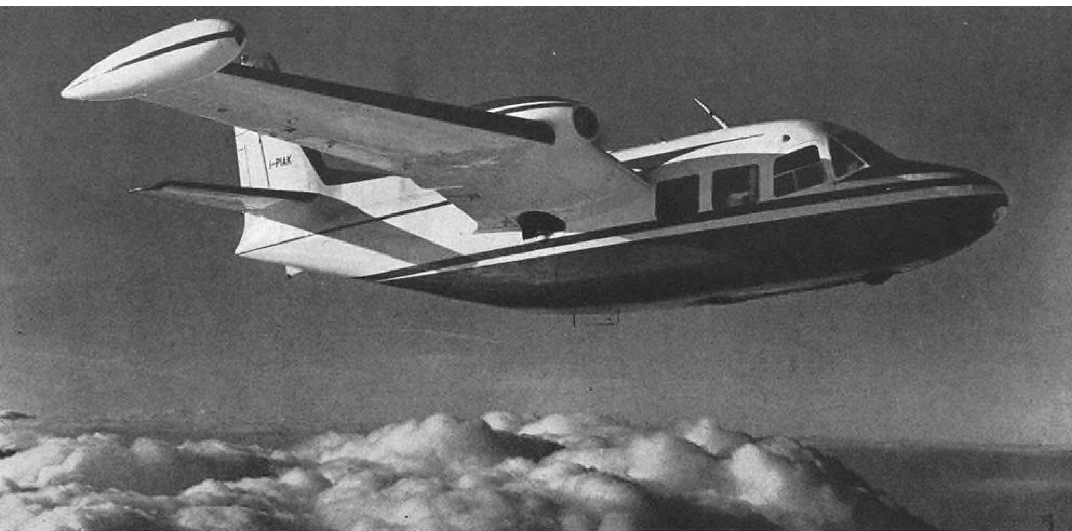
PIAGGIO P.166 has a range of 1,155 stat. mi., with 30 min. fuel reserve. Cruising speed runs to 208 mph. Gross weight is 8,100 lb.
