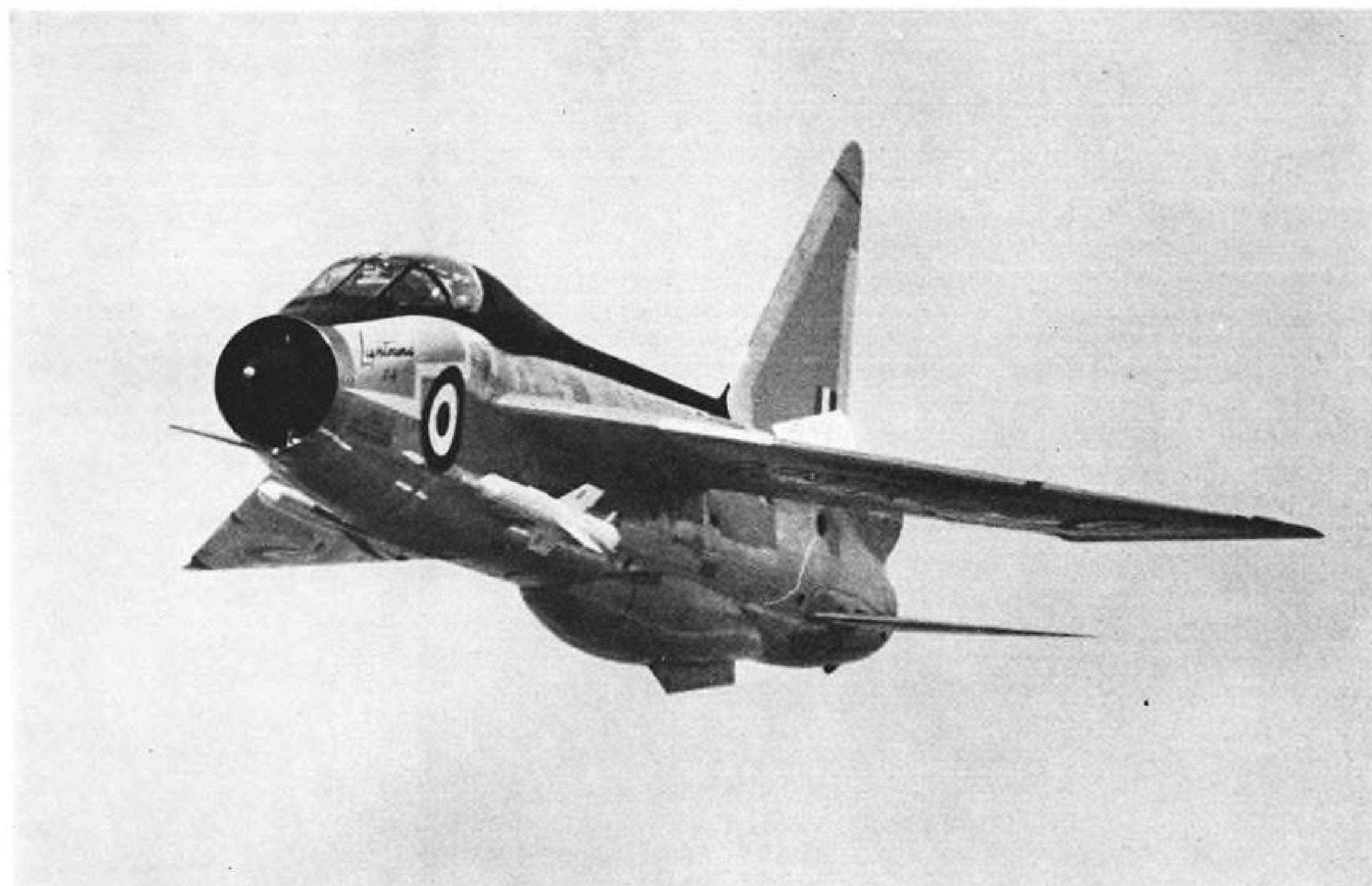
Blasting across the field like a fighting bull across the ring, the English Electric Lightning T.4 supersonic trainer shows the bulged form of area-ruling near the cockpit. The aircraft is basically a two-seat Lightning. The trainer is carrying two de Havilland Firestreak infrared homing missiles. The ventral tank carries extra fuel. The aircraft can also mount a Napier Scorpion rocket for boosting performance at altitude. Powerplants are twin Rolls-Royce Avons with afterburners.
