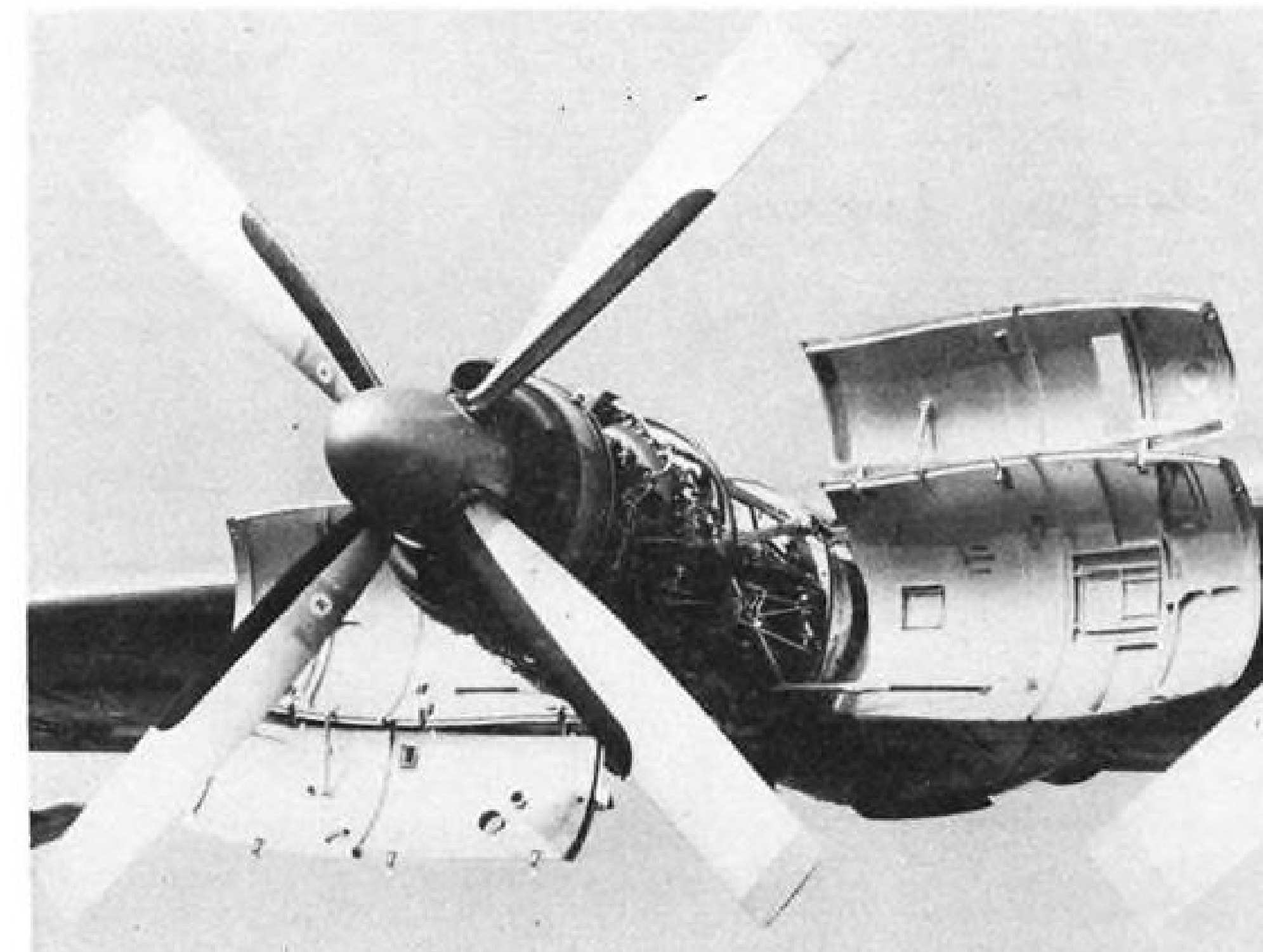
ONE of four Rolls-Royce Dart turboprop installations on the Armstrong Whitworth AW 650 Argosy transport shows the cowling arrangement, designed for accessibility.
