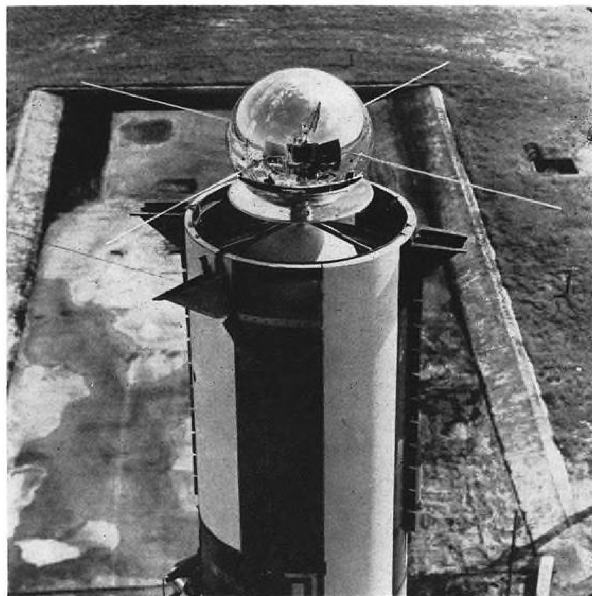
FOUR ANTENNAE of Vanguard III satellite are extended for prelaunch tests. Notched strips on vehicle fairing break up wind currents on the launch pad and are jettisoned after launch. Saucer-shaped fixture under satellite protects it from heat and smoke.
