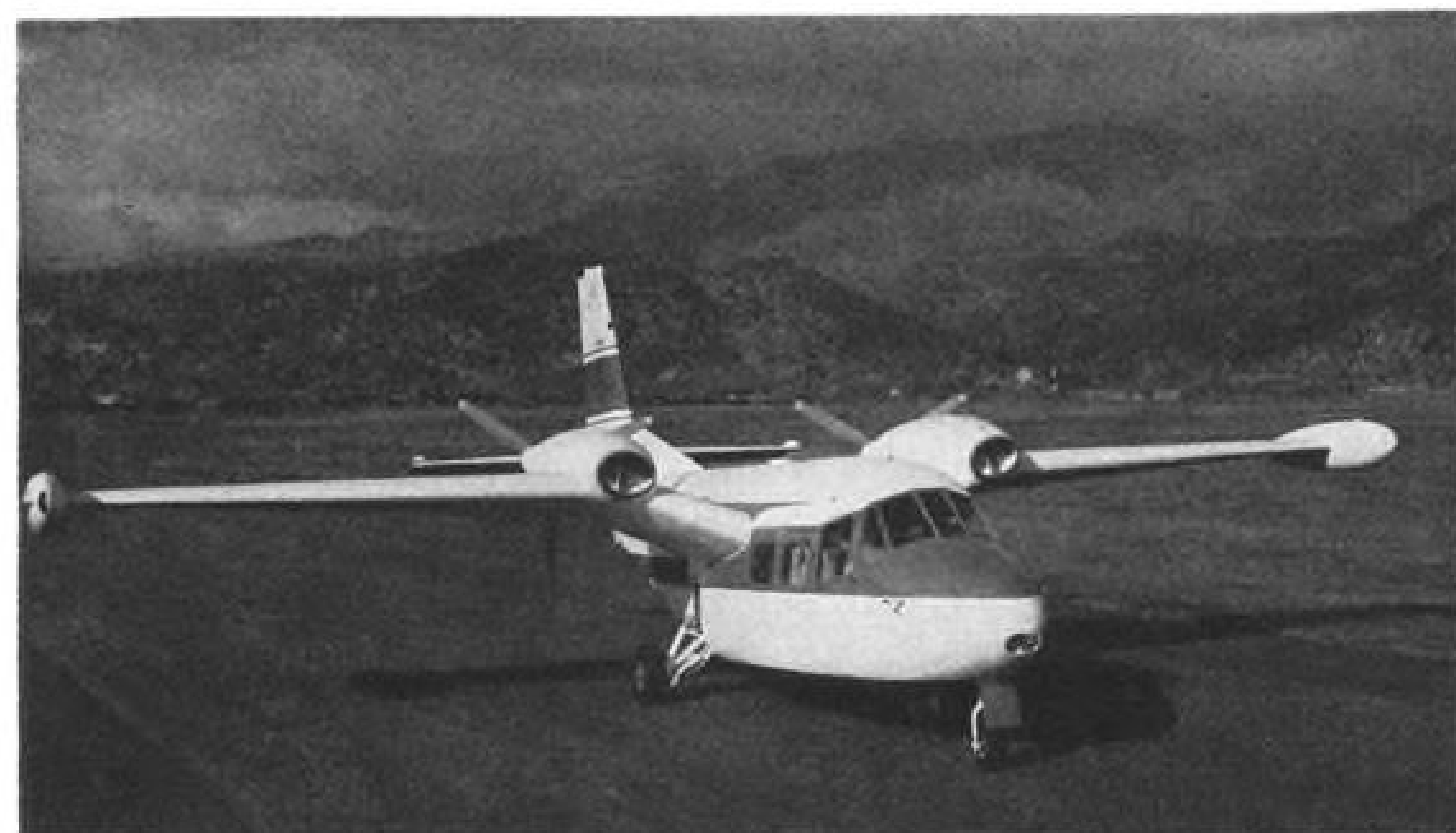
P.166 incorporates the same gull wing, horizontal tail, landing gear and pusher powerplant installation of the P.136 Royal Gull amphibian.
