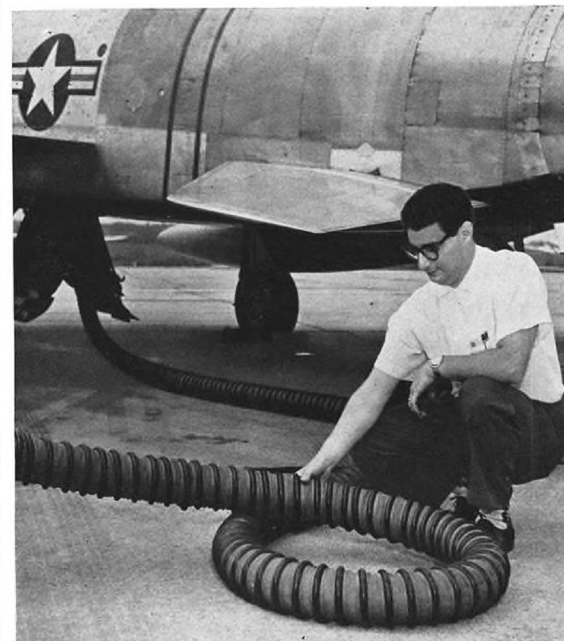
Under flexing tests conducted by Wright Air Development Center engineers, this improved ducting showed no damage after 1,000 flexing cycles, 380-390F temperature, and 90-pound-per-minute air flow.
