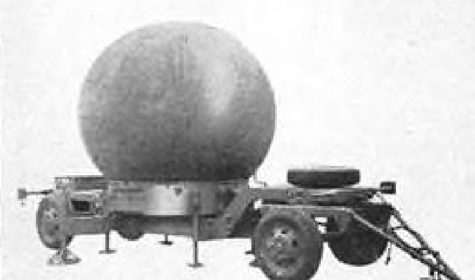
7. RADAR-TRACKER INTERROGATOR OA-1333/MSW-2 with radome (portion of an all-weather system). Developed for Corporal System as a low-priced, high-accuracy and performance radar, uses can now include range instrumentation.
