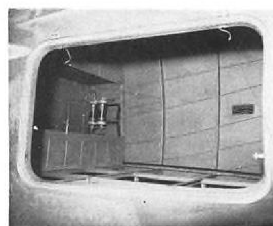
AIRPLANE'S luggage compartment is of 63.6 cu. ft. capacity; takes 300 lb. of cargo.
