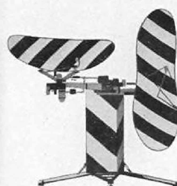
5. LIGHTWEIGHT GCA RADAR SET, QUADRADAR, AN/FPN-33 is a highly mobile surveillance, approach, landing and taxi system that has achieved an enviable world-wide record of operation with both military and civilian users.
