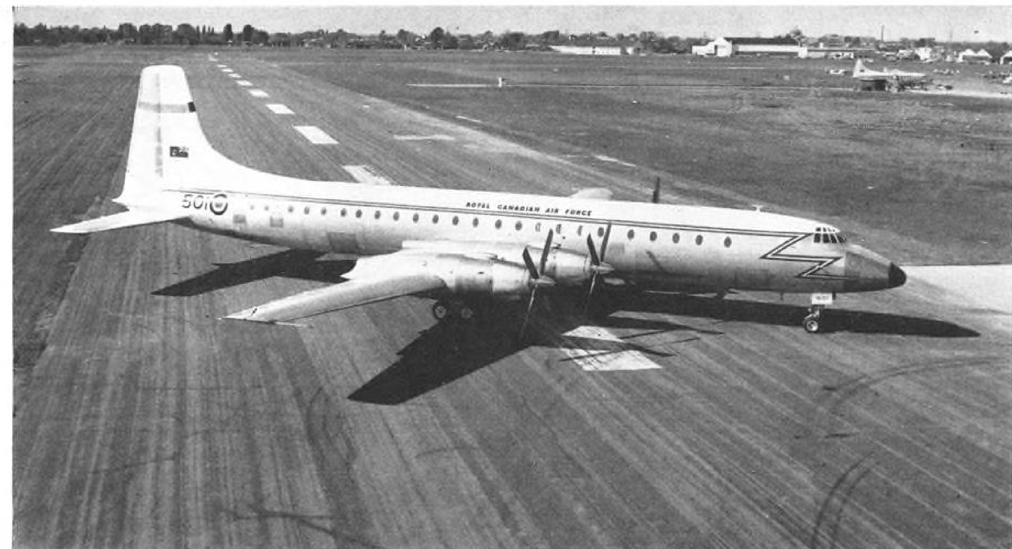
ROLLS-ROYCE Tyne 12 Mark 515/10 turbine engines power the CL-44D-4. Each engine generates 5,305 eshp. at sea-level takeoff. Three-view below shows sweep of swing-tail. The CL-44 is a cantilever low-wing airplane of two-spar box wing structure.
