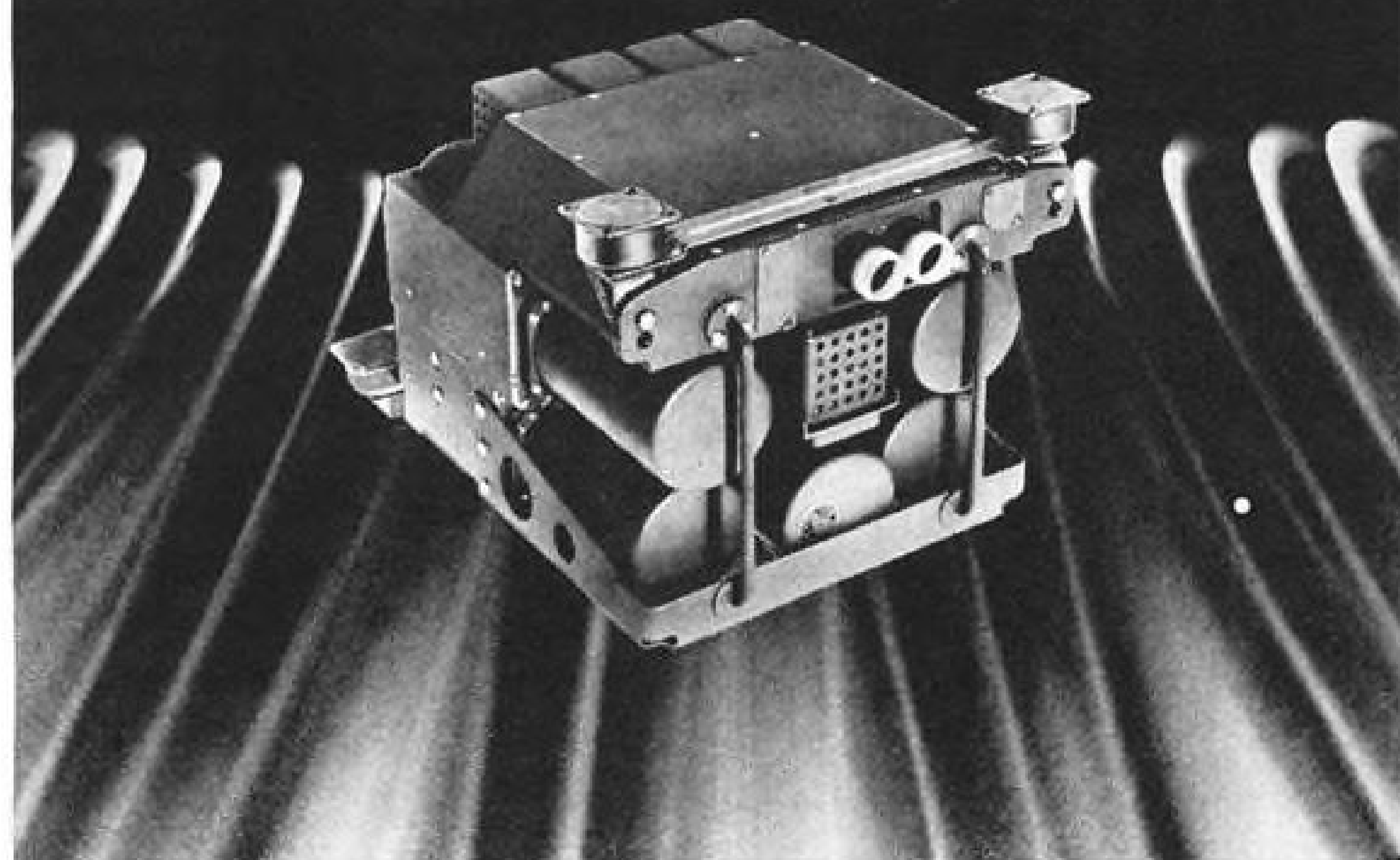
• AiResearch Central Air Data Computer for North American's A3J, Navy's first weapon system, provides information dealing with bombing, navigation, engine inlet control, radar, automatic flight control and cockpit instrumentation.
