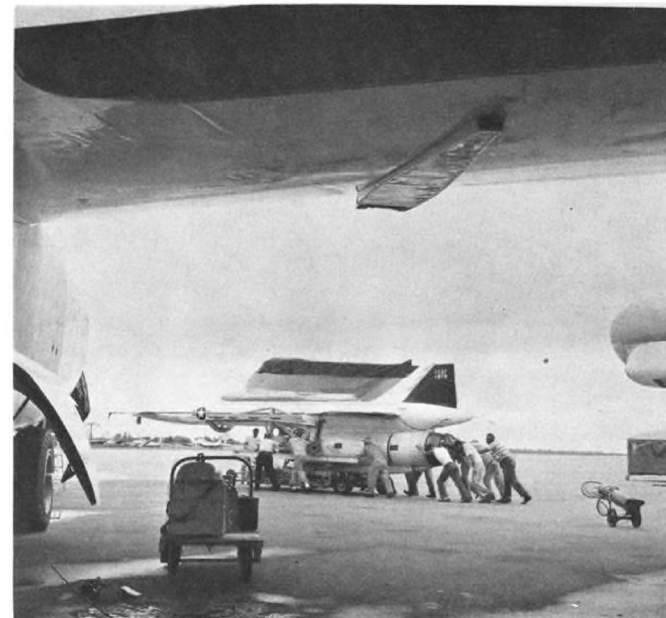
GAM-77 missile is pushed on ground transporter to combined systems checkout area after being unloaded from a Douglas C-124 which flew the missile from Downey, Calif., to Eglin AFB, Fla. Fitting on B-52 wing (above) is for the air-launch pylon.
