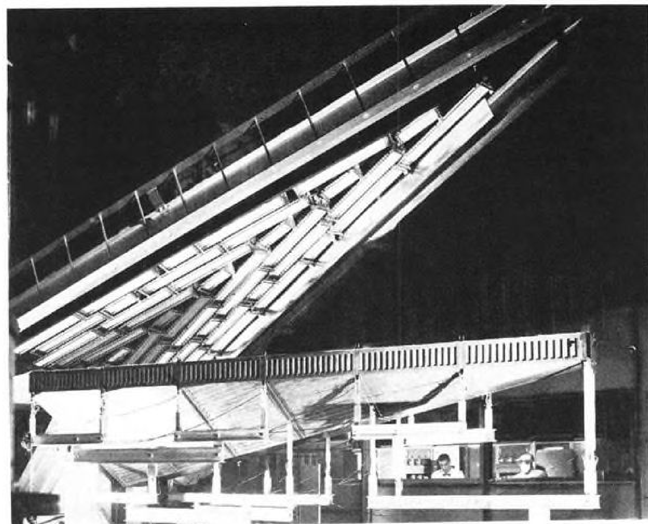
QUARTZ LAMPS are used to heat the bottom of the re-entry glider structural model shown inverted above. Air loads on the glider are simulated at the same time through the "whiffle-tree" arrangement of levers hanging below the model.
