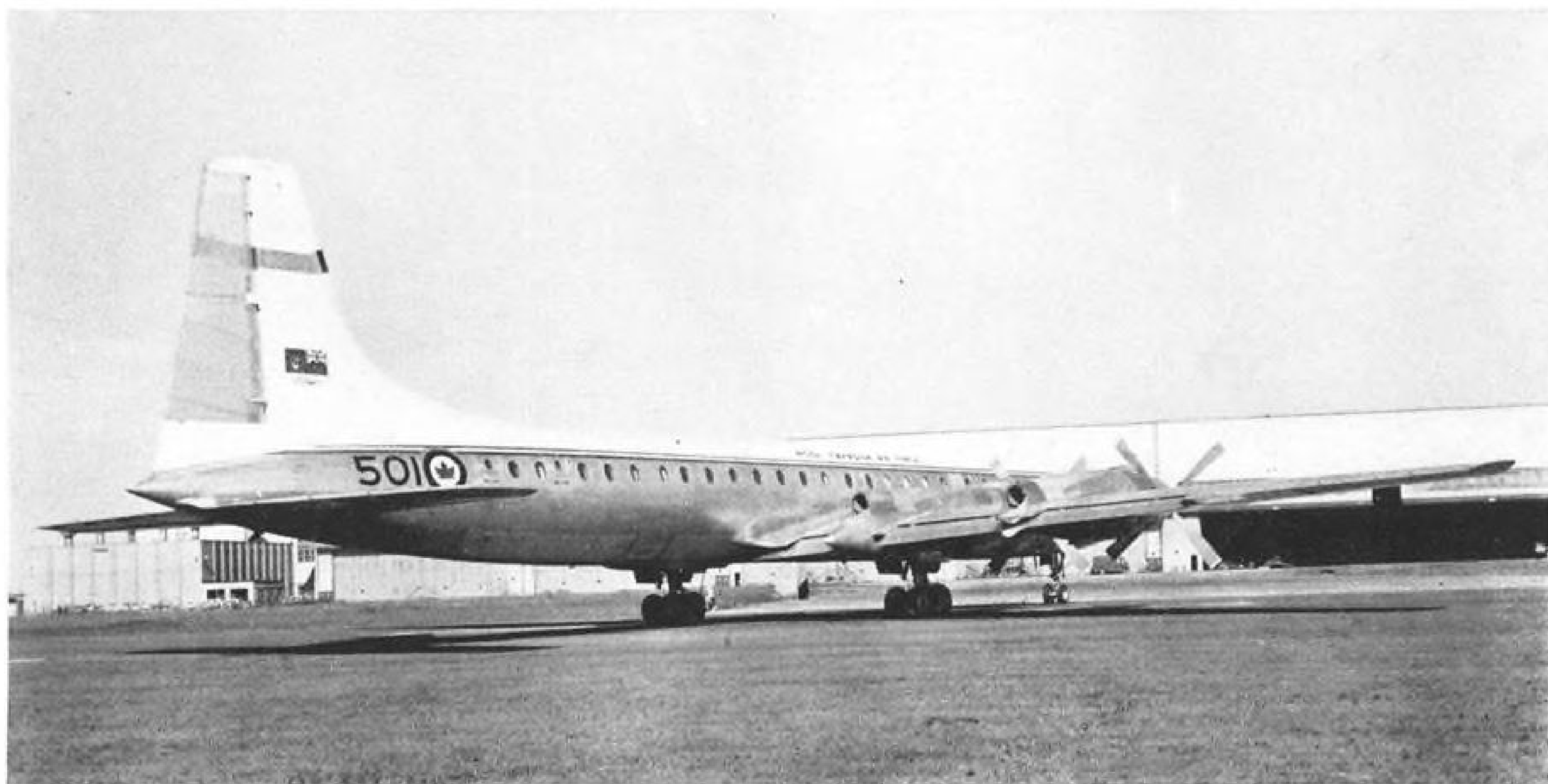
PROTOTYPE Canadair CL-44D-4 turbine-powered cargo-troop transport, one of 12 CC-106s ordered by the Royal Canadian Air Force, is scheduled to make its first flight this month. This aircraft is a side-loading version; the first swing-tail will be No. 9 aircraft.
