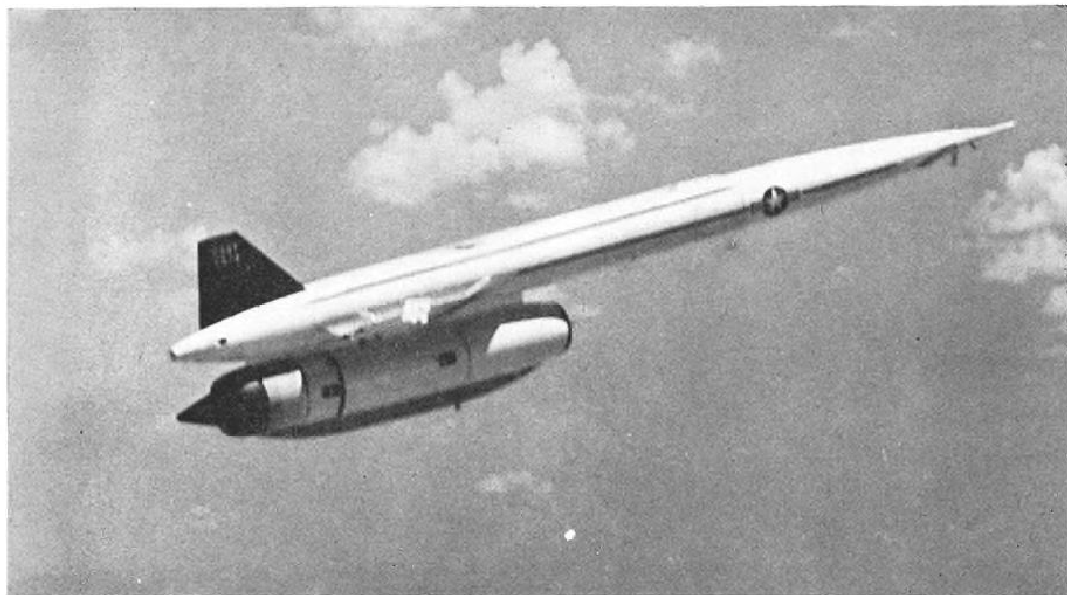
HOUND DOG air-launched missile, powered by 7,500-lb.-thrust Pratt & Whitney J52 turbojet engines, is fired at Eglin AFB.
