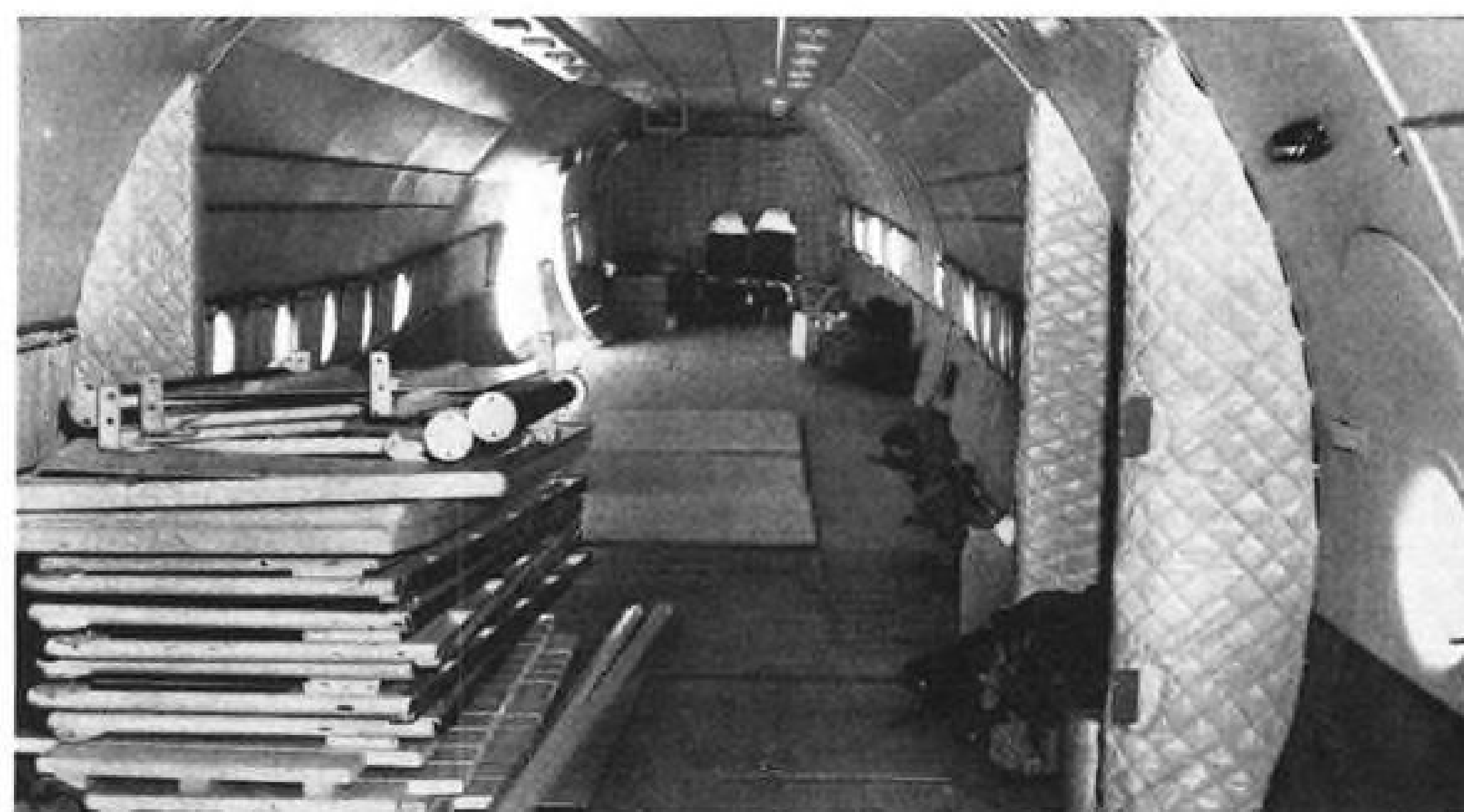
INTERIOR of An-10A flown to U. S. (left) has all but 16 of its 100 seats and all its carpeting removed. Wall and ceiling furnishings are standard for passenger use. Four padded sections against the wall support galley bulkheads. Long strips with tie-down rings attached may be screwed into floor to secure cargo load. Wing carry through structure protrudes slightly into the cabin ceiling. Passenger seats (right) have individual lights mounted on headrest. Three buttons on arm of each seat allow the passenger to call the stewardess, listen to radio with a small earphone and operate his reading light. Movies also are shown on the forward bulkhead.
