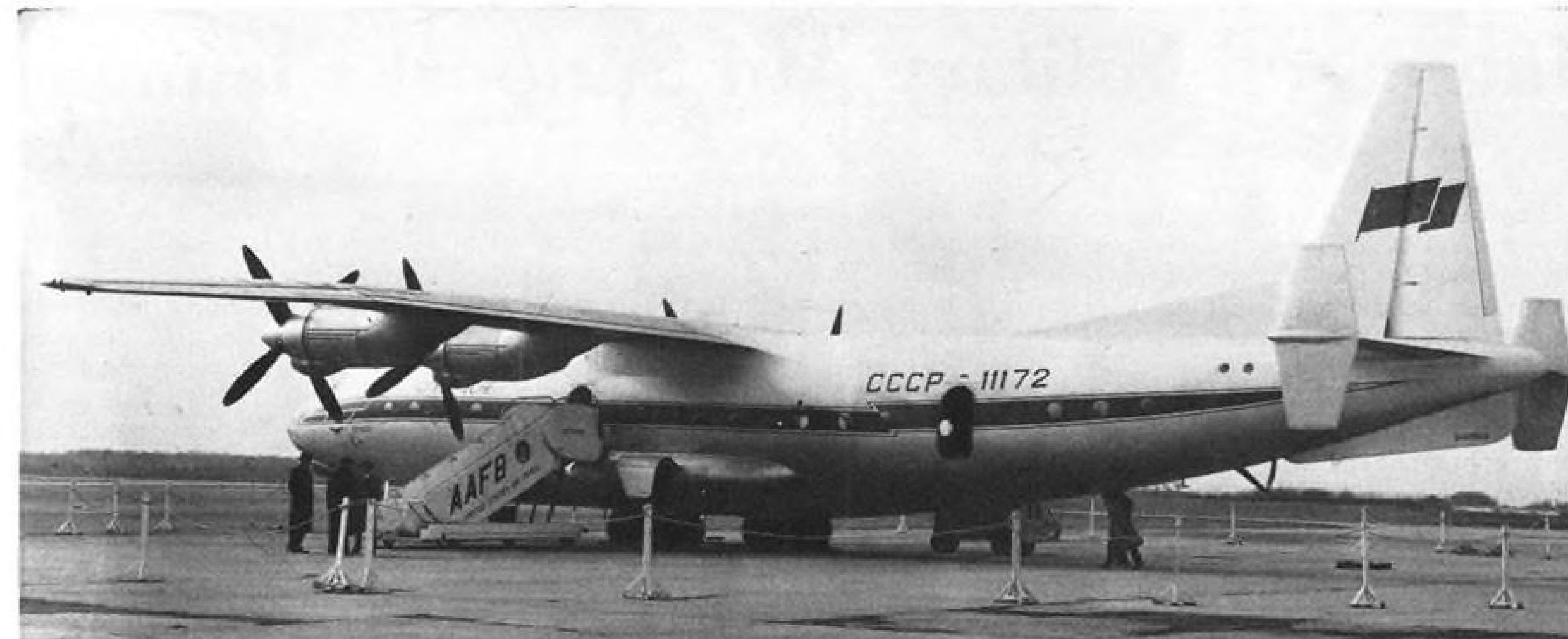
DIRECTIONAL stability problems encountered with the Ukraina series is indicated by the addition of large vertical surfaces on the tips of horizontal tail on the An-10A. The dorsal and ventral fins were on the An-10.
