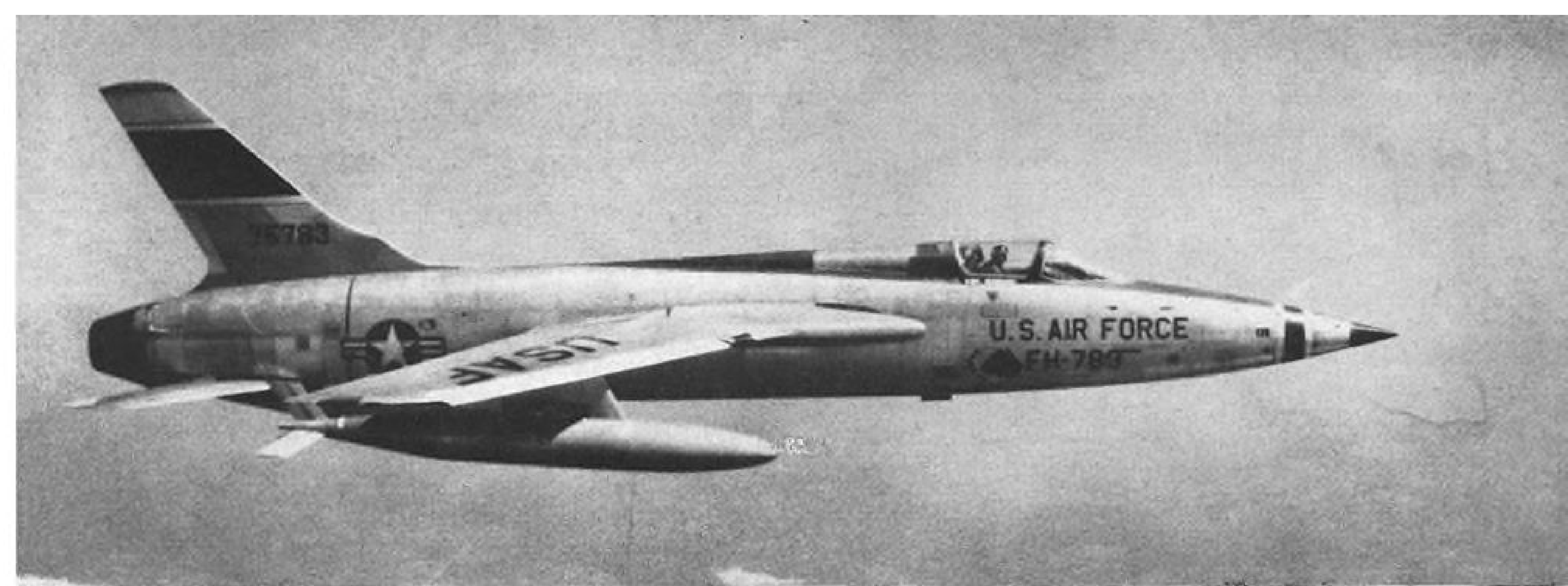
F-105 can carry three 450-gal. external tanks plus bomb bay tanks. Airplane is approaching 2,000 stat. mi. range without refueling.
