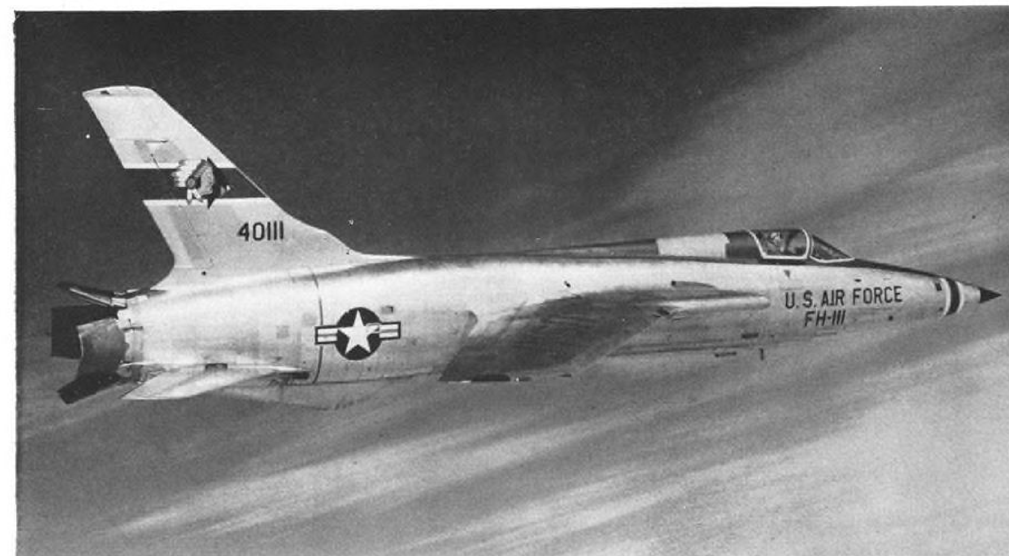
SUPERSONIC all-weather Republic F-105 has flown faster than Mach 2 at 38,000 ft. Petal-type speed brakes operate at Mach 2.
