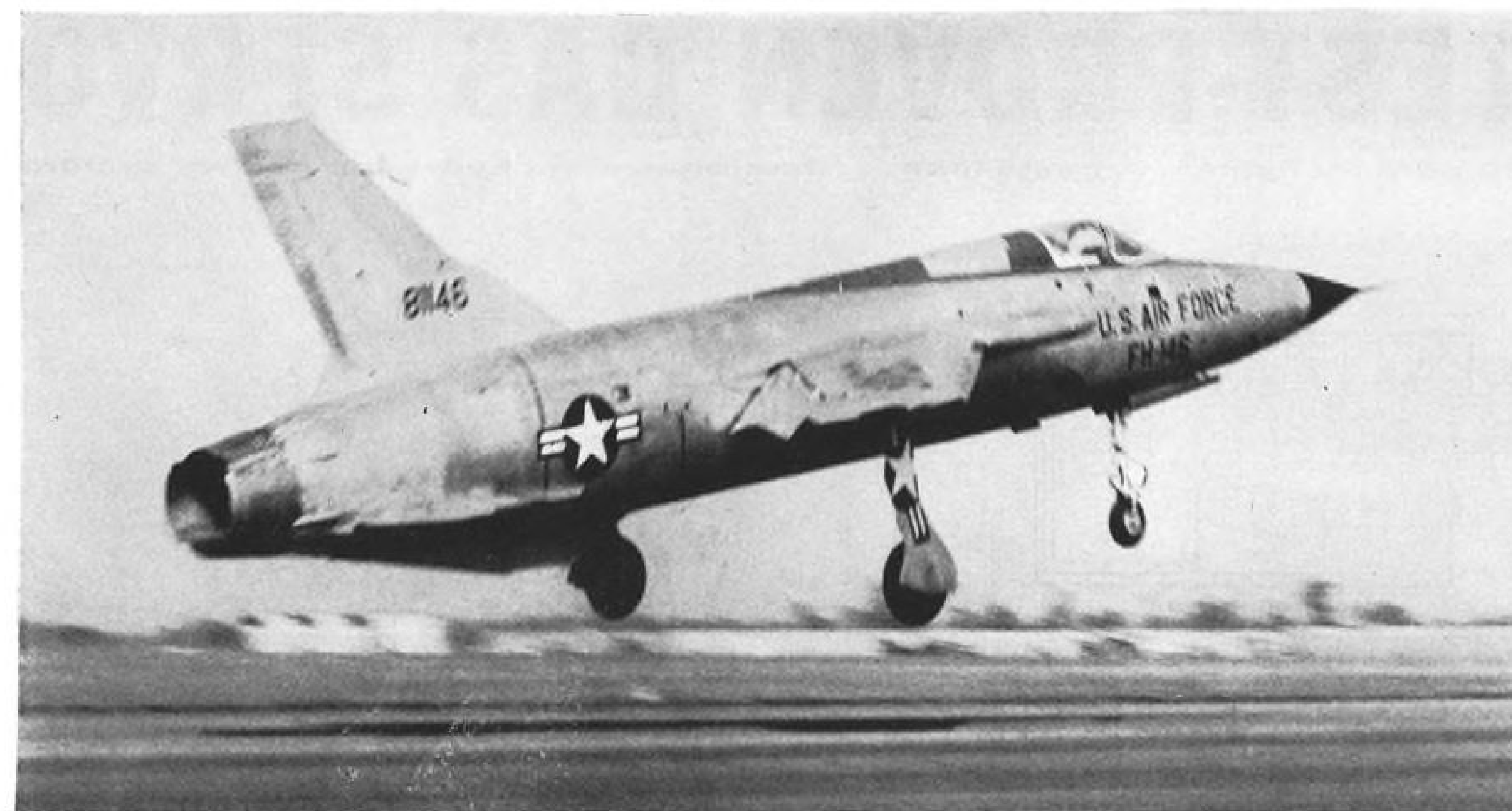
F-105 has climbed to 8,200 ft. in 55 sec. from a standstill. Following gear retraction, the Thunderchief has climbed to 40,000 ft. in 2 min. 1 sec. The Pratt & Whitney J75 powerplant is expected eventually to reach the 30,000-lb. thrust range.
