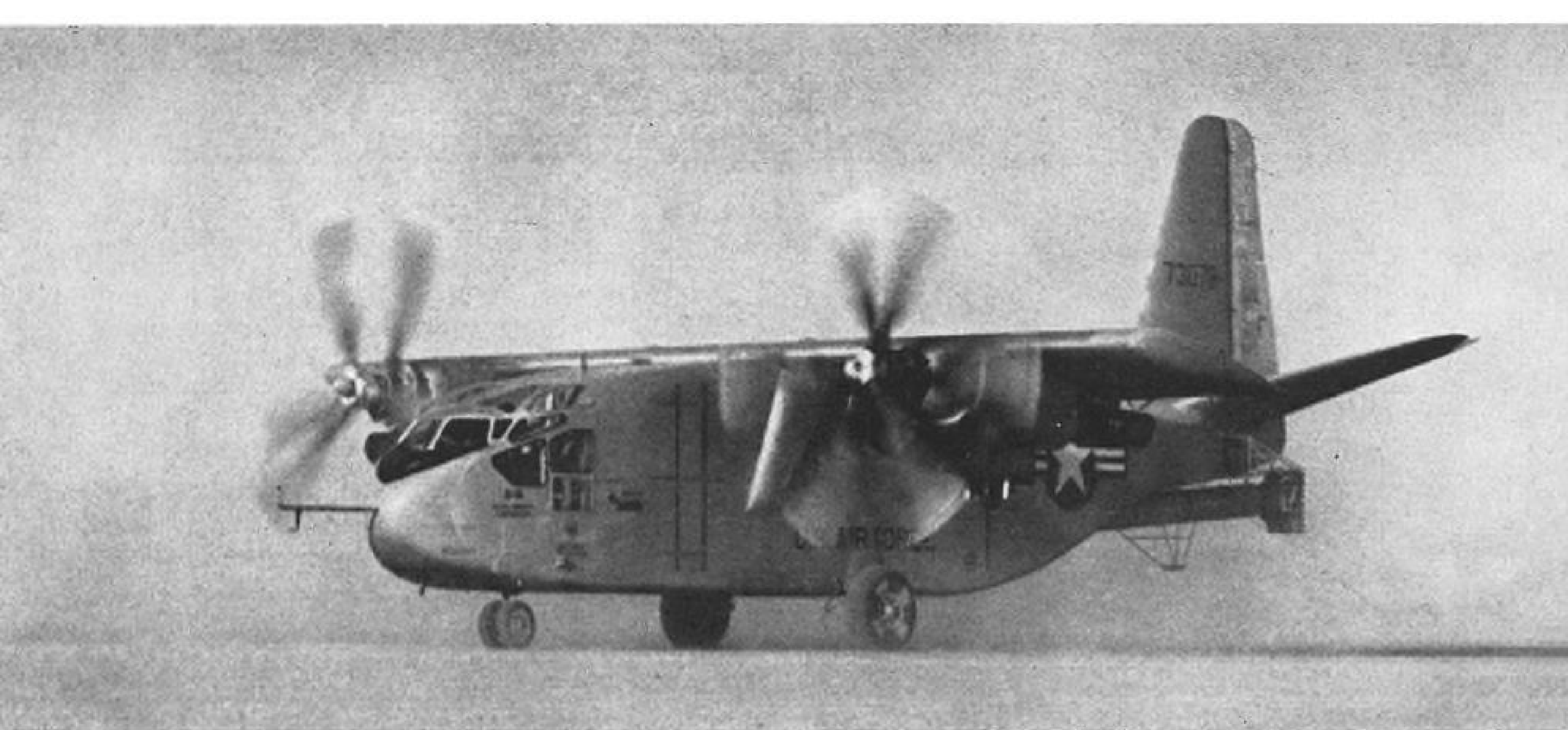
Hiller X-18 makes a conventional takeoff at Edwards AFB, Calif., with wing fixed in normal position. Vehicle weighs 16½ tons.
