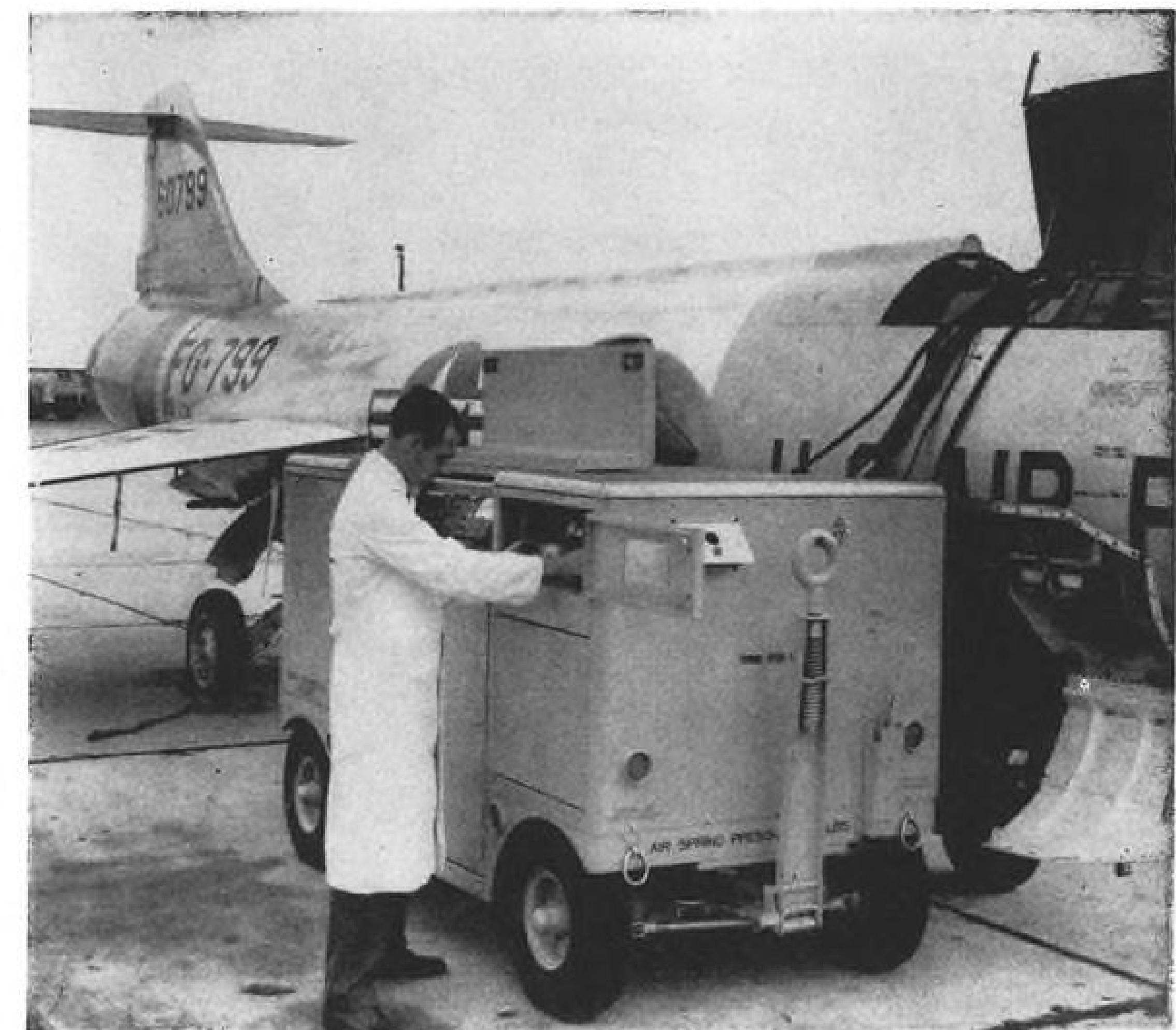
HONEYWELL automatic systems analyzer, shown in use on an F-104, will be used to check out and trouble-shoot flight control system and air data computer on F-101B. Air Force tests indicate new analyzer will slash checkout time by at least 80%.
