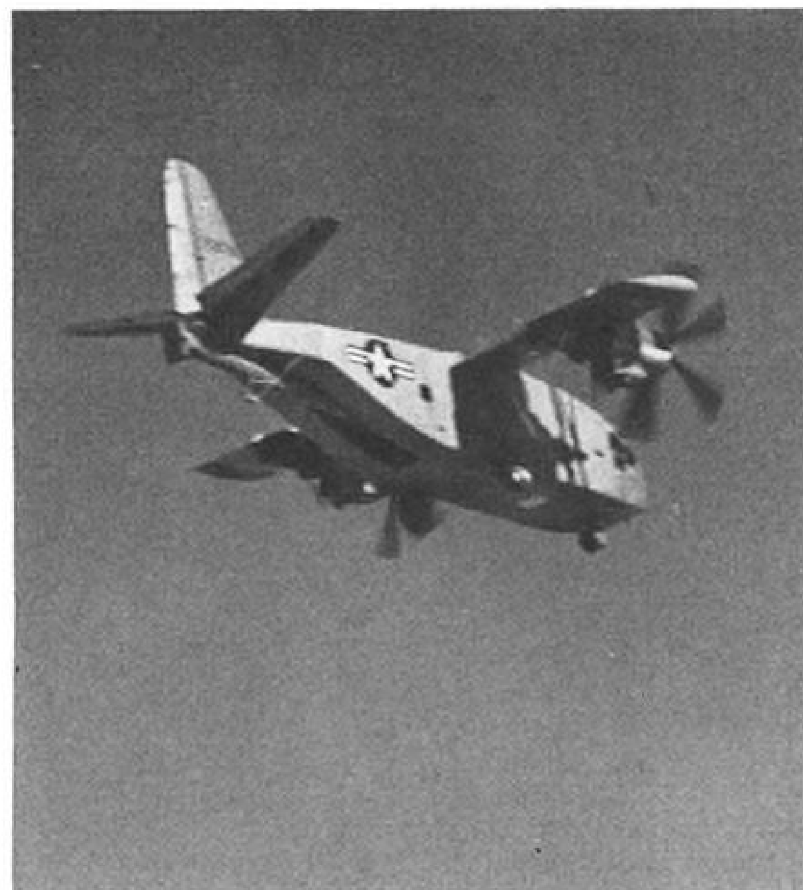
Tilt-wing X-18 climbs out (left) during test flight with wing locked in horizontal attitude. At right the vehicle gains altitude. Air Force chase plane is just above the horizon. Diverter pipe at tail provides jet blast for pitch control during hover and transition.
