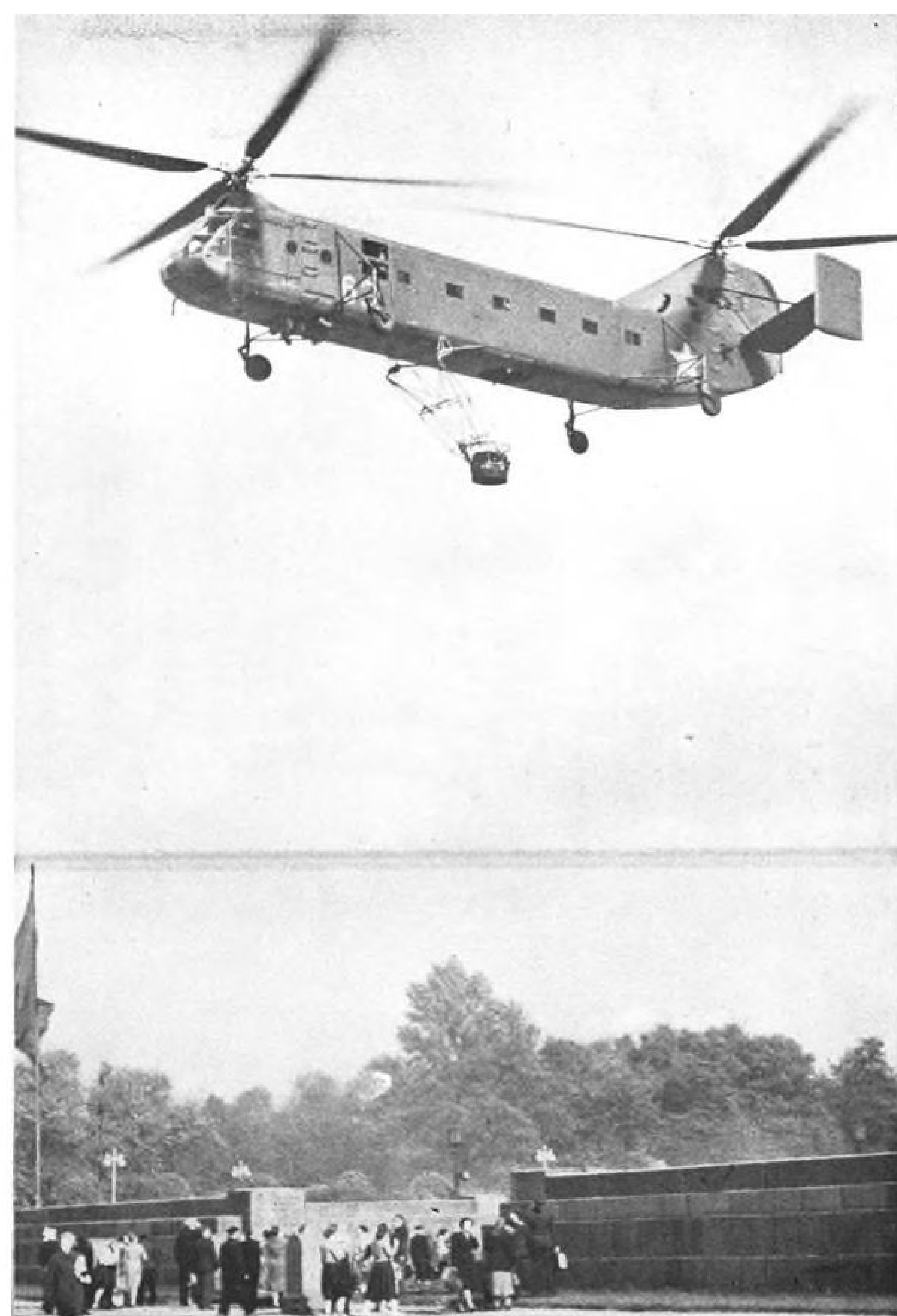
YAK-24 has carried a four metric ton payload to an altitude of 9,521 ft.
