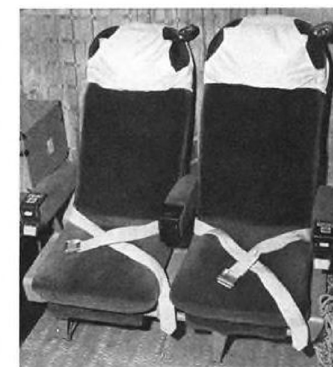
INTERIOR of An-10A flown to U. S. (left) has all but 16 of its 100 seats and all its carpeting removed. Wall and ceiling furnishings are standard for passenger use. Four padded sections against the wall support galley bulkheads. Long strips with tie-down rings attached may be screwed into floor to secure cargo load. Wing carry through structure protrudes slightly into the cabin ceiling. Passenger seats (right) have individual lights mounted on headrest. Three buttons on arm of each seat allow the passenger to call the stewardess, listen to radio with a small earphone and operate his reading light. Movies also are shown on the forward bulkhead.
