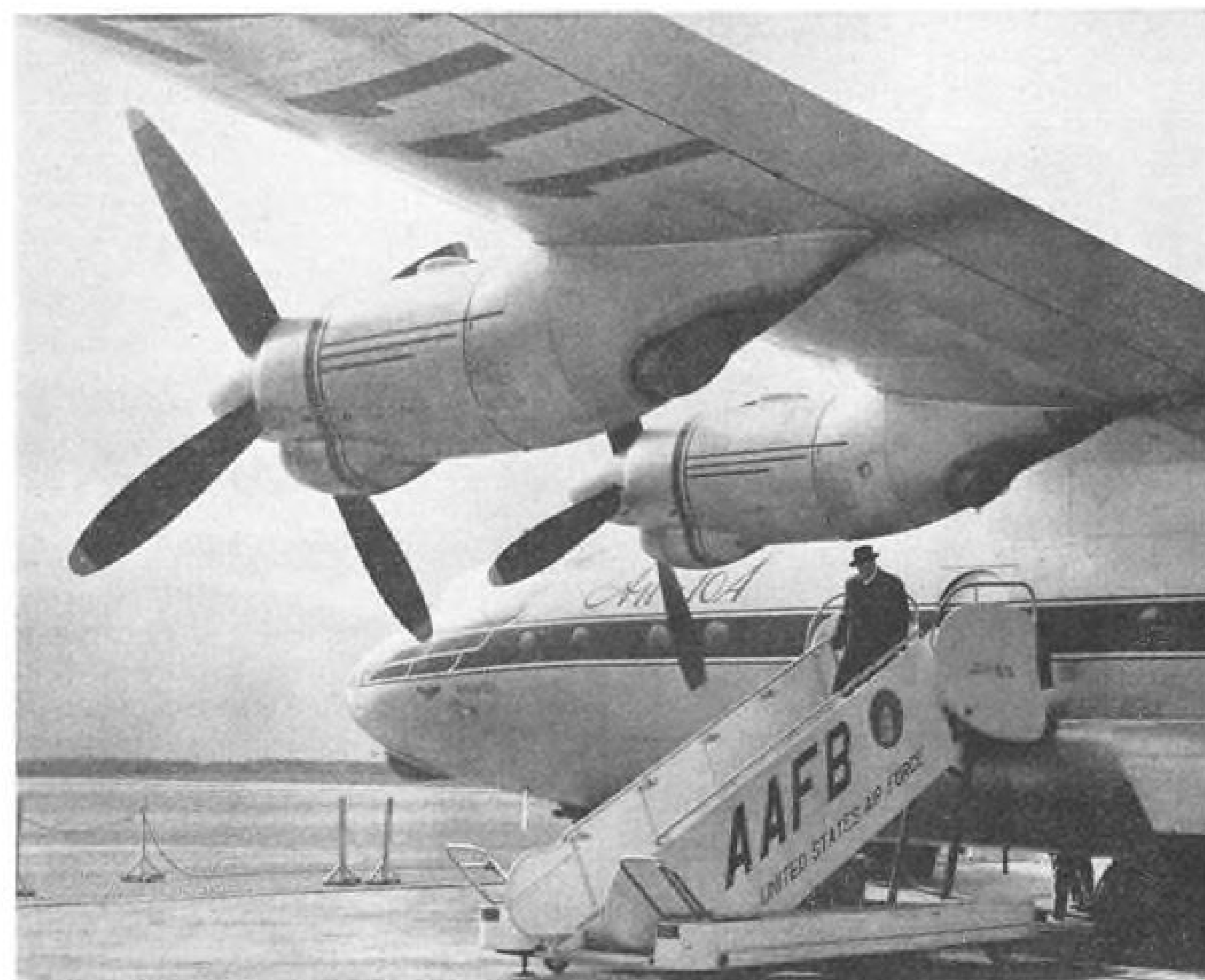
IVCHENKO 4,000 hp.-plus turboprop engines on the An-10A are the same as those used on the Il-18 Moscow transport. The early An-10 Ukraina had Kuznetsov turbine engines of approximately the same power. High wing arrangement reduces the amount of dust and dirt blown up during operation from unimproved fields.
