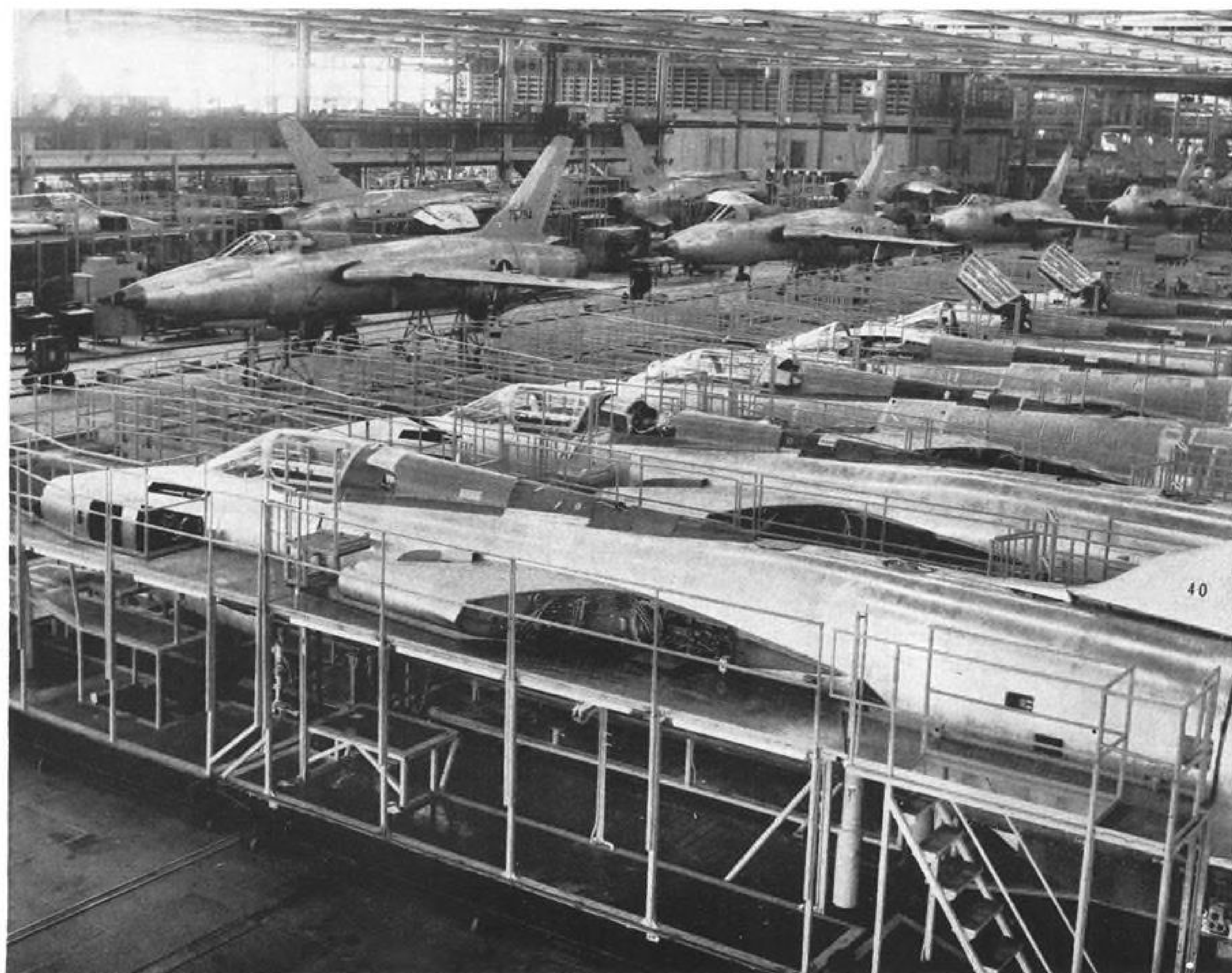
ASSEMBLY line at Republic's Farmingdale, N. Y., plant. Fighter-bomber is 63 ft. 1 in. long. Span is 34 ft. 11 in.; height is 19 ft. 8 in.
