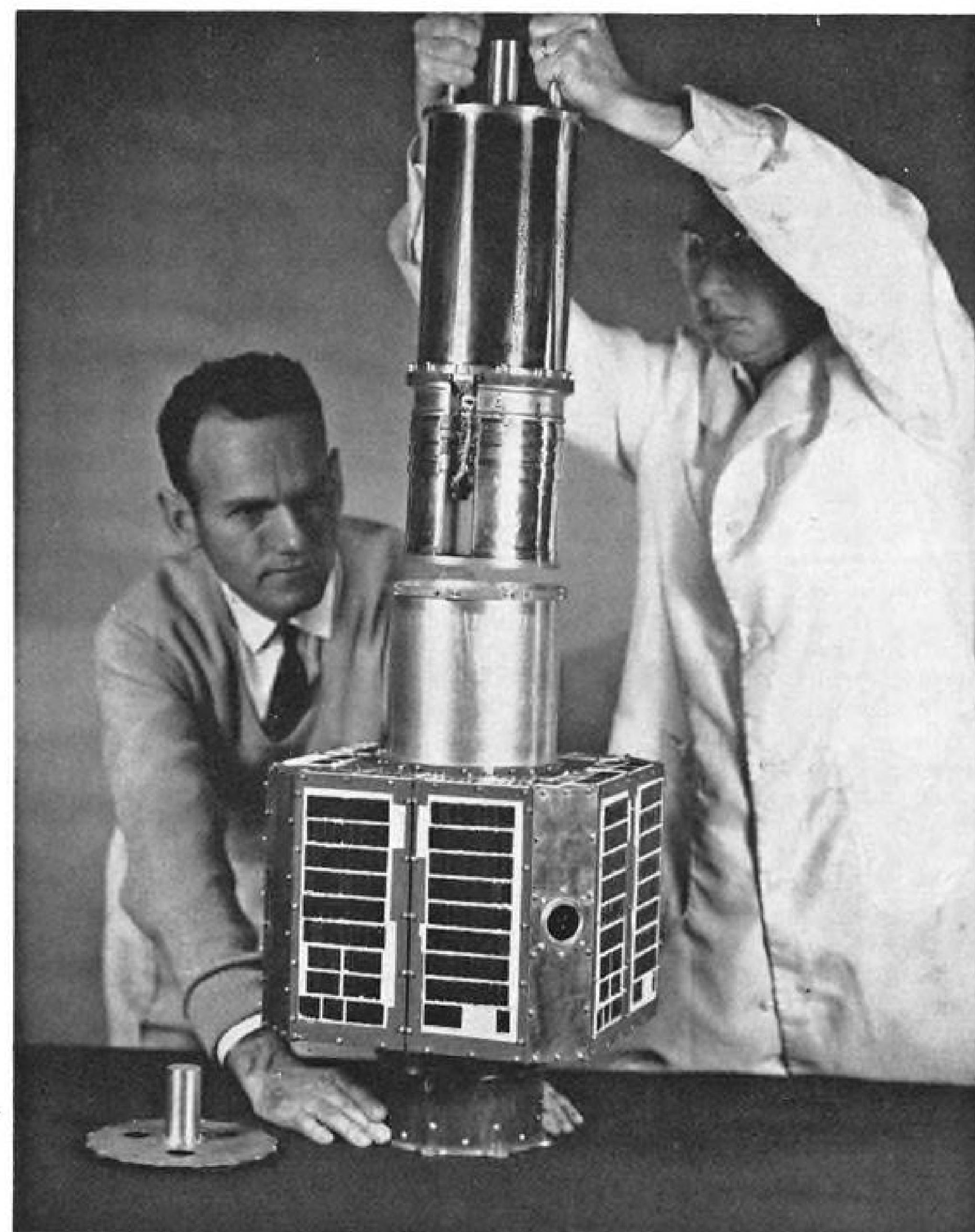
COSMIC RAY DETECTOR package containing five radiation counters is positioned into cylindrical housing of Juno II radiation belt satellite. Telemetry transmitter components are at bottom of package. Cylinder is surrounded by 1,184 solar cells.
