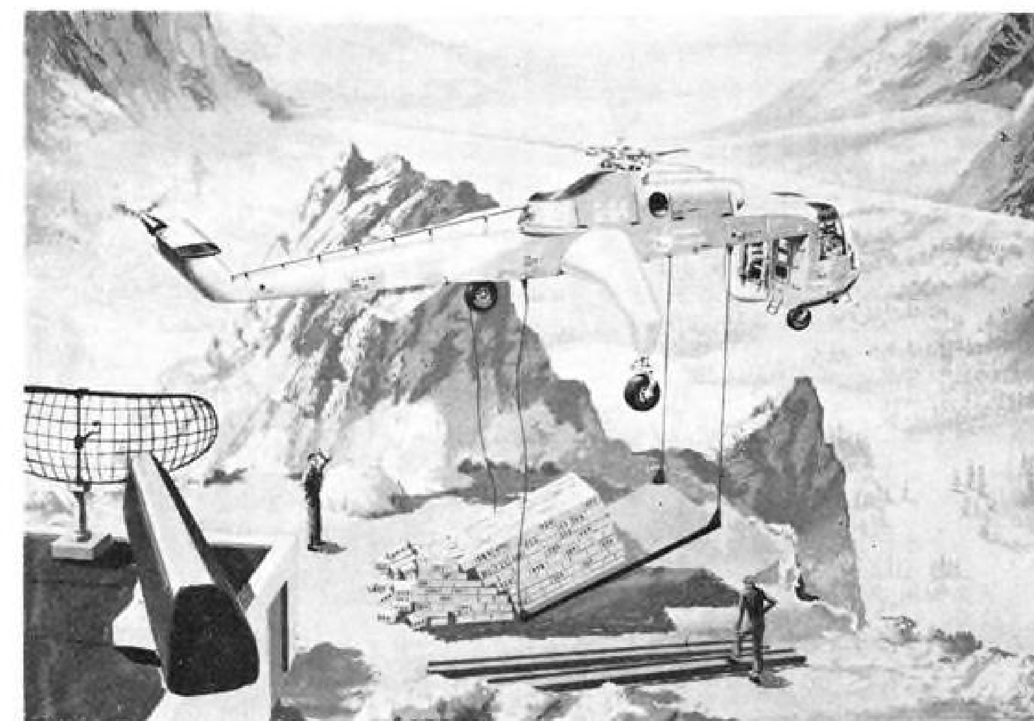
SIKORSKY ARTIST'S CONCEPTION shows a twin-turbine S-64 using a dump truck technique to supply an isolated construction site. The S-64 will carry an eight-ton payload.
