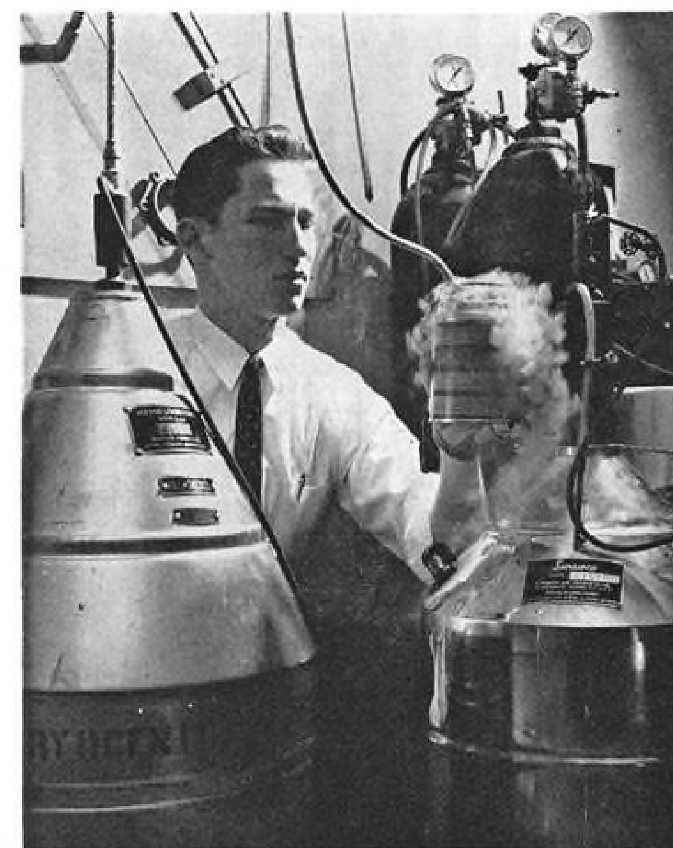
VAPORIZING NITROGEN in dewar flask at the Martin Co. (left) produces 77K temperatures for tests of vacuum-deposited specimens. Circular holder and necessary masks for depositing film flip flop at Space Technology Laboratories, Inc. (right) are shown half true size.
