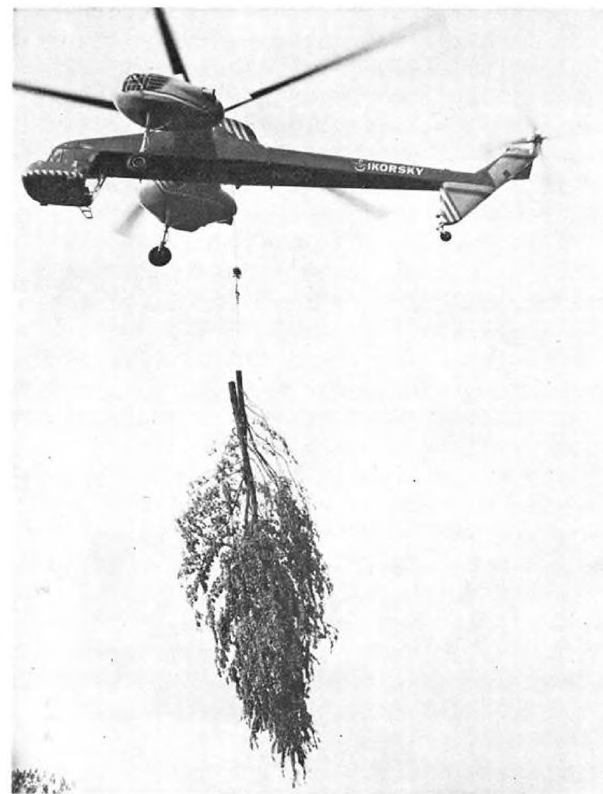
S-60 CAN LOWER its cargo hook from a hovering position, winch up a tree with its cargo hoist and fly away, or it can drag trees along the ground in a towing operation.
