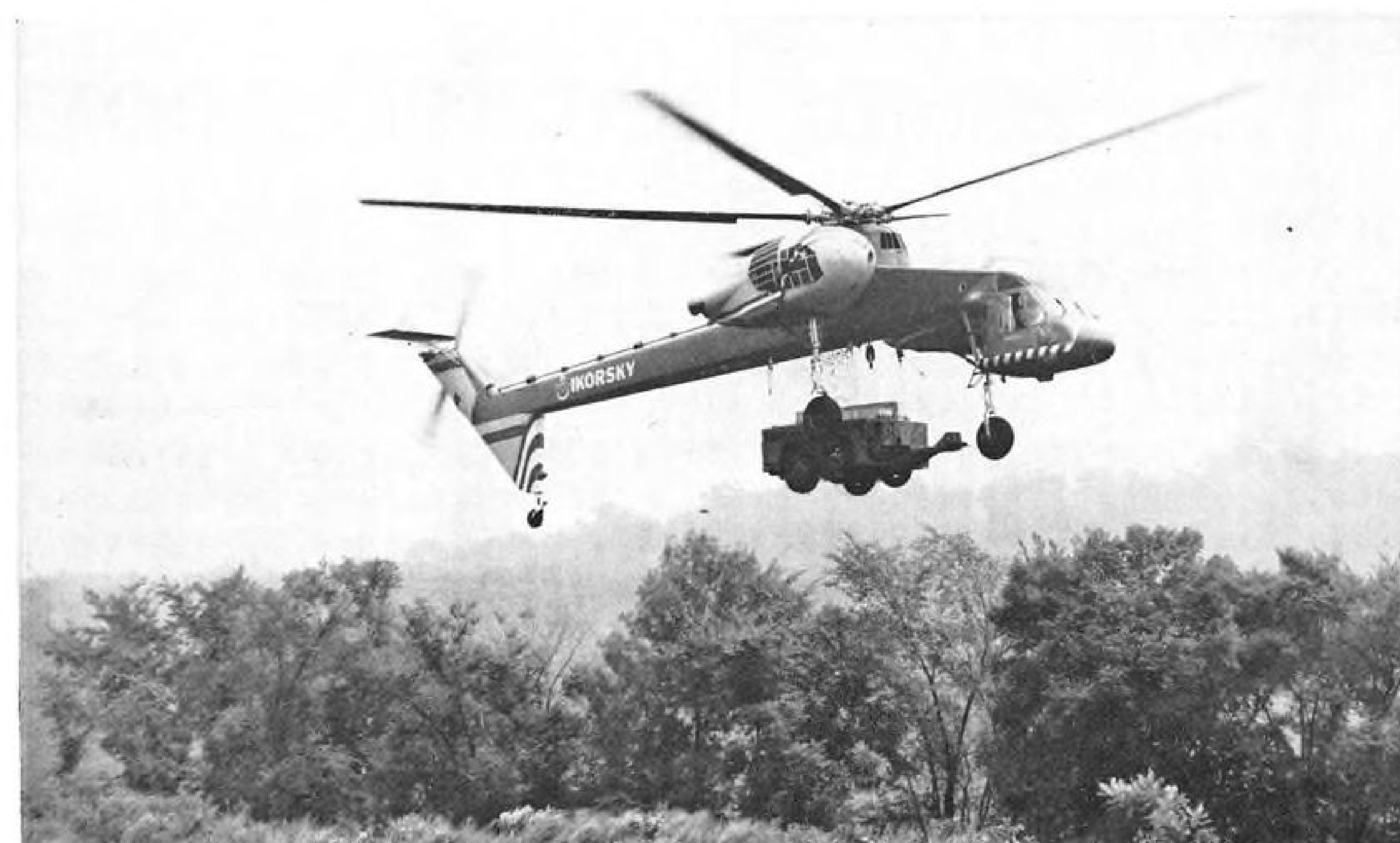
SIKORSKY S-60 , powered by two reciprocating engines, is the forerunner of a family of turbine-powered cranes which will be designed to carry payloads as great as 50 tons. Sikorsky's first turbine crane will be the S-64, due to fly this year.
