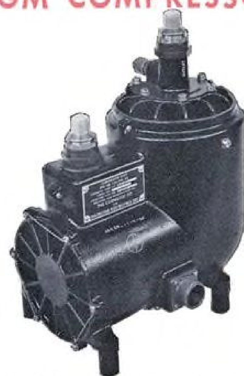
MODEL 3650200 DIAPHRAGM COMPRESSOR — Provides 2 CFM of standard air at sea level (3456 cu. in.); 0-25 psig. output pressure. Weighs 10 lbs. with motor and measures 9 3/4" x 7" x 11 3/4" including motor. Designed for 1000 hrs. continuous duty operation in temperatures of -65° to +160° F.
