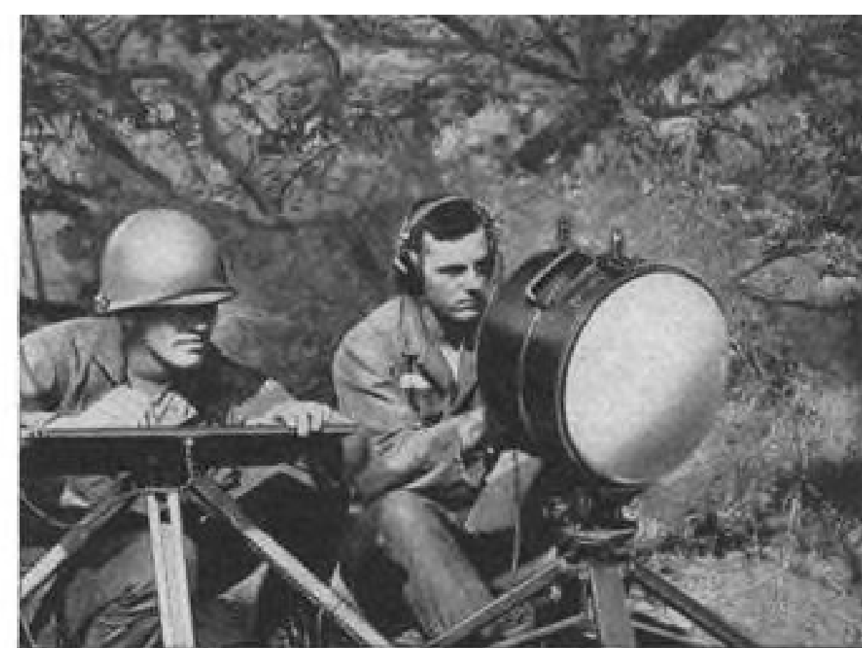
PORTABLE FIELD RADAR provides Army with combat surveillance of enemy movements. Head-phone signal reveals presence of moving vehicles or personnel in battle area.
