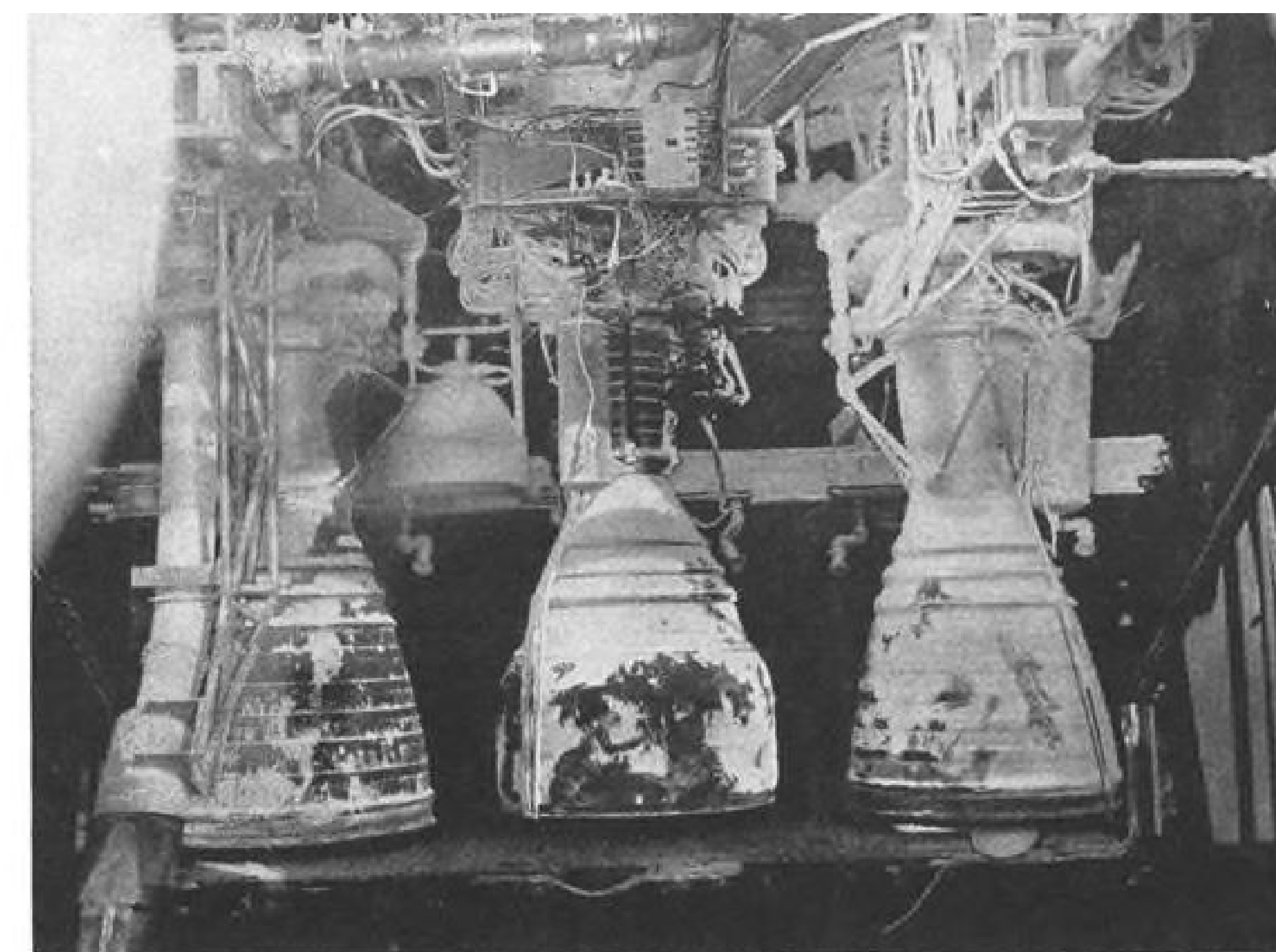
ENVIRONMENTAL CHAMBER has been removed from around the MA-3 cluster (above) after cluster was exposed to 160F in 95% humidity for five days followed by cold soak at minus 65F for 24 hr. Cluster is fired (below) as soon as the environmental chamber is removed. Ice is shown being shaken from the cluster two seconds after ignition.
