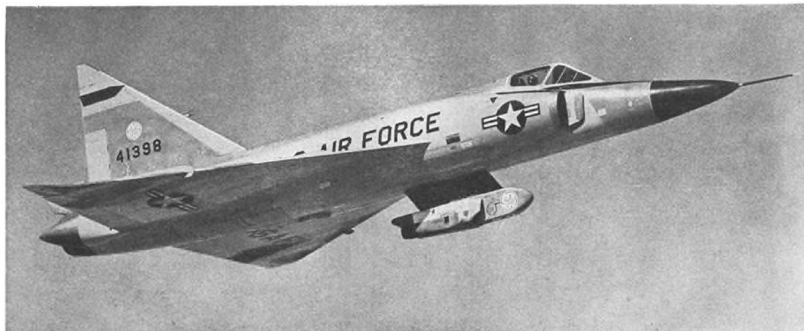
J85-7 powers GAM-72 aboard F-102A. Test flights have included afterburner operation to 50,000 ft. and speeds to Mach 1.23.
