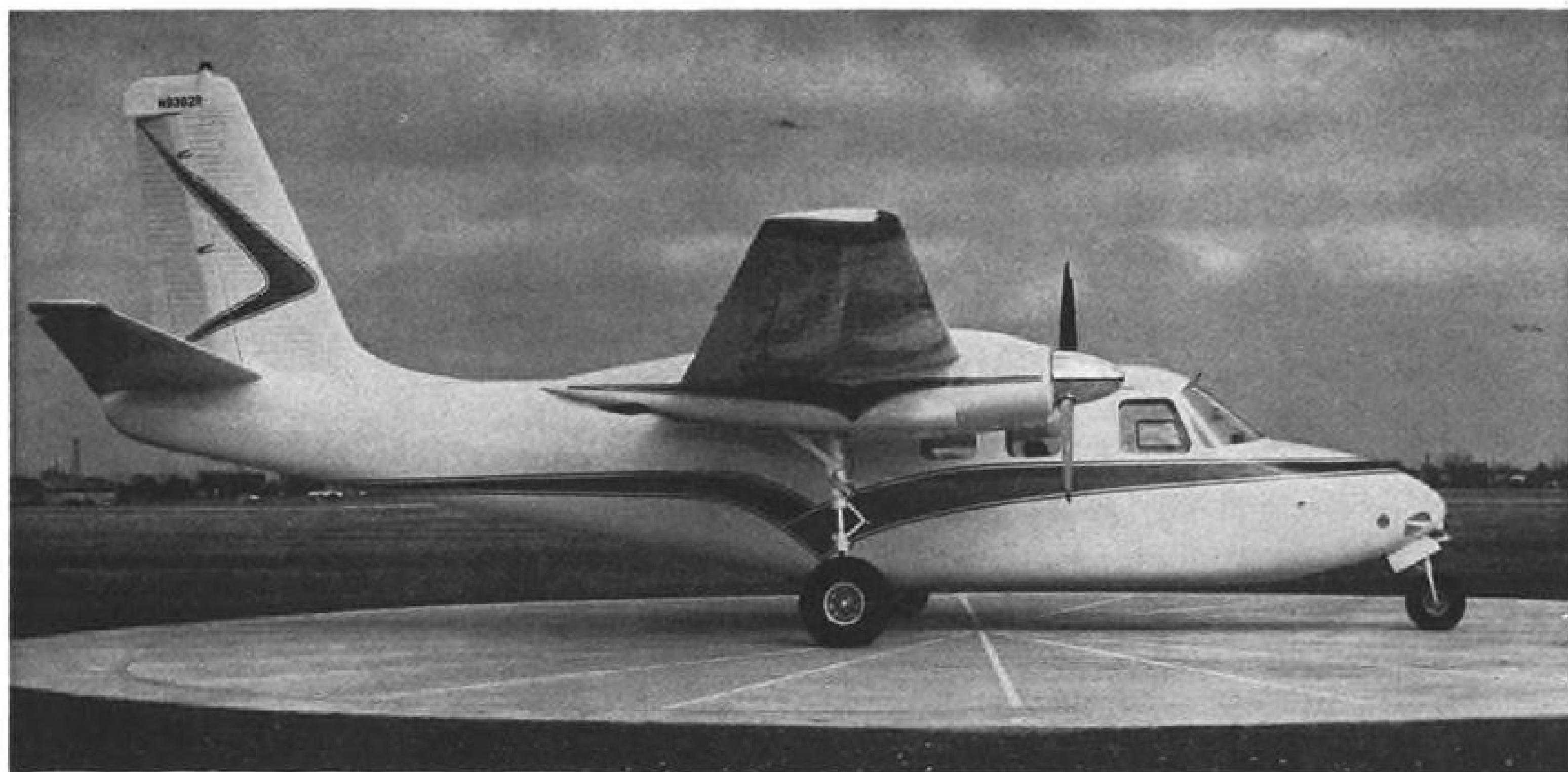
PROFILE of new engine cowlings shows its resemblance to NASA 65000-series airfoils. New design features in the first Continental-powered Commander, Model 500A, are also present in other models.
