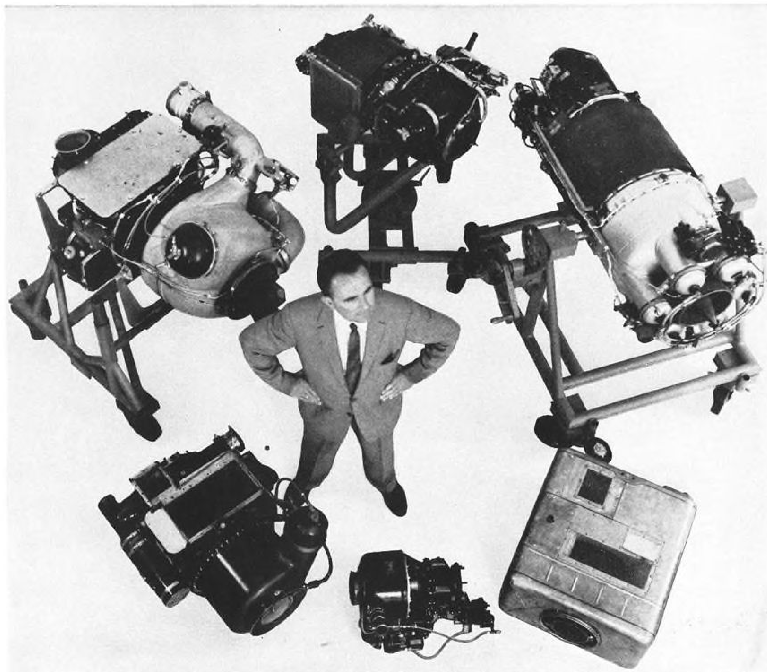
Helmut Schelp, chief engineer, AiResearch Manufacturing Division of Arizona, Phoenix, surrounded by typical gas turbines now in production ranging in size from 30 to 850 hp. Clockwise from the top: GTC 85-20, GTCP 105, GTP 70-6, GTP 30-1, GTP 70-10, GTU 85-2.
