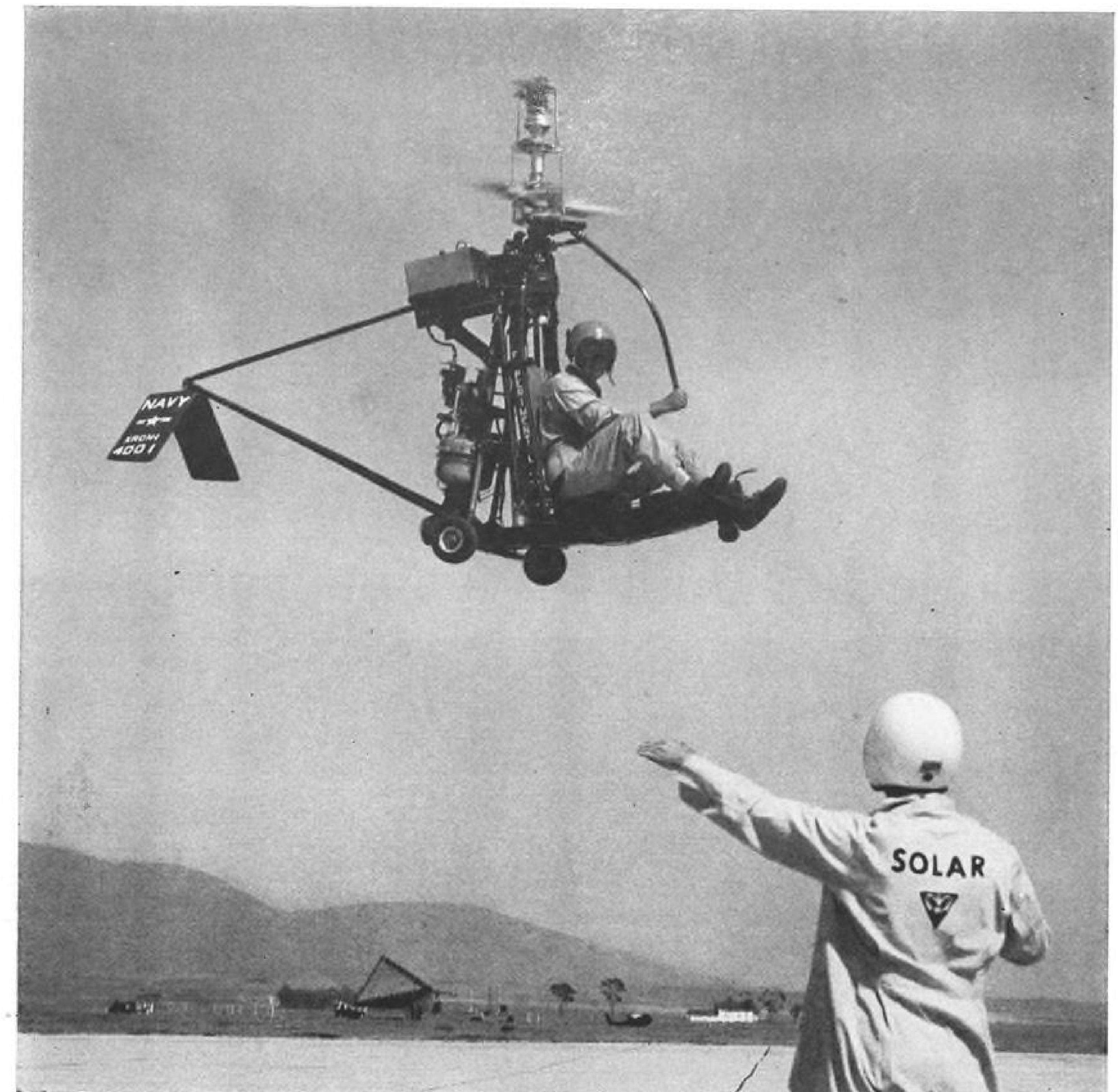
Solar Titan turbine being flight tested in Gyrodyne Rotocycle helicopter.
