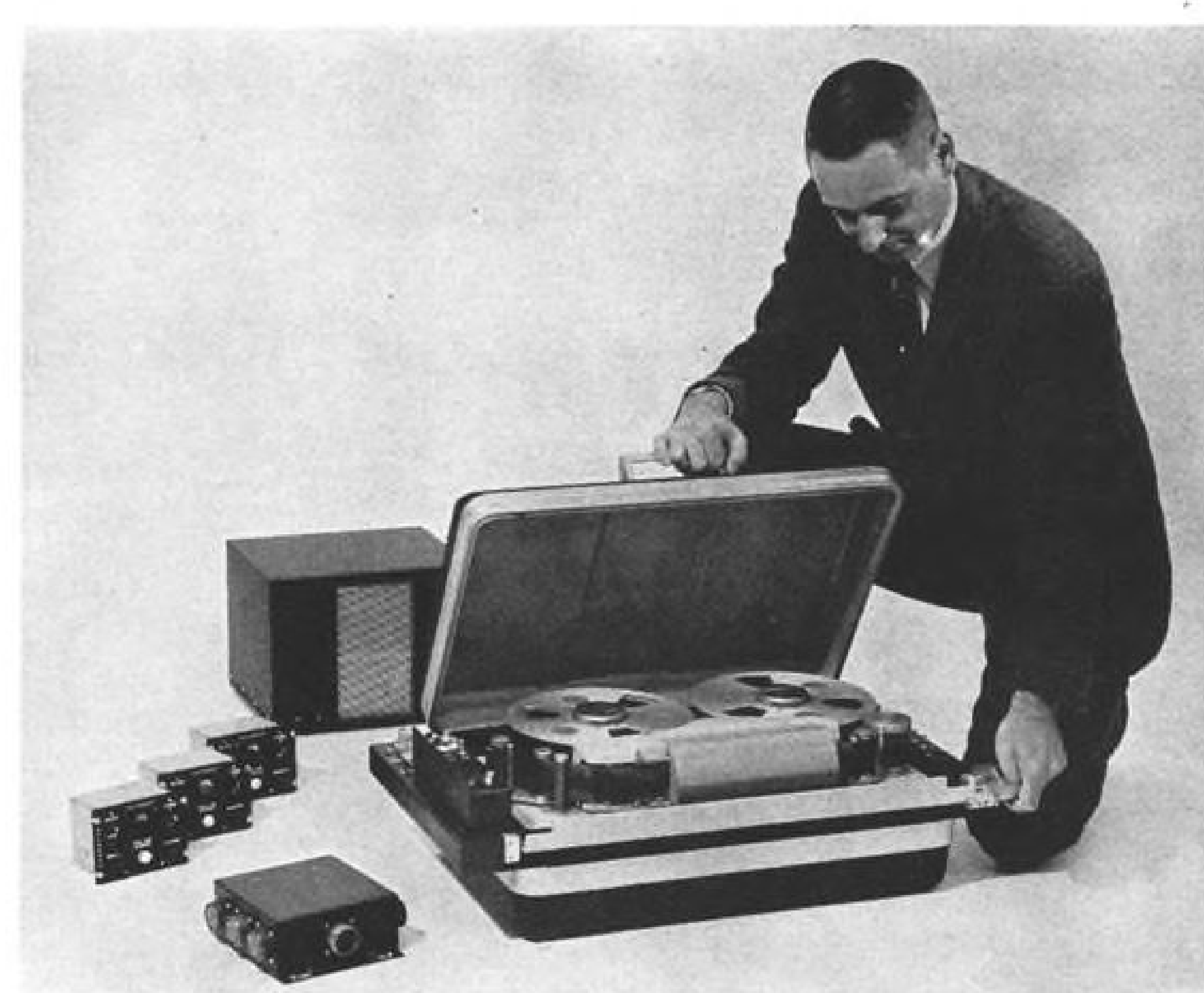
AMPEX AIRBORNE WIDE-BAND TAPE RECORDER , with frequency range of 10 cps. to 4 mc., making it suitable for electromagnetic reconnaissance, weighs only 150 lb. Behind tape transport is power supply. Small units at left are remote control panels.
