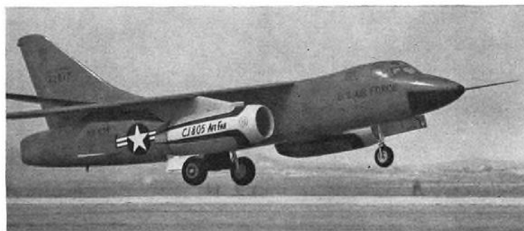
RB-66 modified to accommodate General Electric CJ-805-23C, has been flying since February, 1960. Aircraft recently completed cross-country tour.
