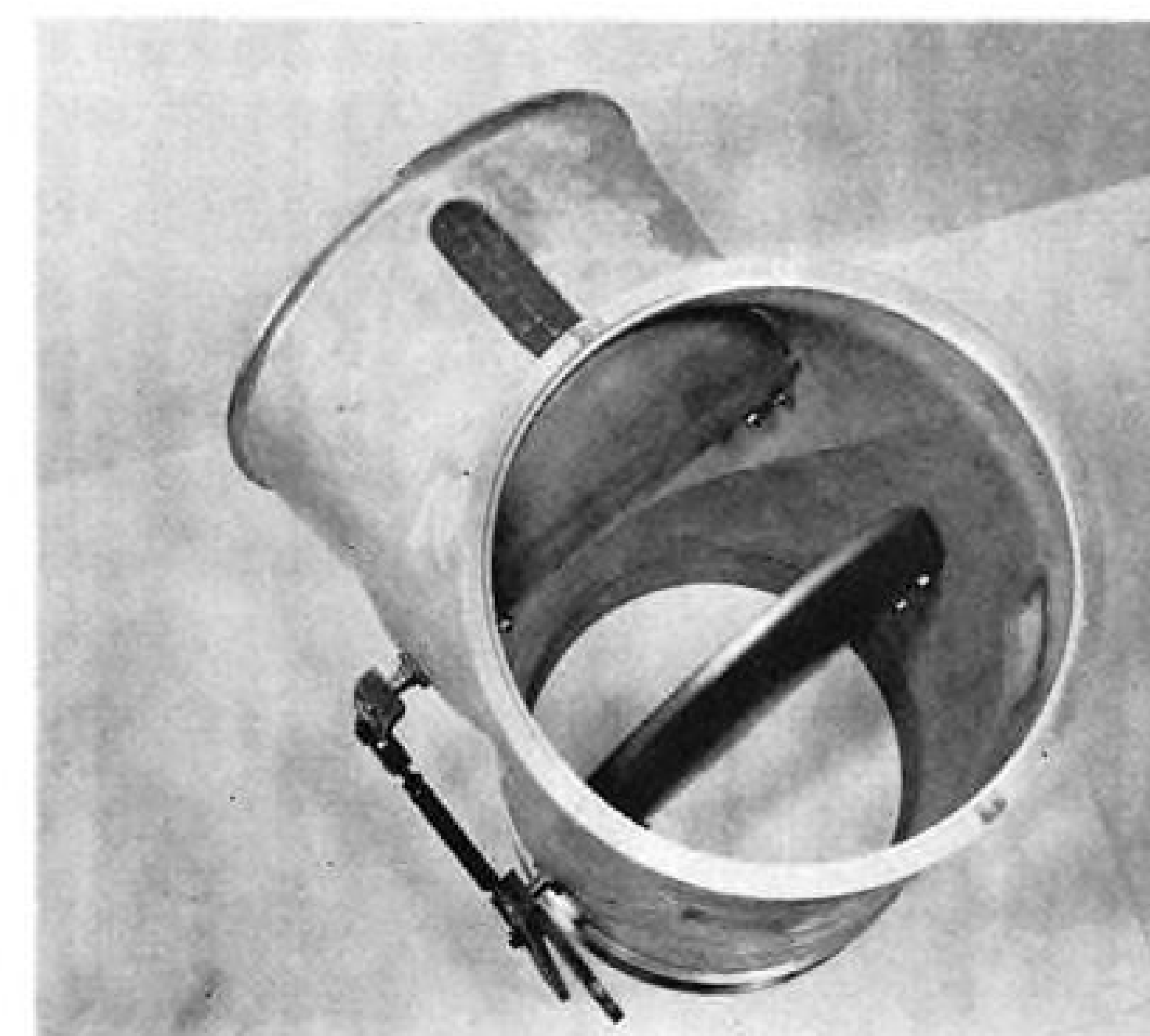
DIVERTER valve (above) is used to direct the hot air from the gas generator either to the lift-fan or into a nozzle to provide horizontal thrust. The valve is then positioned to turn the flow 90 deg. into the fan scroll.
