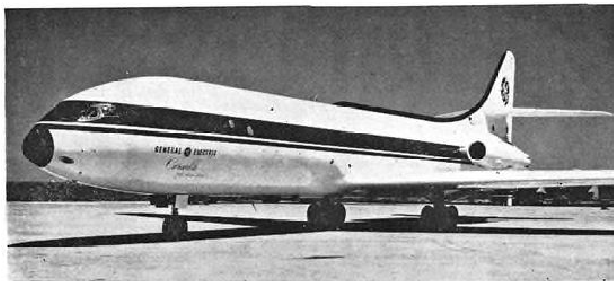
GENERAL ELECTRIC will fit its Caravelle III with CJ805-23 aft-fan engines later this year, using the airplane as a demonstrator and for engine testing.
