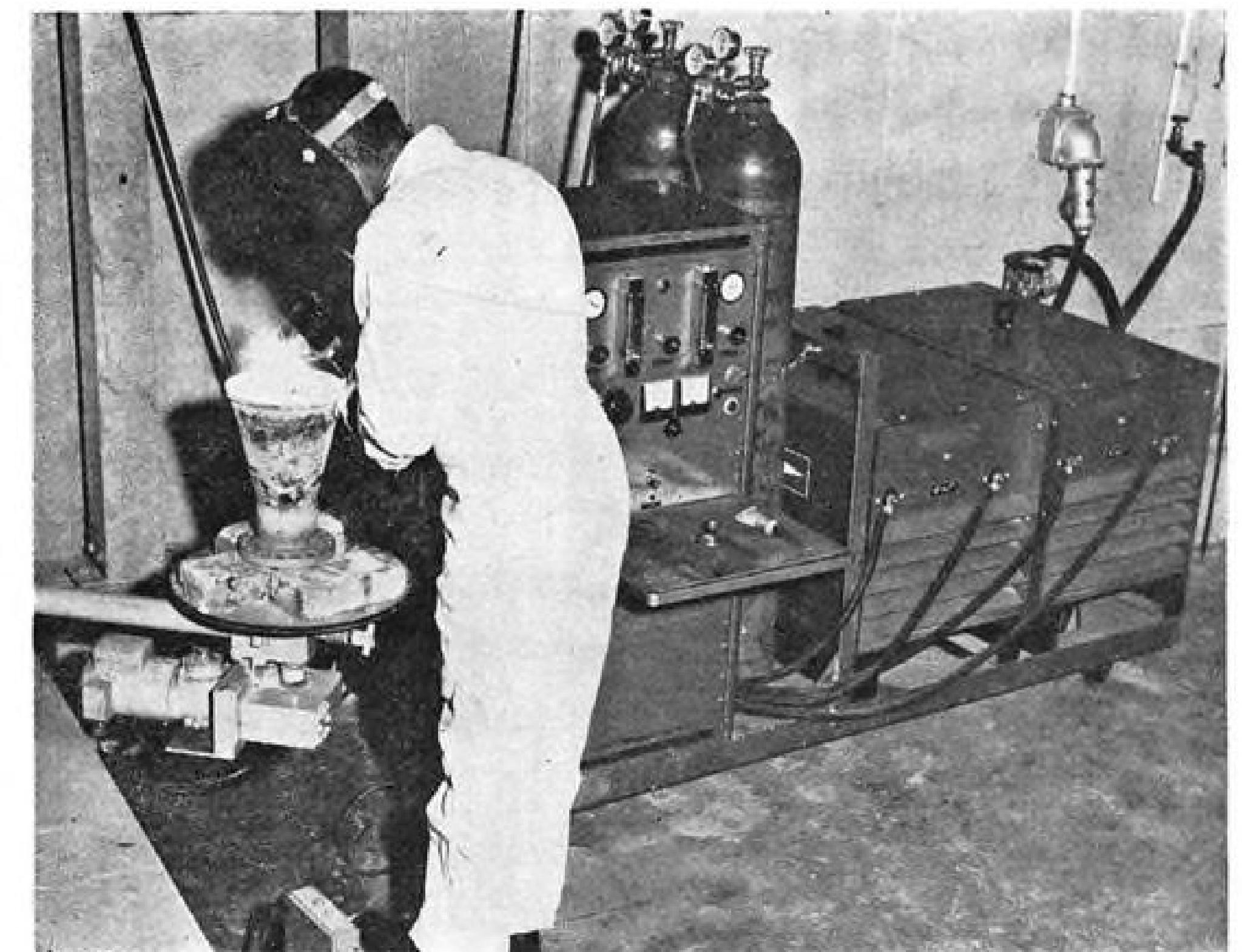
PLASMA coating is applied to an experimental rocket motor nozzle to be tested by Solid Propellant Operations at McGregor, Tex. Coating permits high degree of erosion protection and use of same nozzle for numerous tests at great cost savings.
