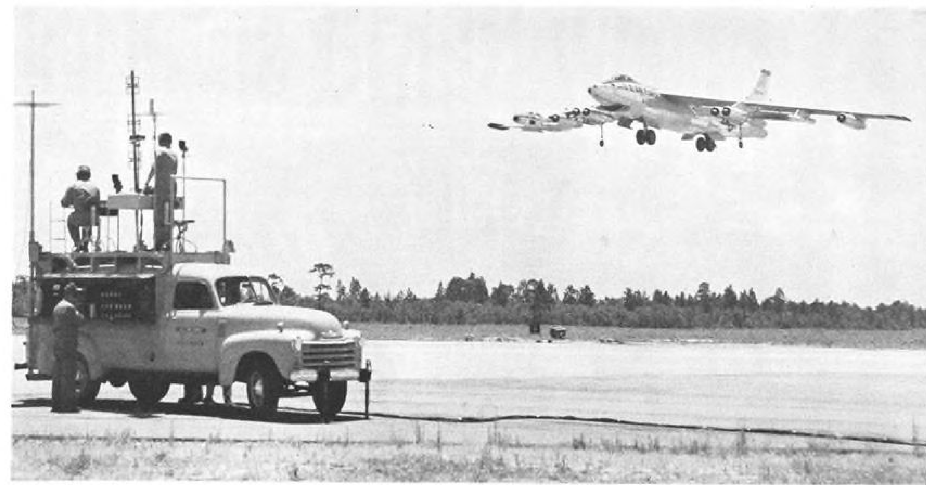
BOEING QB-47 target drone is landed at Duke Field by ground controllers atop MRW-5A following Bomarc intercept mission. Controllers atop truck split QB-47 throttle, elevator and rudder functions; airman at side of truck monitors complete drone panel.
