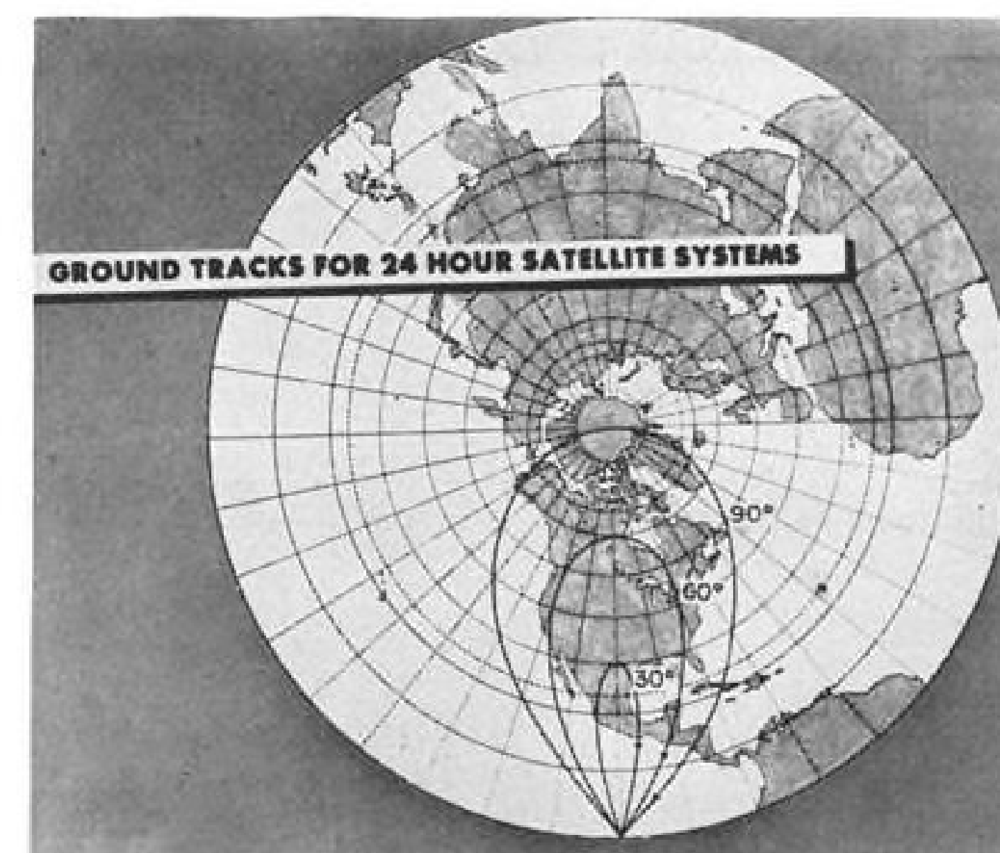
INCLINED orbit synchronous satellite circles the earth; earth-based observer sees ground track as a figure eight crossing equator every six hours. Two synchronous satellites in equatorial orbits could handle bulk of U. S. overseas commercial traffic.
