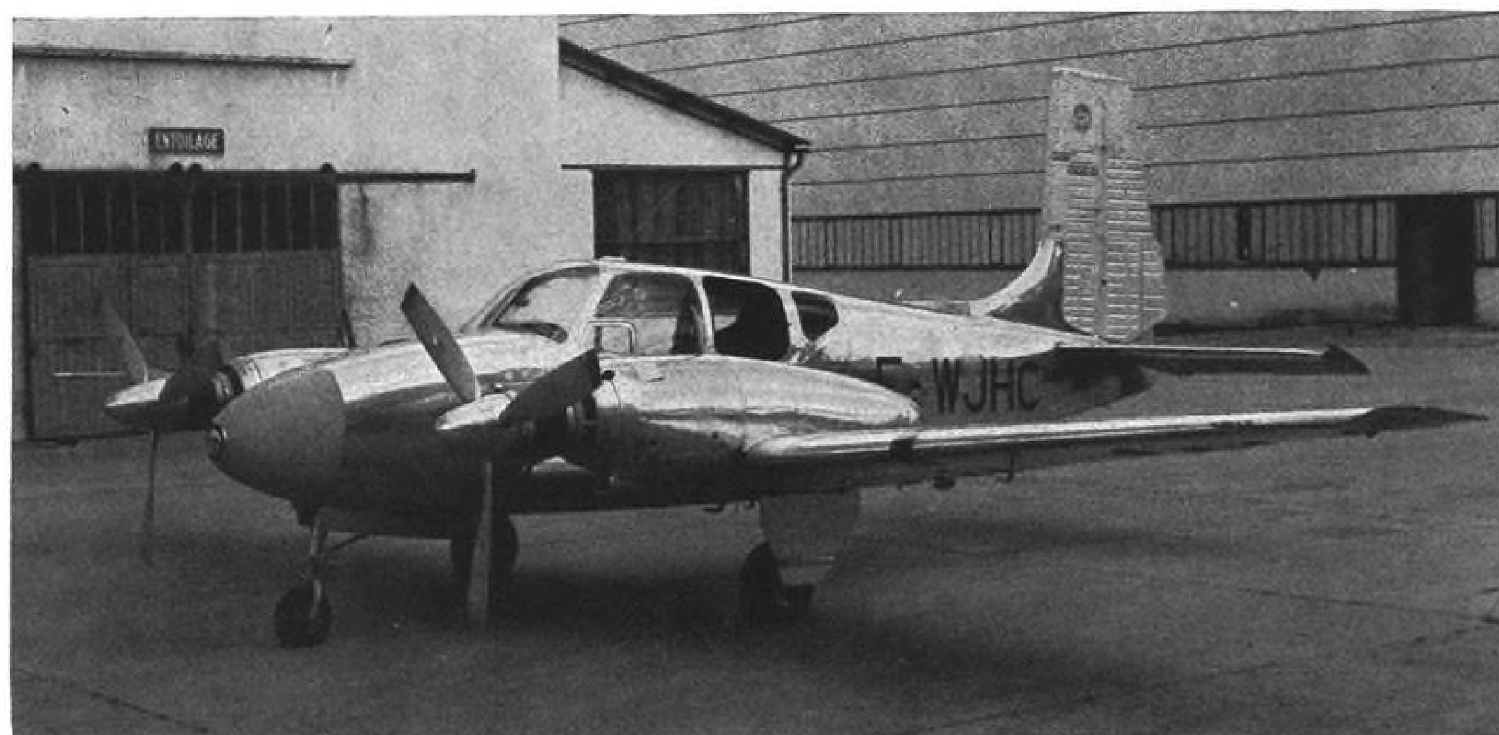
SIMILAR to the 1960 B95 version of the piston Beech Travel Air, SFERMA's 01 turbine Travel Air has a taller (about one foot), squared-off fin, curved dorsal fillet and a wider span tailplane. Plane is equipped with two Turbomeca Astazou 470 chp. turboprops.
