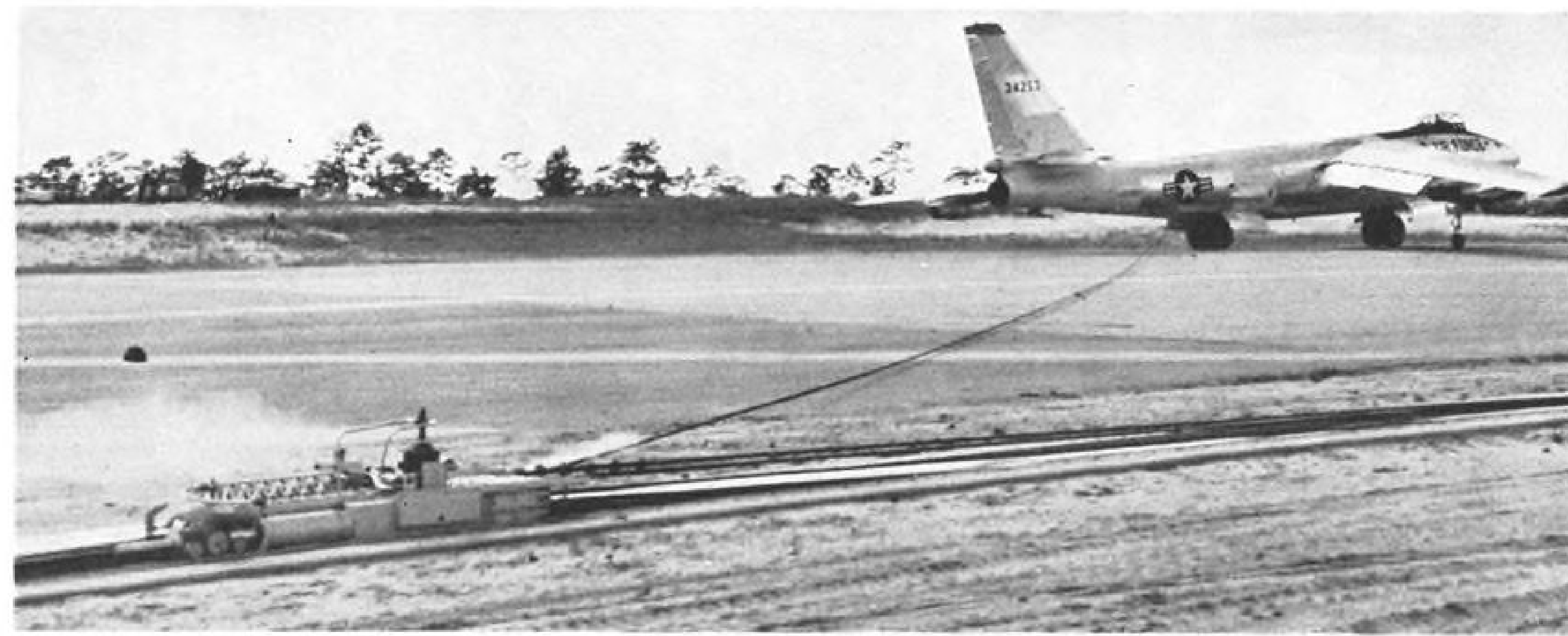
SPECIAL arresting gear lessens hazards of remote control of six-jet QB-47. All-American Engineering Co. built and installed the system, comprising a one-inch cable attached to connecting pulley and gearbox mechanism.
