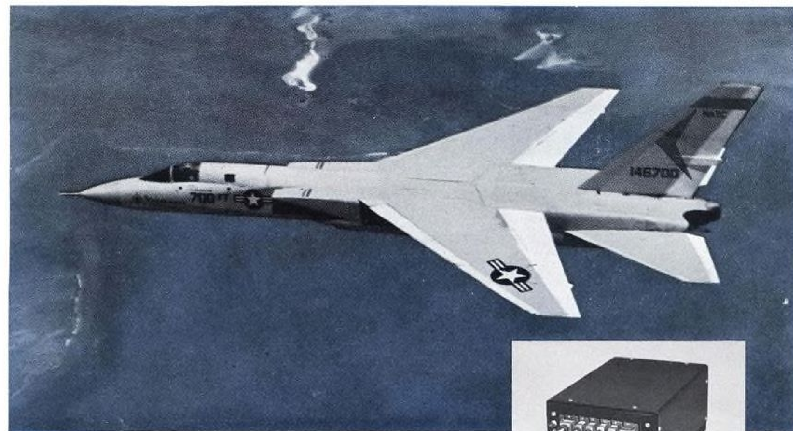
North American's highly versatile A3J Vigilante is an all-weather aircraft with atomic fire-power capability. Chatham designed and supplies the 28VS200BL silicon power conversion equipment which furnishes the dc power. There are two units on every A3J, each delivering 200 amps.
