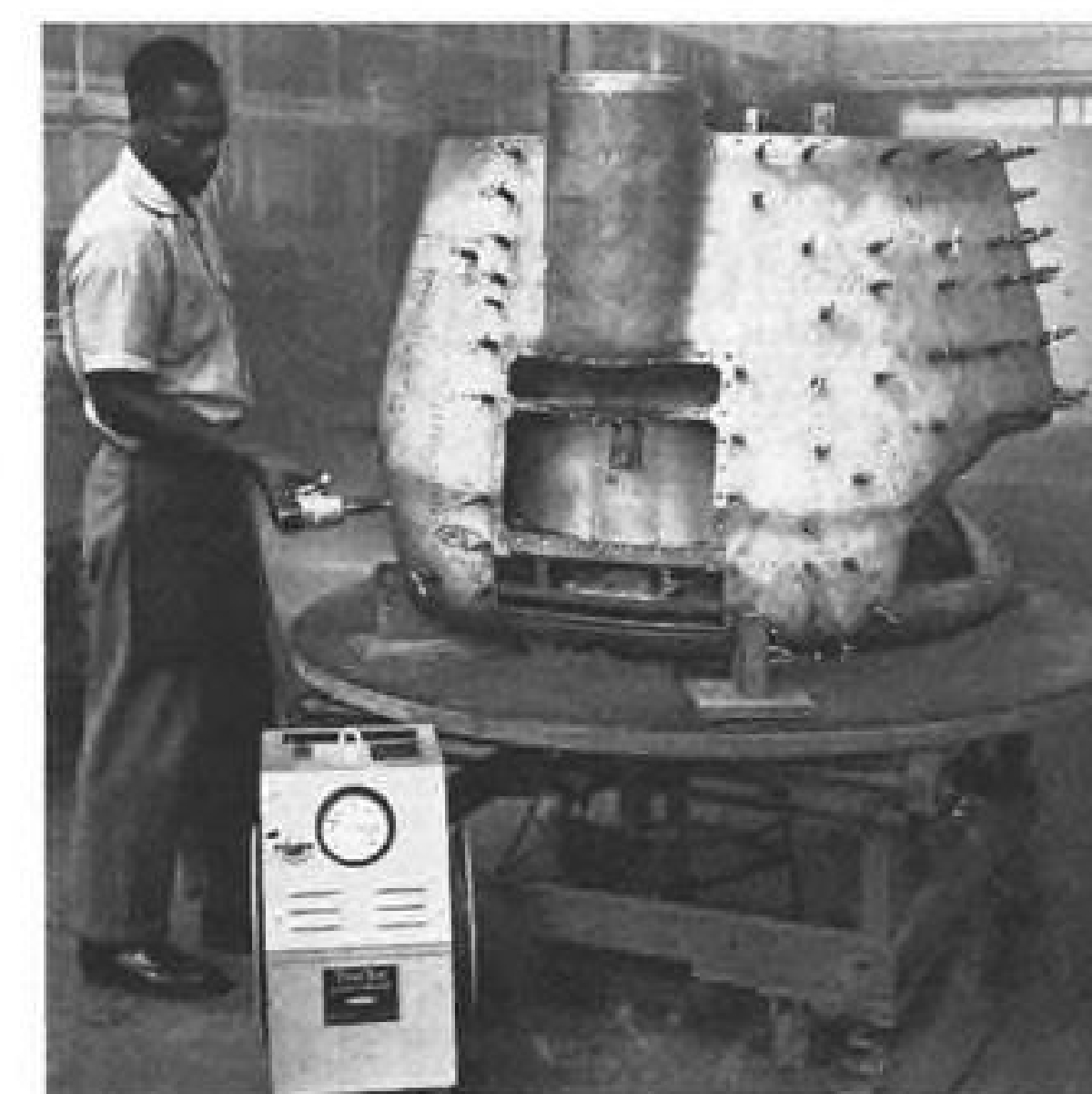
Above photo shows portable electric-hydraulic Power Unit (3000 psi max....110 v. source) actuating hand held Gun to drive 1200 Blind Bolts in each Ejector and Thrust Brake. Air-Hydraulic Power Units are safely used in flight ramp areas for repairs on fueled aircraft. Hand installation tools are also available.
