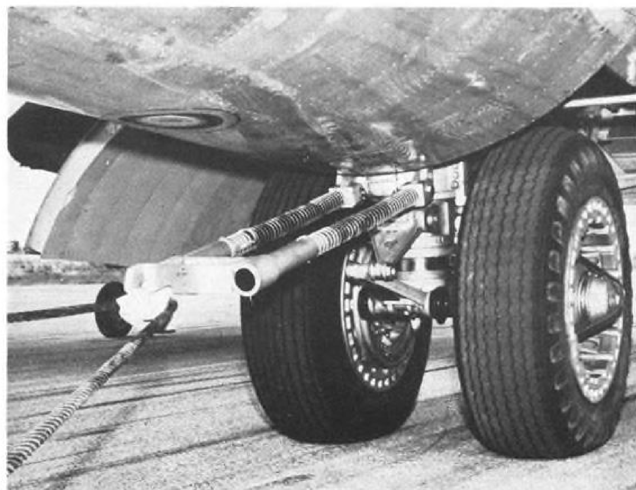
CABLE engagement hook is fitted between the rear wheels of the QB-47. Hydraulically operated brake pucks press against stainless steel rails to halt the aircraft.
