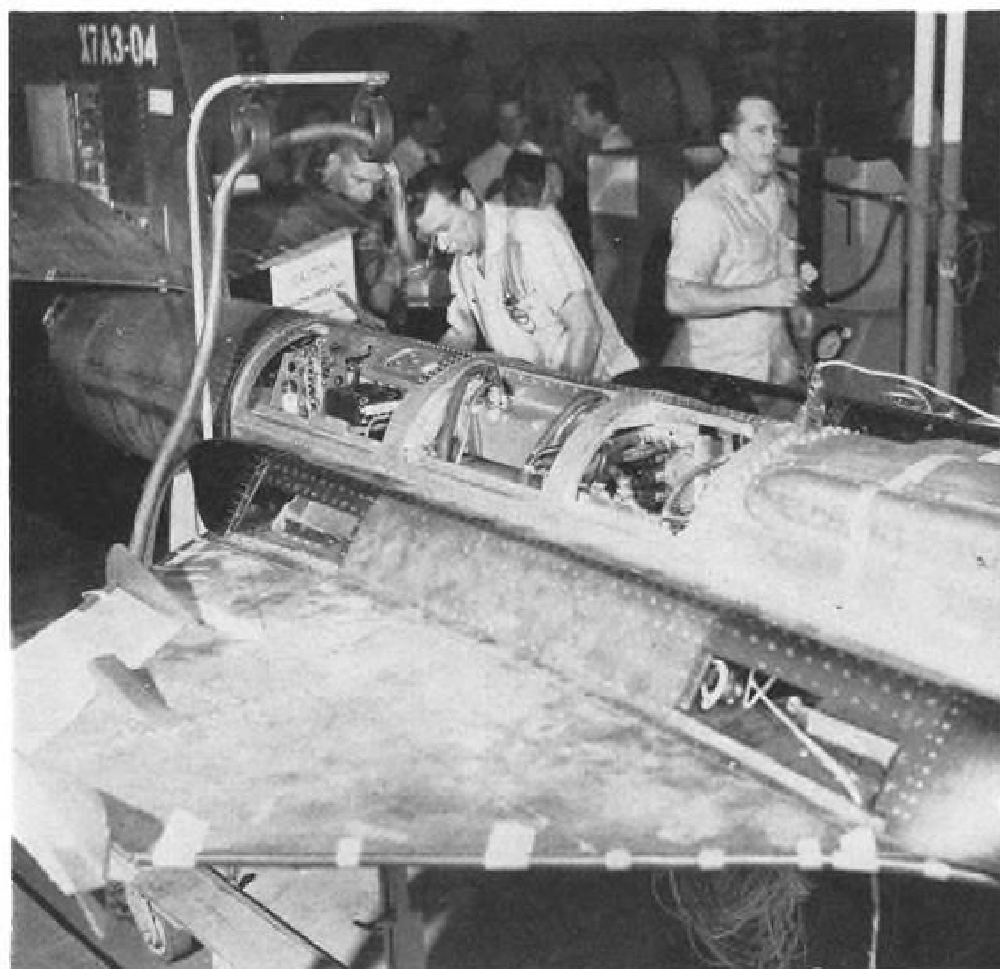
LOCKHEED X-7A-3 undergoes systems checkout at company's Van Nuys, Calif., facility. Note exceptionally rugged steel structure which permitted average of five flights per vehicle and up to 12 flights for a single craft.
