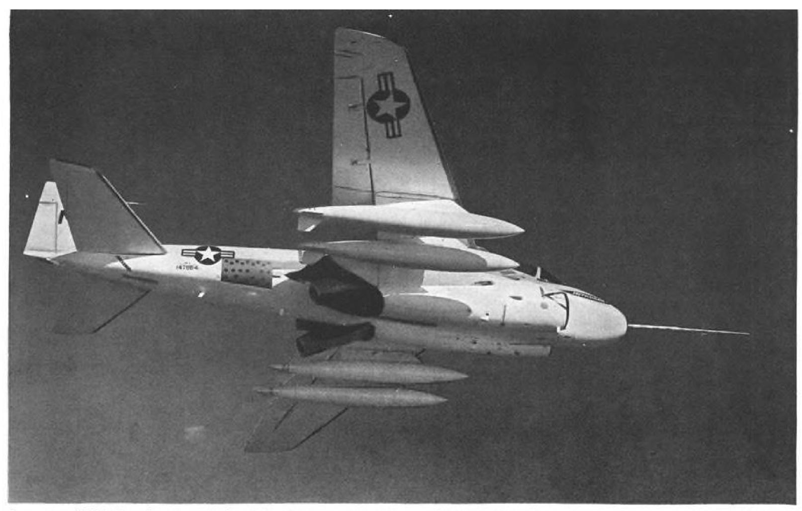
Grumman A2F-1 Intruder, a carrier-based low-level attack bomber capable of holding Mach .9 at sea level, is equipped with brazed honeycomb stainless steel speed brakes mounted behind jet exhausts. A2F-1 is powered by two Pratt & Whitney J52-P6 turbojets.
