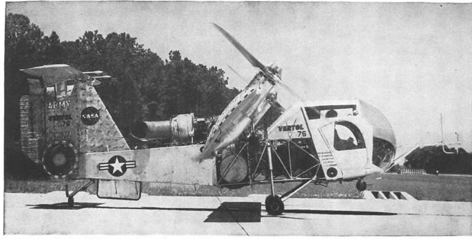
VERTOL 76 tilt-wing VTOL research aircraft, powered by single Lycoming T53 free-turbine engine, was evaluated by NASA pilots during one-year program of flight tests. Changes made in configuration by NASA included extra dorsal and ventral fin area, and closed rear fuselage. Wing position is shown set for short takeoff and landing performance. Wool tufts taped to vertical tail and wing surfaces provide visual qualitative indication of airflow patterns.
