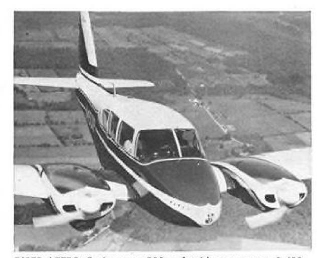
PIPER AZTEC. Cruises over 200 mph with range up to 1,400 miles. Powered by two Lycoming 250 hp engines, has highest single-engine ceiling of any airplane in its class carrying a similar payload. Carries five passengers in luxury of super-quiet cabin. Selected by U.S. Navy for utility transportation duty. \$49,500.
