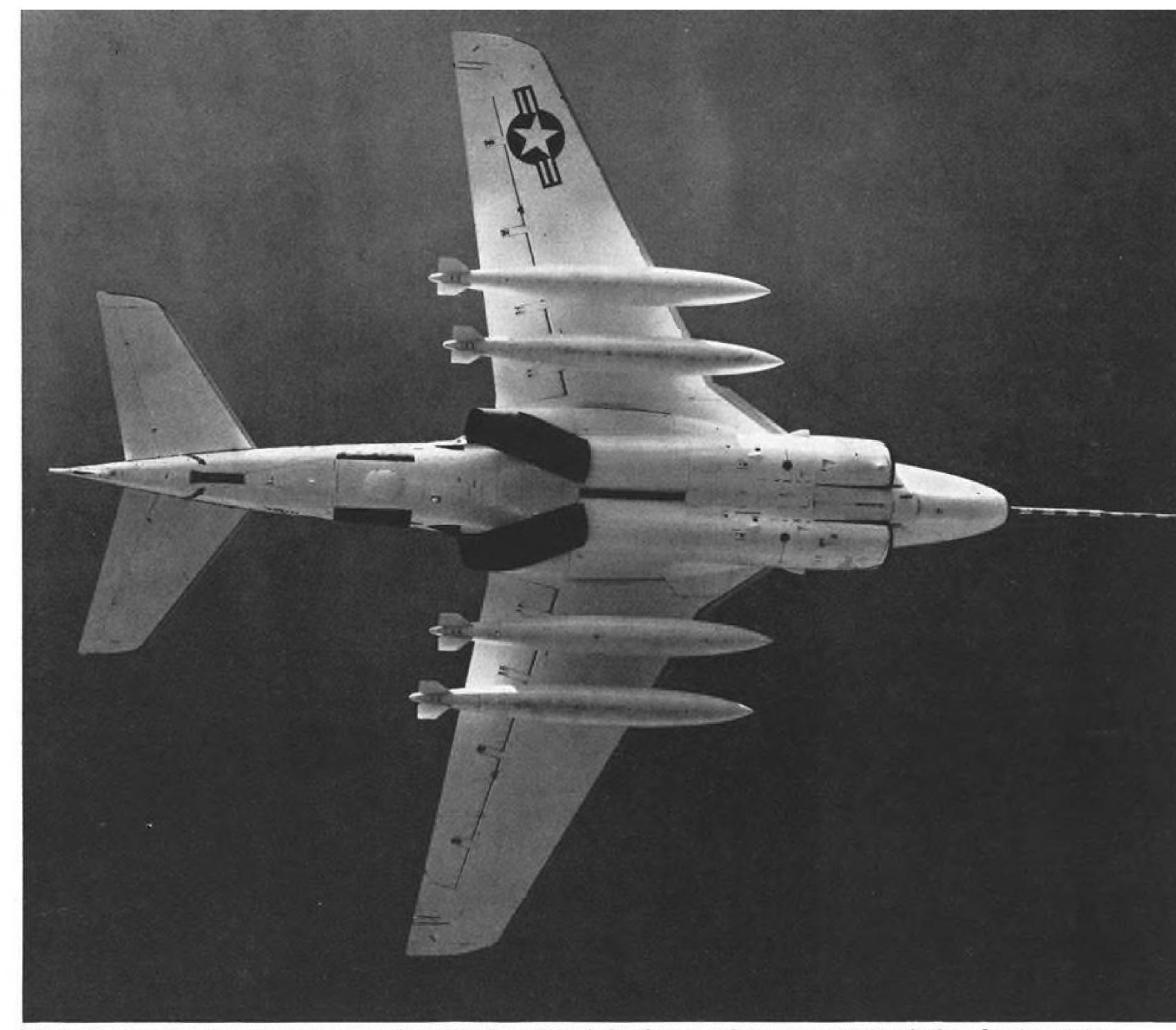
Side-by-side two-place Intruder above carries four 300-gal. auxiliary fuel tanks mounted on weapons stations for long duration missions. A2F-1 carried three Mk. 84, 2,000 lb. GP bombs mounted outboard on each wing and under belly, and two Martin ASM-7 Bullpups.
