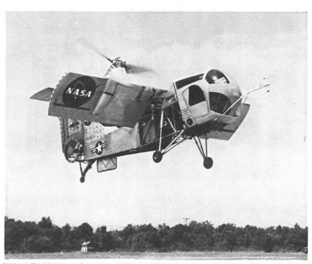
SHORT TAKEOFF performance of Vertol 76 enables the testbed aircraft to get off the ground with a run of about two fuselage lengths. Variable wing position allows anything from vertical liftoff to normal takeoff run along a paved runway surface.
