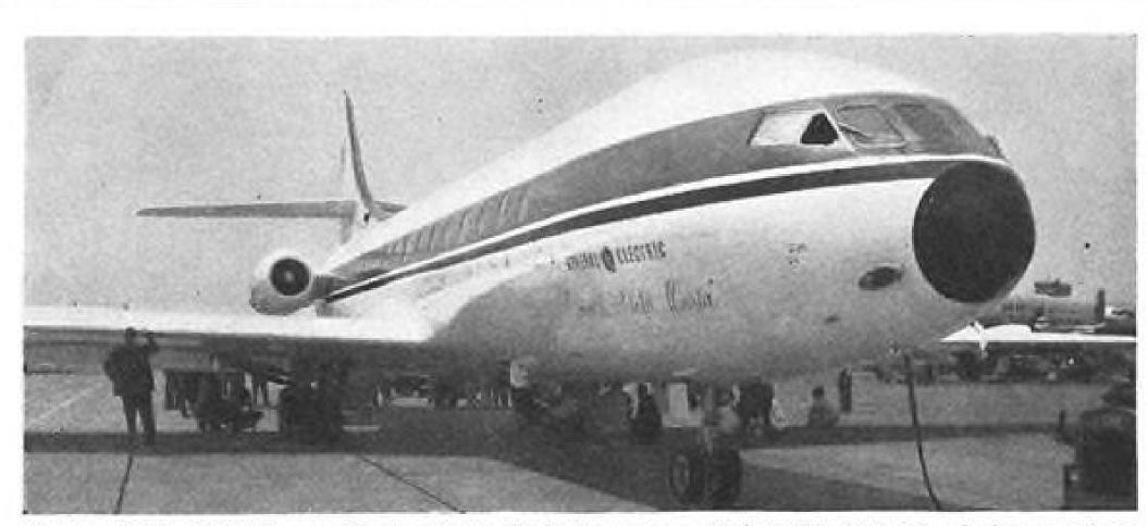
General Electric's Caravelle is currently being converted to CJ-805-23 aft-fan engines at Edwards AFB, California. Production aircraft have been designated Caravelle VII.
