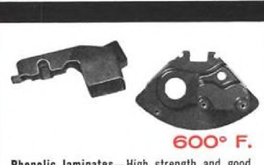
Phenolic laminates — High strength and good electrical properties at high temperatures characterize a fast increasing variety of Swedlow phenolic laminates. High dimensional stability and minimum thermal expansion make these laminates useful for nose cones, fins, stabilizers, adapter rings. Shown: molded switch cover and switch case.
