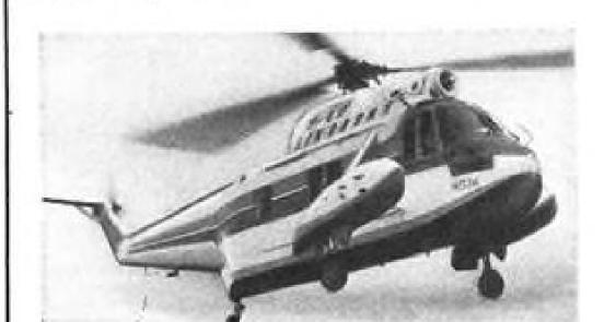
CT58 powers the Sikorsky S-62, first American turbocopter certificated for commercial operation.
