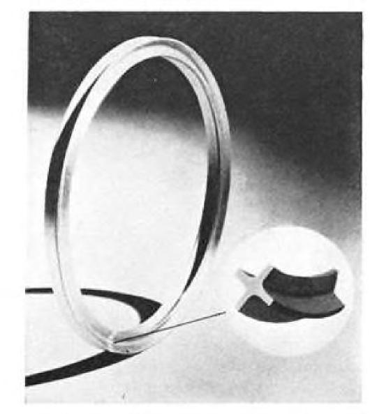
psi. The "X" configuration seal, reported to provide elastic deflections and high sealing forces, has provided zero leakage from room temperature to 1,000F with dry nitrogen at 1,000 psi. in a static seal application.
