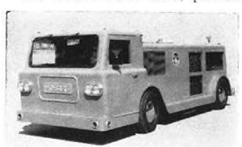
by a GMC Diesel engine, is rated at 125 kva, 0.8 psf. three phase, four wire, 400 cps. The enclosed control cab is 71 in. high. Noise levels are reduced by the use of a centrifugal blower and two mufflers.
