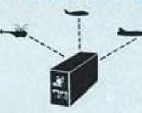
By a simple change of modules, these systems may be adapted to any aircraft from a hovering helicopter through a 230 knot observation plane to a mach 2 bomber or fighter plane. The same modular design permits ease of access for servicing and reduces quantity of parts to be provisioned.
