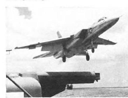
A3J catapults from the USS Saratoga, powered by two G-E J79 engines.
