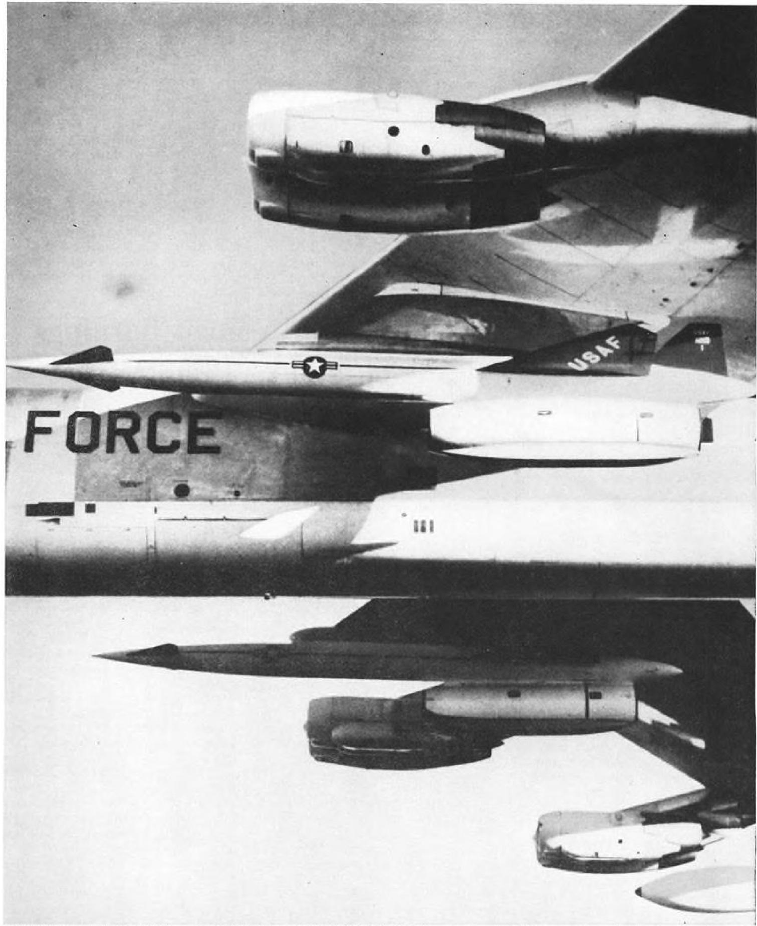
POWER TO FLY...POWER TO PROTECT... by Pratt & Whitney Aircraft. Today the Strategic Air Command's Boeing B-52 bomber has a new profile. Inboard from its J-57 turbojets, two more Pratt & Whitney Aircraft jet engines have been added...a pair of J-52s. These engines power the North American Hound Dog guided missile,
