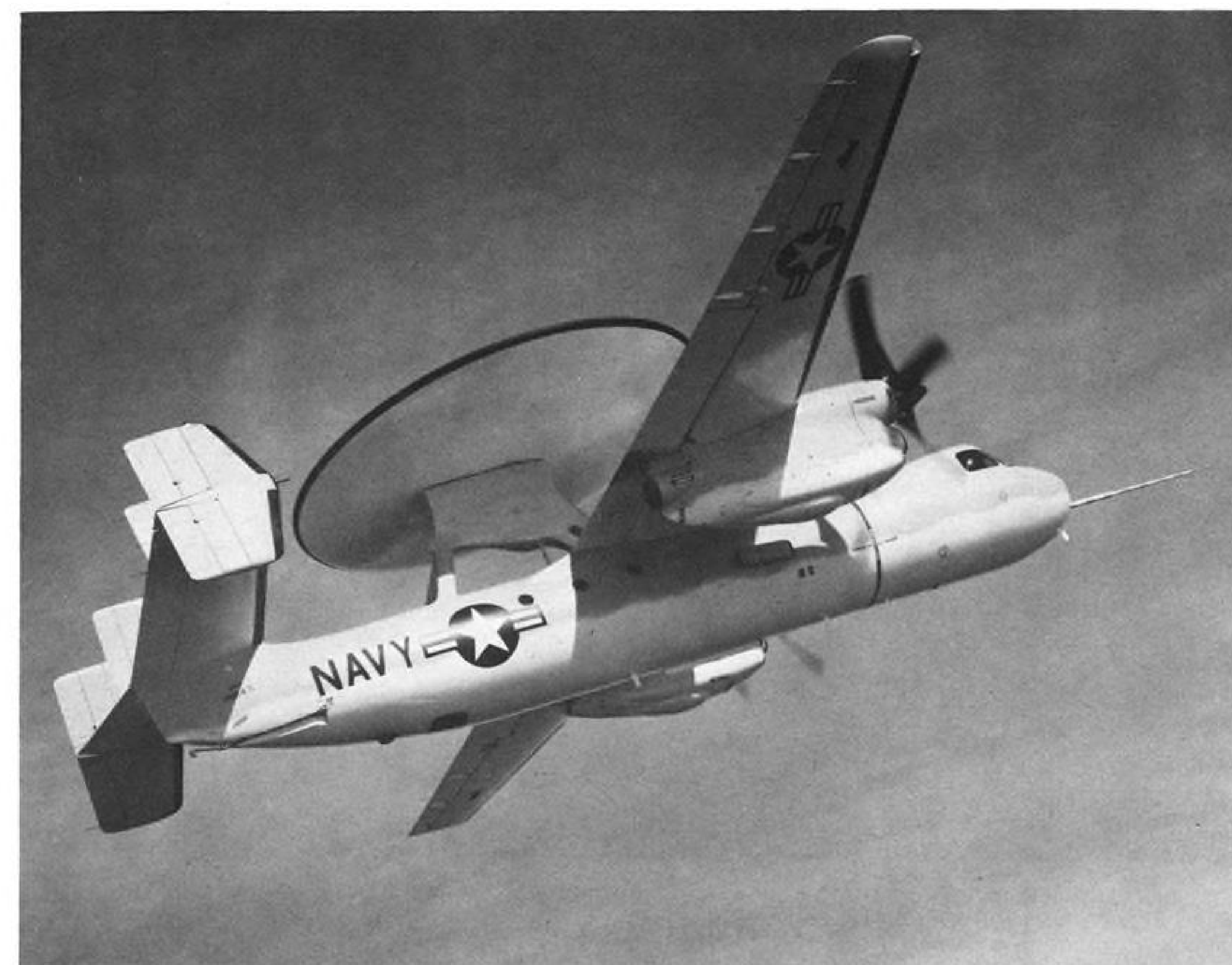
GRUMMAN W2F-1 Hawkeye early warning aircraft serves as a platform for 20-ft.-dia. rotodome which revolves at a 6-rpm. scanning speed. General Electric-designed radar housed in the rotodome provides height-finding and azimuth target information.
