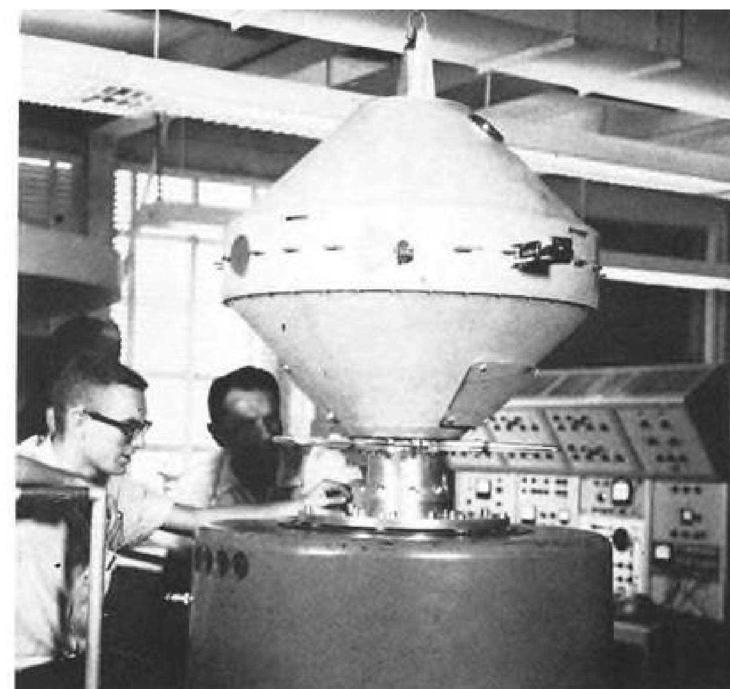
EXPLORER VIII satellite package is subjected to vibration test at left. Instrument column is assembled at right.
