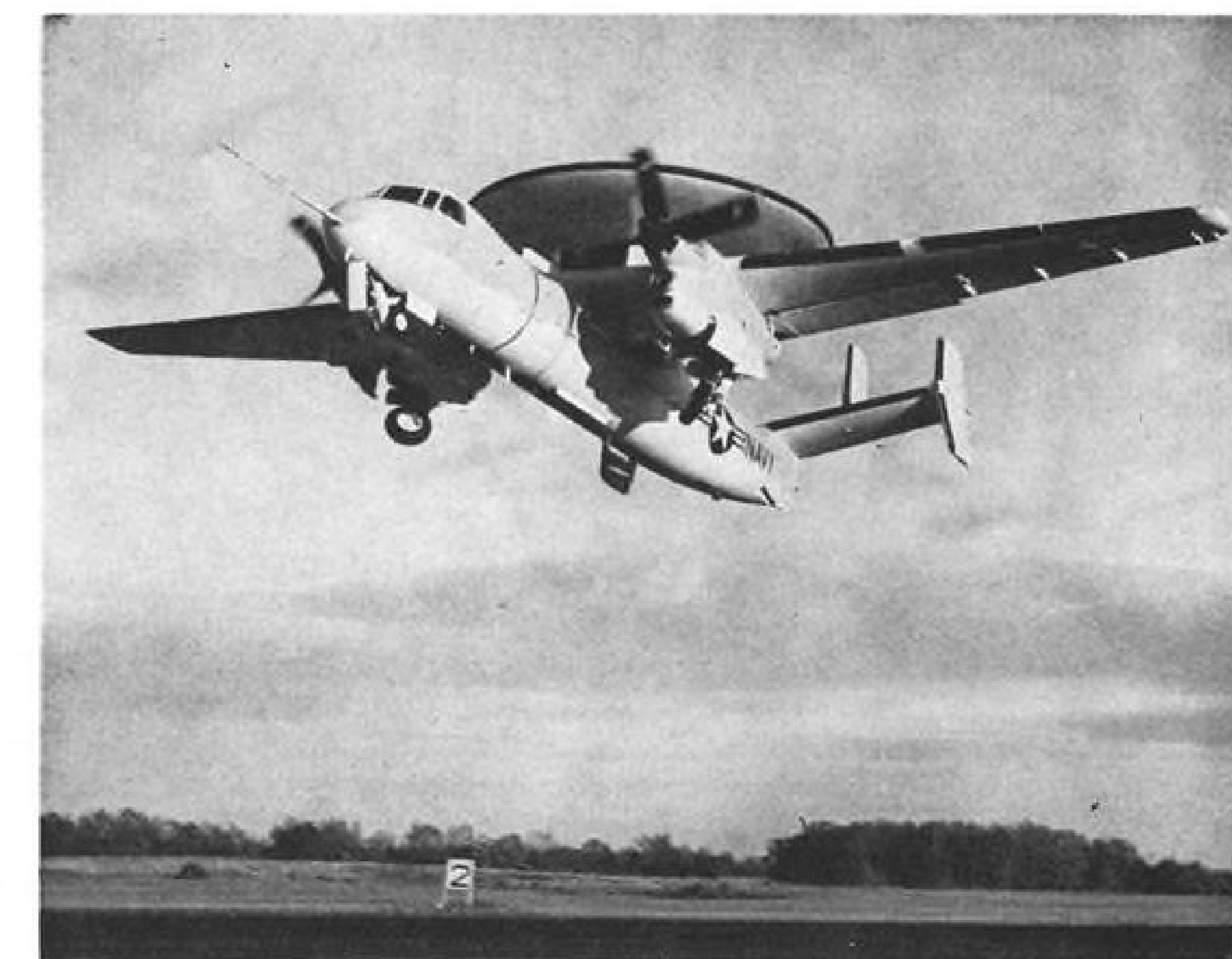
MAIN landing gear swivels up into nacelles of Allison T56-A8 turboprop engines rated at 4,050 eshp. each. Aircraft is designed for nose gear catapult launches.
