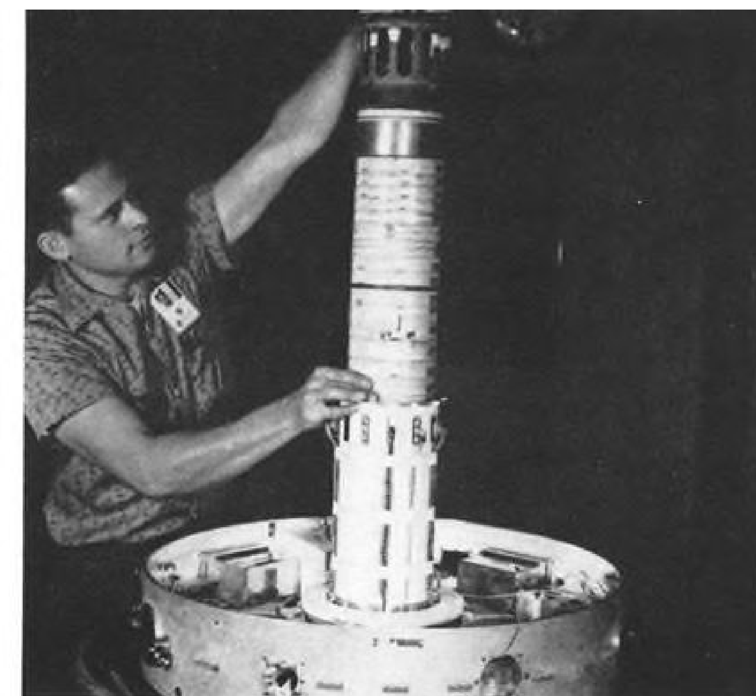
EXPLORER VIII satellite package is subjected to vibration test at left. Instrument column is assembled at right.
