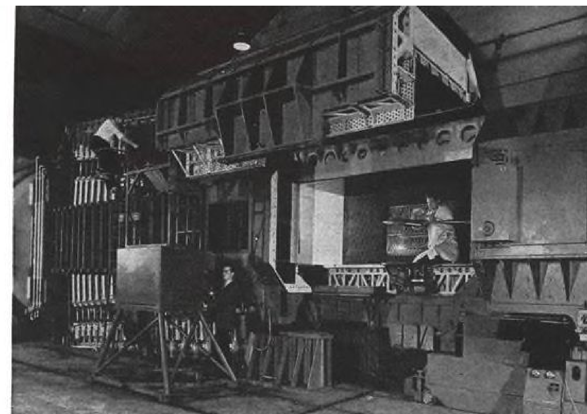
MAXIMUM running time of English Electric's Mach 4 test tunnel is 41 sec. at Mach 3.4.
