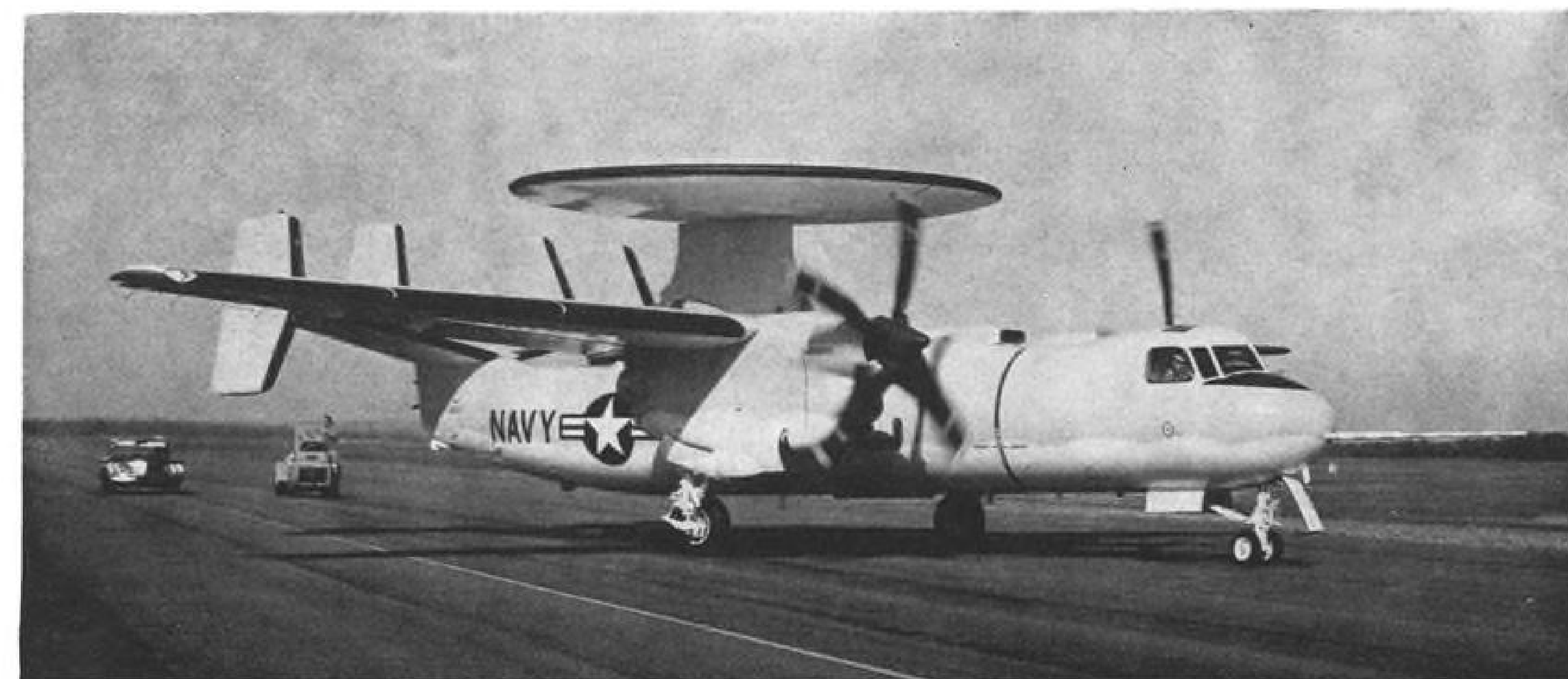
HAWKEYE is one of the largest aircraft designed for carrier operations. The rotodome must be lowered 2 ft. before the W2F can be taken below deck. The four-fin tail provides directional stability without exceeding 15-ft. hangar deck clearances.
