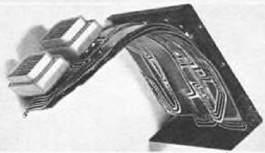
AFTER — Wiring Errors Eliminated; Weight, Cost and Time Saved Using Flexprint Wiring
