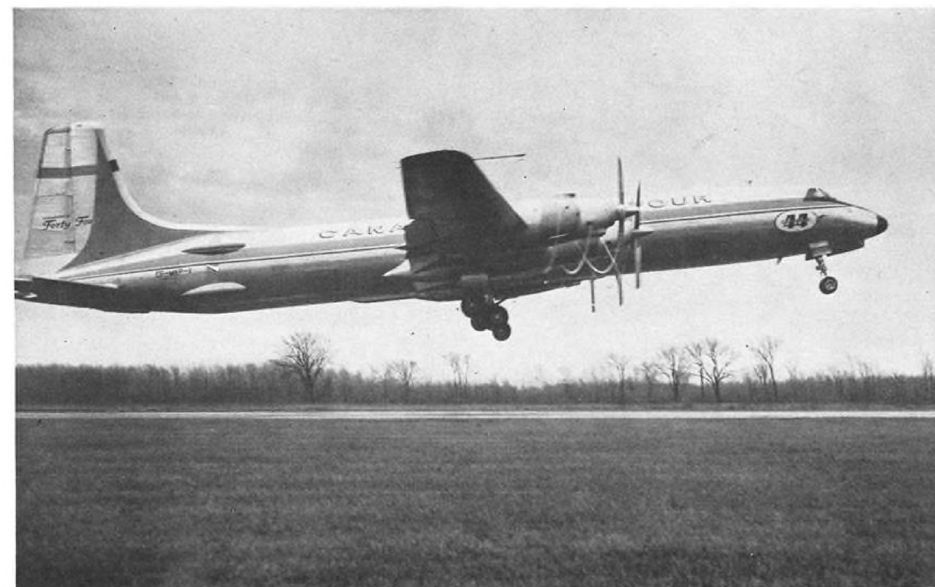
Swing-tail CL-44 is powered by four Rolls-Royce Tyne two-spool turboprops rated at 5,730 eshp, each at 15,250 rpm. at sea level.
