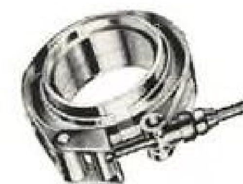
Lightweight and medium weight CONOSEAL tube and duct joints for lines from 1" through 12", pressures up to 20,000 psi., temperatures -325°F. to +1500°F. CONOSEALS are also available for rigid coaxial transmission line connections. Conform to MIL-1-26600 specifications.
