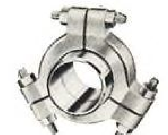
Heavy Duty CONOSEAL pipe joint for 1" through 12" nominal pipe sizes in a wide range of pipe schedules, pressures up to 20,000 psi., temperatures from -450°F. to +2000°F.
