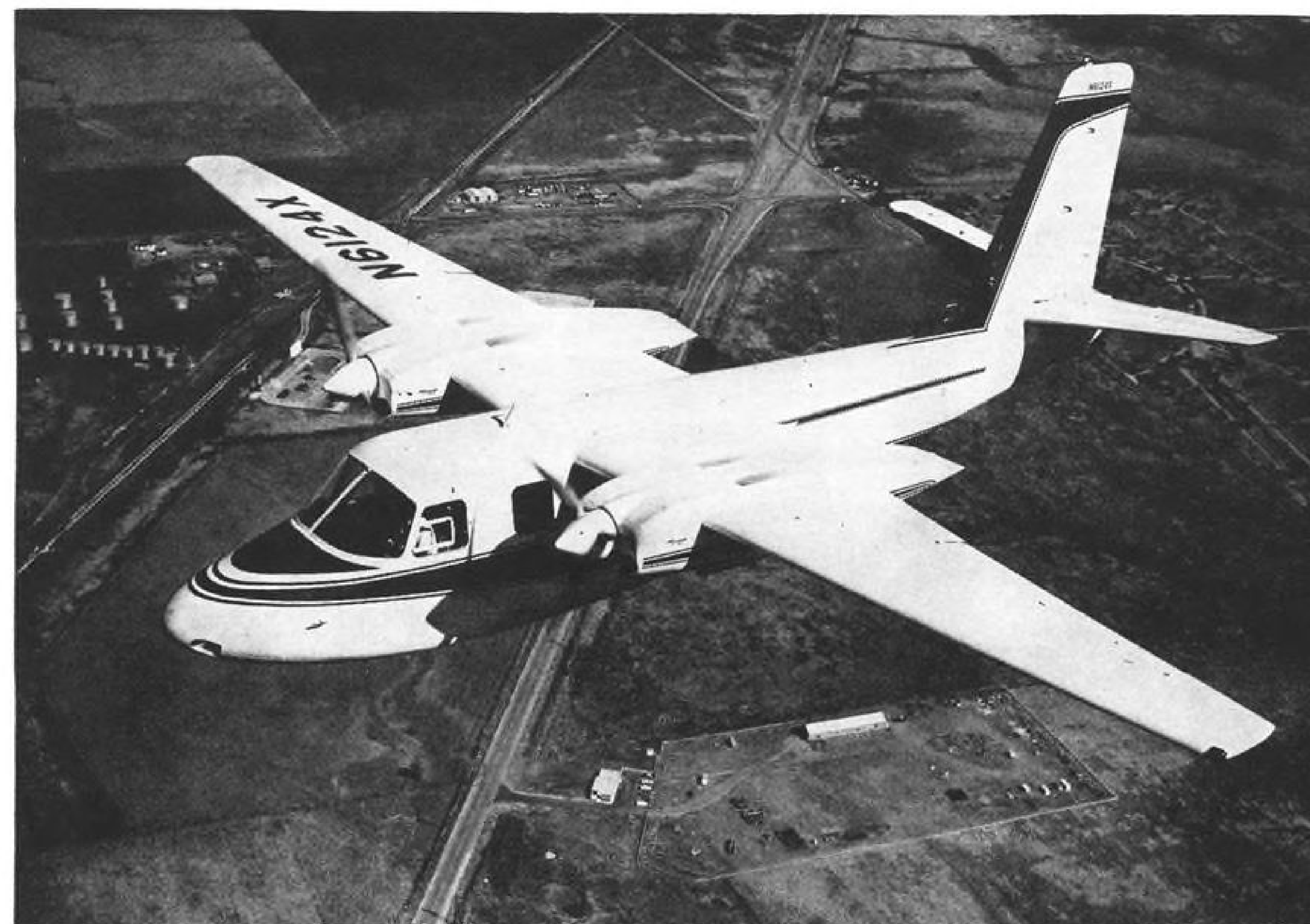
AERO COMMANDER 680F has new engines for higher power and speed. Nacelle air intakes have been repositioned. Price is $113,500.
