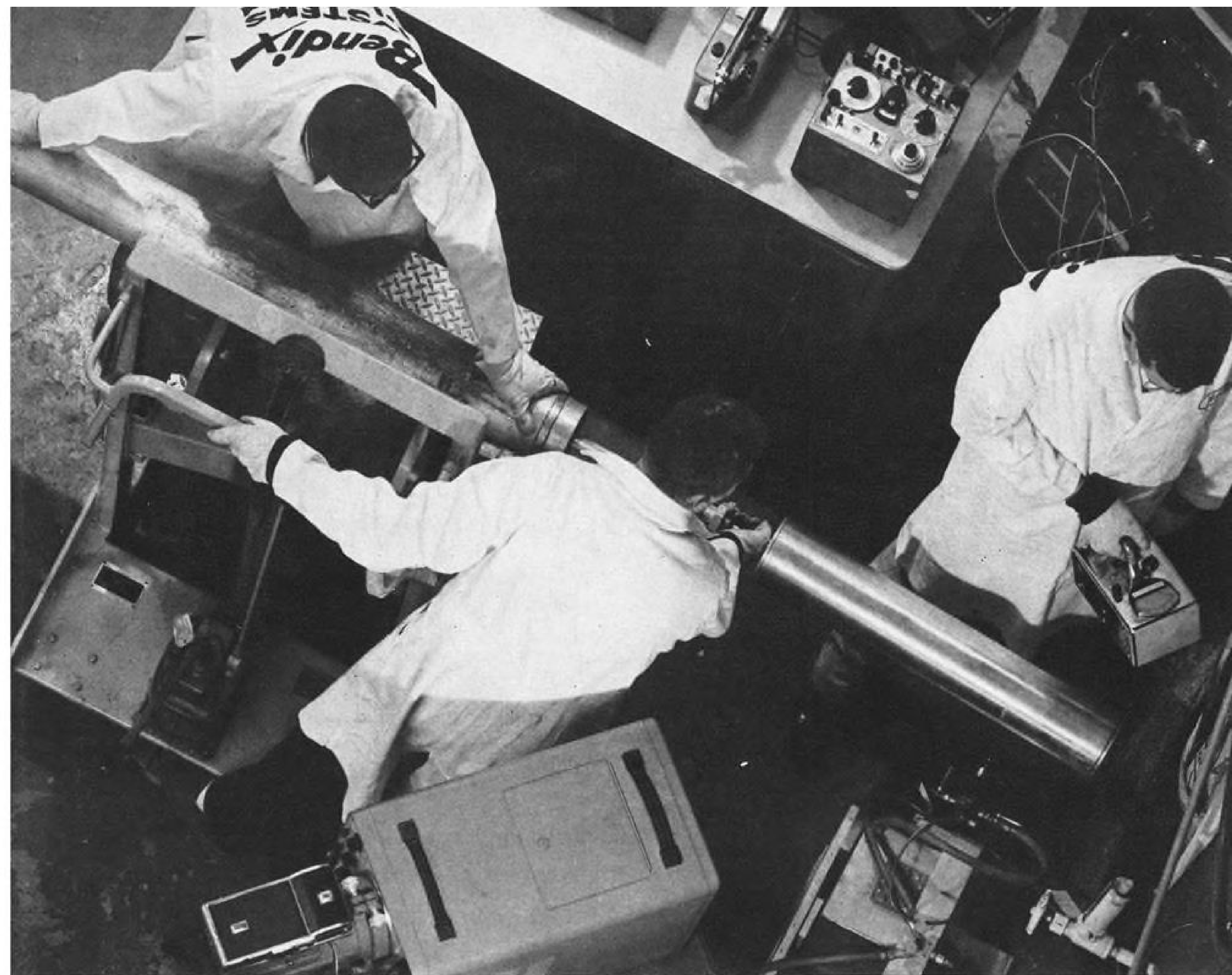
Electronic module being inserted into reactor beam port for irradiation.
