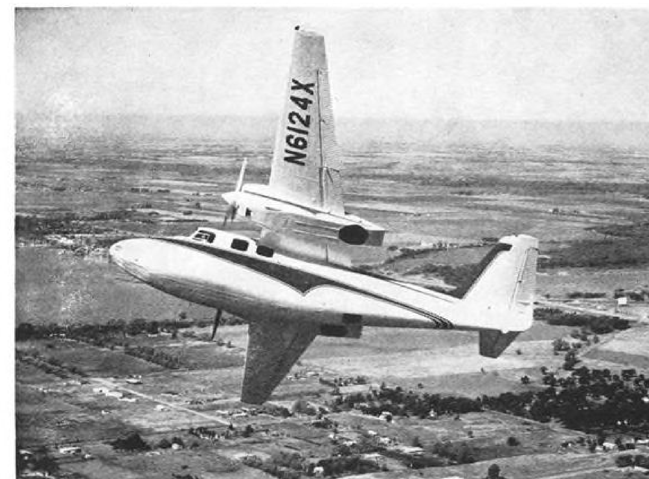
LANDING GEAR retracts flush into nacelle after a 90-deg. turn.
