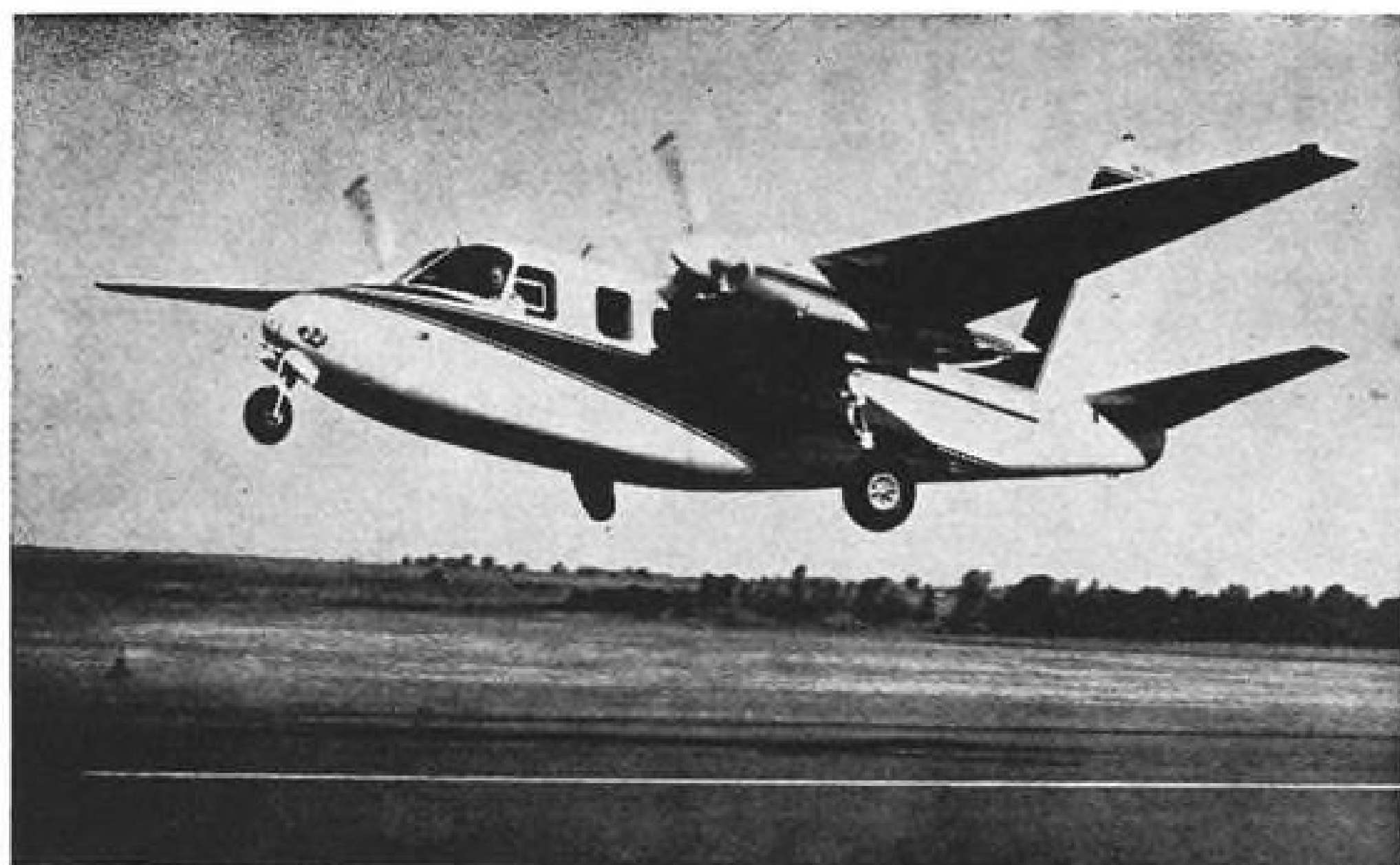
GEAR has just started retraction cycle in this view of a takeoff. Unstick speed is 80 mph.
