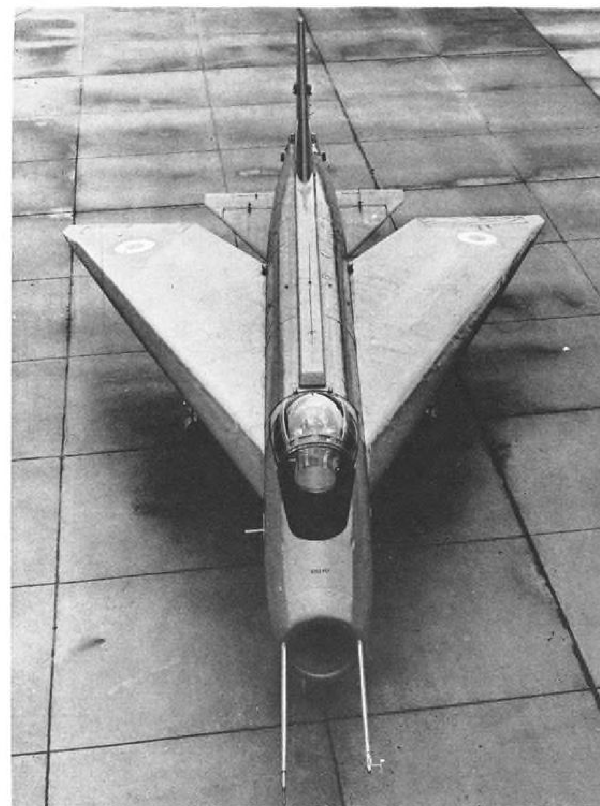
SHORT SB.5 recently made flight with adjustable wings swept back at 69-deg. angle.
