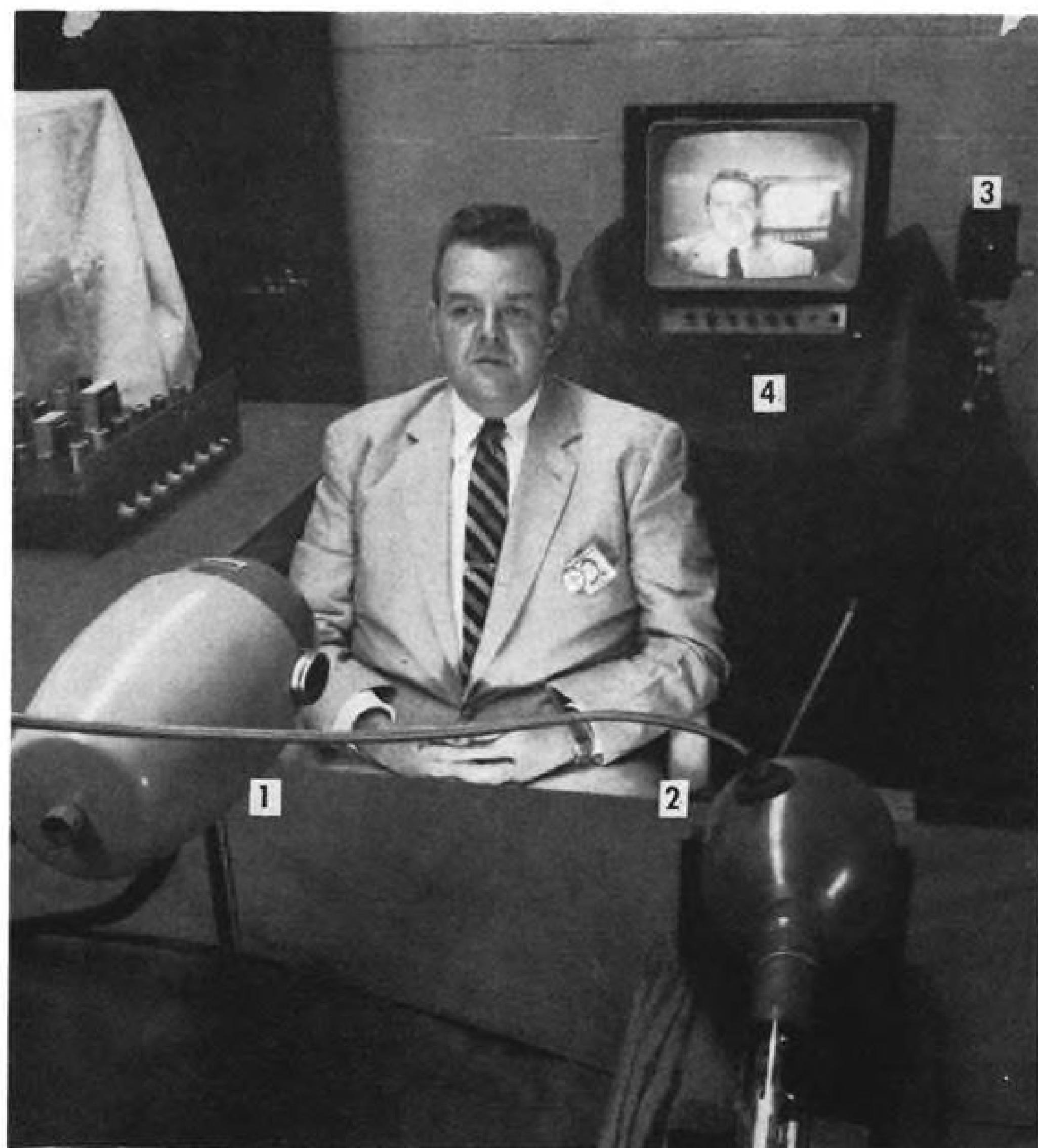
ULTRAVIOLET communications system, developed by Westinghouse Electric for use by space vehicles and communication satellites, is demonstrated in laboratory. Television camera (1) trained on subject produces signal used to modulate cathode ray tube (2) which produces narrow beam of ultraviolet radiation (not visible in picture). Ultraviolet beam is directed at photometer (3), which converts modulated ultraviolet into video signal displayed on TV monitor (4).
