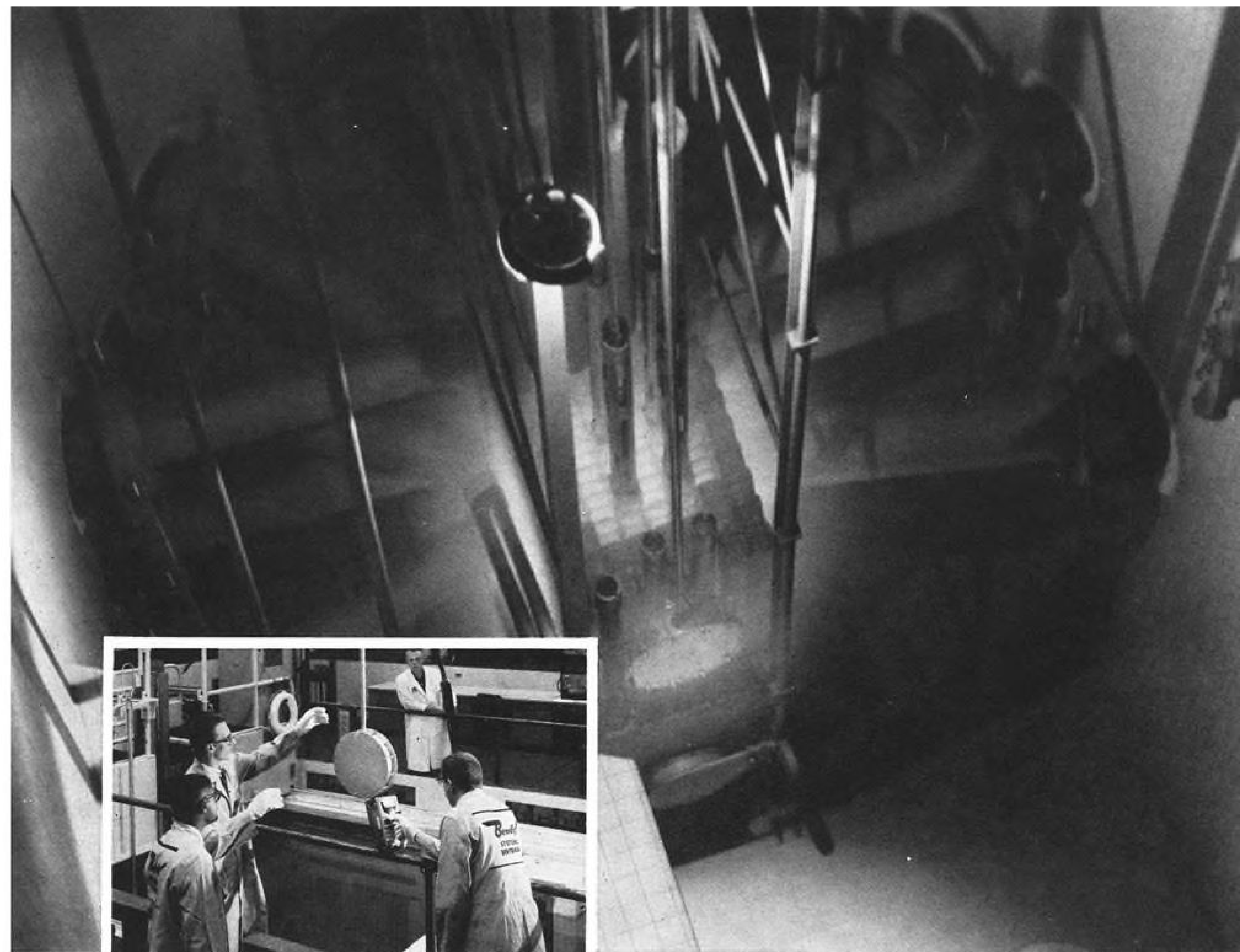
Electronic modules, enclosed in the Bendix "hot banjo" test chamber, are subjected to fast neutron and gamma radiation produced by The University of Michigan nuclear reactor.
