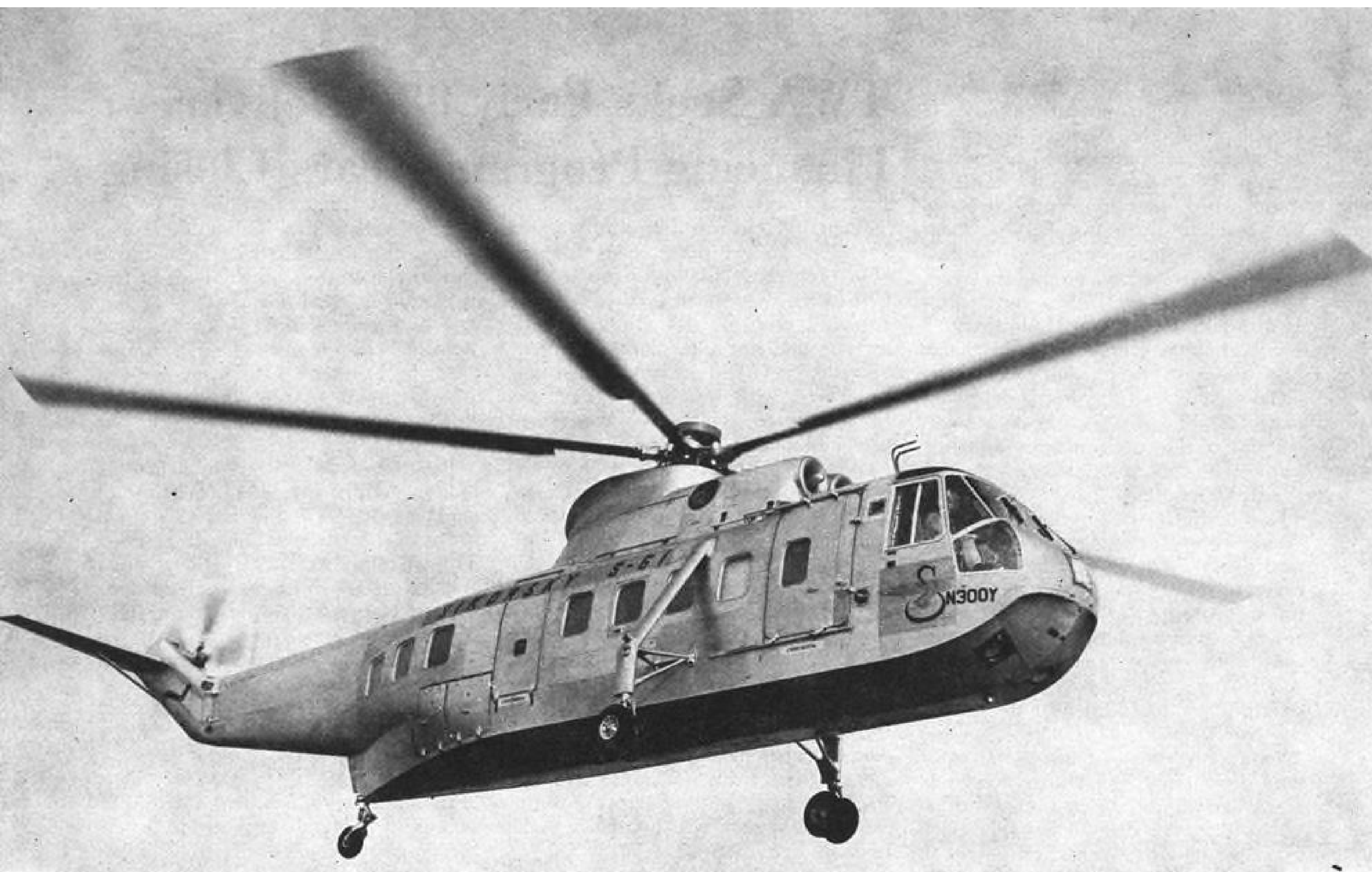
MAXIMUM capacity of Sikorsky's twin-turboshaft S-61L is 28 passengers. In this configuration, helicopter's cargo space totals 116 cu. ft., split between a removable baggage pod and two side-by-side bins in the aft right fuselage.
