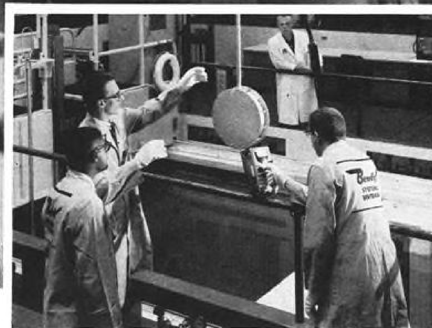
Electronic modules, enclosed in the Bendix "hot banjo" test chamber, are subjected to fast neutron and gamma radiation produced by The University of Michigan nuclear reactor.
