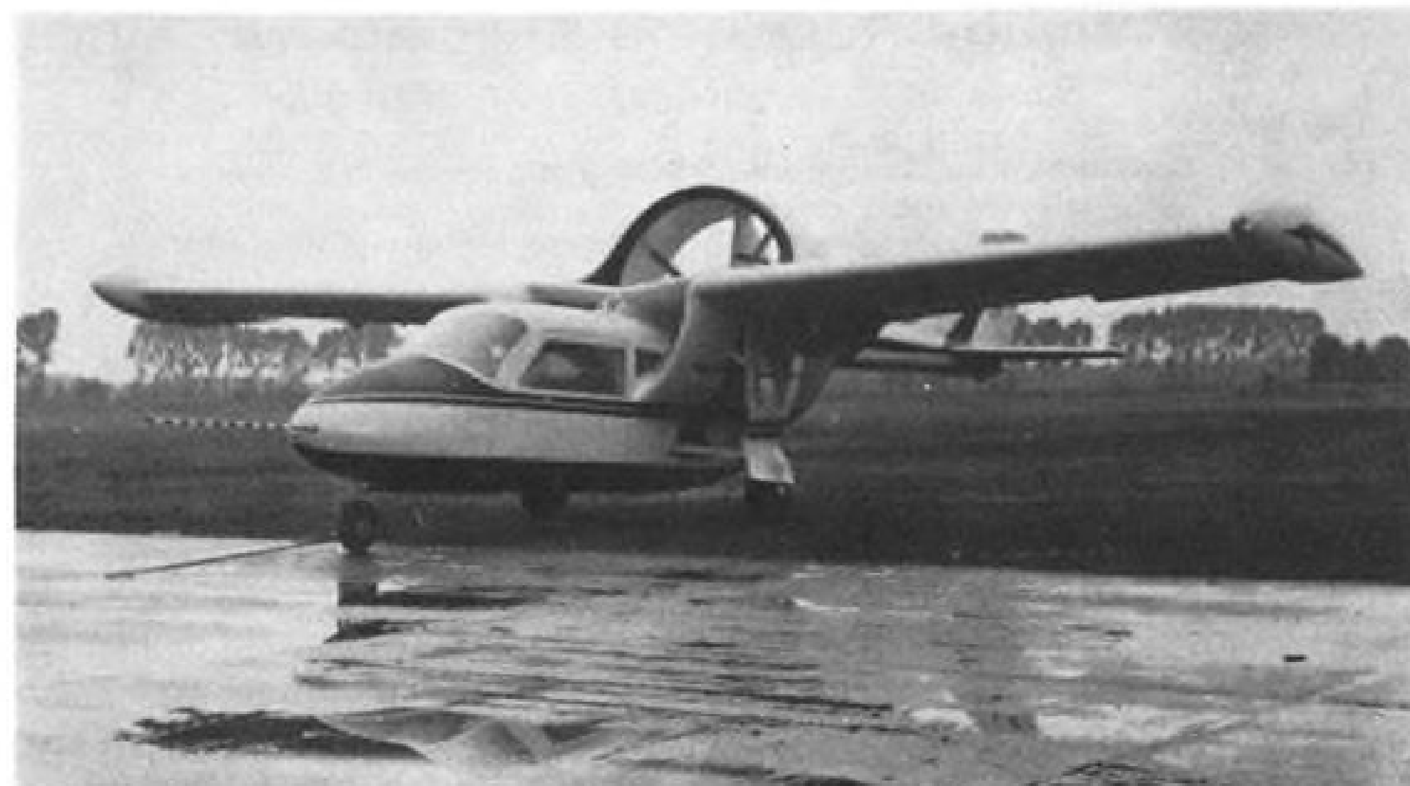
RF-1 executive plane features half-ring wing, thrust deflection flap and a pusher propeller mounted in the ring. Aircraft is scheduled to begin flight trials shortly.
