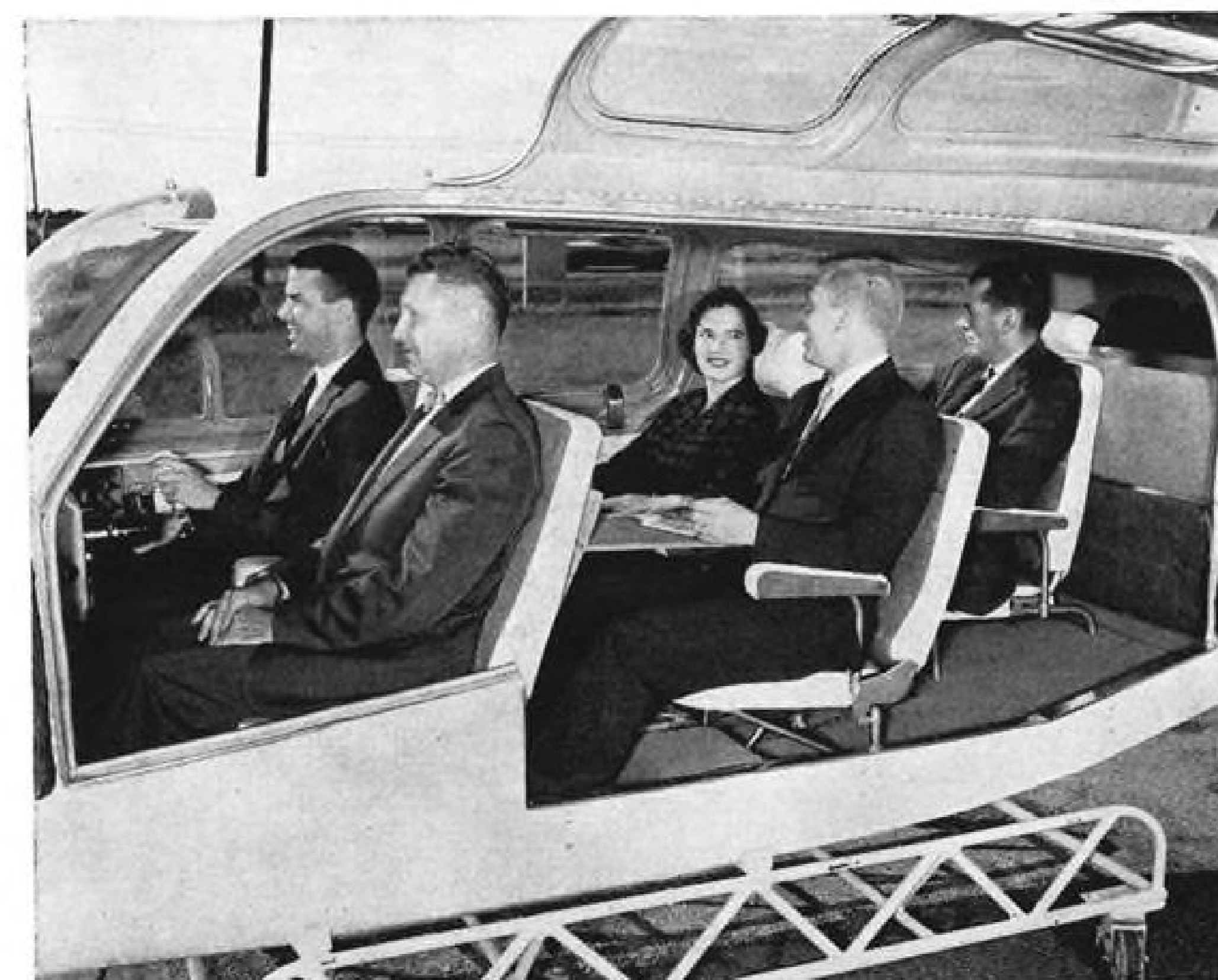
FIFTH seat installed in Baron cabin mockup is optional. Note rear baggage shelf above. Cabin configuration of the Baron is derived from Beech Travel Air cabin design. Baggage also is carried in the nose section of the Baron.
