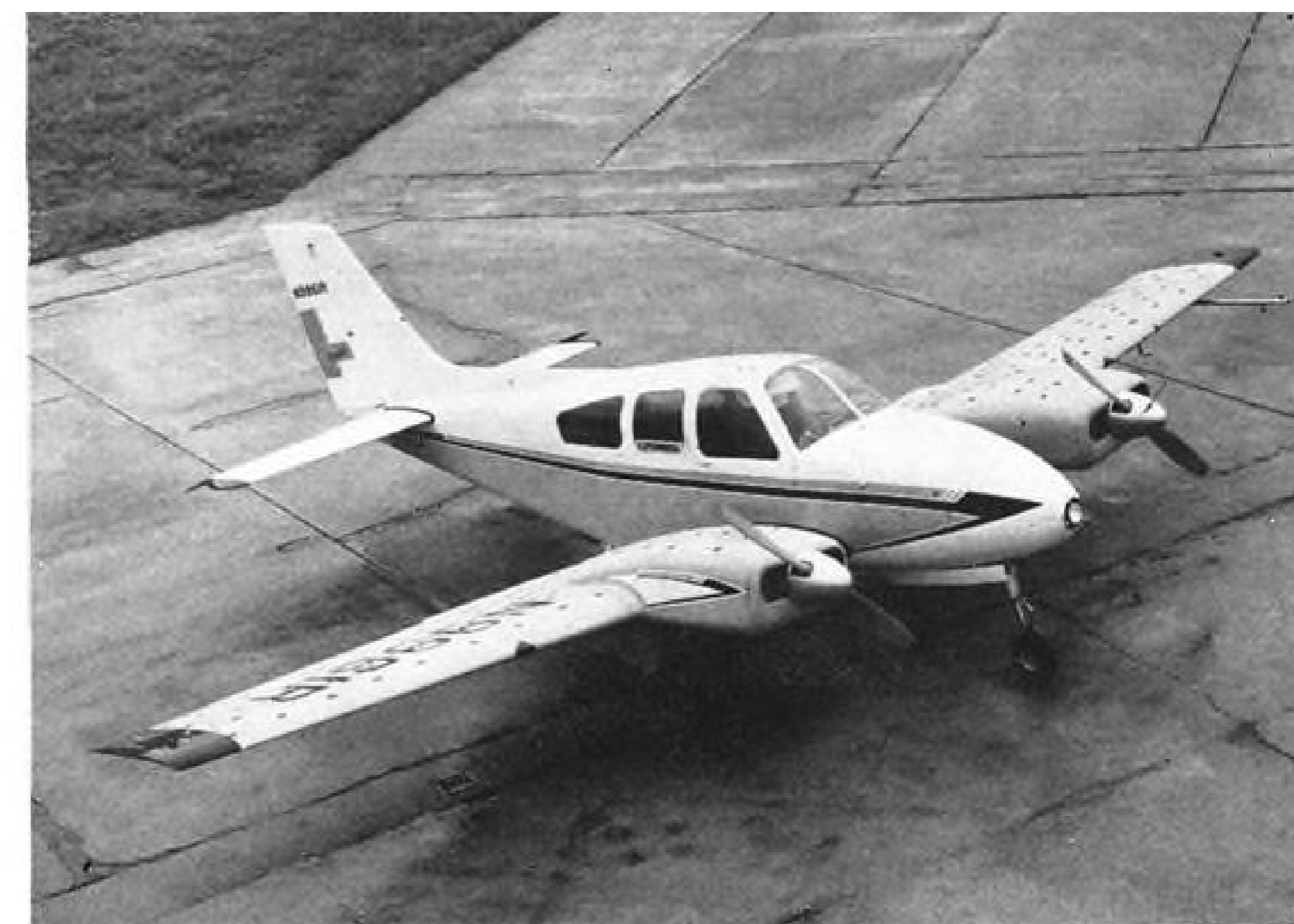
PROTOTYPE Baron has tufted wings for flight testing at Beech's Wichita plant.
