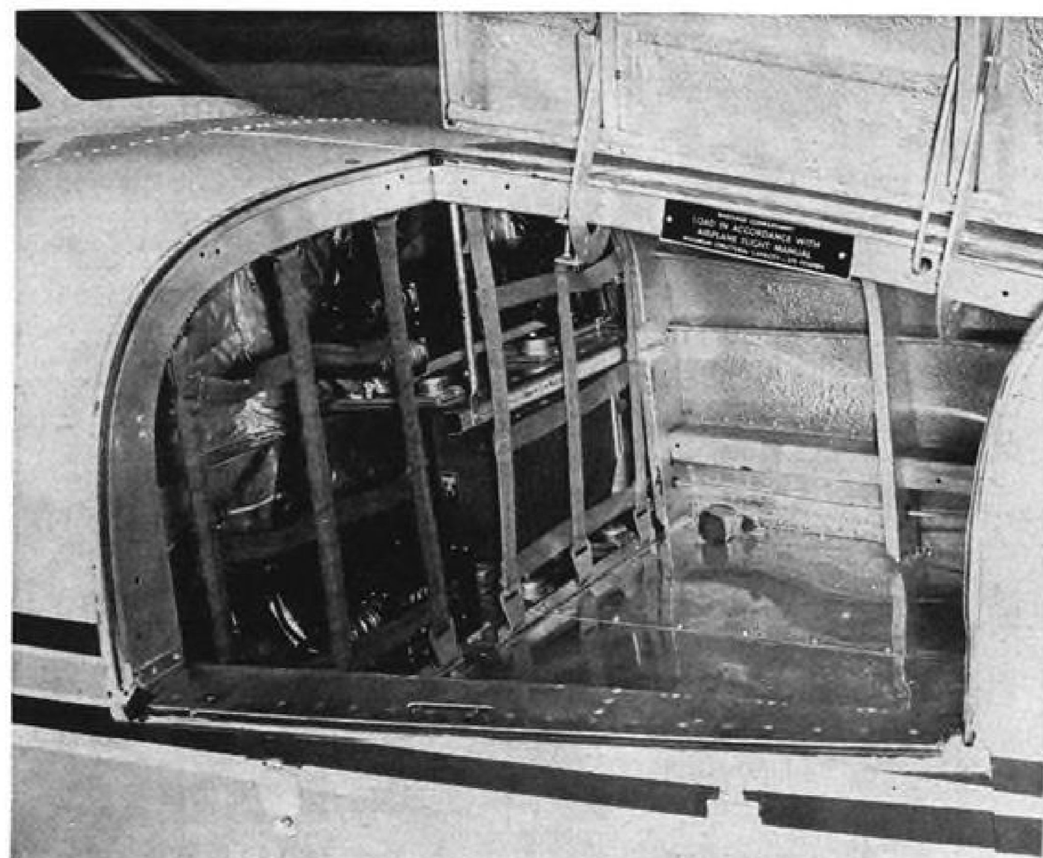
RADIO gear is stowed in aft of nose baggage compartment. Battery is below flooring level.
