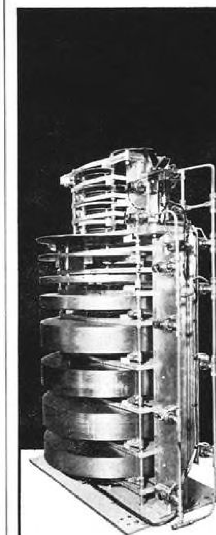
BINARY LOADING 60,000 POUND DEAD WEIGHT CALIBRATOR
