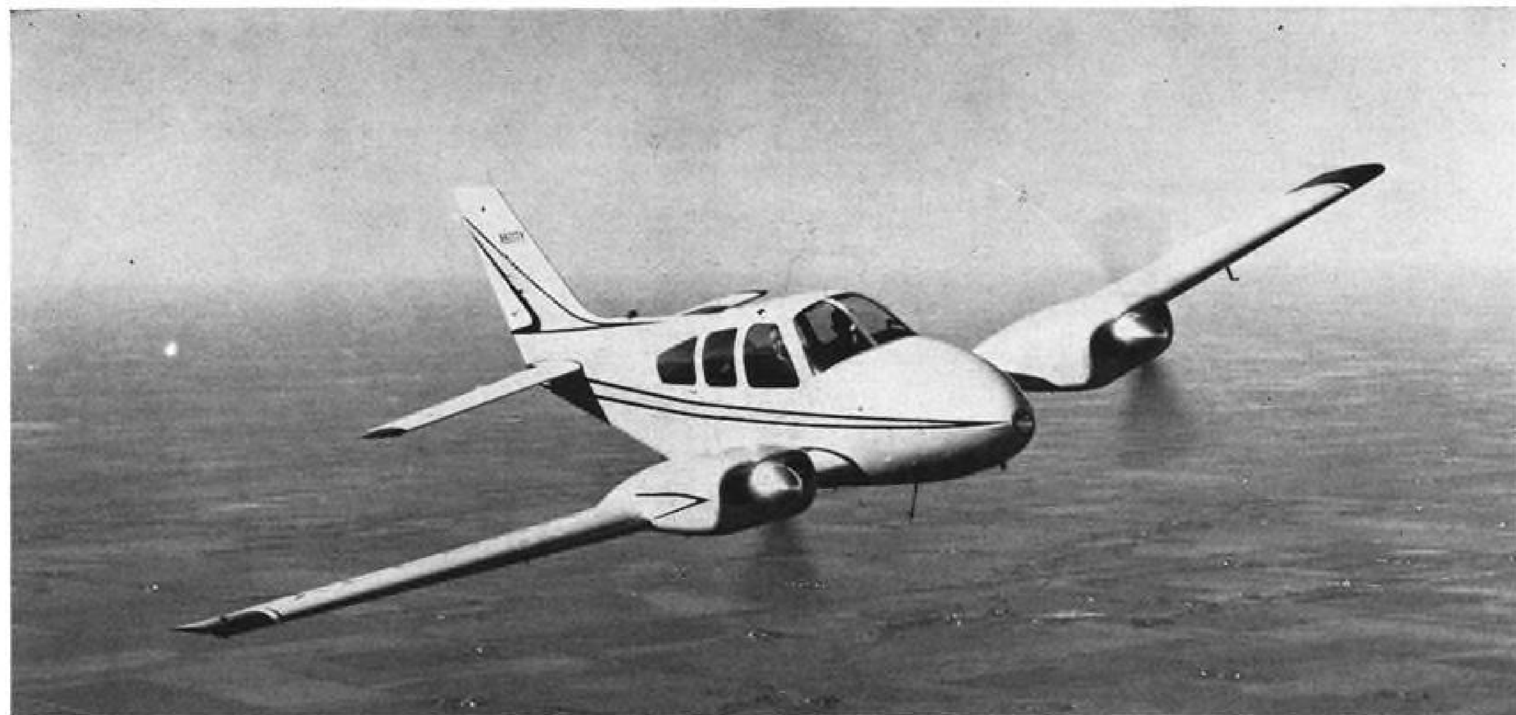
FLAT nacelles designed for the Continental IO-470-L fuel injection engines on the Beech Baron twin are 78 in. wide.
