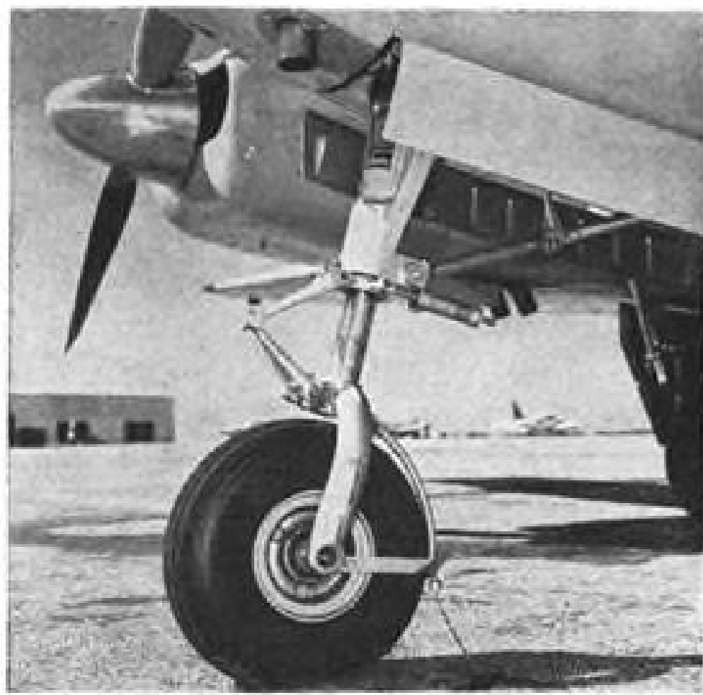
NOSE wheel is adapted from Travel Air; gear is stressed for 600 fps.
