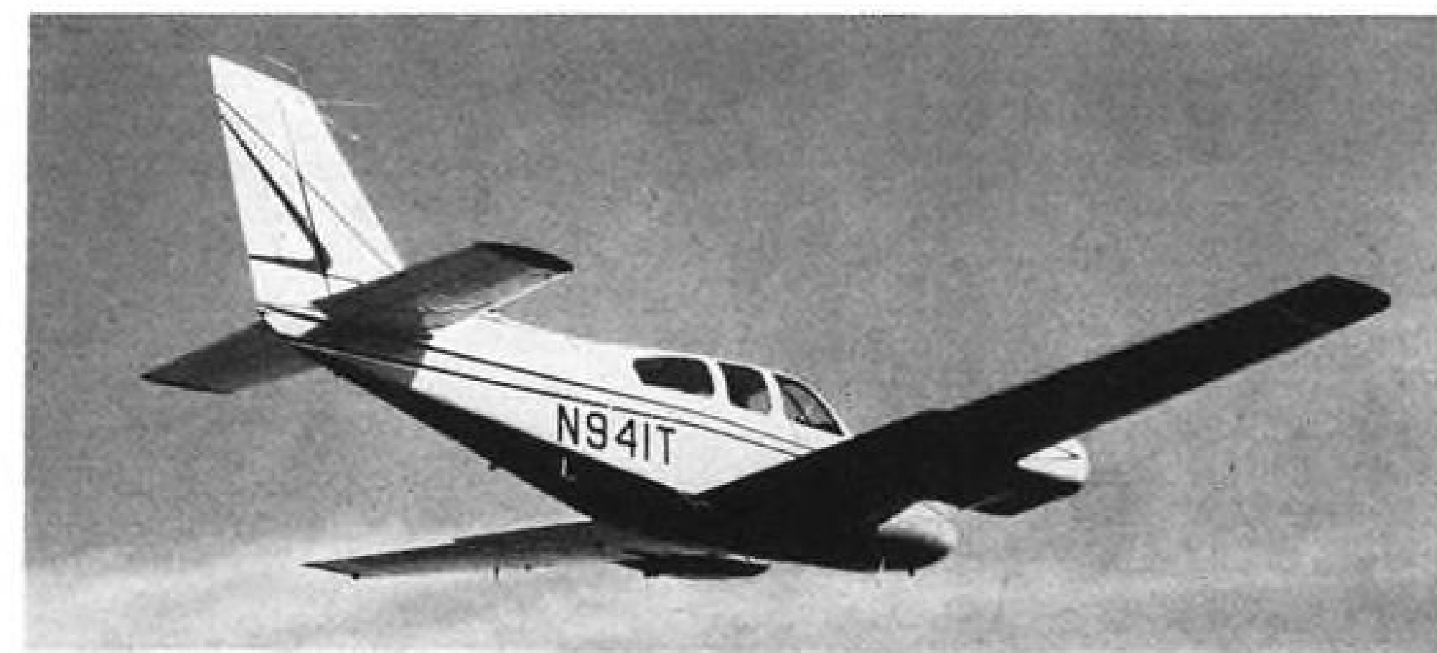
SWEPT tail is dominant design feature of the new Beech Baron twin, now in production.
