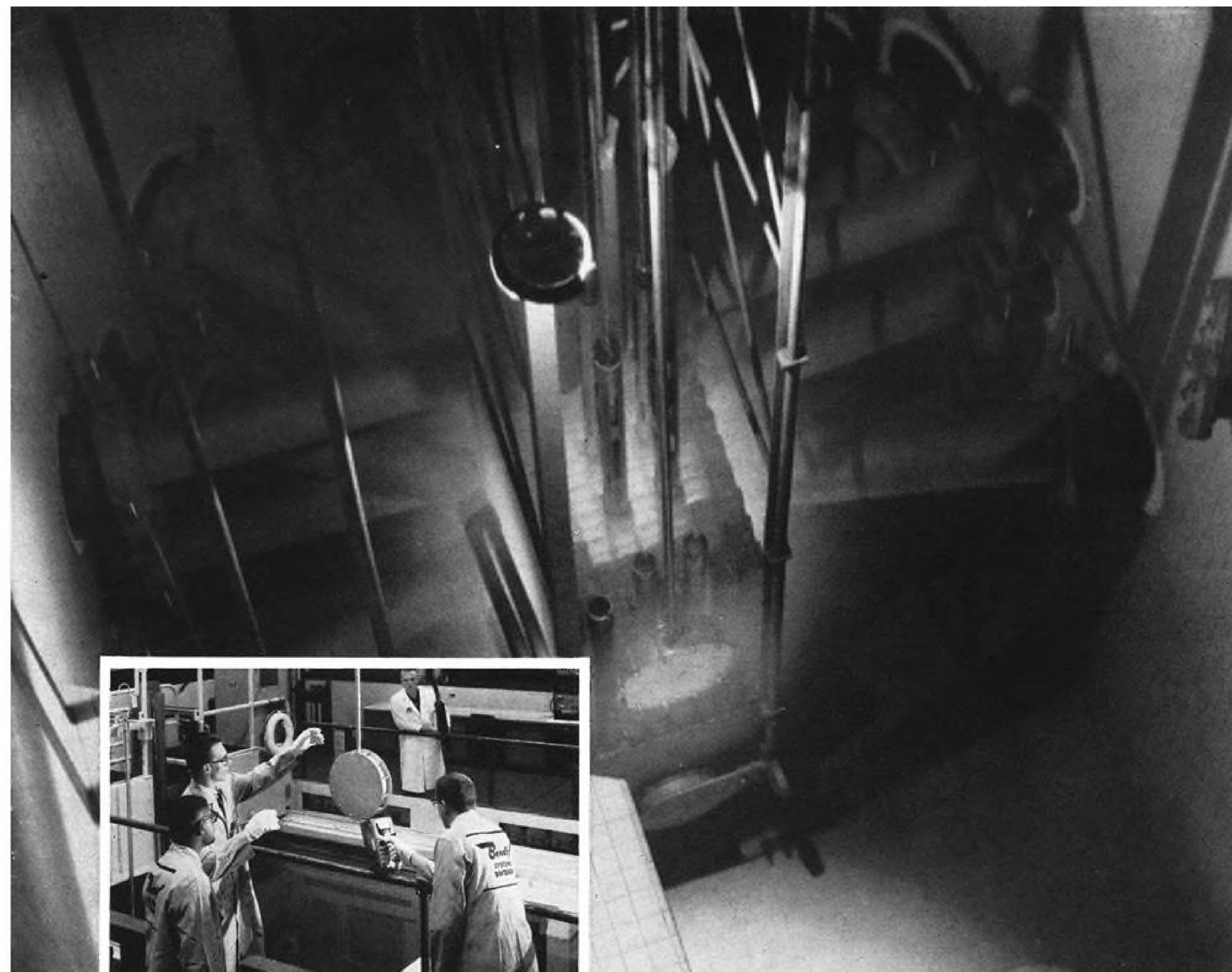
Electronic modules, enclosed in the Bendix "hot banjo" test chamber, are subjected to fast neutron and gamma radiation produced by The University of Michigan nuclear reactor.
