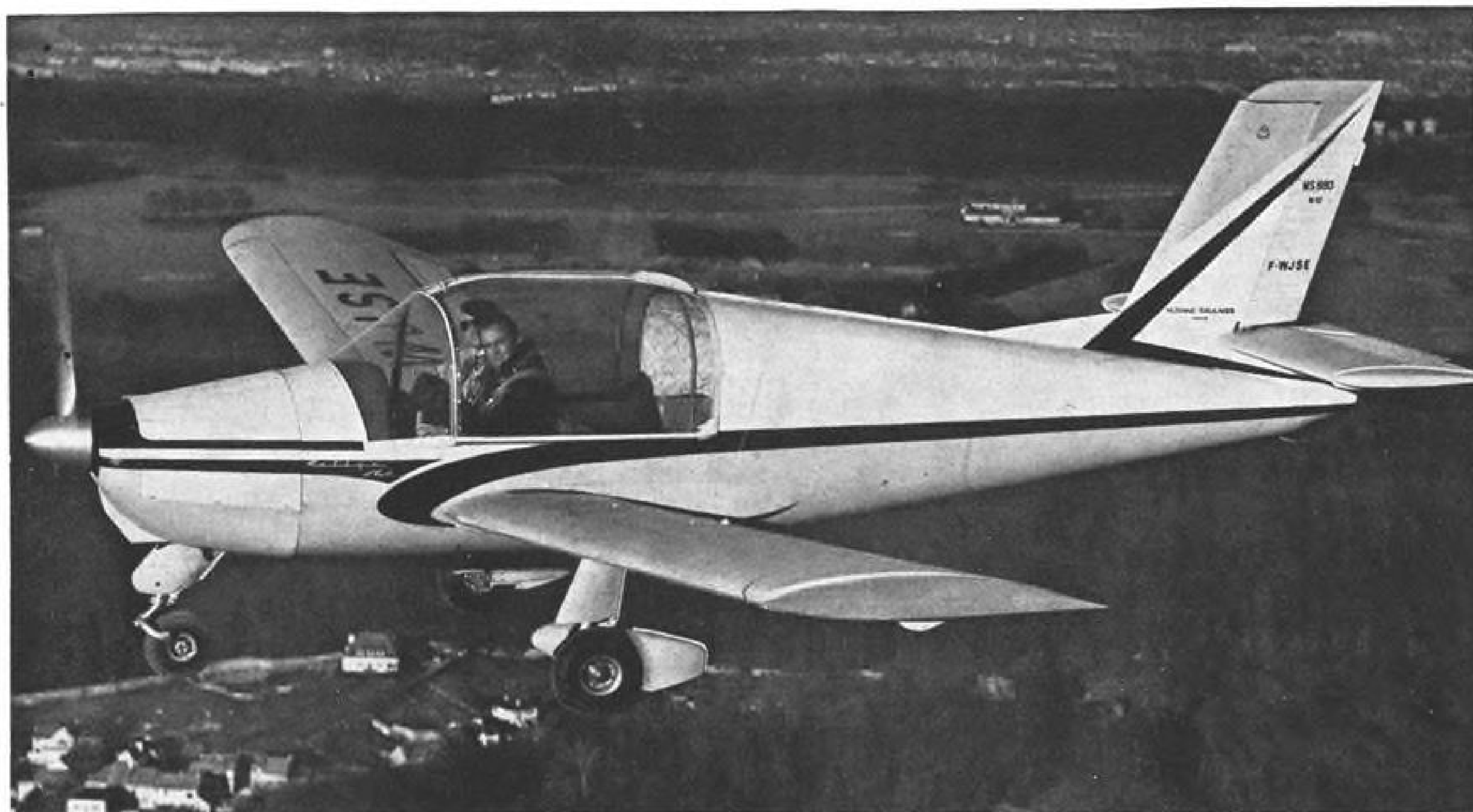
SECOND prototype of Morane-Saulnier MS-880 Rallye is shown on its first flight Feb. 10. Plane is powered by a 100-hp. Continental engine. The No. 3 airplane will be sent to the U.S. for demonstration purposes. Marked change for first Rallye is its sweptback tail.
