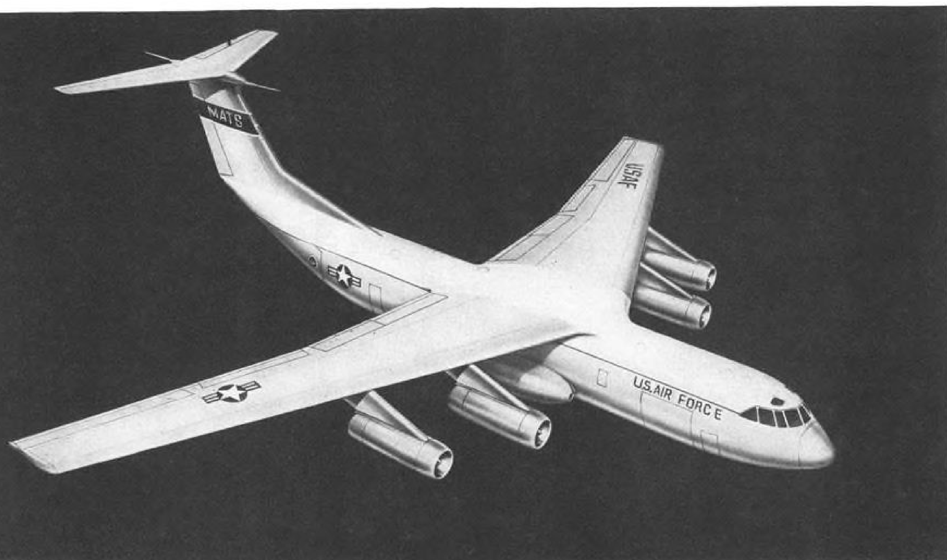
LOCKHEED SS-476L TRANSPORT , which the company calls the Super Hercules, has a full-width fuselage loading ramp to expedite movement of bulky cargo and an aerial delivery system that permits dropping cargo in flight. It will be powered by turbofans.
