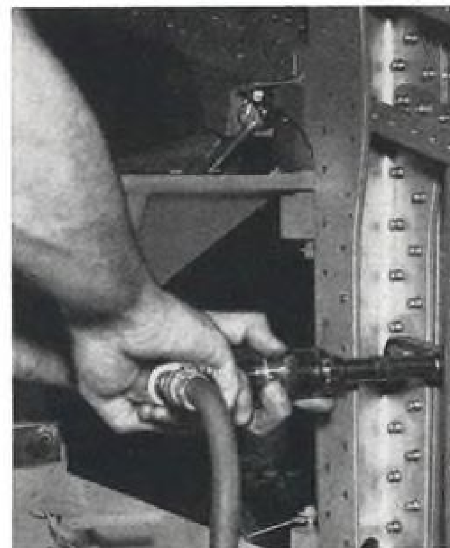
Hi-Lok 2" offset extended adaptor fitted to an Ingersoll-Rand Air Motor reduces a 2-man, 32-hour assembly job on the landing gear steel support rib to a one-man, 4-hour job. Additionally, the change to Hi-Loks reduced the installed fastener rejection rate from 30% to practically nil.
