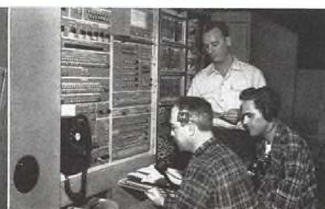
The Checkout Data Processor generates simulated missile attacks and evaluates the BMEWS response to the simulation.
