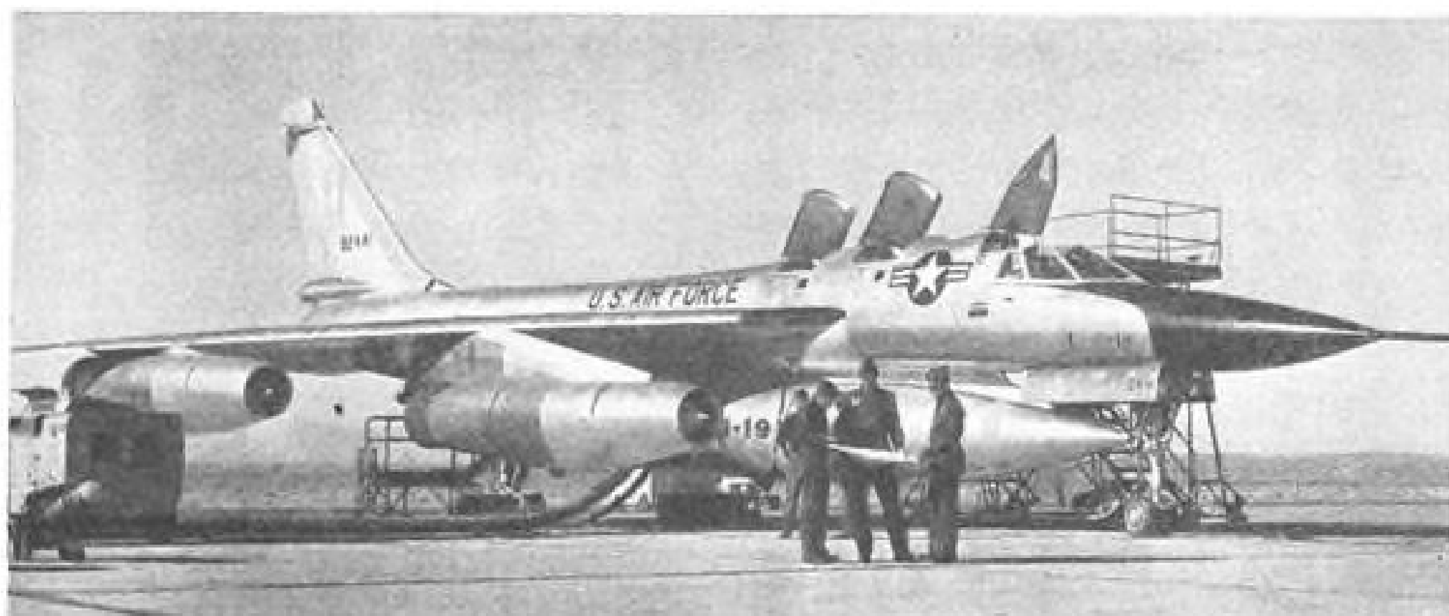
One of SAC's record-breaking B-58 flight crews checks final flight plan prior to takeoff. This J79-powered Hustler logged a top speed of 1430 mph during its run.
