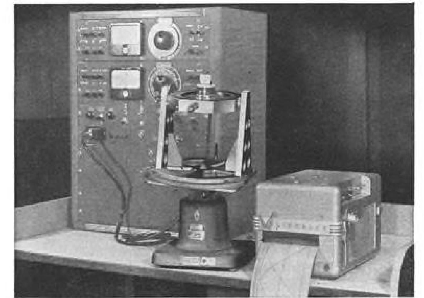
In this simple bench set-up, the 906 Visicorder is at right. Between it and the control panel is the Scorsby table on which the gyro is mounted, ready for test.
