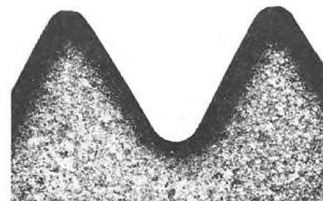
Carburization because of faulty atmosphere control during heat treatment. Surface carburization—indicated by dark layer—results when bolt is heat treated in high carbon atmosphere after threads are rolled.
