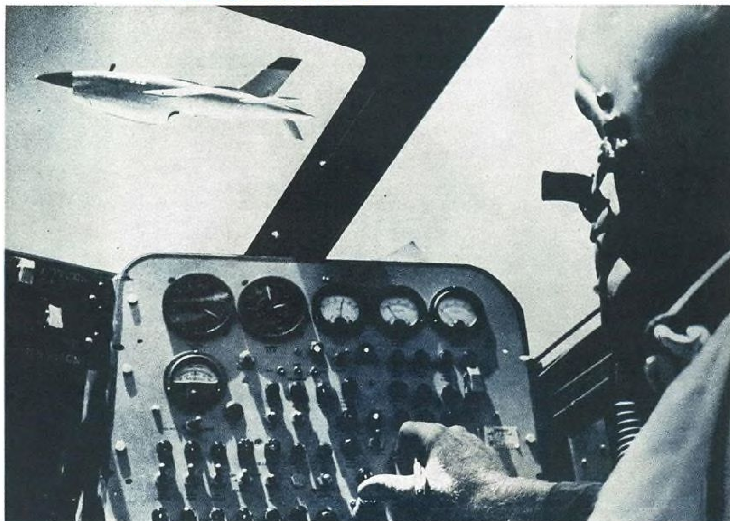
Firebee is precisely maneuvered by remote controller as he receives flight data transmitted from Dorsett telemetry system in the drone.
