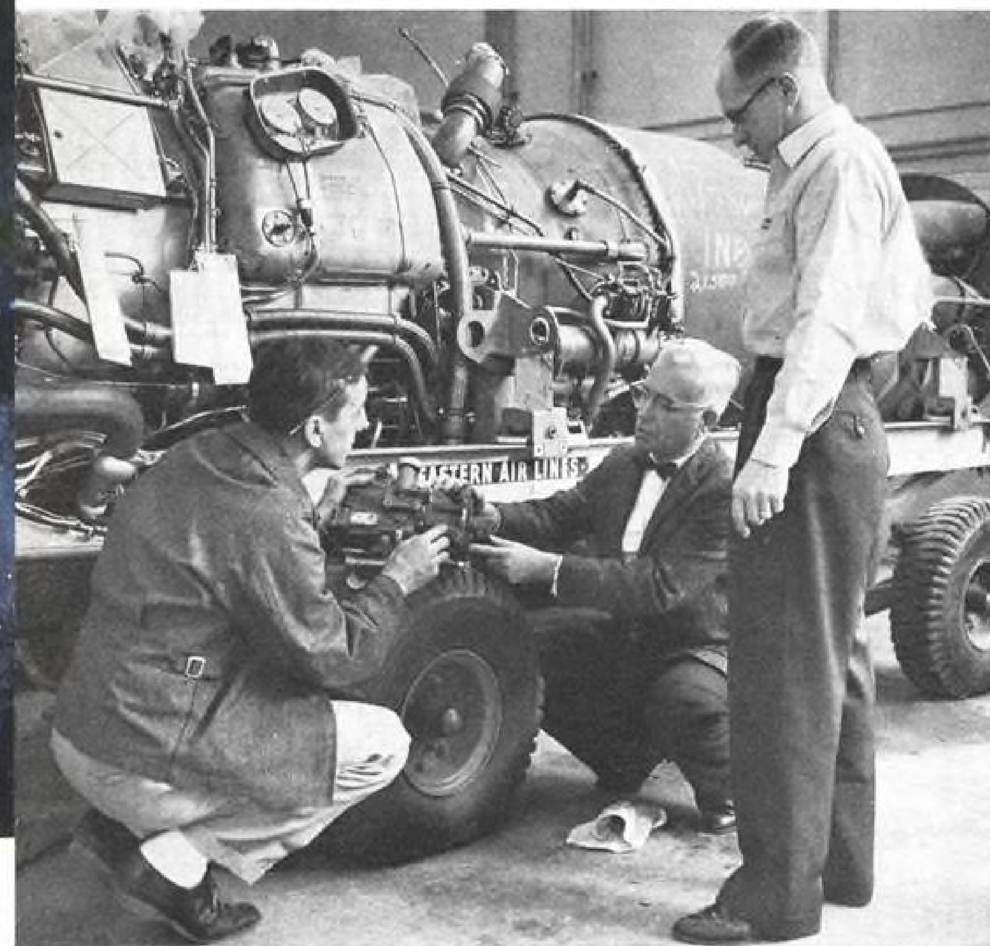
At Eastern Air Lines Miami base Howard Crothers of Vickers checks installation of DC 8-B pump at service test unit with L. Nuchols, foreman, and J. Schoettle, lead mechanic.
