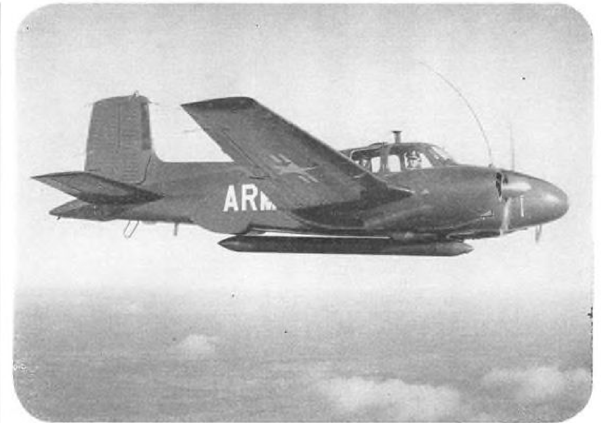
U. S. Army L23D produced by Beech Aircraft—equipped with AN/APQ-86 all-weather, high resolution reconnaissance radar, developed and built by TI in cooperation with the U. S. Army Signal Corps.
