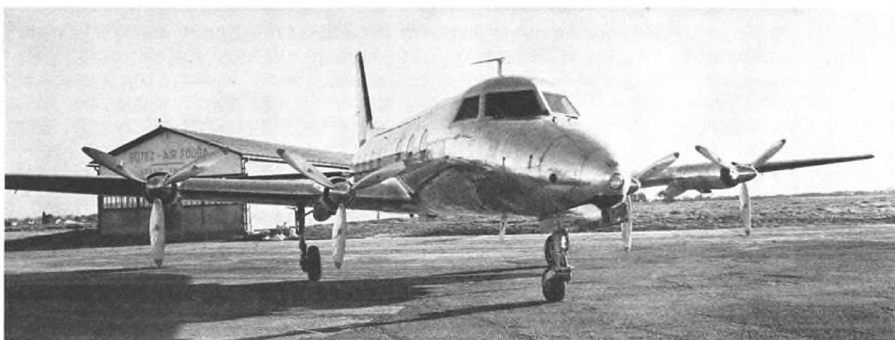
Gross weight of P.840 light transport is 16,750 lb. Plane, being prepared for first flight at Toulouse, is powered by four Turbomeca Astazou II turboprops delivering 530 hp. each, and can carry a 5,300-lb. payload at 300 mph. cruise speed (AW Feb. 29, 1960, p. 50).
