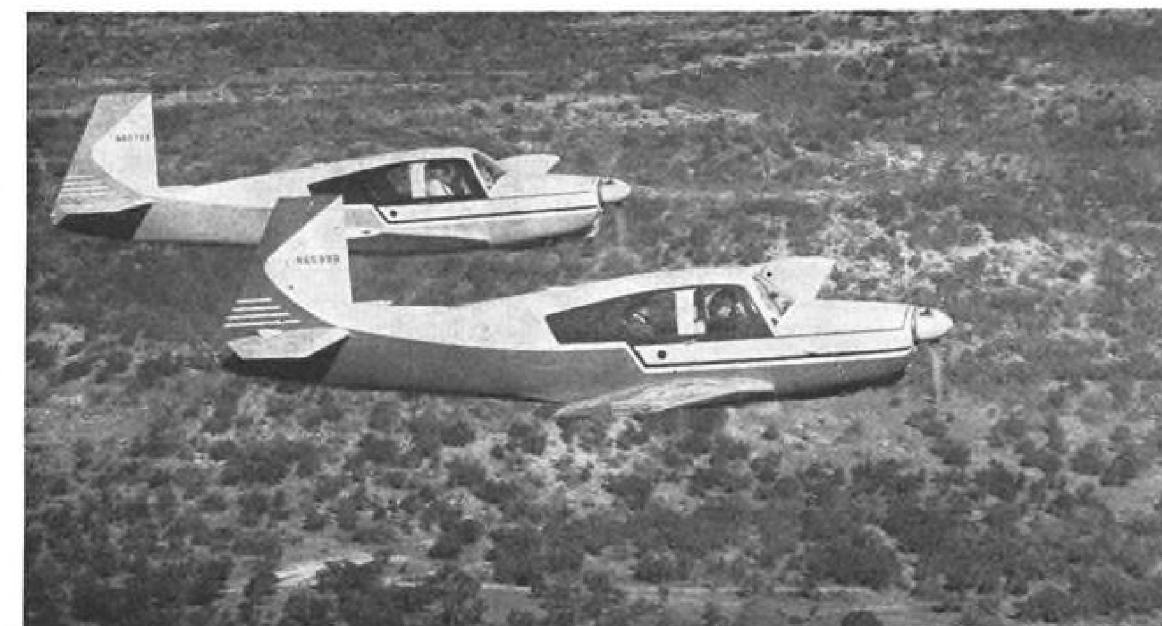
MARK 21 fuselage consists of welded chrome-molybdenum steel tube frame with aluminum skin. Fuselage tail cone section has been redesigned for added strength.
