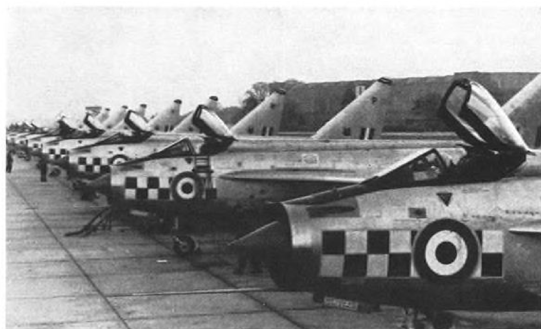
ENGLISH ELECTRIC Lightning pilots man their aircraft on 3 min. alert at Wattisham RAF station. Only one of these Lightnings was kept on ground during scramble. Bullet in nose intake of each plane contains Ferranti Airpass radar.
