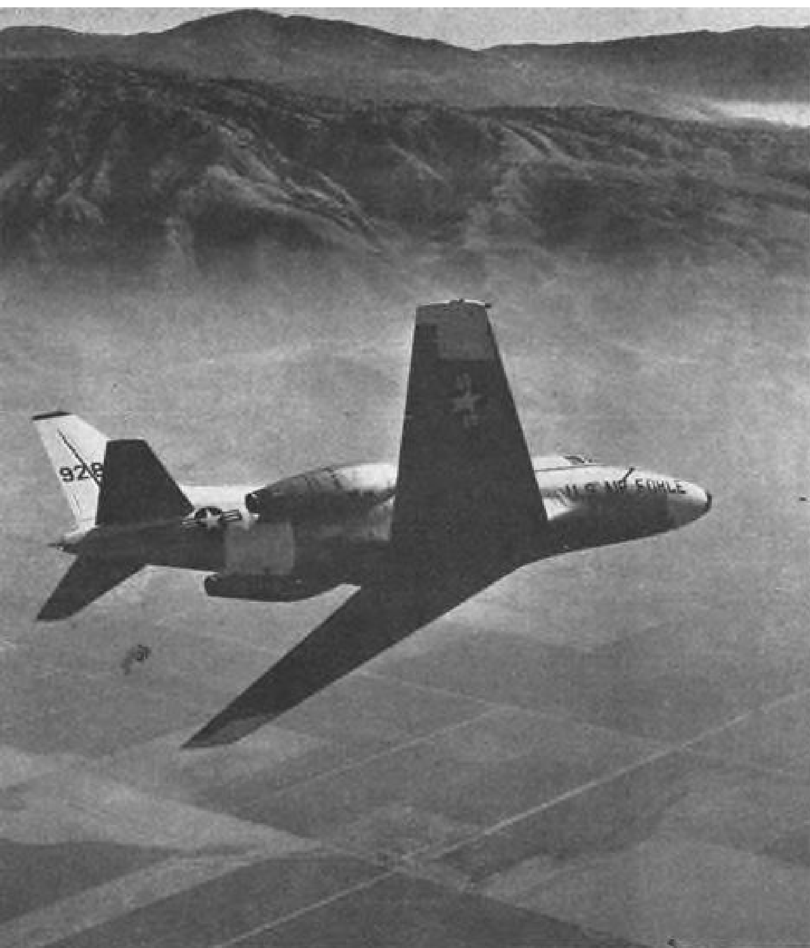
T-39 SABRELINER shown during test flight over Palmdale, Calif. Plane can be flown by one pilot, so all flight controls and instruments are accessible from left seat. Copilot's panel is fully instrumented for navigational and instrument proficiency training.
