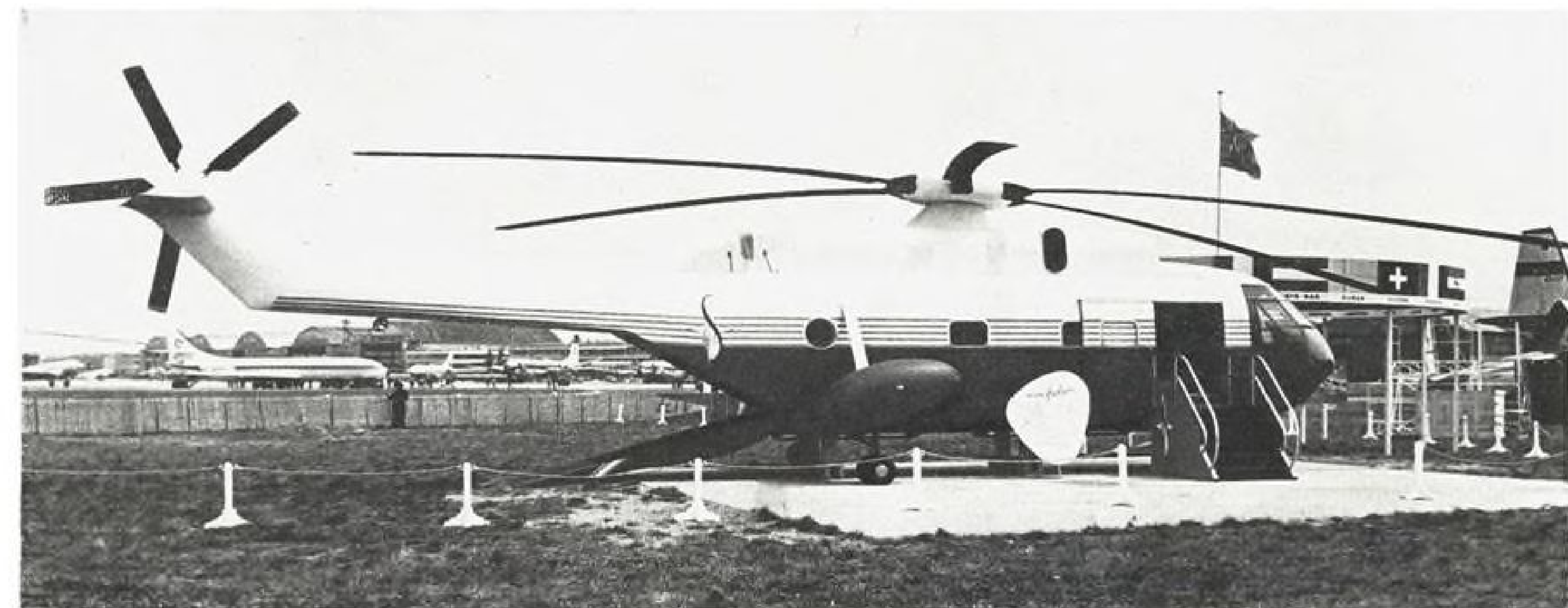
FULL-SCALE MOCKUP of the Sud 3210 Frelon heavy helicopter, successor to the Frelon 3200 prototype now undergoing flight test trials, can carry a total of 27 troops at a maximum gross weight of 24,250 lb. and a useful load of 11,020 lb. On order by the French navy and West German Defense Ministry, the 3210 has six main rotor blades as opposed to four on the 3200. Tail rotor blades also have been lengthened and a horizontal tail fin added to aid stability. Powered by three Turmo IIIC turboprop powerplants rated at 1,320 hp. each, the Frelon has a maximum sea level speed of 135 kt., a cruising speed of 119 kt.
