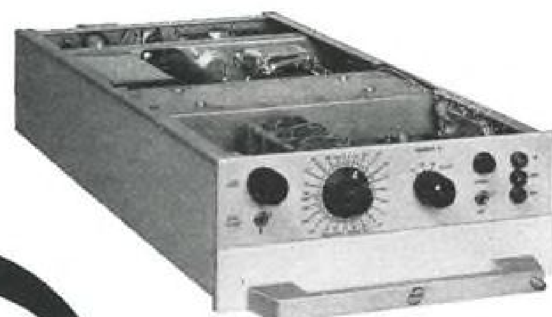
SWITCHABLE FM TEST OSCILLATOR Single channel continuously variable from 200 cps to 500 KC. All IRIG channels indexed. Provision for arbitrary center frequency index storage. Capable of precision voltage-controlled FM modulation. Standard deviations \pm 7.5 , 15, and 40%. Fixed or adjustable intermediate deviation values available. MODEL GSO-1
