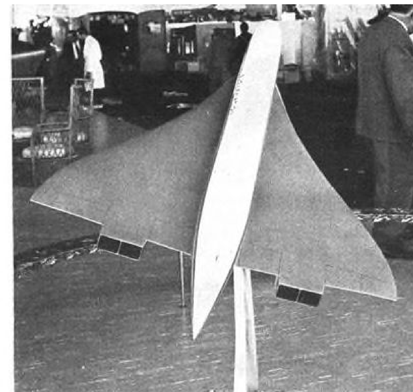
MODEL of the proposed Sud-Dassault Super Caravelle supersonic transport shows wing design configuration. Plane will be developed jointly by Sud Aviation and Marcel Dassault. Powerplants to be used on the Super Caravelle have not yet been determined. Inlet design under the wing is boxed-intake type similar to that on the B-70.
