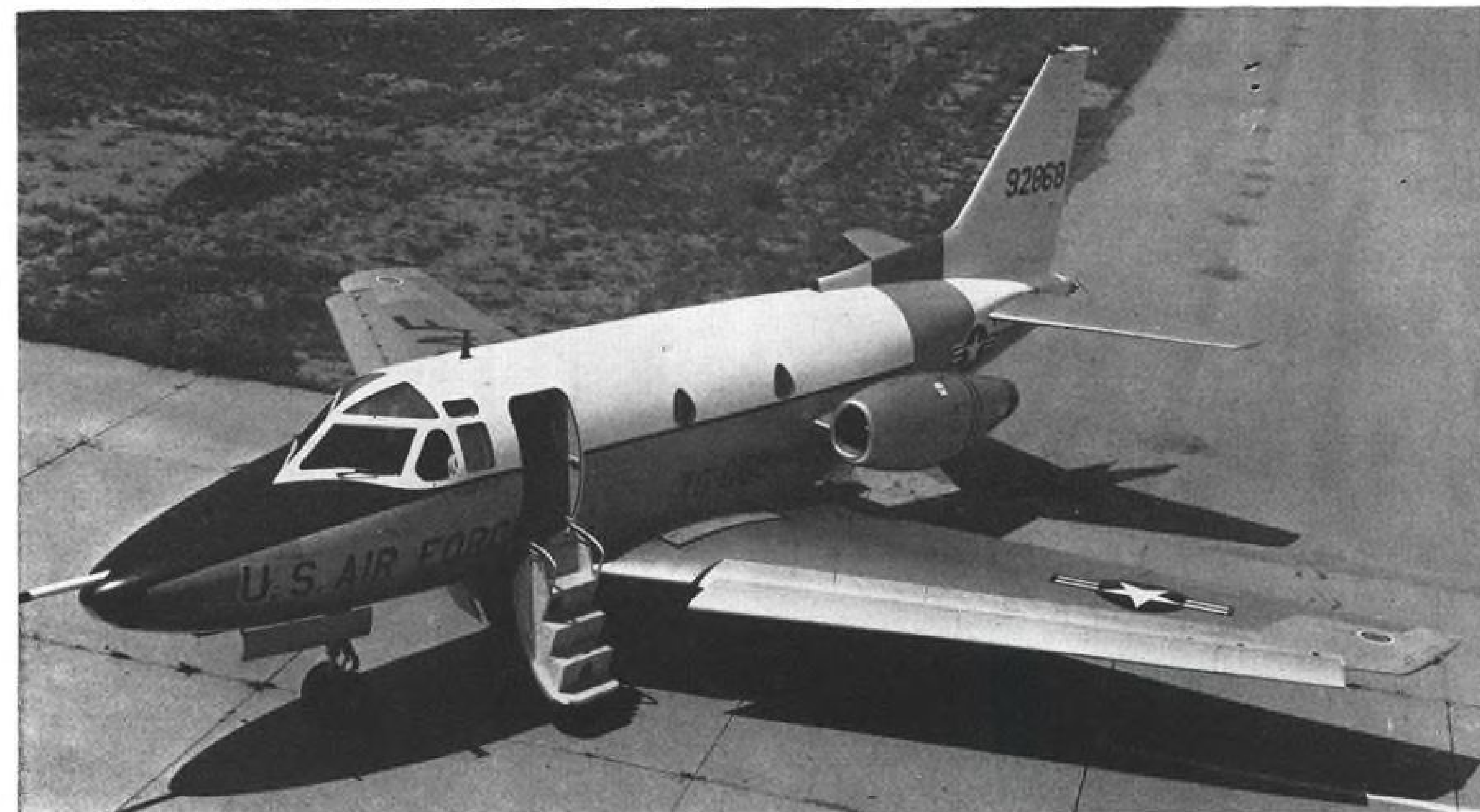
CURRENTLY being flown with four passenger seats, tests are under way to prove out installation of six passenger seats. Cabin maintains 8,000-ft. pressure altitude to 45,000 ft., and 8.8 psi. differential above that altitude. Teardrop-shaped windows limit passenger visibility.
