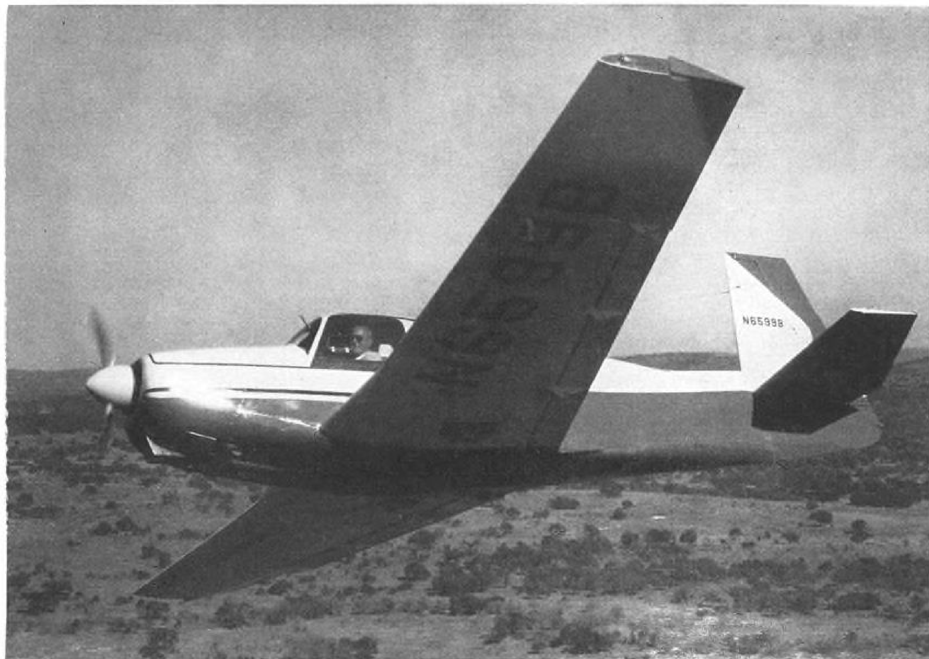
ALL-METAL Mooney Mark 21 is powered by a 180-hp. Lycoming O-360-A1A engine fitted with a McCauley constant speed propeller.
