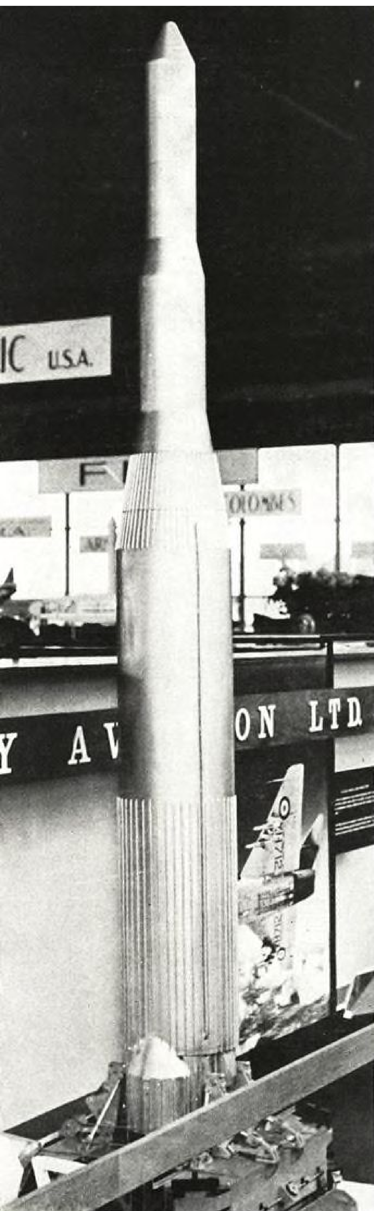
HAWKER-SIDDELEY model represents British space vehicle which would place a 2,000-lb. payload into a 300-mi. orbit. It envisions the use of the British Blue Streak IRBM as the first stage, the French Veronique as the second and an adaptation of the British Skylark research rocket as the third. A fourth stage could be added to obtain greater distances and/or heavier payloads.
