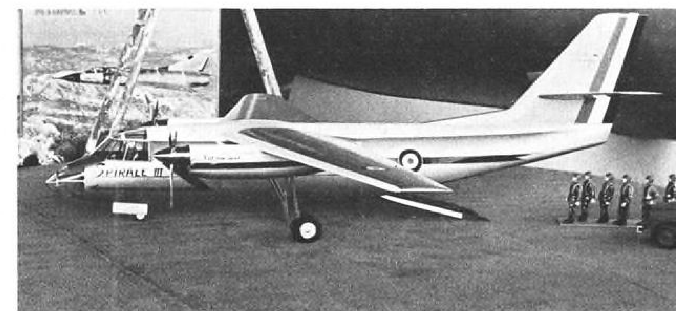
SPIRALE III , powered by two Turbomeca Turmo turboprop engines, is a military version of Dassault's Communaute transport (AW Apr. 24, p. 103). The military transport is designed for STOL operations in tropical areas. Model above shows hydraulically-operated rear ramp loading platform. The nose of the aircraft houses the observer's position. Spirale III will have a 3,300-lb. payload when operated over a 935-mi. stage length. As a medium-range cargo aircraft, the plane can be operated with a 7,700-lb. payload on 560-mi. route lengths or a 4,400-lb. payload over 740 mi.
