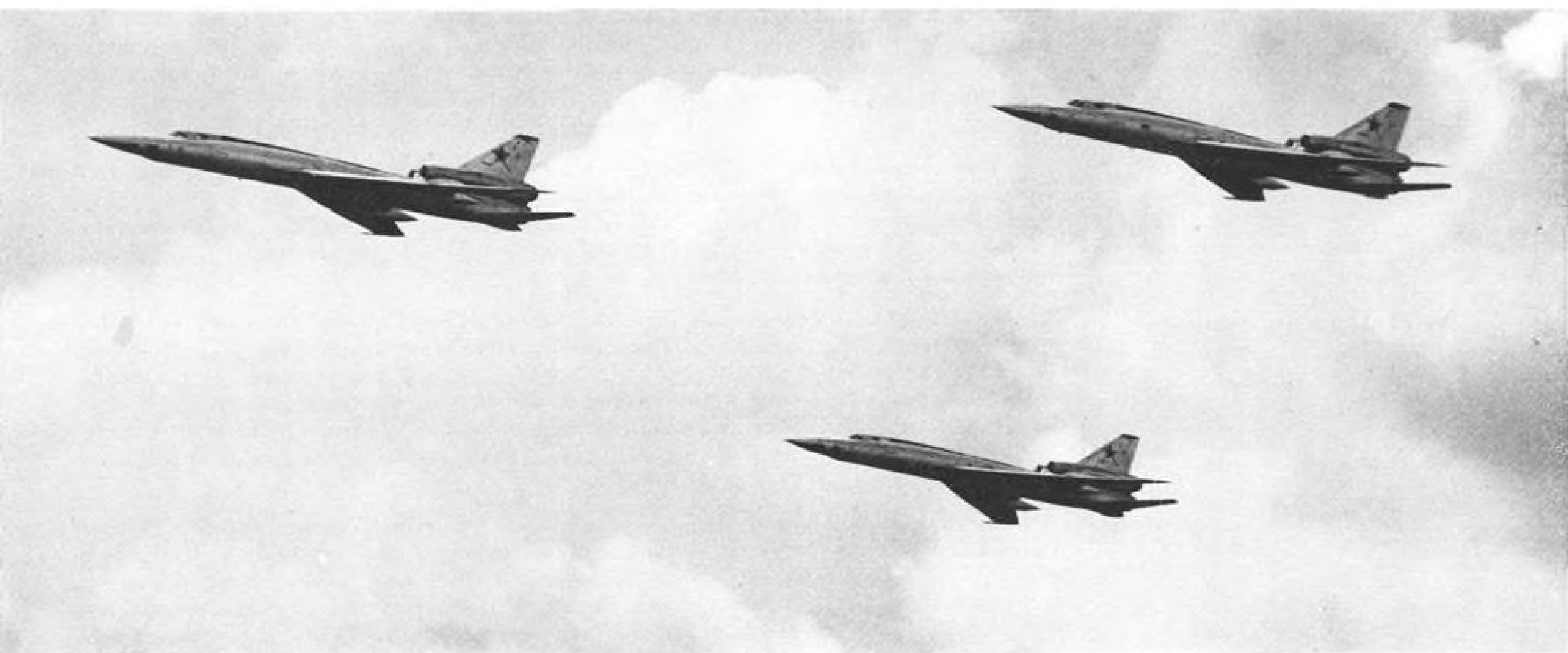
Formations of Beauty bombers indicate early operational status of this Mach 2-plus heavy bomber and reveal additional design details. Note bombing radar bulge under nose just below auxiliary air intakes. Tail radar and remotely operated turret are visible between engine tailpipe and tail fin. Highly swept thin wings house main landing gear in nacelles. Note dihedral on low set horizontal tail.
