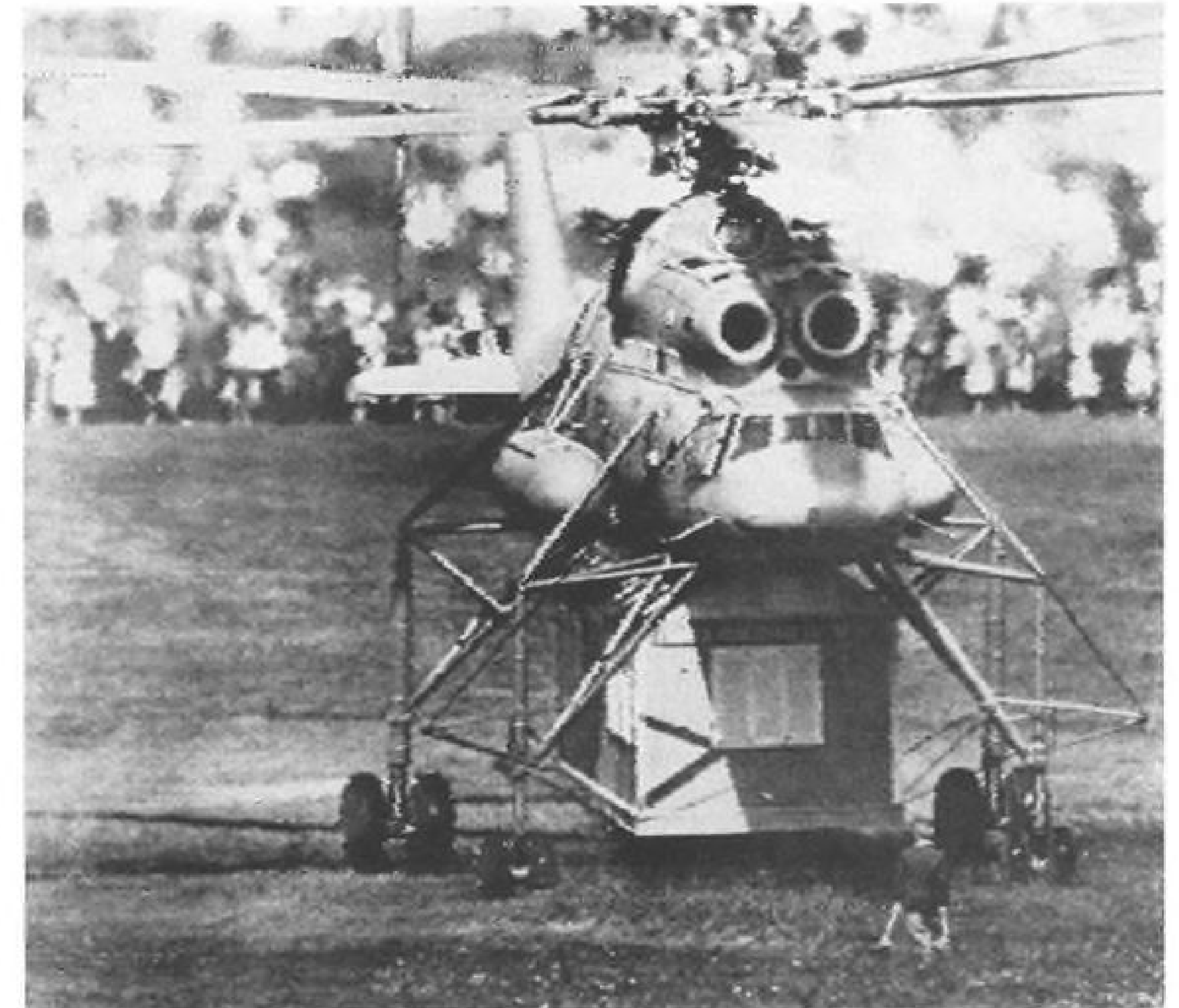
MIKHAIL MIL'S flying crane design demonstrates cargo capacity by lifting prefabricated house size of a U. S. railroad freight car. Note external fuel tanks along fuselage, one tailpipe of twin-jet powerplant installation and unusual cockpit configuration. Rotor system appears to be the same as Mil-6 but transport type cabin is of a smaller diameter.
