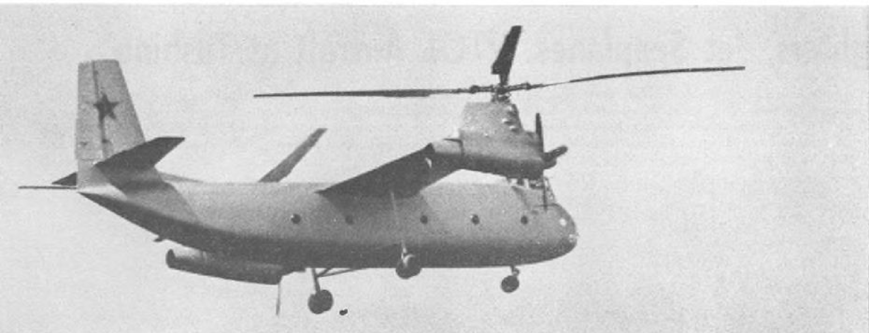
Hoop convertiplane shown above has twin rotor systems each about the size of Mil-4 rotor system and uses An-10 transport fuselage with 80-passenger capacity. Note conventional vertical tail and high-mounted wing. Powerplants are Ivchenko 4,000 eshp. turboprops, one housed in each wing tip pod, driving both rotor system and conventional propellers.
