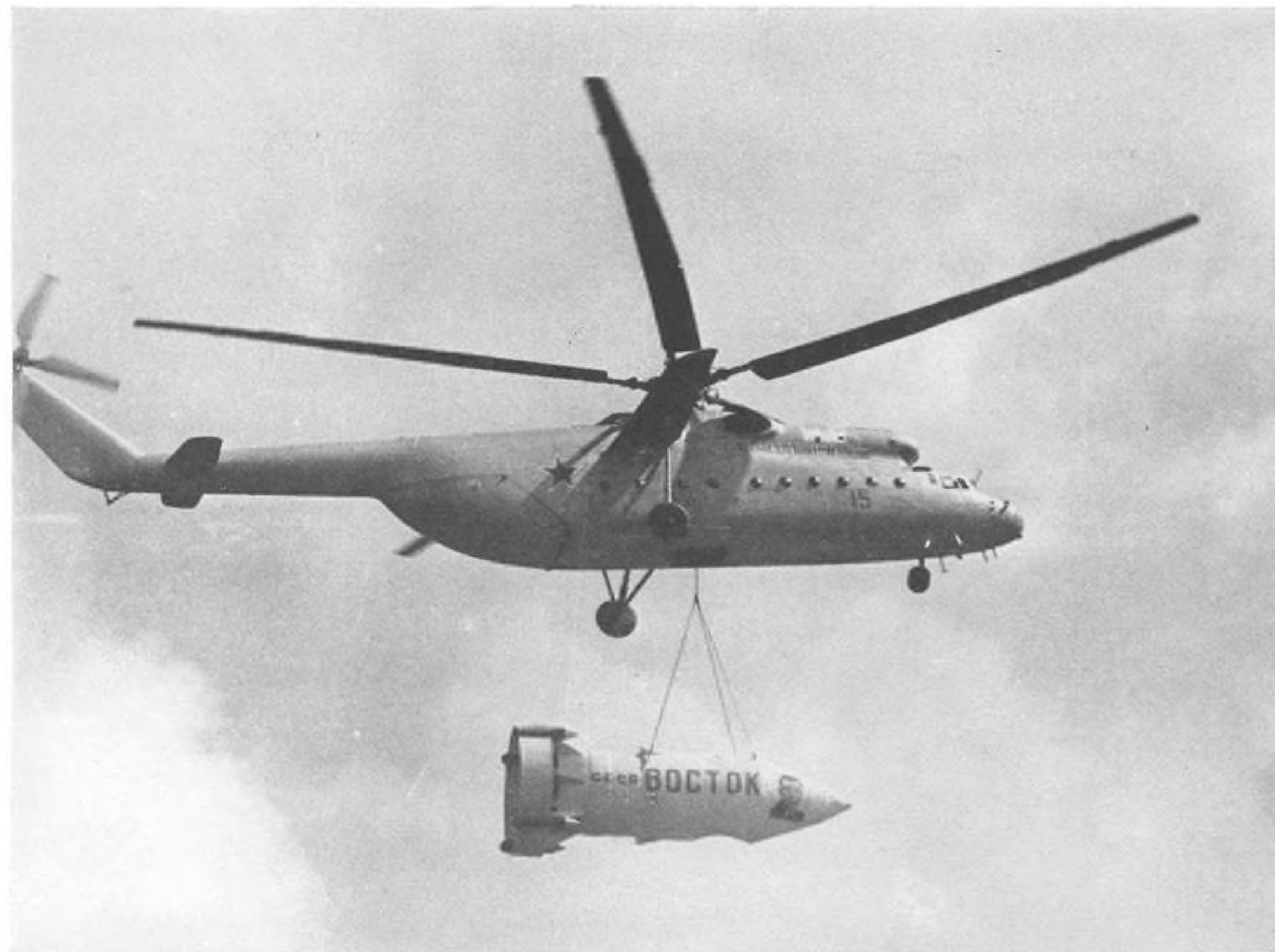
Mil-6 helicopter carries what Soviets said was Vostok space ship past crowd at Tushino. Labels say USSR and Vostok, carry picture of Yuri Gagarin on nose. Large radome is visible on capsule belly and four retrorocket housings are contained in stern circular housing. Other helicopters carried earlier Sputniks and space probes in flypast.
