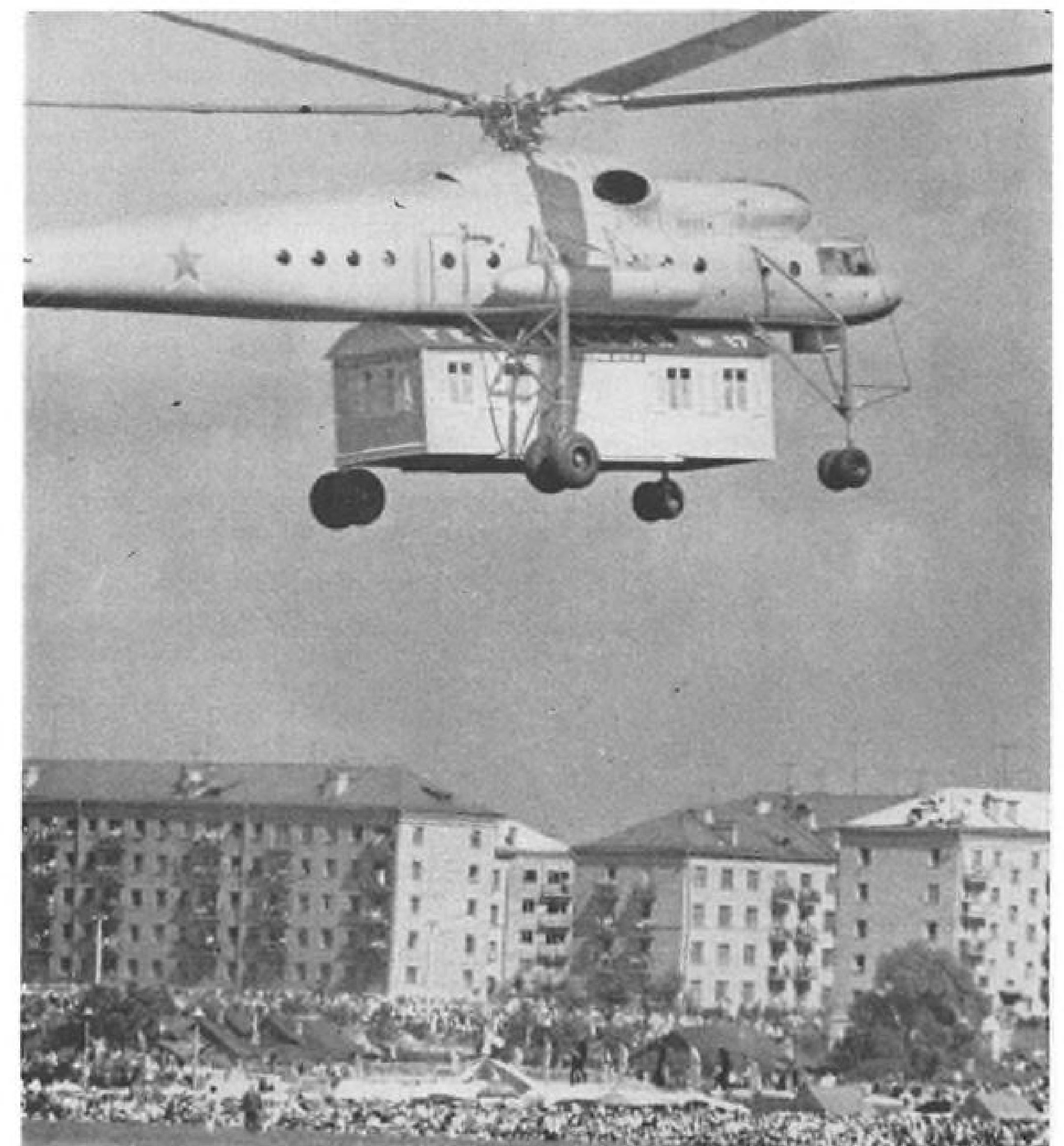
MIKHAIL MIL'S flying crane design demonstrates cargo capacity by lifting prefabricated house size of a U. S. railroad freight car. Note external fuel tanks along fuselage, one tailpipe of twin-jet powerplant installation and unusual cockpit configuration. Rotor system appears to be the same as Mil-6 but transport type cabin is of a smaller diameter.
