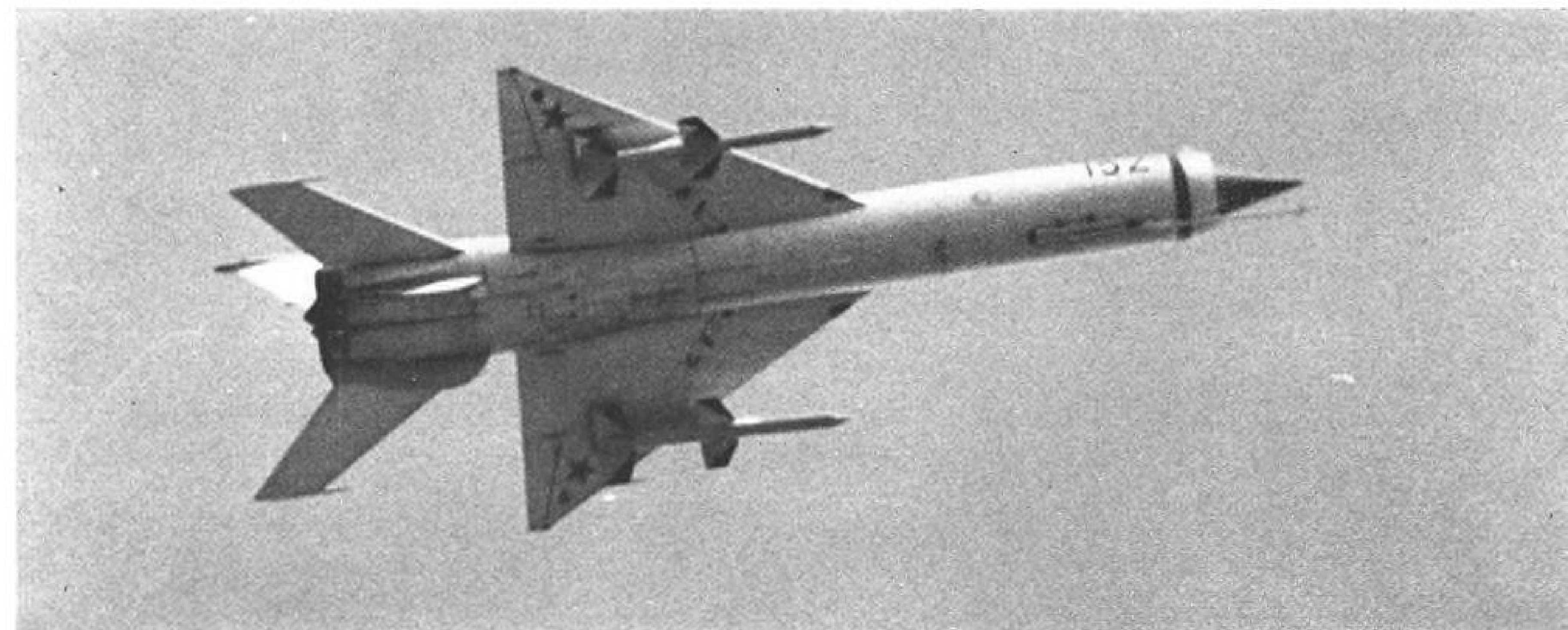
New Mikoyan Mach 2-plus long-range interceptor (below) has large airborne radar in conical nose air intake and carries two large air-to-air missiles. This is latest development of earlier Fishbed design aimed at countering USAF bomber threat.
