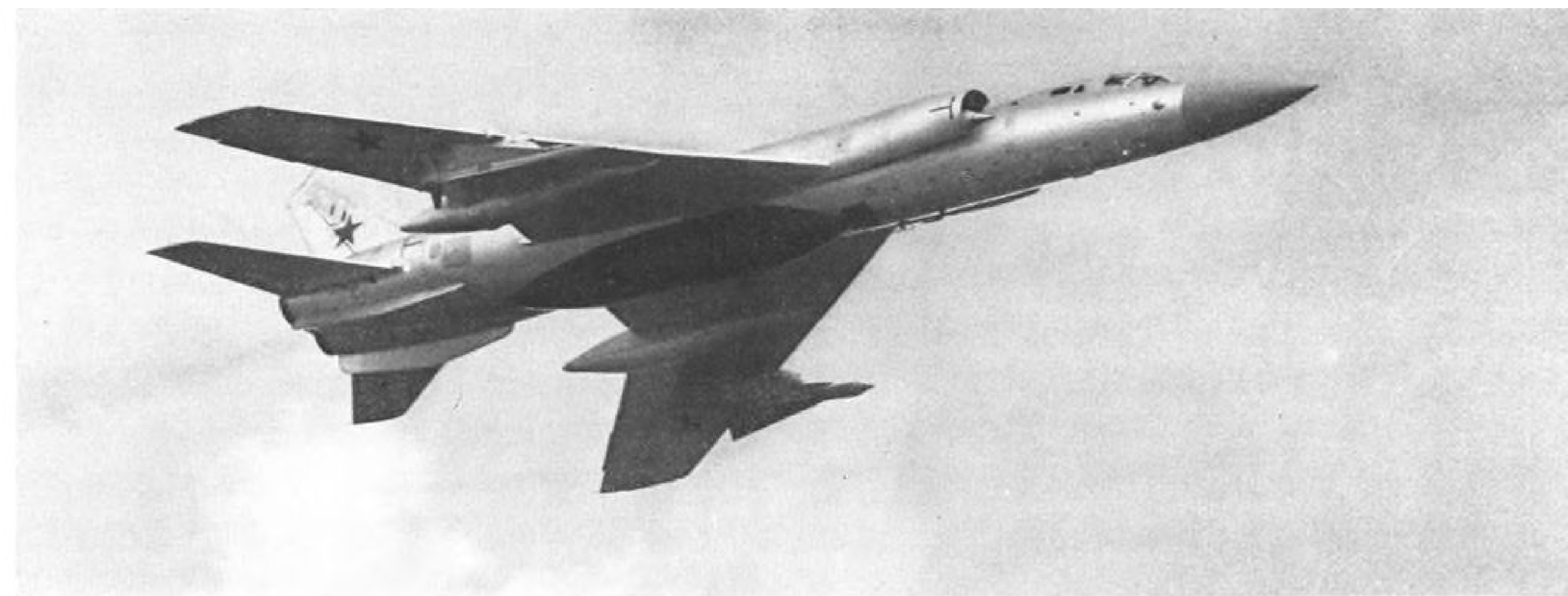
Two views of Yakovlev Blinder (above and below) indicate Mach 2-plus performance and dual role as long-range interceptor armed with missiles or as a bomber. Note shoulder-mounted twin-jet intakes merging into single bifurcated tailpipe, large airborne radar in nose and large auxiliary fuel tank under belly.
