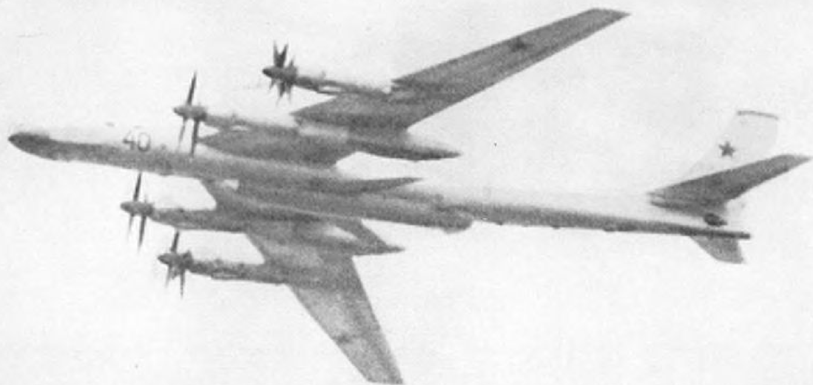
Bear turboprop intercontinental bomber is equipped with 300-mi. range air-to-ground guided missile slung under its specially modified belly. Note large radome nose on missile, swept wings, big fuselage denoting large nuclear weapon capacity, and large jet tailpipe. Bear nose radar has been modified for missile guidance.
