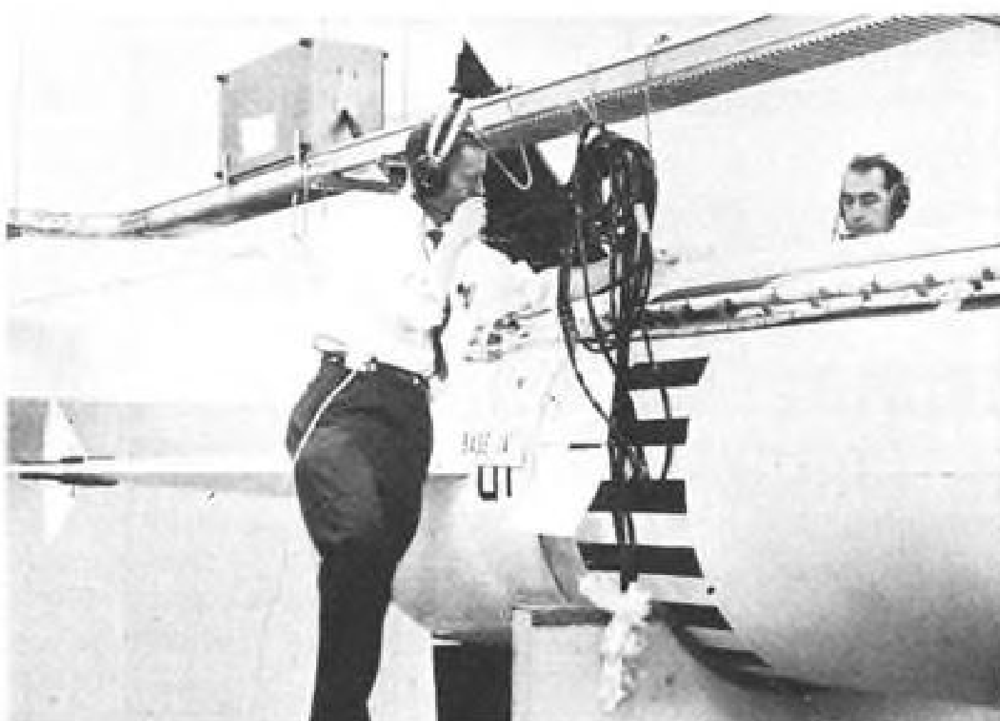
Electrical evaluator (above) checks ignition and destruct systems in Vought Astronautics Scout checkout. Procedure also includes assessment of control and guidance packages (below, left) and installation of wiring harness on first and second stages (below, right).
