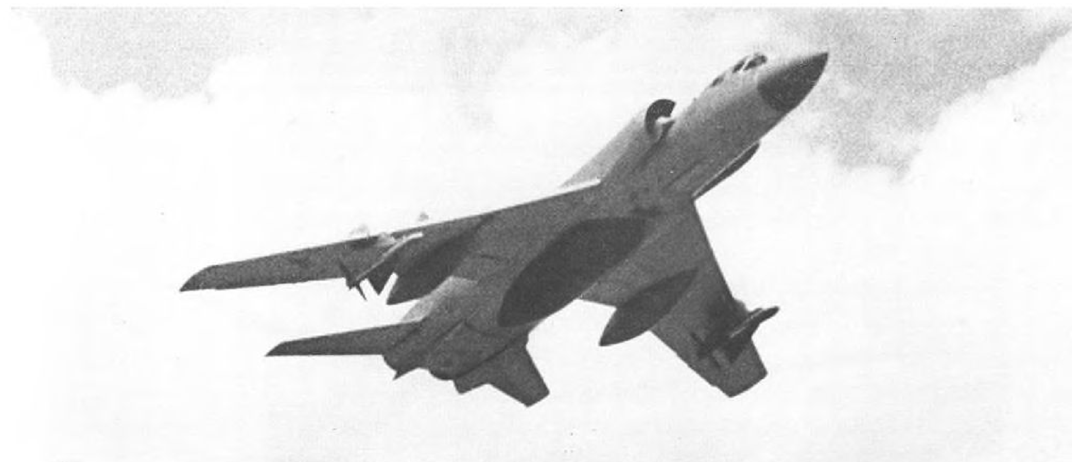
New Mikoyan Mach 2-plus long-range interceptor (below) has large airborne radar in conical nose air intake and carries two large air-to-air missiles. This is latest development of earlier Fishbed design aimed at countering USAF bomber threat.
