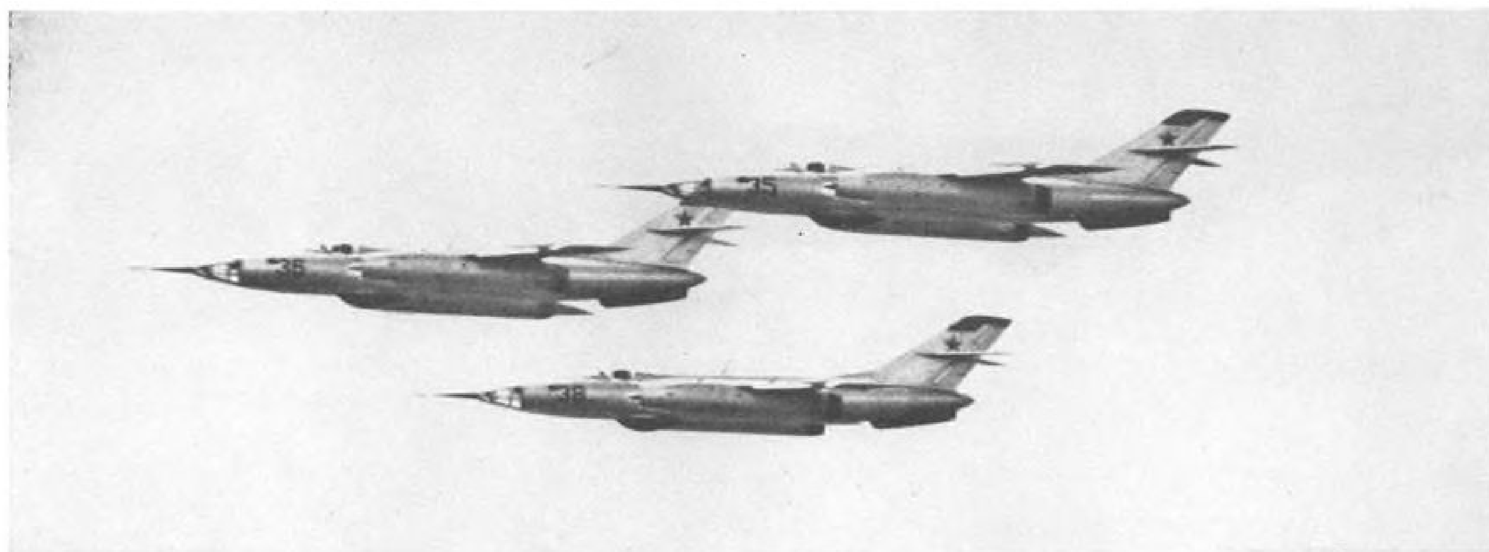
Two advanced versions of Yakovlev Flashlight series include the Model B (above) all-weather interceptor equipped with large airborne intercept radar in the nose, twin-jet engines with afterburners mounted under the swept wings and large air-to-air missile armament. Production version of Flashlight B shows many changes over the prototype first seen at Tushino in 1956. Attack version, Flashlight C, (below) appeared in squadron formations indicating the 1956 Tushino prototype went into production with modifications such as addition of ventral fin, bombing radar in belly and supersonic spiked engine inlets. Both versions of Flashlight shown are in Mach 1.2 class.
