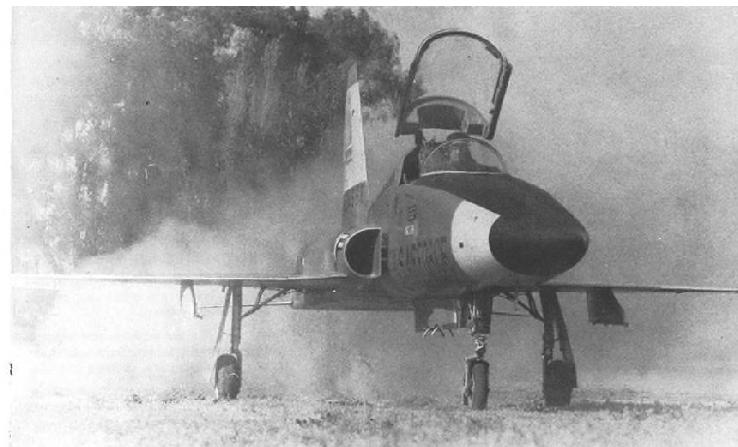
Northrop N-156, equipped with oversize, under-inflated tires, is run up for takeoff from semi-prepared sod runway at Culver City, Calif.
