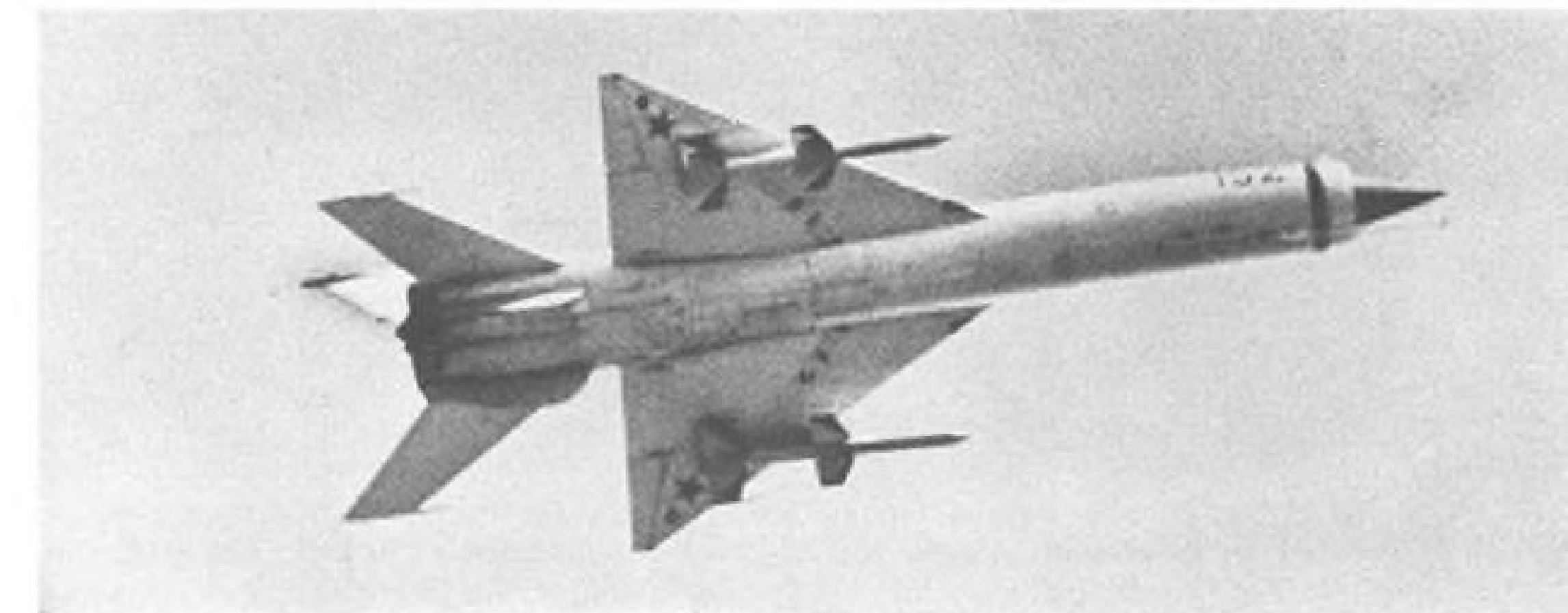
Both designs shown above differ from the new Mikoyan design shown here (AW July 10, p. 25 and July 17, p. 29) which carries another type missile and has two large turbojets with twin tailpipes and a rocket engine faired in between them at the tail.
