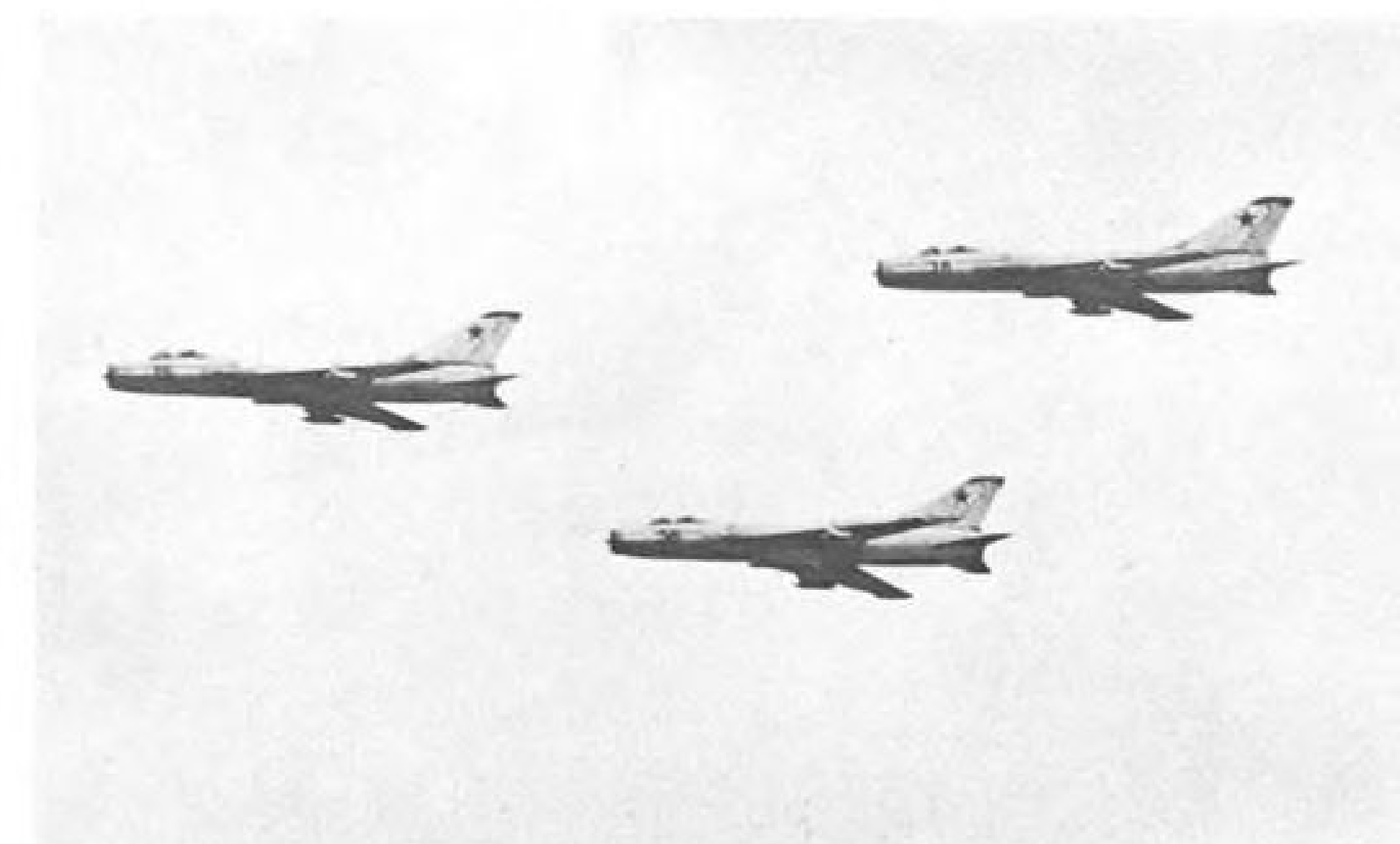
Two types of operational supersonic day fighters are shown over Tushino. Fishbeds (left) carry three Sidewinder-type missiles one under the belly and each wing. Sukhoi-designed Fitters (right) carry rocket-firing pods under each wing and belly fuel tank.
