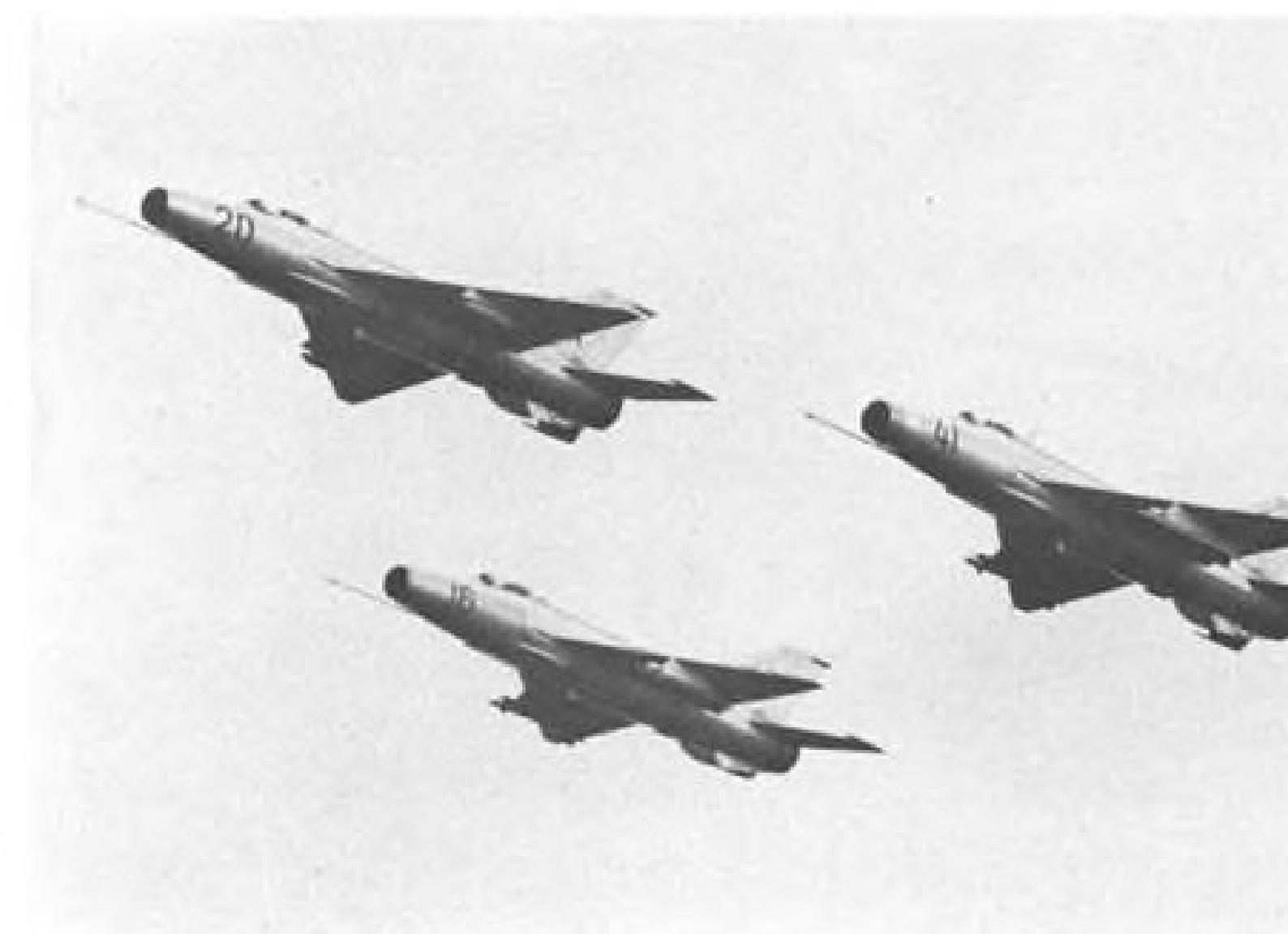
Two types of operational supersonic day fighters are shown over Tushino. Fishbeds (left) carry three Sidewinder-type missiles one under the belly and each wing. Sukhoi-designed Fitters (right) carry rocket-firing pods under each wing and belly fuel tank.
