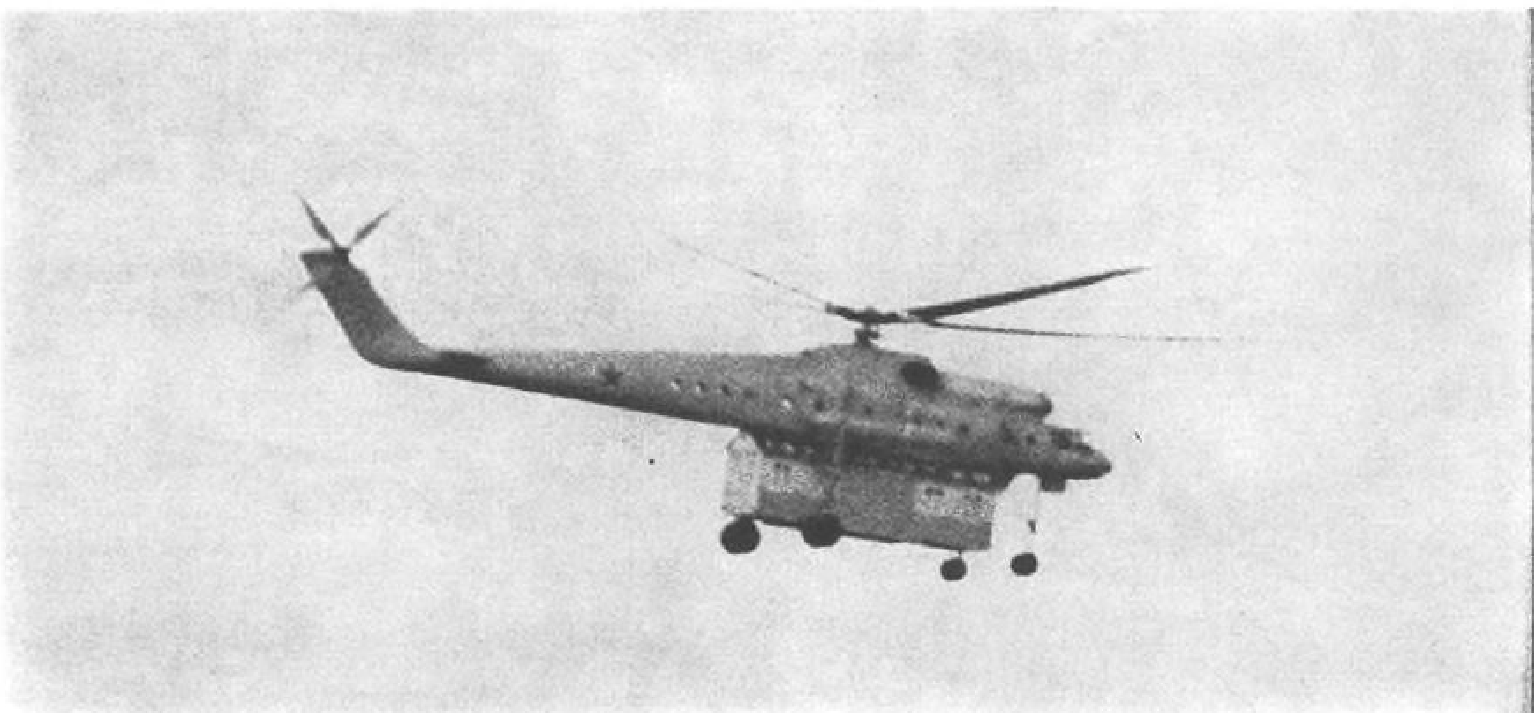
Mil Flying Crane, in flight at Tushino lifting a freight-car sized house, is derived from the Mi-6 but has a larger rotor hub and longer blades needed for its mission. Cockpit visibility has been increased with larger and more numerous windows and fuselage appears longer than the Mi-6. Circular extension below cabin just ahead of the front landing gear is probably a telescoping compartment for a crewman to provide aft viewing for cargo handling. This permits either forward or aft removal of loads.
