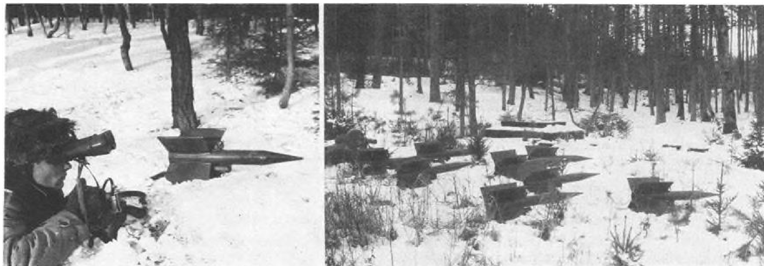
BATTERY OF EIGHT Cobra wire-guided, anti-tank missiles may be launched and controlled by a single infantryman. In combat, missiles (right) would be more widely dispersed. Controller (left) follows flight of the missile through binoculars mounted on control box. Control stick in his right hand guides missile to target.
