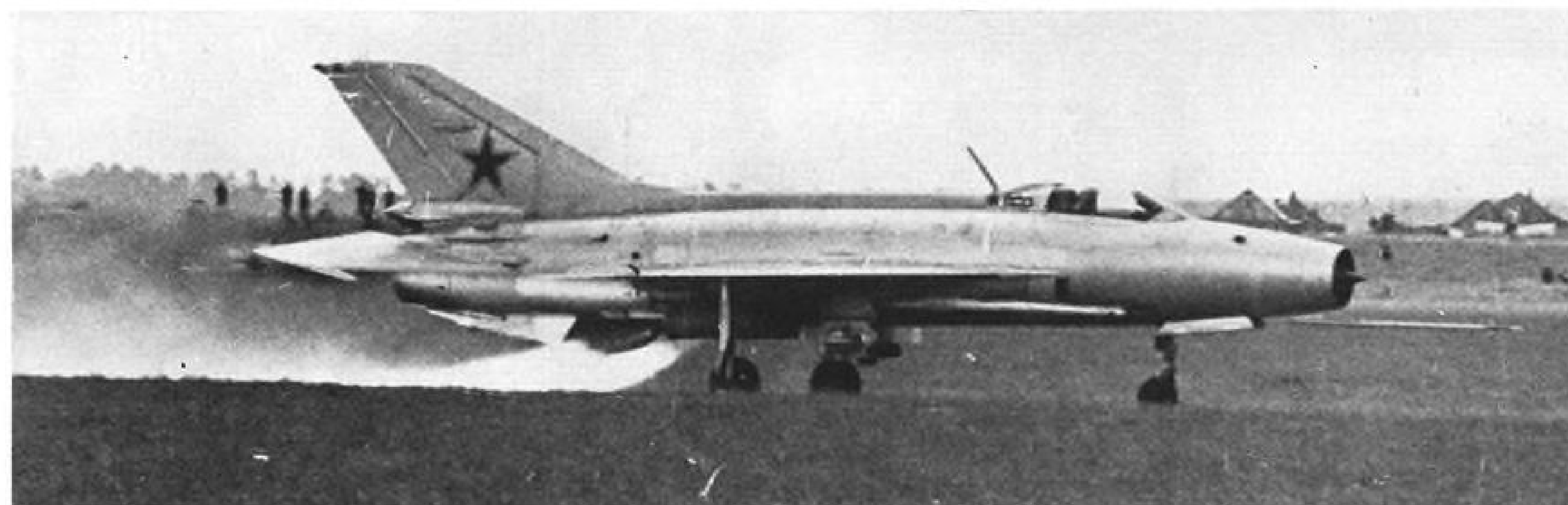
Rocket booster used for takeoff from sod field by Mikoyan Fishbed (below) appears to be a shorter unit than one demonstrated at Tushino (above, right). Flame pattern (below) suggests use of two small units instead of single large one at Tushino (AW July 17, p. 27).
