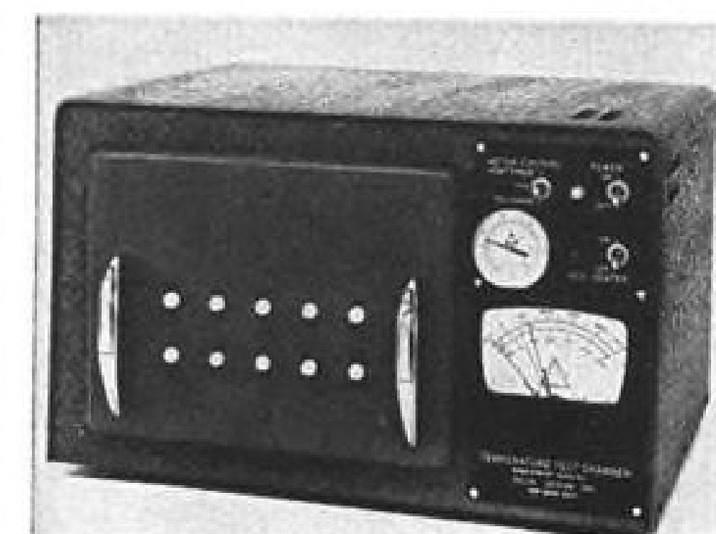
• Portable temperature chamber, Model 1060F, for rapid temperature cycling has a test chamber measuring 10 x 7 x 7 in. Temperature can be cycled from -100F to 500 F in less than 12 min. with temperature control accurate to within 1/2 deg. F. At -65F temperature, device consumes less than 3 1/2 lb. of carbon dioxide per hour. Test chamber weighs 40 lb. Manufacturer: Delta Design, Inc., 3163 Adams Ave., San Diego 16, Calif.
