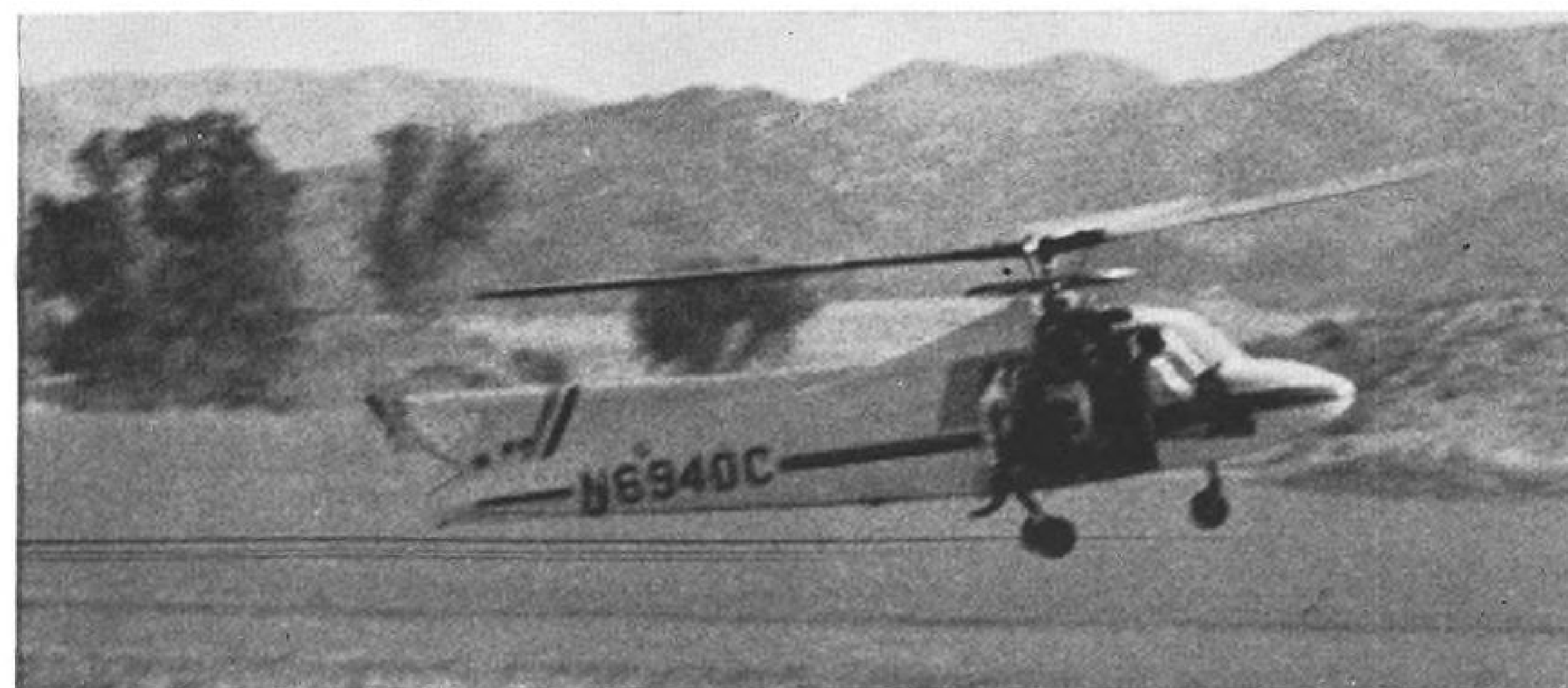
RING between rotor and fuselage top has three arms extending to each of the rotor blades and rotates with rotor.
