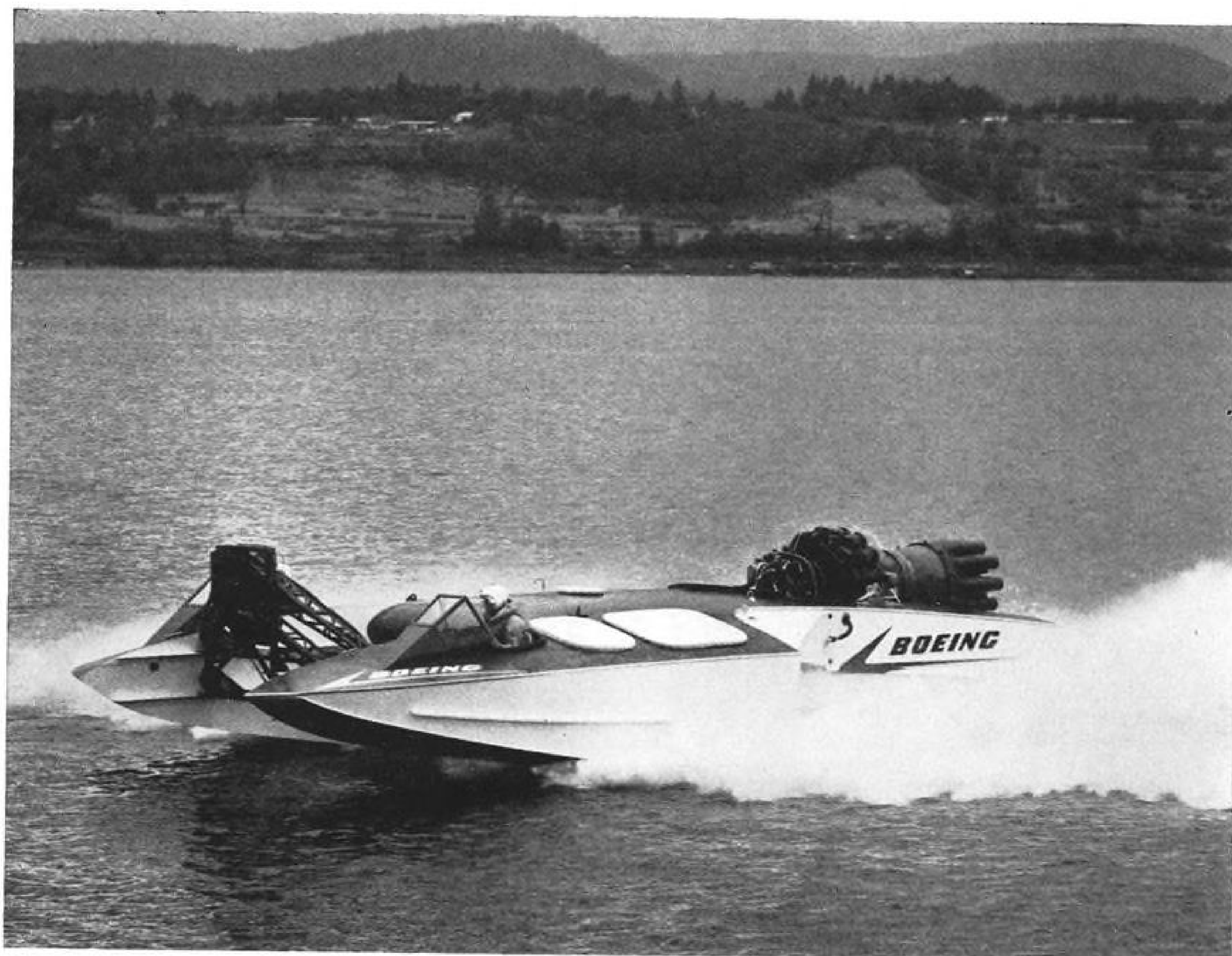
JET TEST BOAT. Boeing jet-powered research hydroplane, capable of speeds up to 100 knots, is newest addition to Boeing equipment devoted to advancing man's knowledge. Aqua-Jet will be used to test experimental hydrofoil designs. Test model is
