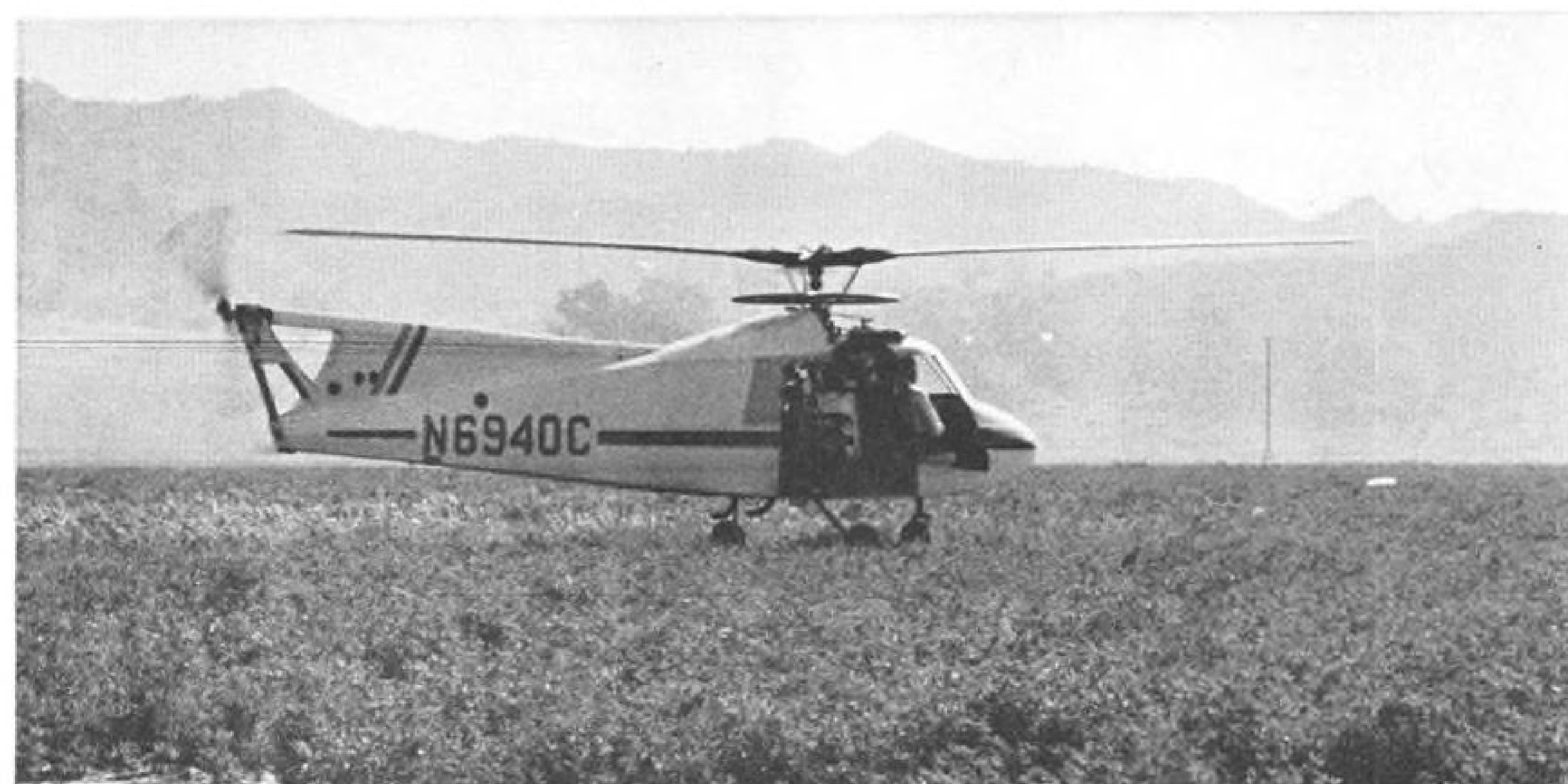
RING between rotor and fuselage top has three arms extending to each of the rotor blades and rotates with rotor.
