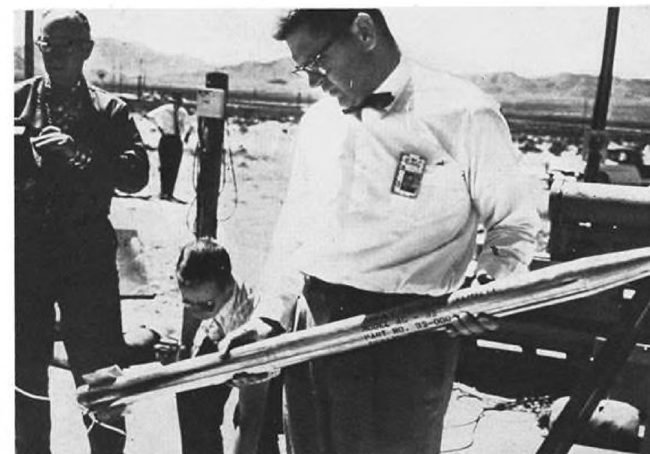
RAMJET-POWERED AG-32 meteorological sounding rocket is produced by Anderson, Greenwood & Co. Left photo shows rocket booster.
