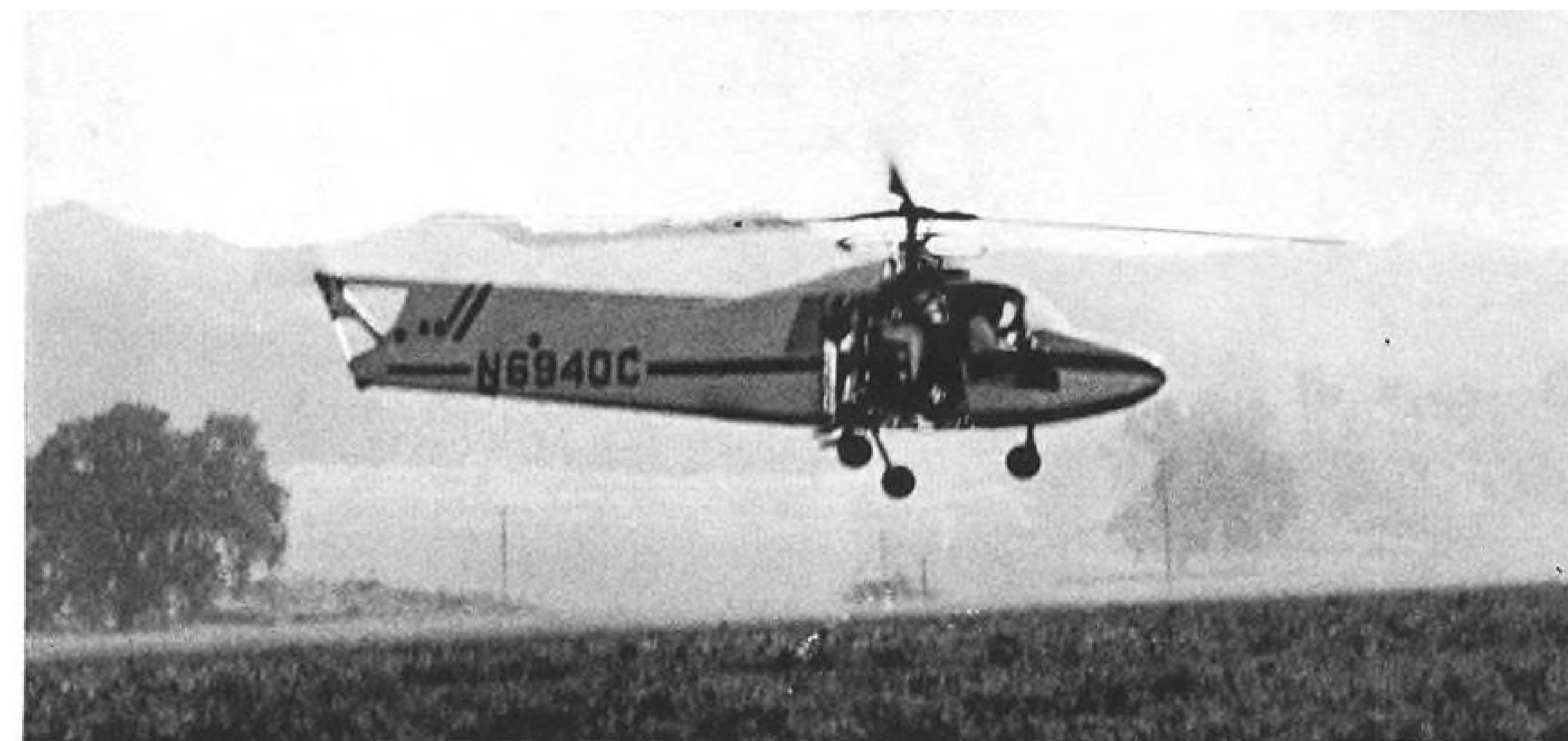
TAIL ROTOR is protected from ground contact by deep aft fuselage structure. Helicopter has two side-by-side seats.
