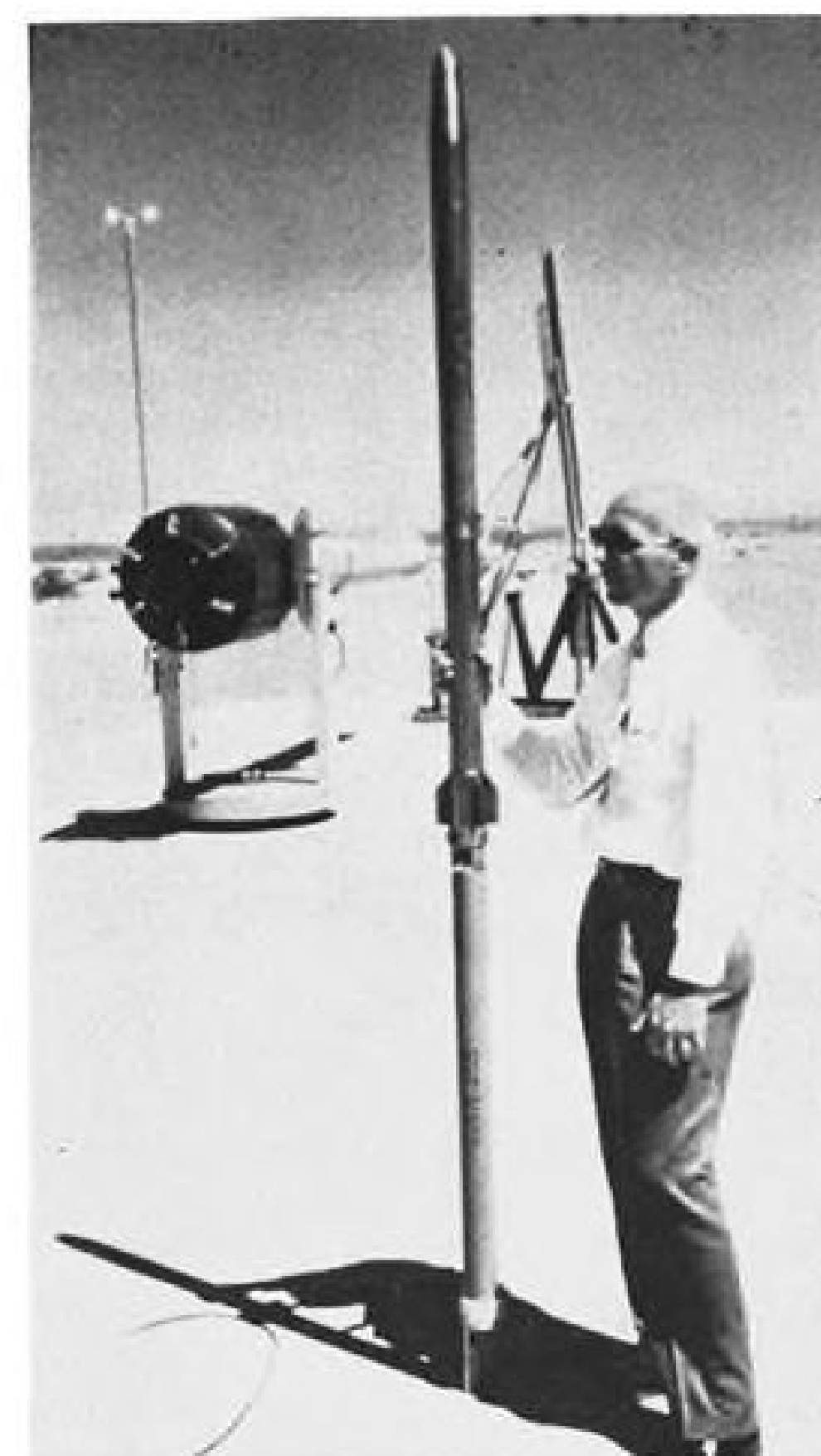
RAMJET-POWERED AG-32 meteorological sounding rocket is produced by Anderson, Greenwood & Co. Left photo shows rocket booster.
