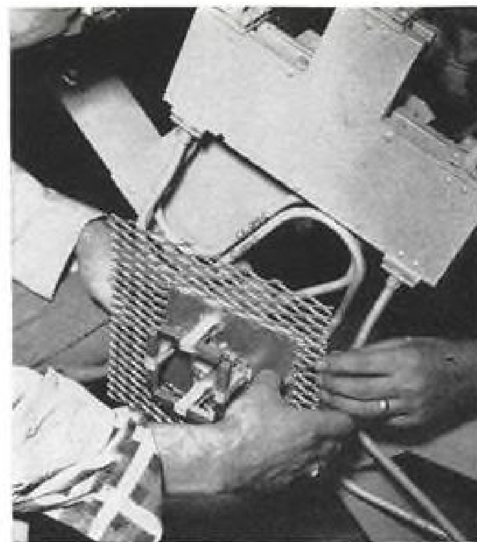
Individual unit assembly is first step in construction of antenna. Here four dipole antennas mounted on ground screen are being connected to one end of Foamflex feed lines. Special Phelps Dodge connectors are used to link the lines to the dipoles and four-way power dividers.
