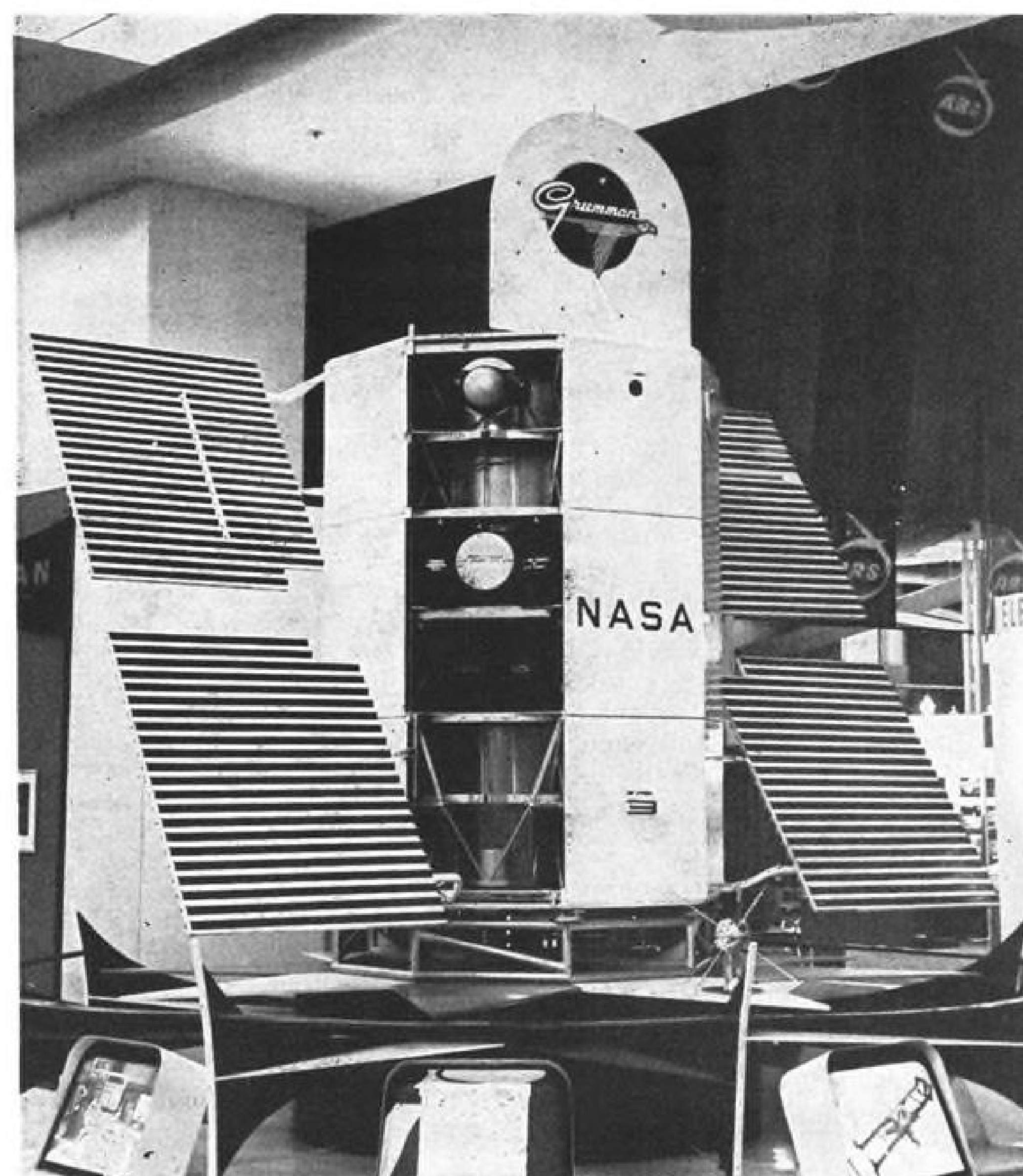
Grumman OAO (Orbiting Astronomical Observatory) is shown in first full-size representation of the design. Huge paddles are solar cell arrays for power collection.
