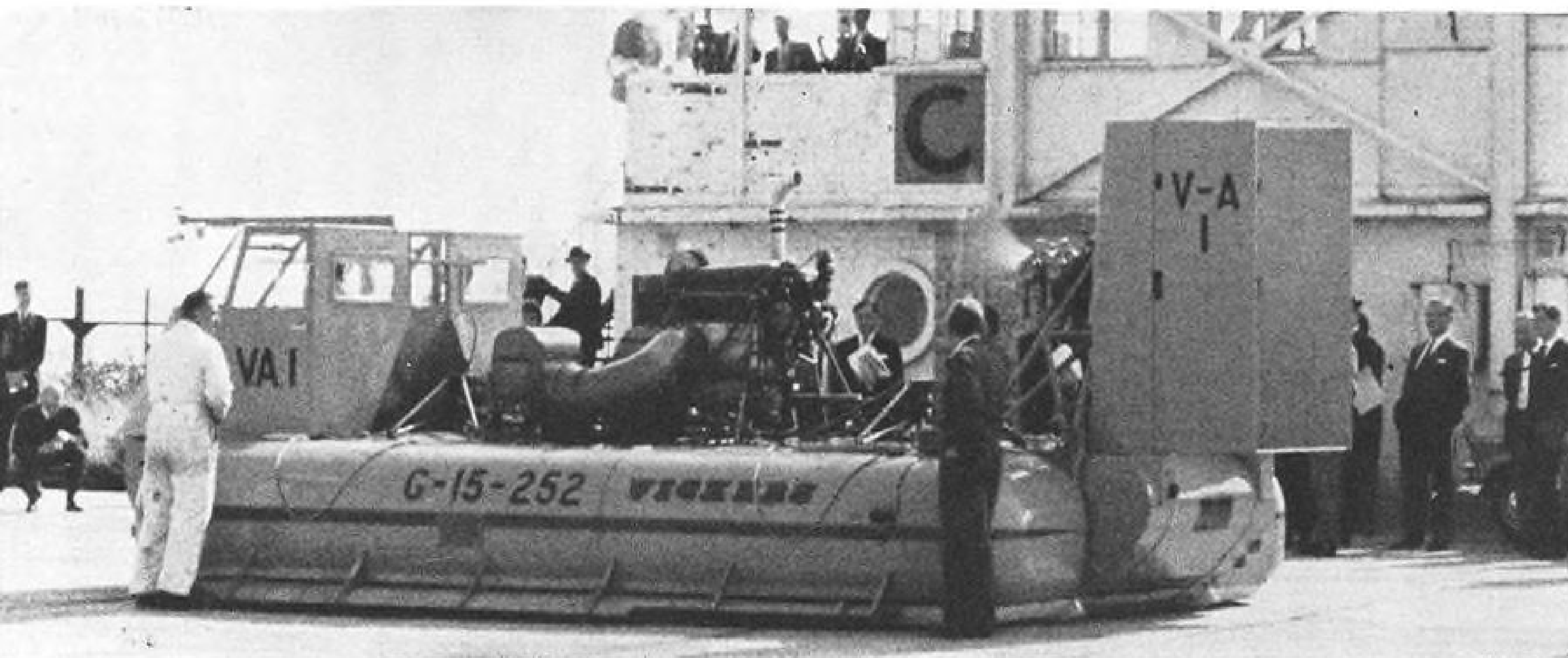
VICKERS-ARMSTRONGS VA-1 hovercraft research vehicle readied for demonstration run. Control problems at 30-kt. are being analyzed.
