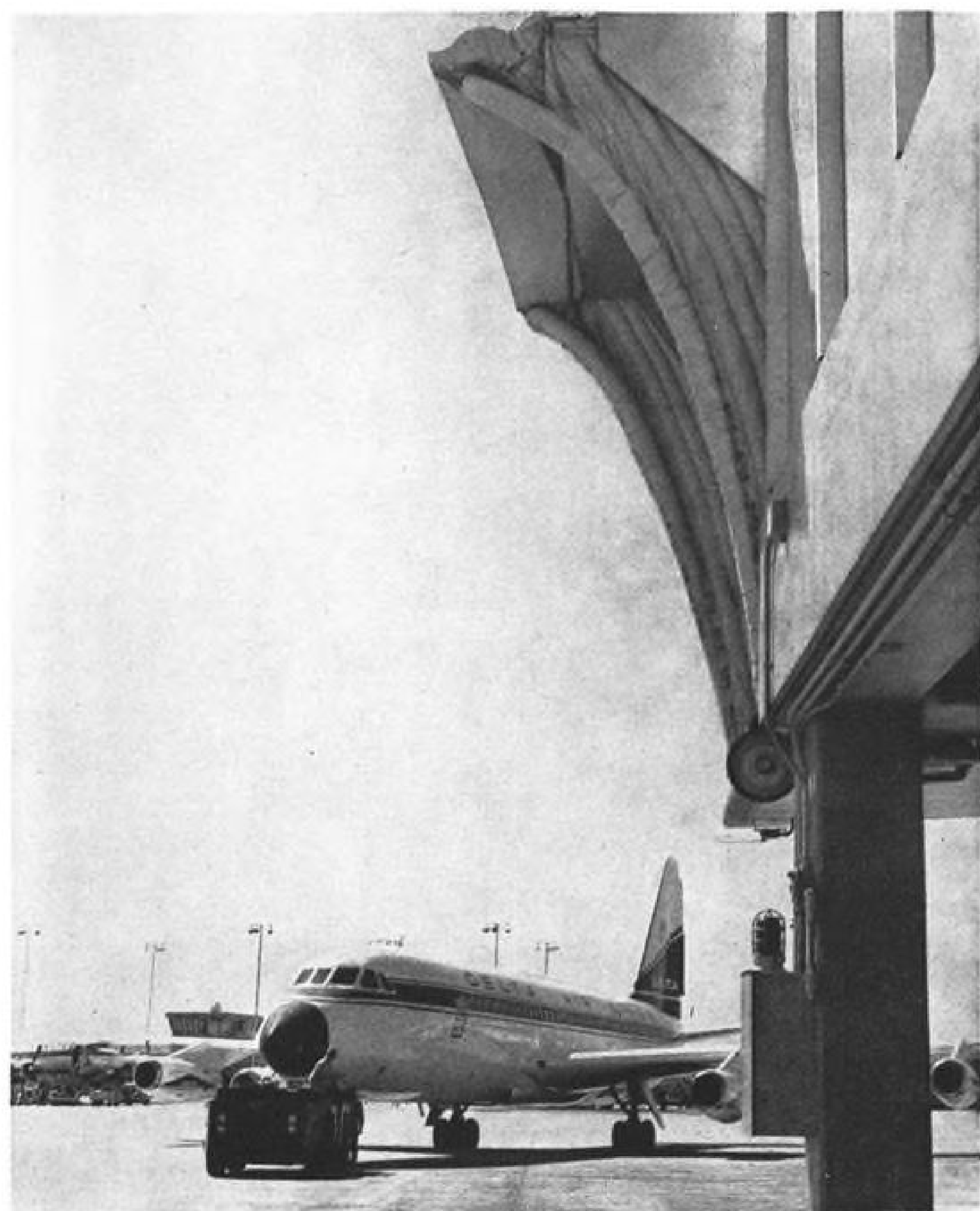
CONVAIR 880 is pushed out for departure at Atlanta. Delta's "jetway" covered loading bridge, above, is now at Atlanta, Idlewild and Miami, will be installed at other stations.
