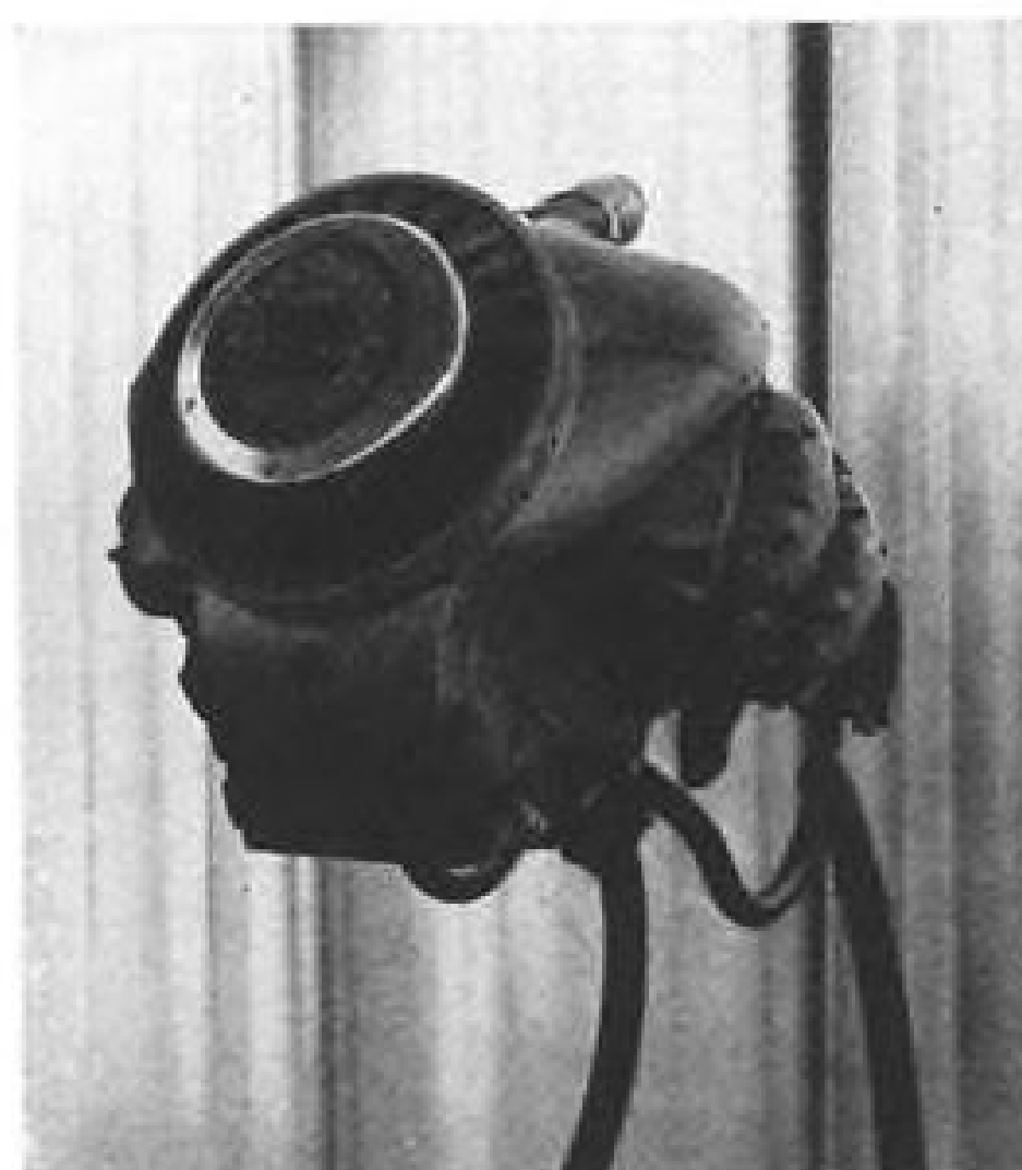
NEW FOUR-STROKE air-cooled engine, designated the M 110 H, suitable as a powerplant for both fixed-wing and small rotary-wing aircraft and for other industrial uses, was displayed at Brno for the first time. Engine has a dry weight of about 202 lb. When adapted as a helicopter powerplant, the complete unit weighs 277 lb.
