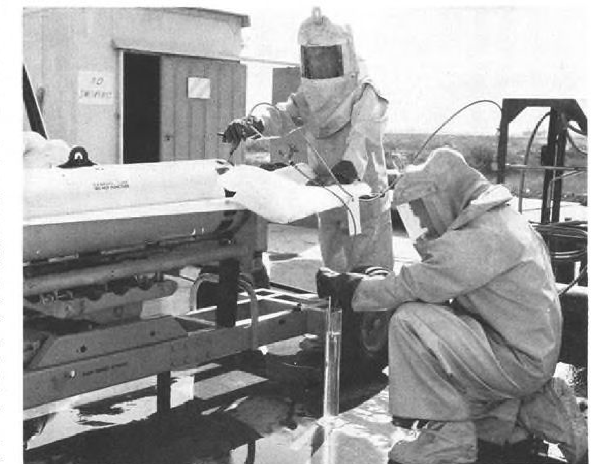
TARGET'S ROCKET ENGINES , above, are easily accessible. Below, crewmen fuel target at Pt. Mugu, where contract flight program was conducted.
