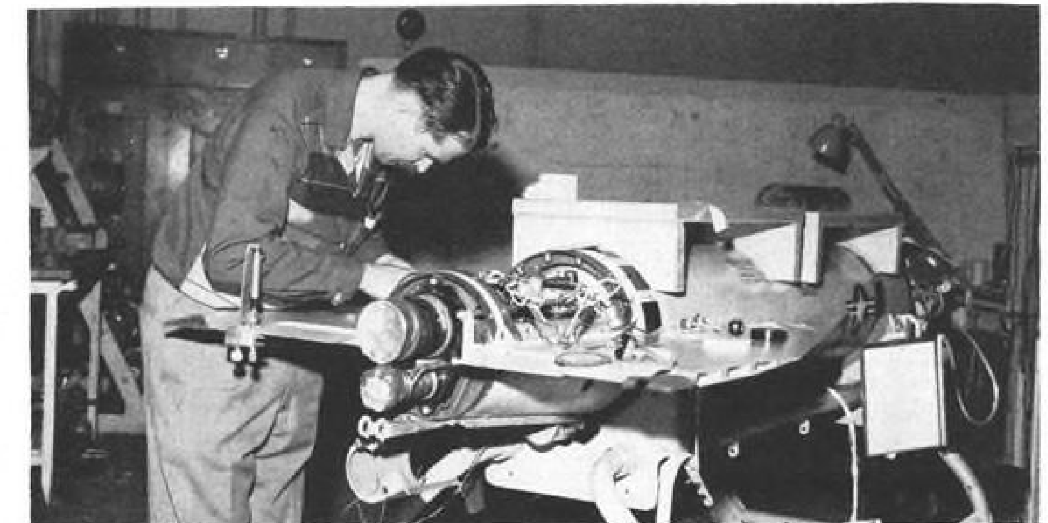
TARGET'S ROCKET ENGINES , above, are easily accessible. Below, crewmen fuel target at Pt. Mugu, where contract flight program was conducted.
