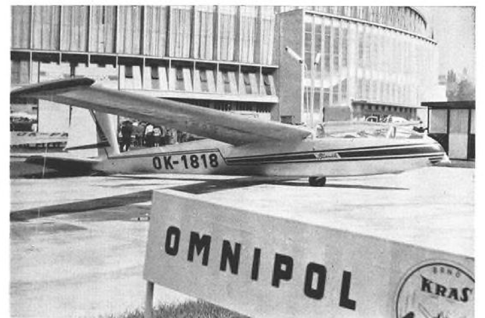
ALL-METAL two-seat tandem L-13 Blanik sailplane is being marketed in tropical countries where the normal plywood construction used in such aircraft does not withstand the extreme temperatures as well as metal. Of the 300 Blaniks built, Russia has received 200.
