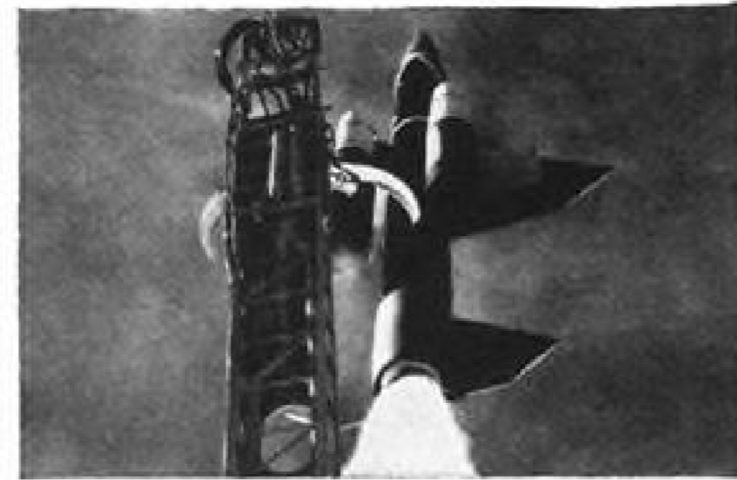
AUTOMATIC SKY FIGHTER. Supersonic Boeing Bomarc missile, now operational, is the United States Air Force's push-button defense weapon against airborne missiles and attacking bombers. New Bomarc "B" models have scored test intercepts up to 446 miles from base at altitudes of more than 100,000 feet.
