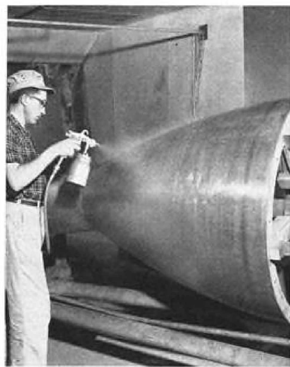
Silicone base aluminum paint, which provides surface protection up to 1700 deg. F., is sprayed on rocket engine jig at Rocketdyne plant of North American Aviation. The paint, known as CI "Extra High," is made by Chem Industrial Co., Cleveland, O., and is based on silicone resins made by Union Carbide.
