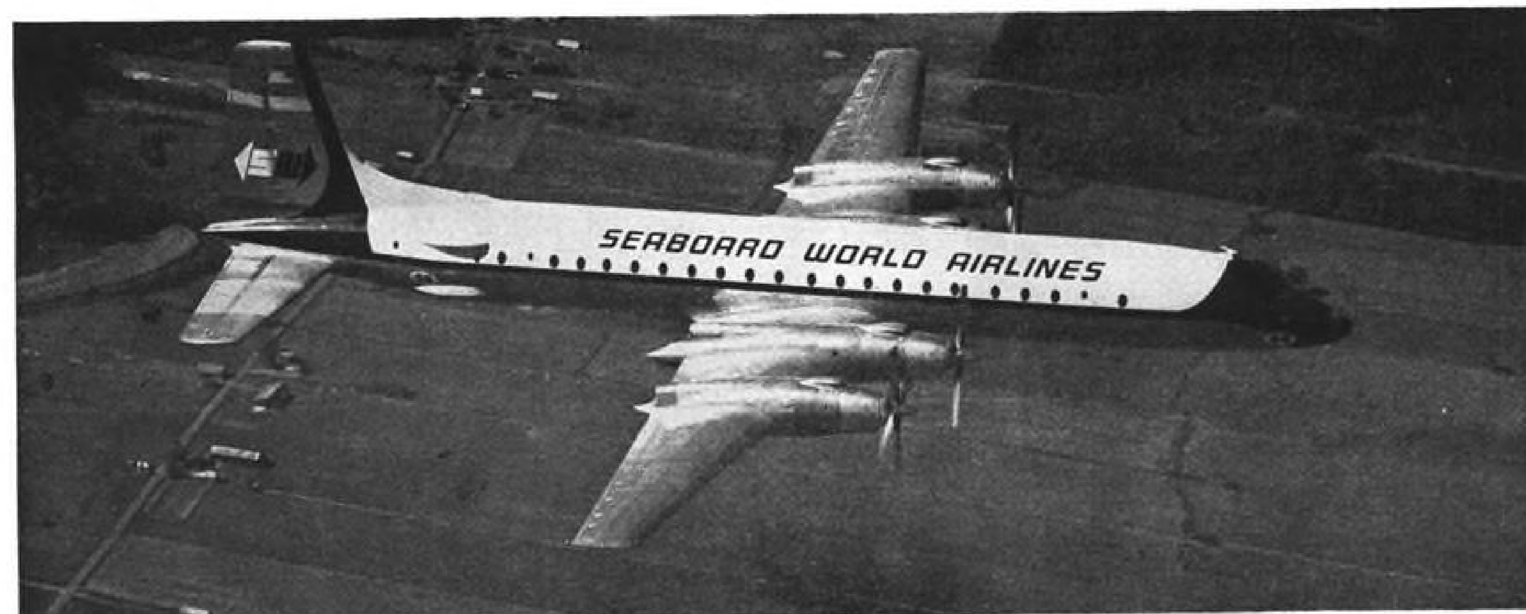
CL-44D IS POWERED by four Rolls-Royce Tynce engines. Bulges forward of horizontal stabilizer house hinges for swing tail.
