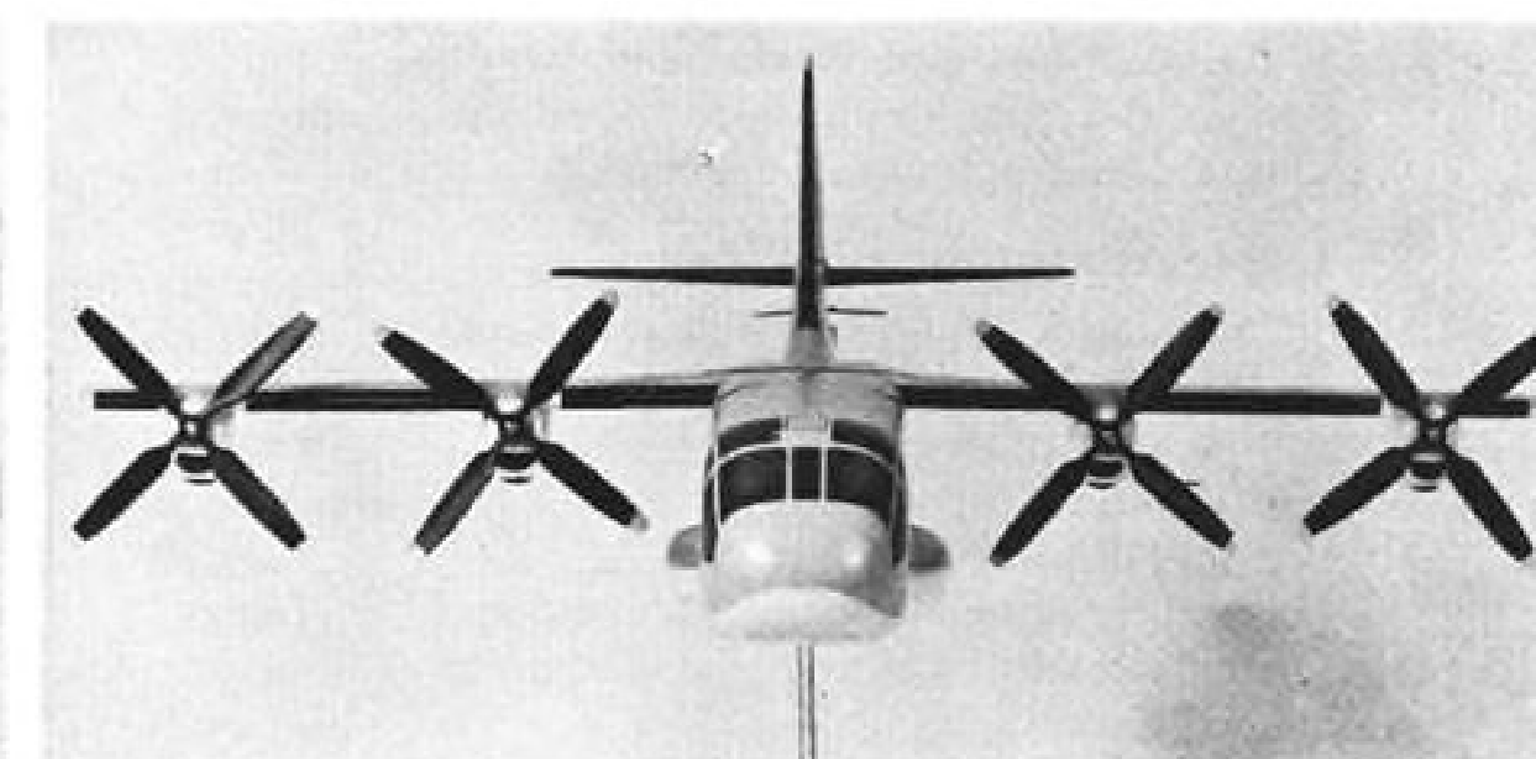
General Electric T64-GE-6s are mounted below wing to reduce need for wing structural cutouts and cross-geared for engine-out safety.
