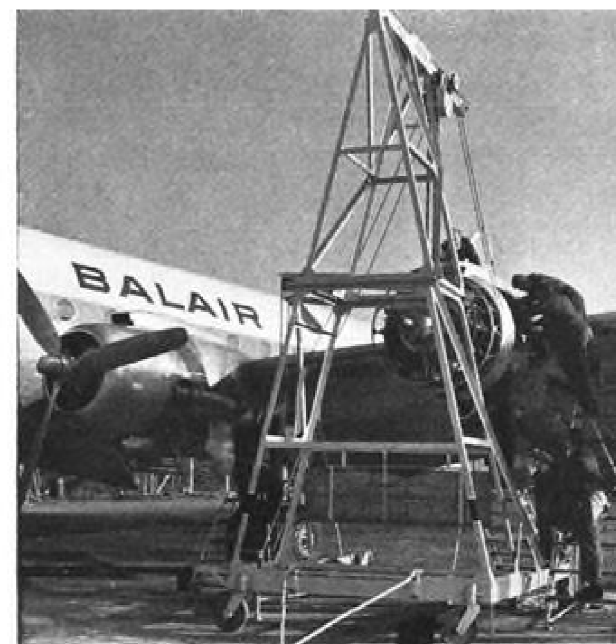
LOCAL MAINTENANCE and overhaul of Balair DC-4s up to 5,000 hr. is done locally. At left, DC-4 engine is changed after 1,500 flight hours. At right, DC-4 undergoes airframe check after 300 flight hours.
