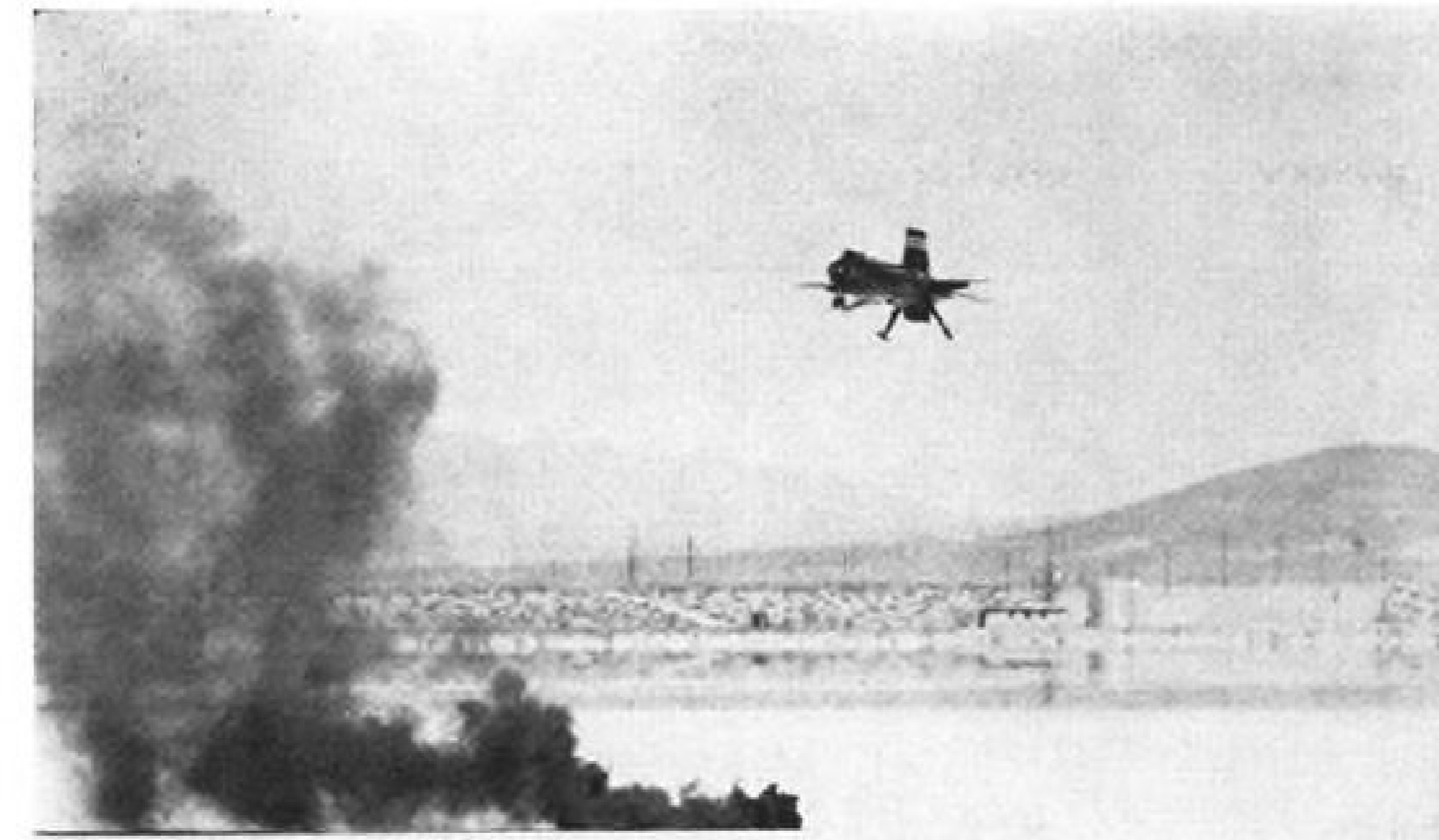
SERIES OF PHOTOS, taken with a Hulcher automatic camera with telescopic lens, shows the X-15 landing on the north lake bed at Edwards AFB. In left photo, the X-15 is completing flareout. Ventral fin already has been jettisoned and the gear extended. Smoke flare is an aid to the pilot in determining wind direction and velocity. Photo at right shows wing flaps extended.
