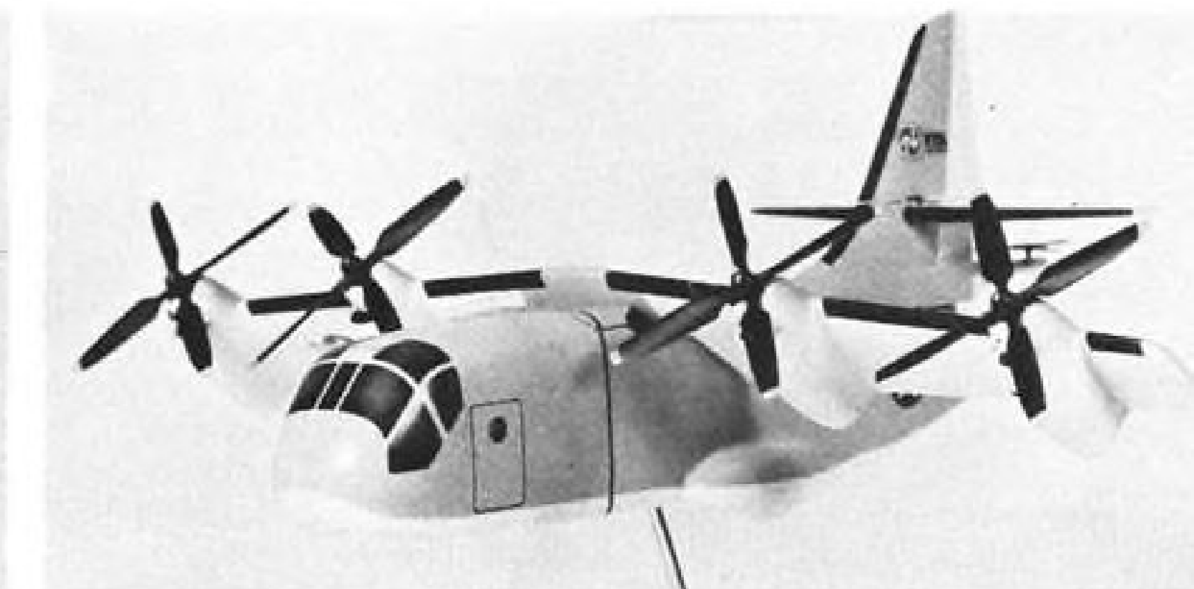
Wing of tri-service VTOL transport will be 67 ft. 6 in. long and will rotate through 100 deg. for vertical takeoffs (AW Sept. 25, p. 352).
