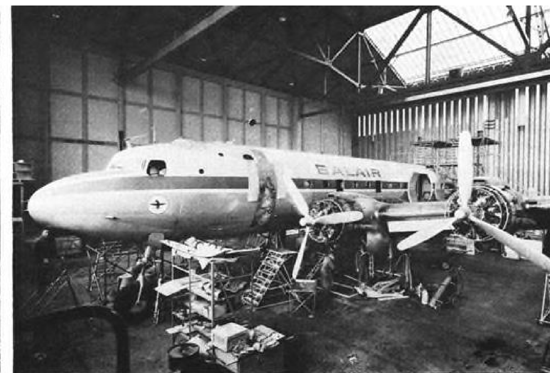
LOCAL MAINTENANCE and overhaul of Balair DC-4s up to 5,000 hr. is done locally. At left, DC-4 engine is changed after 1,500 flight hours. At right, DC-4 undergoes airframe check after 300 flight hours.
