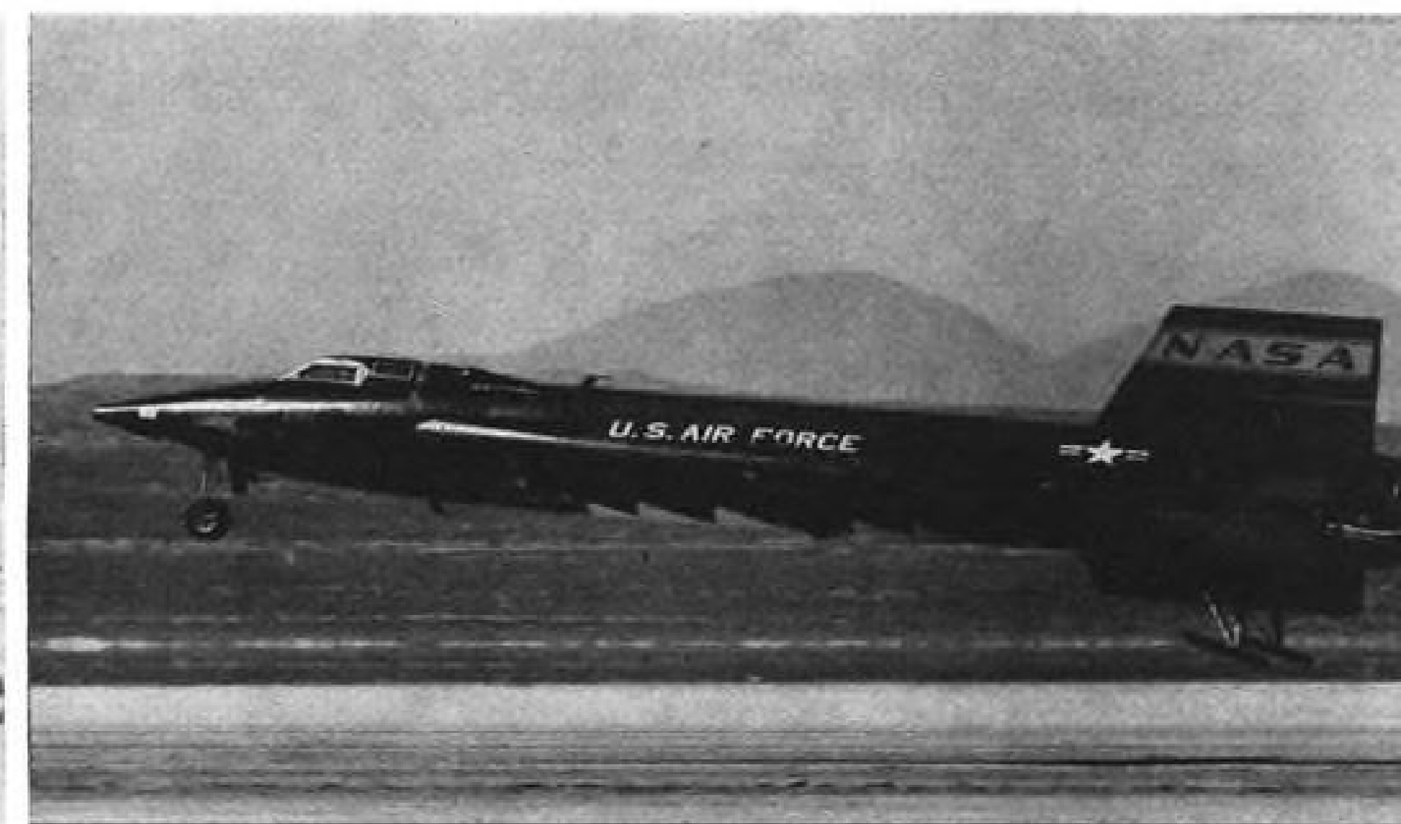
PHOTO AT LEFT in sequence shows the old hangars of the north base in background with a pronounced mirage effect of the hot desert evident. Sawtooth pattern on aircraft's belly is caused by frost collecting on the surface cooled by liquid oxygen. Next picture was taken an instant before touchdown. Airspeed at this time is 185 kt. and angle of attack is about 7 deg. with rate of descent about 4 fps.
