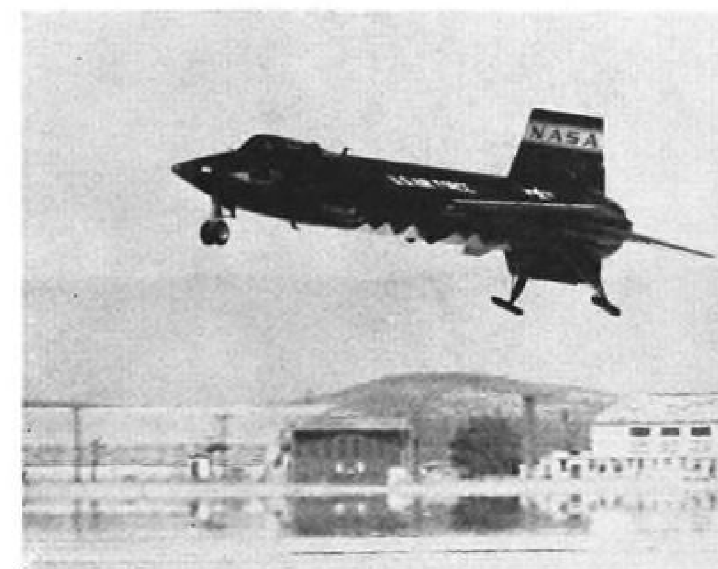
PHOTO AT LEFT in sequence shows the old hangars of the north base in background with a pronounced mirage effect of the hot desert evident. Sawtooth pattern on aircraft's belly is caused by frost collecting on the surface cooled by liquid oxygen. Next picture was taken an instant before touchdown. Airspeed at this time is 185 kt. and angle of attack is about 7 deg. with rate of descent about 4 fps.
