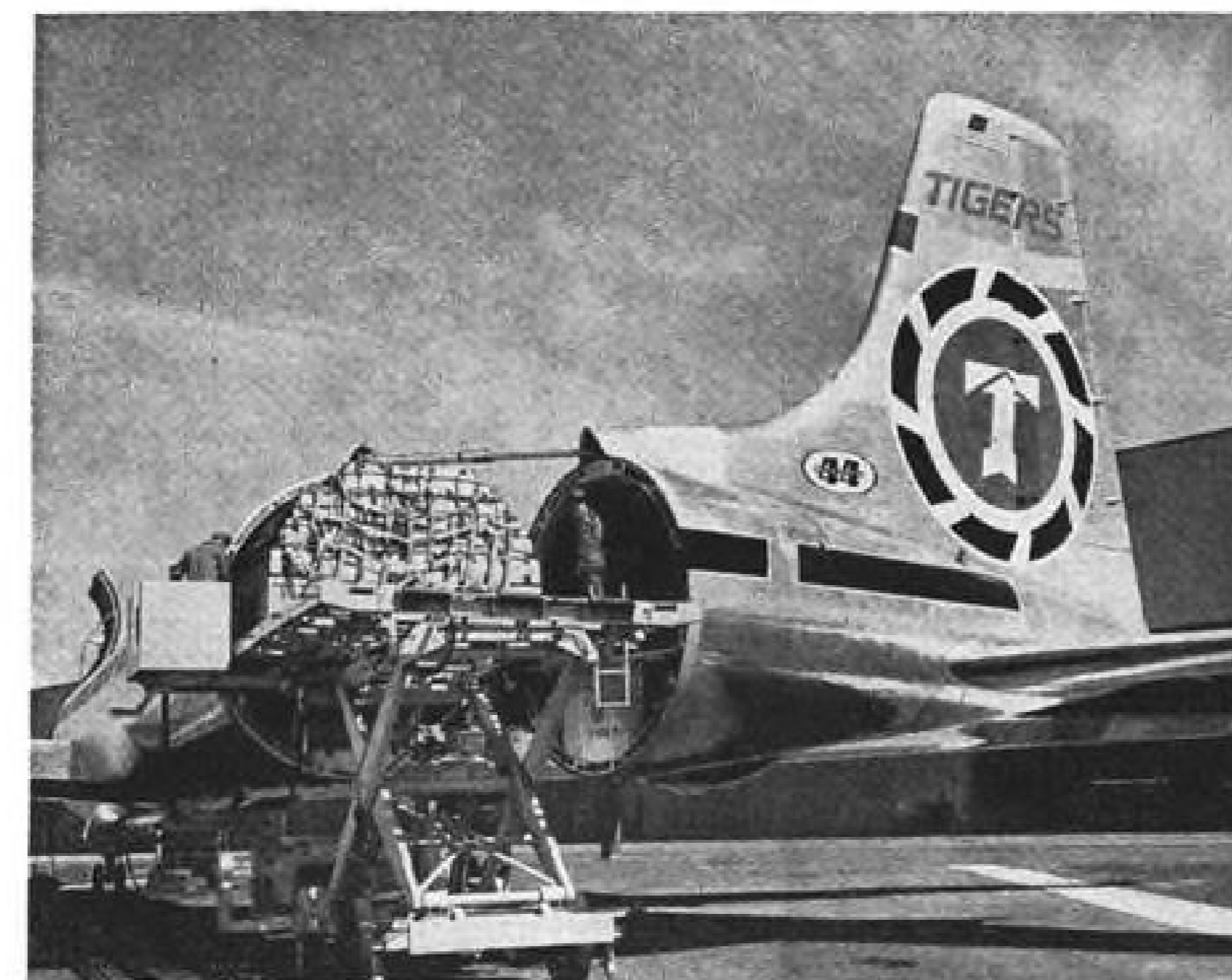
LOADING OF FLYING TIGER AIRCRAFT is speeded by use of mechanical pallet hoist. Cargo may also be loaded aboard tail section while it is open (right) and below main deck. Loading crew exits through door visible at extreme right after tail is shut and manually locked.
