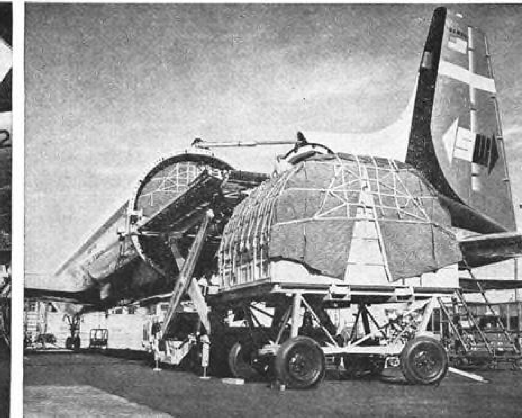
SEABOARD WORLD LOADING SYSTEM is similar to that of Flying Tiger. Pre-loaded pallets are placed aboard carts, towed to aircraft, transferred to loader and hoisted to deck height. Aircraft is ballasted with 10,000 lb. on nose so first pallet aboard doesn't force tail down.
