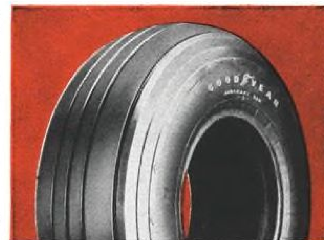
PROVEN RIB TREAD PATTERN gives optimum tire coefficient of friction—optimum tread wear and reliability. Three center grooves "pump" runway clear of water, let tire grip practically dry runway, rain or shine. Wide outer ribs resist excessive tread wear and surface cutting. Shoulder grooves supplement center grooves, maintaining a high coefficient of friction throughout tread life.
