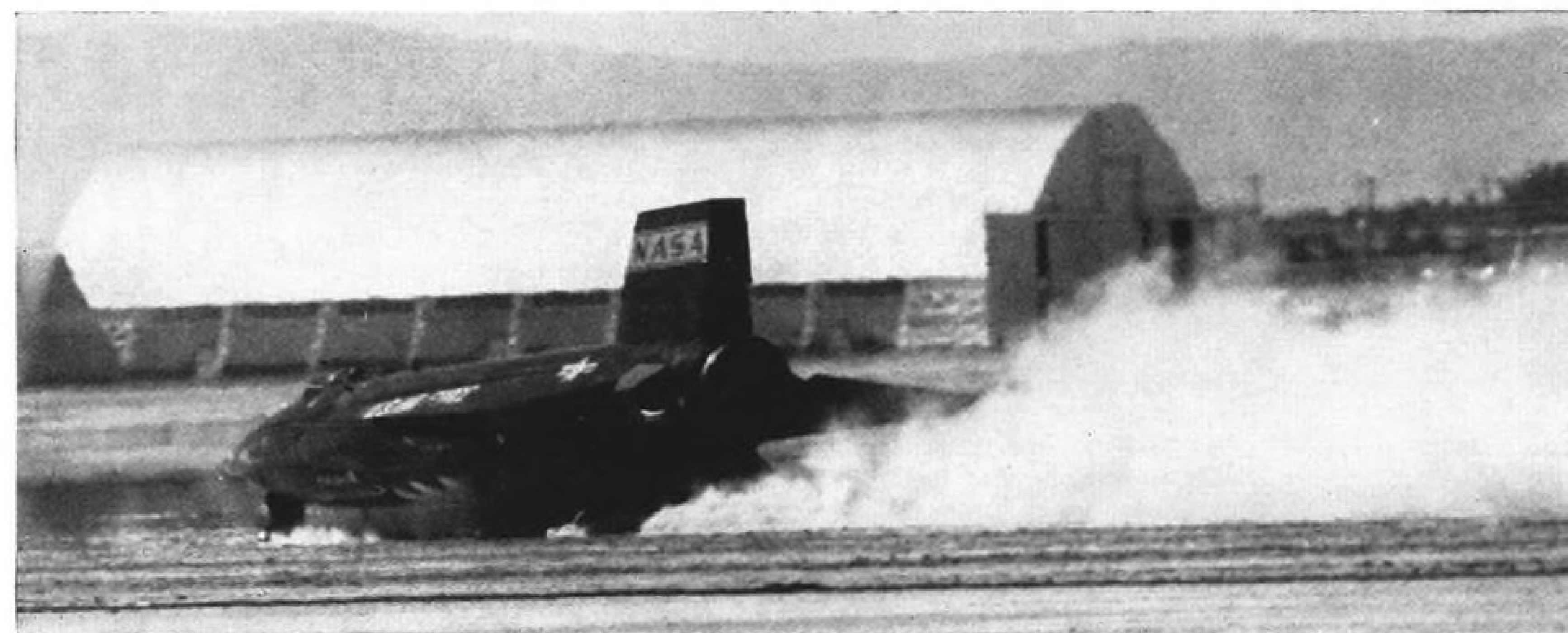
X-15 is shown rolling out after touchdown. Lake bed appears rougher than it actually is due to foreshortening of the surface by the camera's telescopic lens. Directional control is maintained by aileron deflection which places more or less weight on the appropriate skid.
