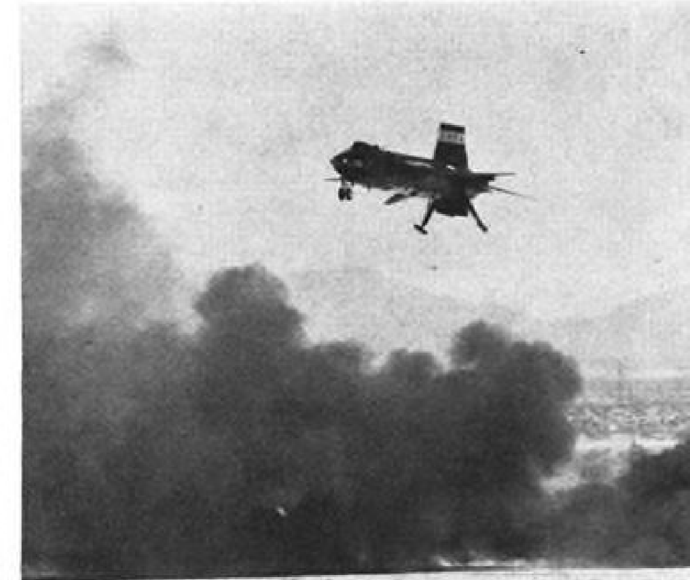
SERIES OF PHOTOS, taken with a Hulcher automatic camera with telescopic lens, shows the X-15 landing on the north lake bed at Edwards AFB. In left photo, the X-15 is completing flareout. Ventral fin already has been jettisoned and the gear extended. Smoke flare is an aid to the pilot in determining wind direction and velocity. Photo at right shows wing flaps extended.
