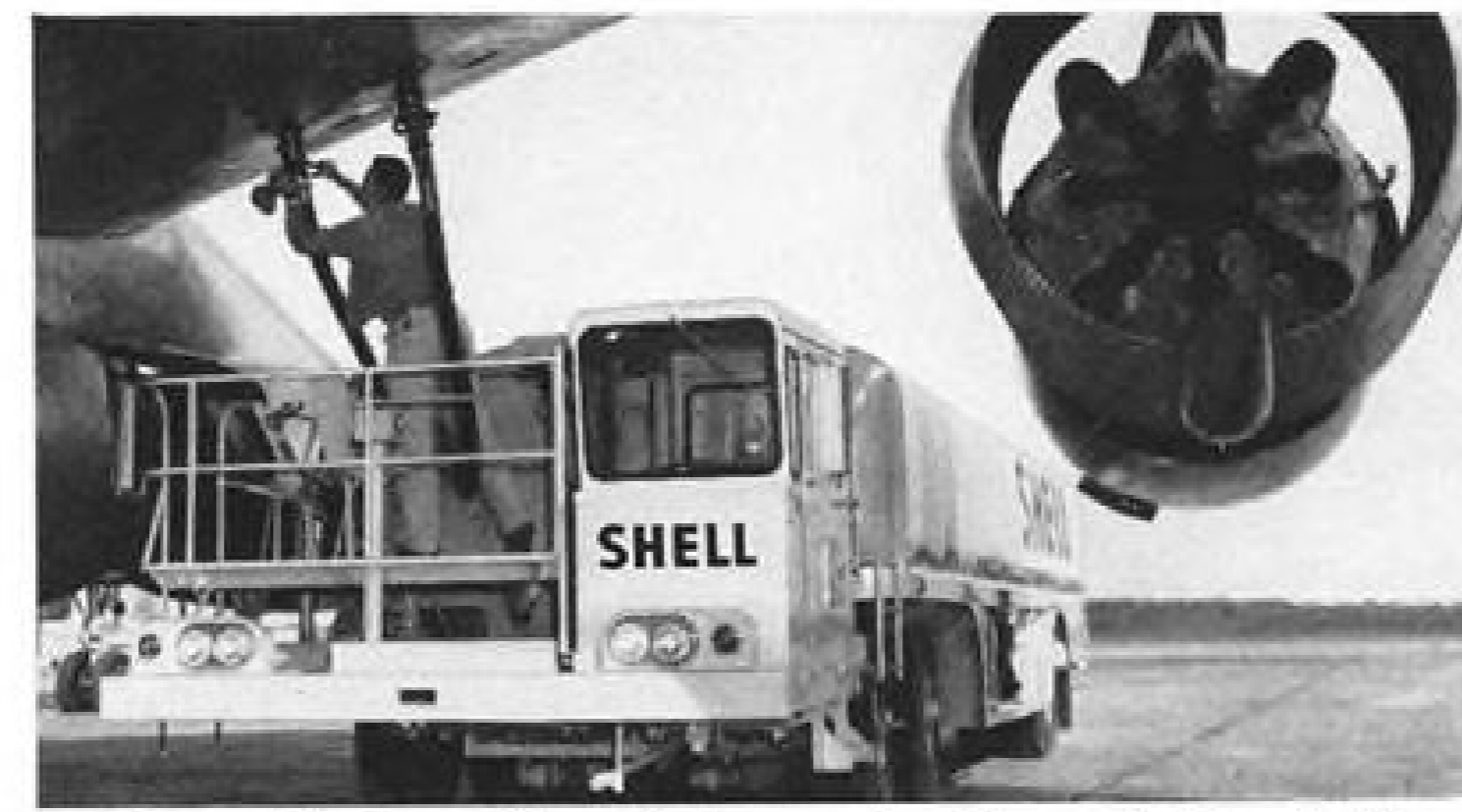
Fast refueling. New 8-thousand gallon refueler, built to Shell specifications, can transfer 8,000 gallons of turbine fuel in 13 minutes. Low silhouette permits safe underwing refueling. Cuts refueling time to the bone.
