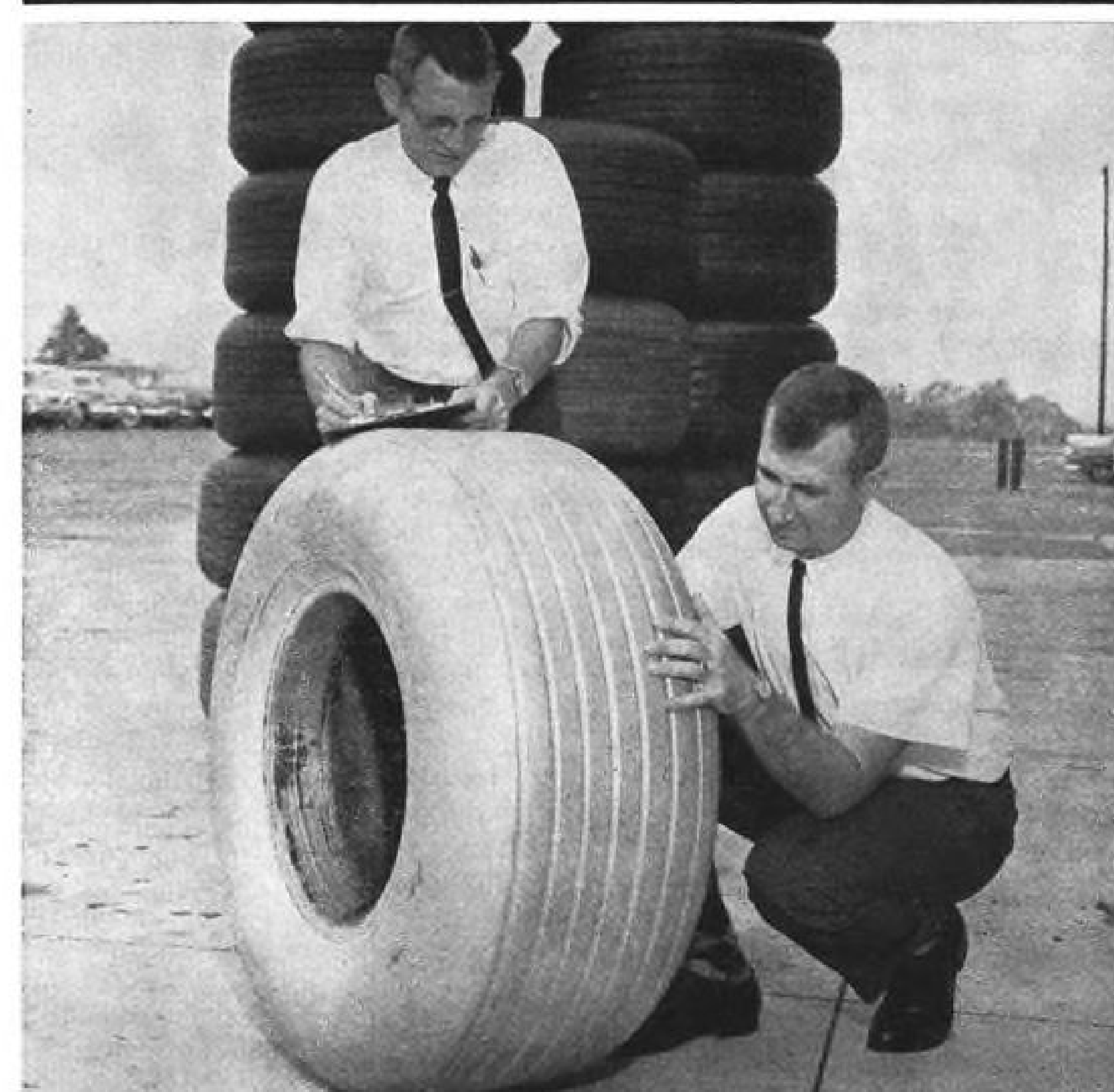
B-70 TIRE , developed by B. F. Goodrich Co., is shown during checks after completing qualification tests at Wright-Patterson AFB, Ohio. Light color is a characteristic of the new rubber compound. Tires stacked in the background were earlier experimental models.
