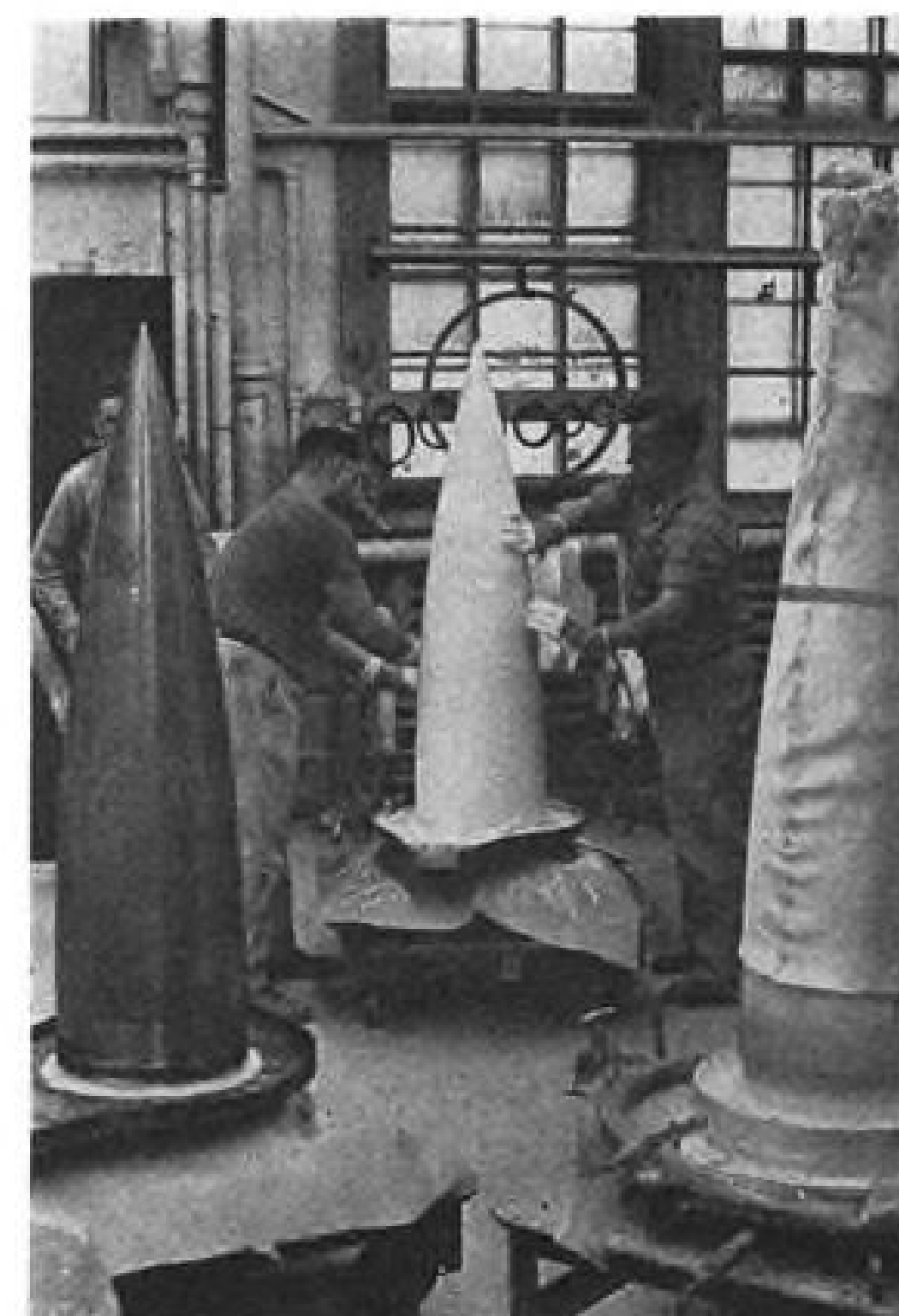
HAWK RADOME is made from layup of 28 glass cloth "socks" pulled over a steel form and hand-worked to eliminate wrinkles and impregnate the cloth. Final step is forcing excess binder out with Hydrosqueegee and curing the layup with heated rubber bag drawn over the built-up form. Cycle takes about one hour per radome.
