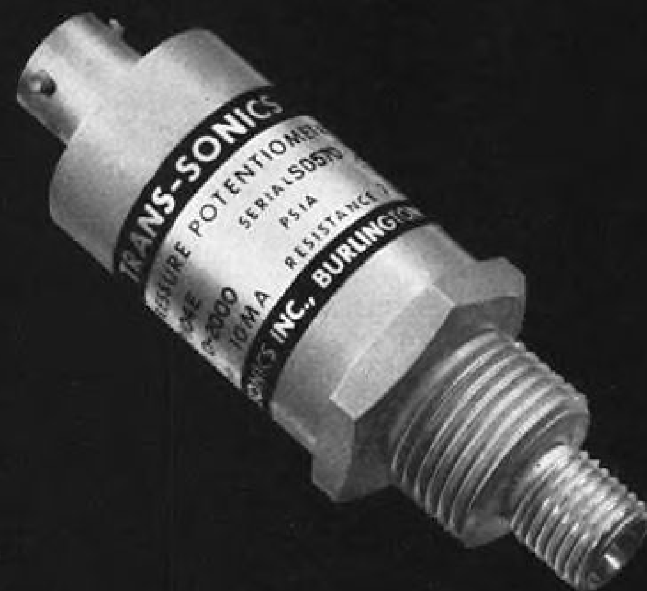
TRANS-SONICS® P104 PRESSURE POTENTIOMETER Accuracy: 1.5% • Time constant: less than 3 milliseconds • Temperature Stability: 0.008%/°F • Vibration: 35g to 2000 cps — without fluid damping • Ranges: 0-500 through 0-5000 psia; gage, differential, and lower range units available. *T.M.
