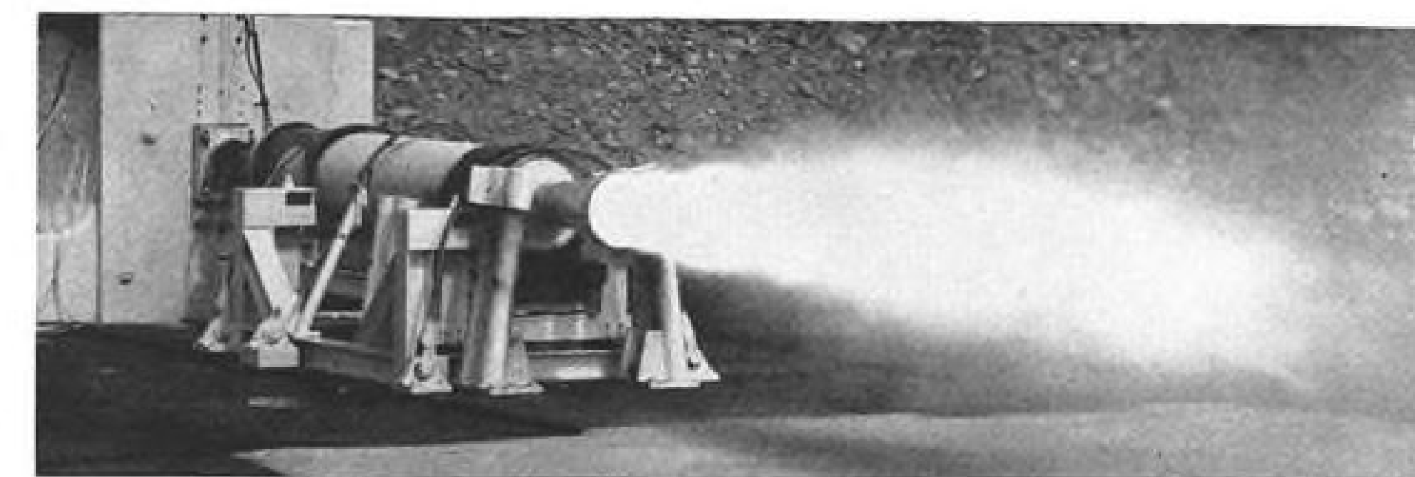
AEROJET-GENERAL solid-propellant rocket engine for Hawk missile fires at two thrust levels: boost (above) and sustaining for cruise (below).
