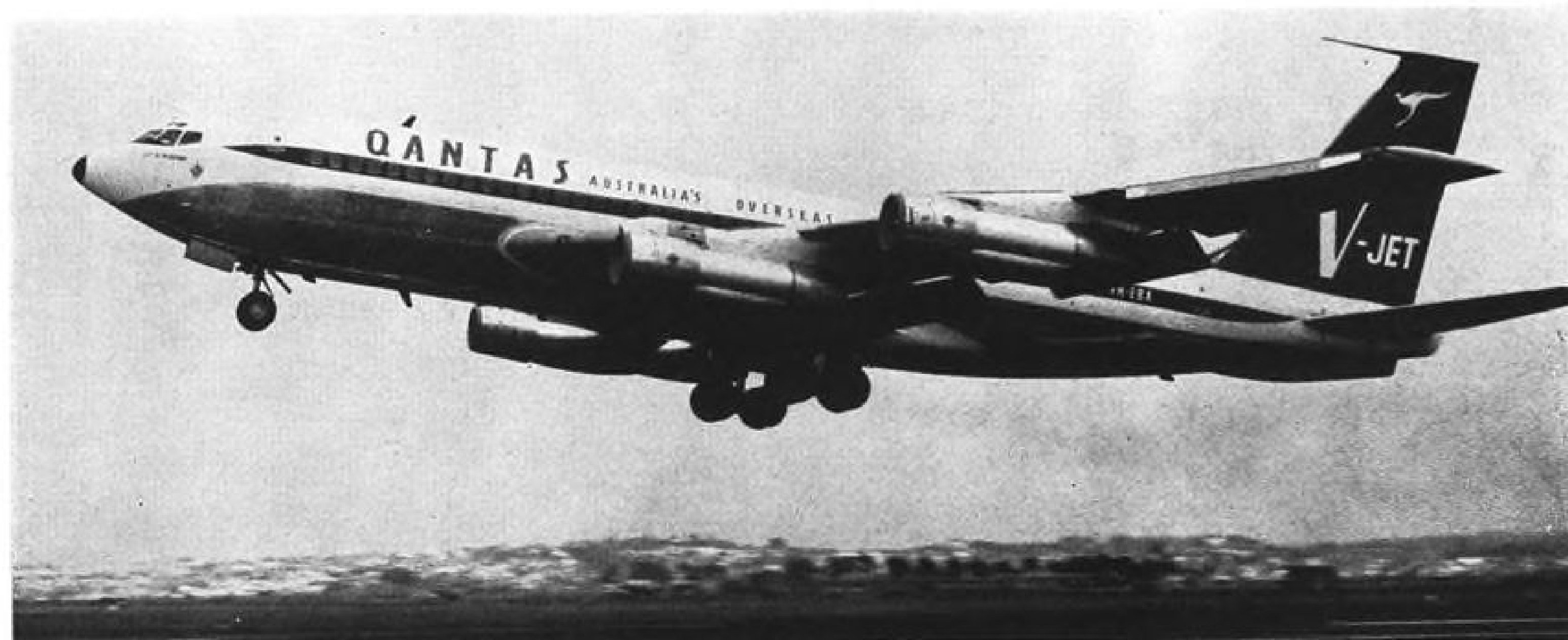
QANTAS will be operating a total of 11 Boeing 707-138B turboprop transports on its system by January. To meet Qantas requirements of limited payload and long-range capability, Boeing reduced fuselage length of the standard 707-120 by 10 ft. and redesignated the modified aircraft as the 707-138 (AW July 31, p. 39).
