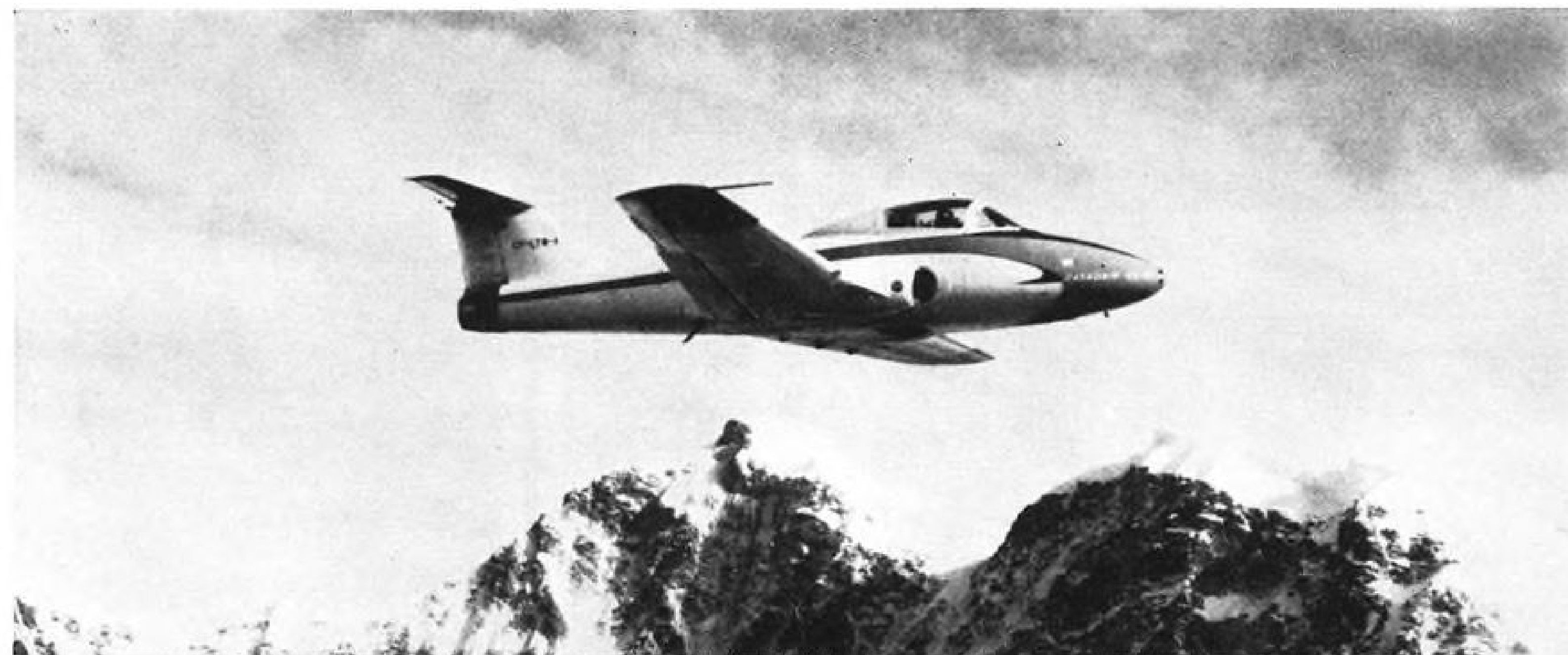
CANADAIR CL-41 is a primary and transitional trainer, designed for clean stalls, automatic spin recovery and low landing speed.
