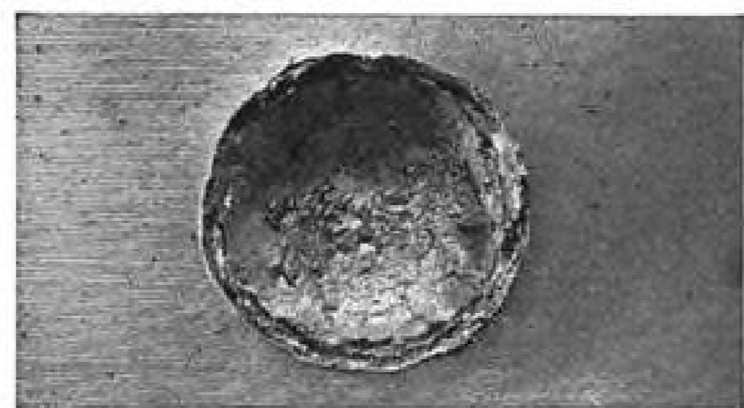
High-Velocity Impact —This is an actual photograph of the crater blasted into a block of solid aluminum by a nylon projectile in tests conducted in DSD's unique Flight Physics Laboratory. Here projectiles from two light gas guns are studied at close range, while flying faster than man has ever been able to fly them before . . . up to 31,000 feet per second. If you can use facilities like these, contact DSD.
