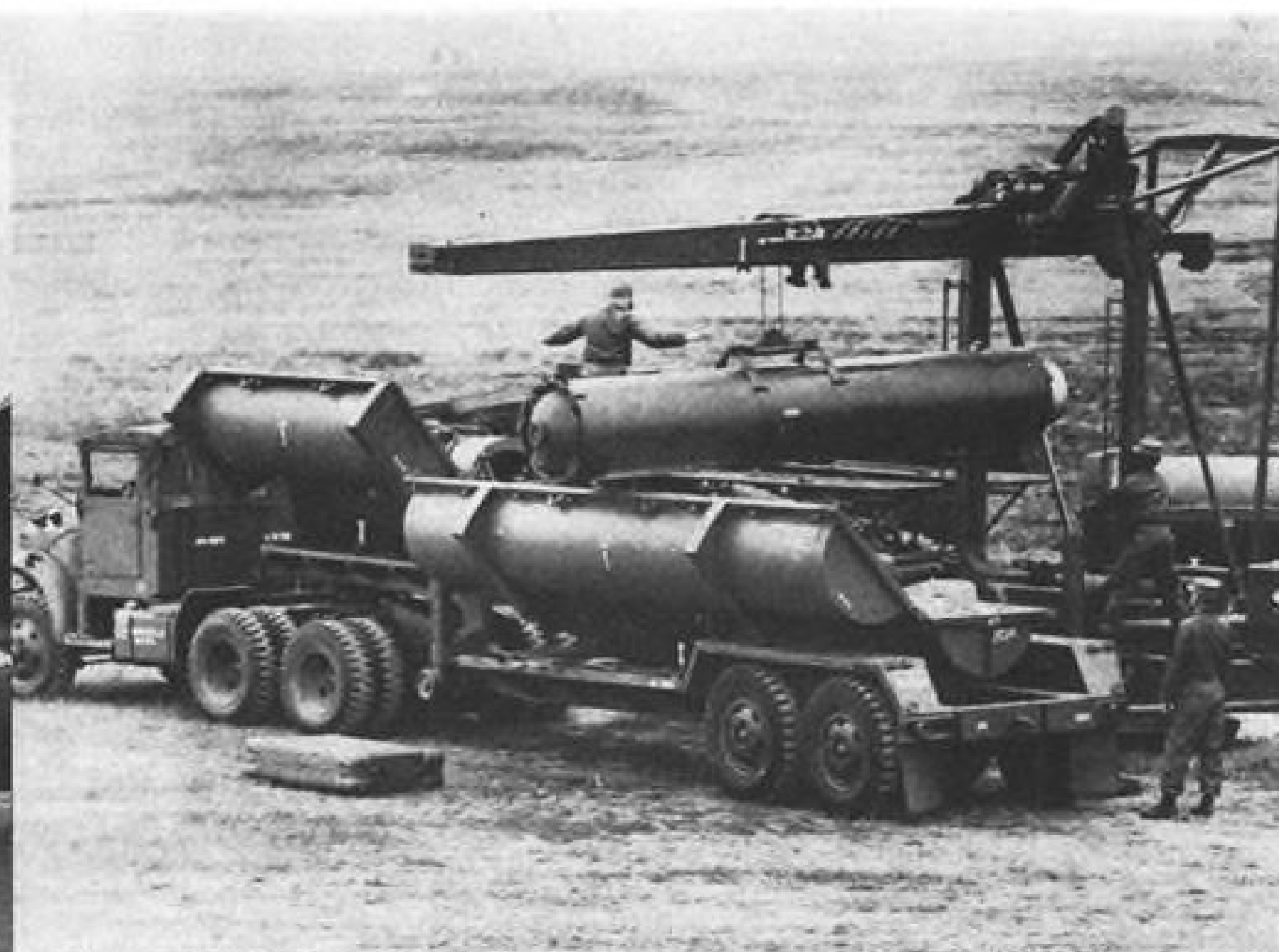
Frame components of special purpose container transport trailers are "T-1" Steel; launcher boom is also "T-1" Steel, for maximum strength and minimum weight.
