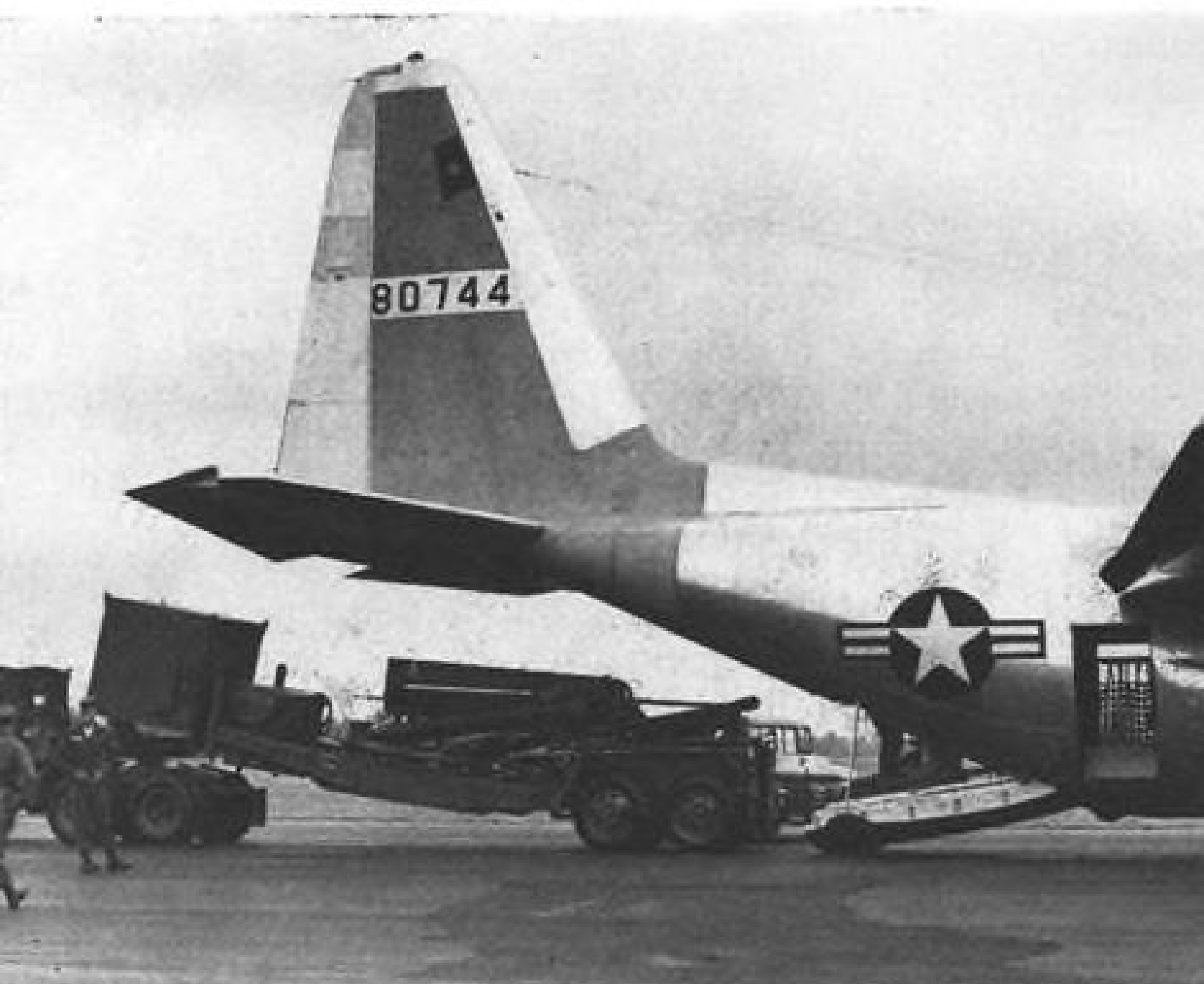
Wide use of USS "T-1" Steel makes the transporter-erector-launcher 7,000 pounds lighter and completely air-transportable.
