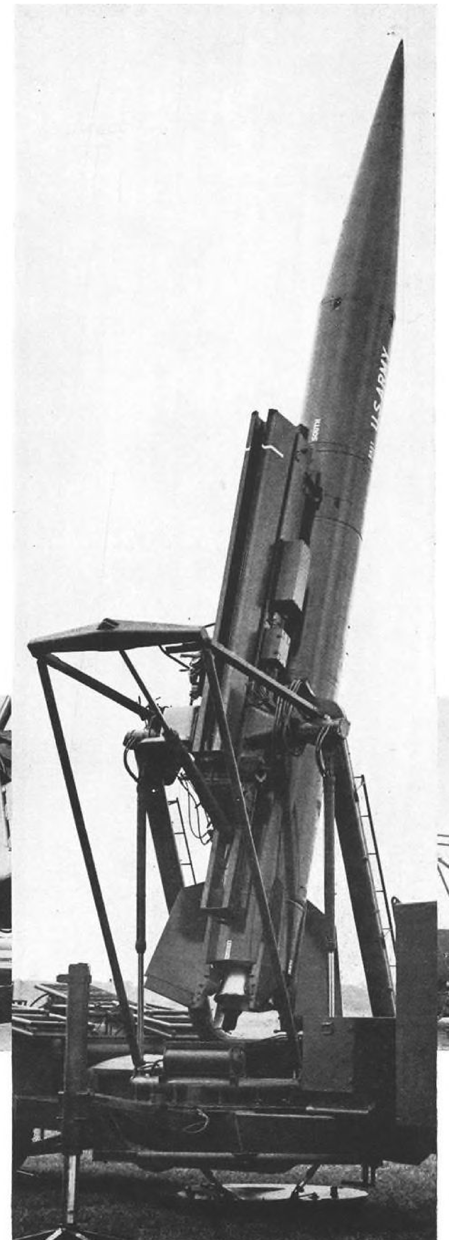
USS "T-1" Steel outrigger legs stabilize the unit in firing position. Also made of "T-1" Steel are the U-frame, extension arms, top and rear tension members and back beam.
