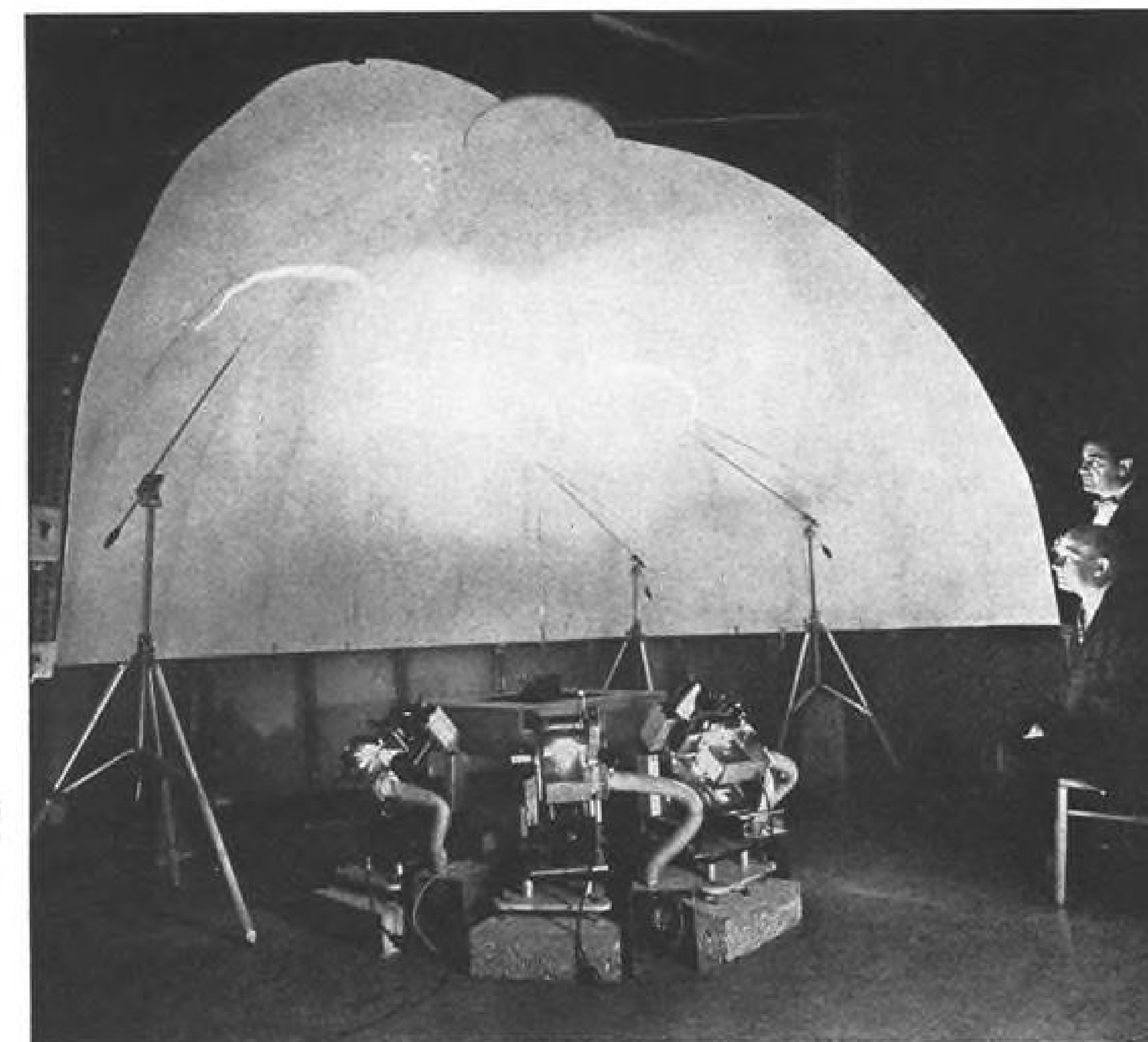
ASTRONOMICAL DOME , constructed by Geophysics Corp. scientists, is used to evaluate data gathered from tracking camera coverage of sodium cloud motion in the ionosphere.
