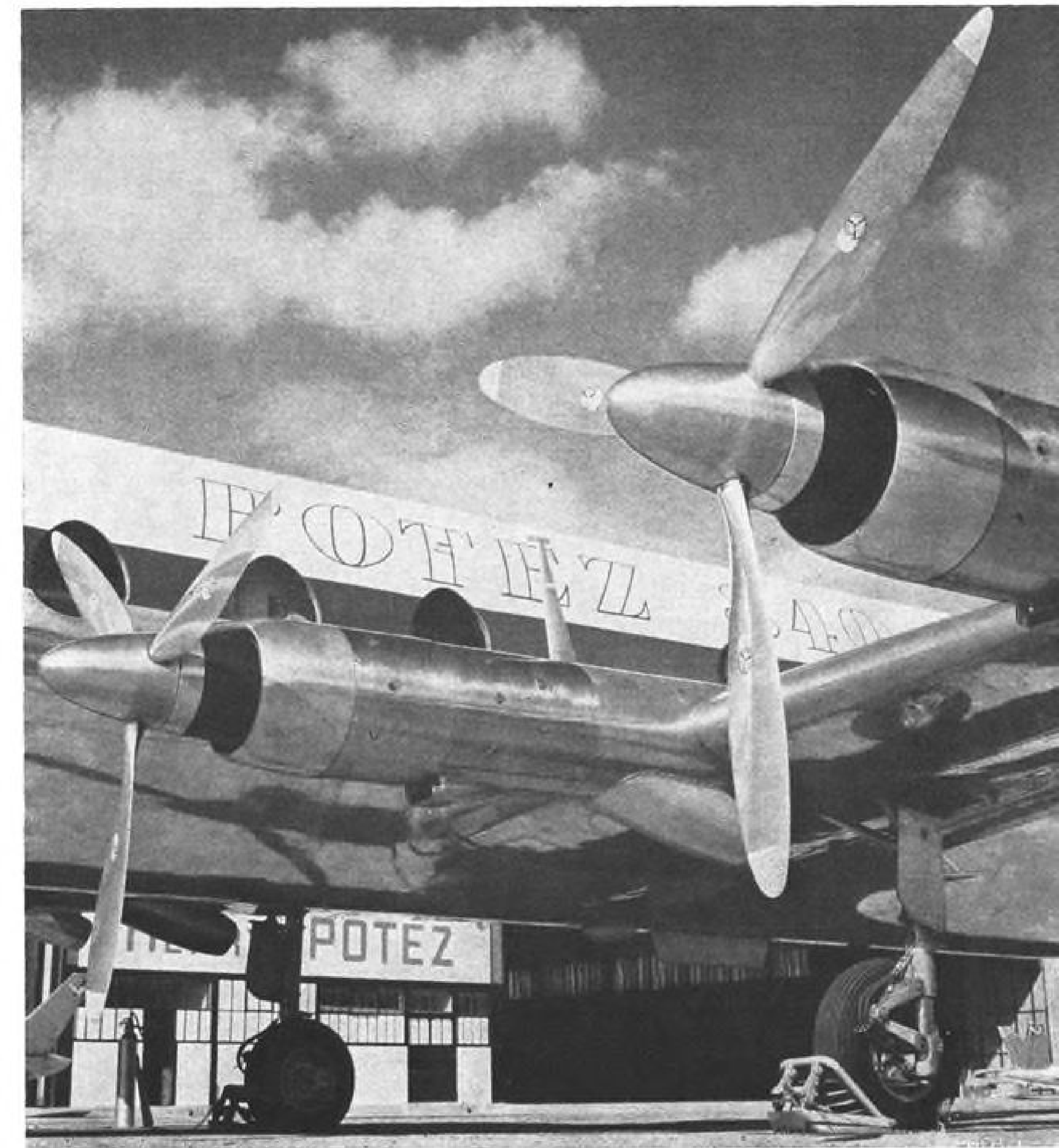
POWERPLANTS for the Potez 840 are four Turbomeca Astazou turboprop engines rated at 522 shp. Main landing gear retracts into wing. Wing skin is an aluminum alloy called Vedal A.5 which is .078 in. thick at wing root and tapers to .039 in. at tips.
