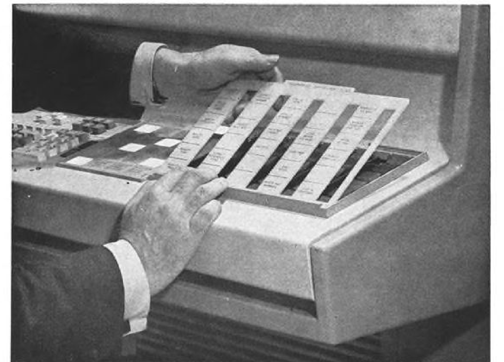
SIMPLIFICATION of communication console controls is made possible through use of 63 different plastic overlays, like one shown above, any one of which can be plugged in to alter computer routine and change functions of 30 pushbuttons on the console.
