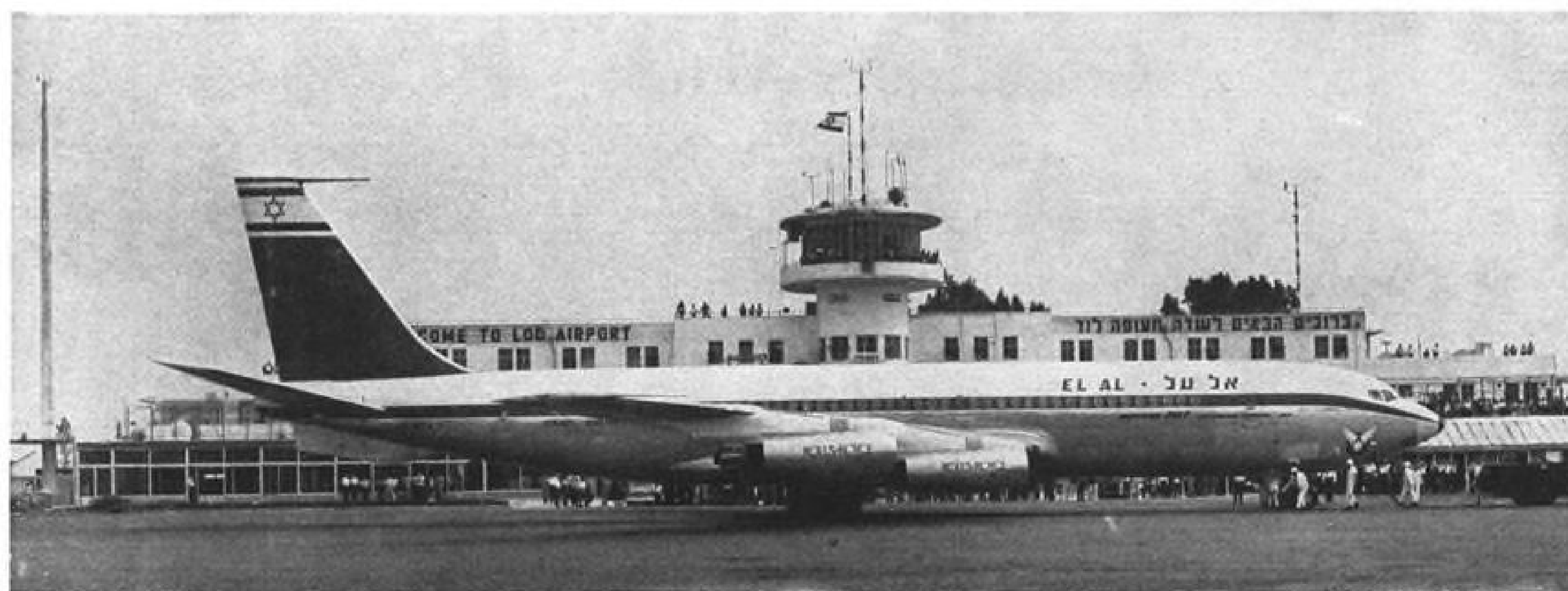
EL AL BOEING 707-420 transatlantic transport equipped with 17,500-lb.-thrust Rolls-Royce Conway bypass engines is being readied to board passengers at Tel Aviv's Lod Airport. An additional wing is being added to the small terminal building in rear to accommodate the increasing number of incoming passengers. Projected new and modernistic terminal is scheduled to be completed by 1965.
