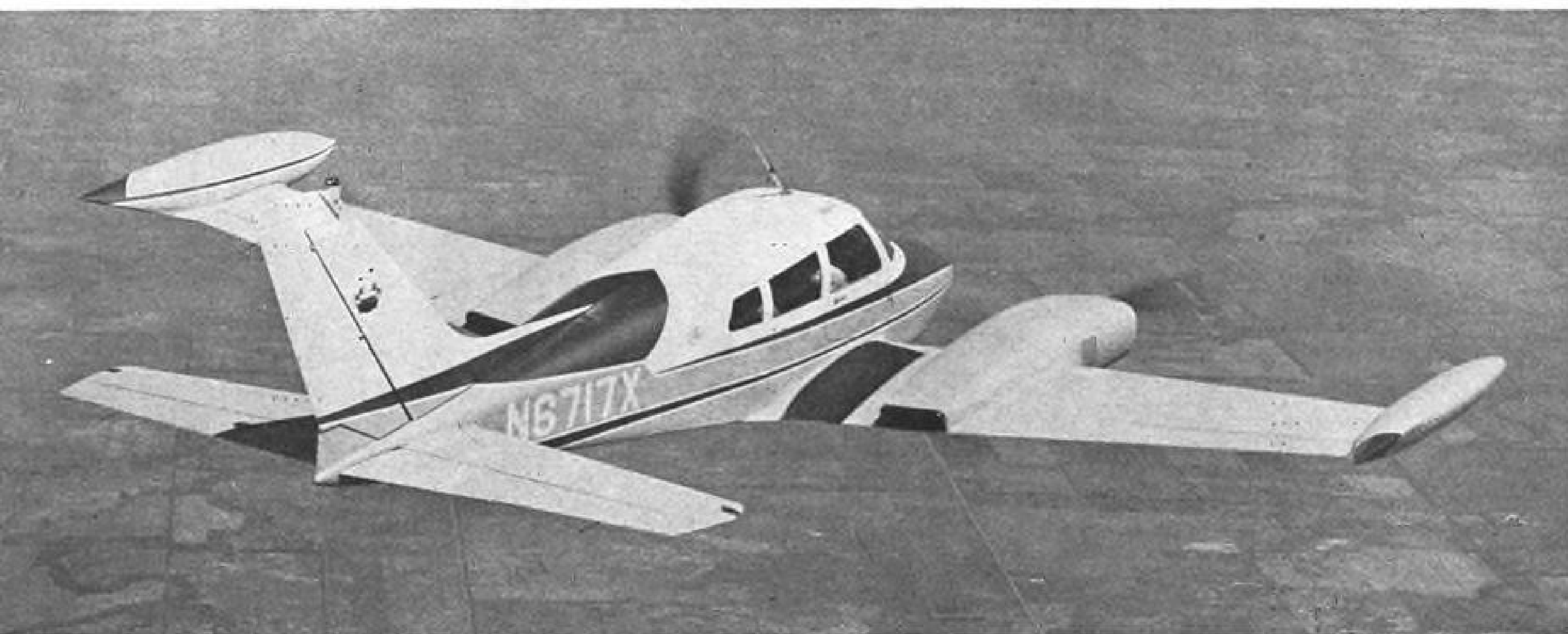
CESSNA 1962 MODEL 310G has new design tip tanks to provide better lateral stability characteristics for the aircraft.
