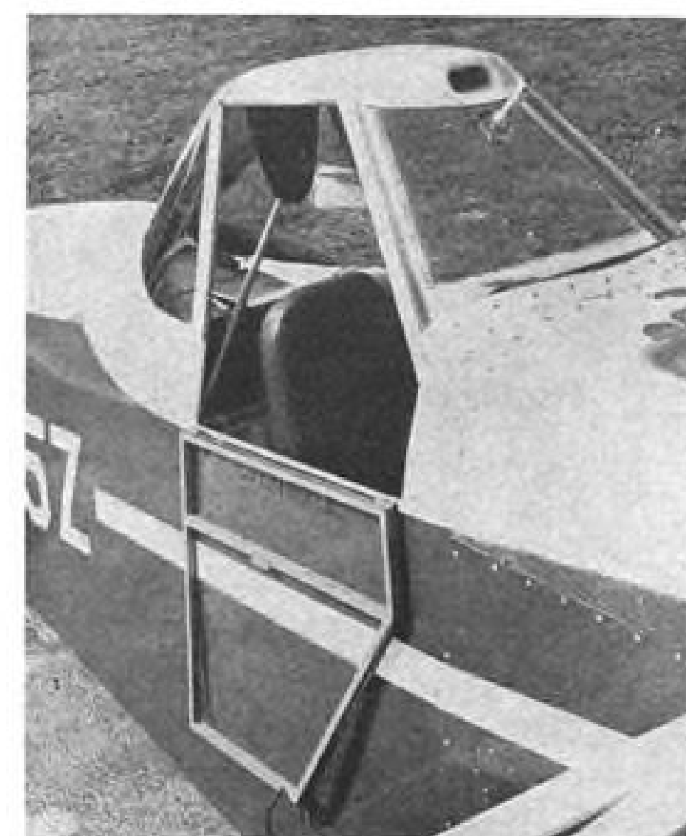
AIR INLET in canopy top above windshield provides improved, controlled cockpit ventilation; replaces former inlet mounted on side of cockpit.
