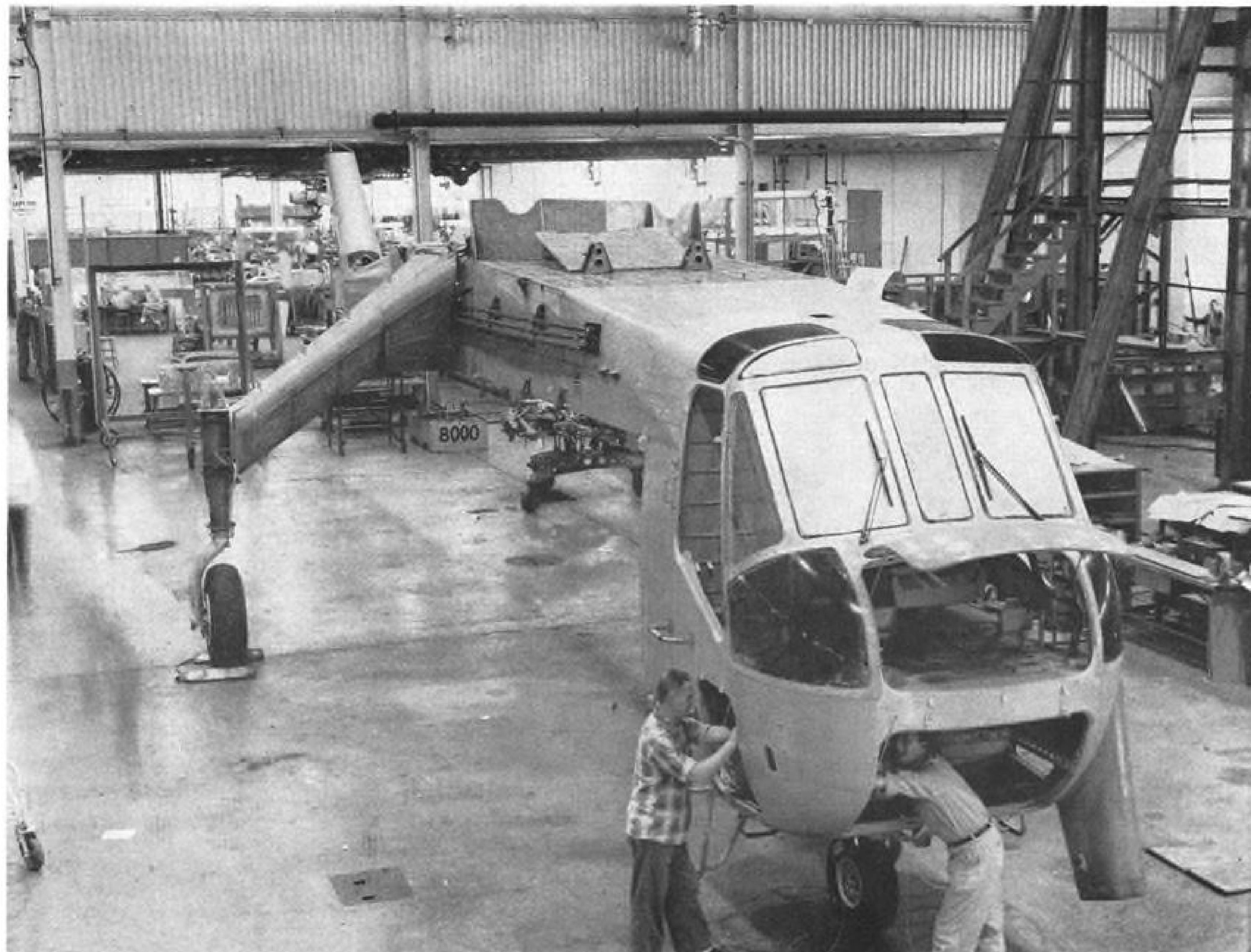
FIRST SIKORSKY S-64 TRANSPORT crane helicopter for West Germany nears completion on final assembly floor of prototype shop. Powered by paired P&WA JFTD-12A turboshafts engines, the S-64 is essentially a lifting machine which can carry a variety of loads externally or in detachable pods. Structure is designed for easy maintenance; entire upper deck of fuselage is walkway area. Hydraulic lines, electrical wiring, and control pushrods run externally along the fuselage sides. Plastic sleeve extending from left-hand side of cockpit is radar altimeter for test flights only.
