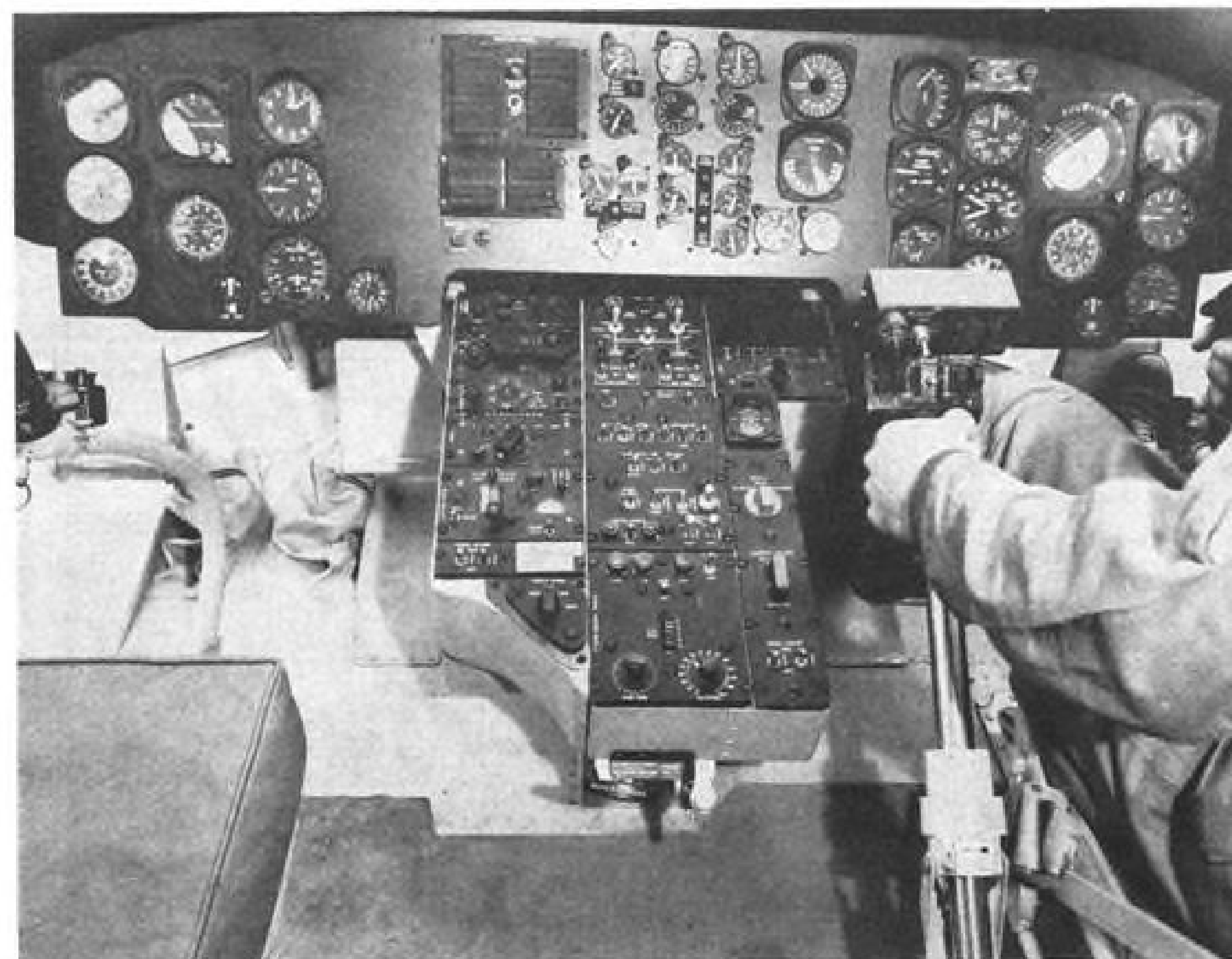
COCKPIT LAYOUT of Sikorsky S-64 is conventional except for extra access space around copilot's position at left. During crane operations, he moves to aft-facing seat behind his normal flight position. Engine instruments and warning lights are mounted on panel between pilots; crane controls and other system controls are console-mounted. Pilot's collective stick mounts tiny console.
