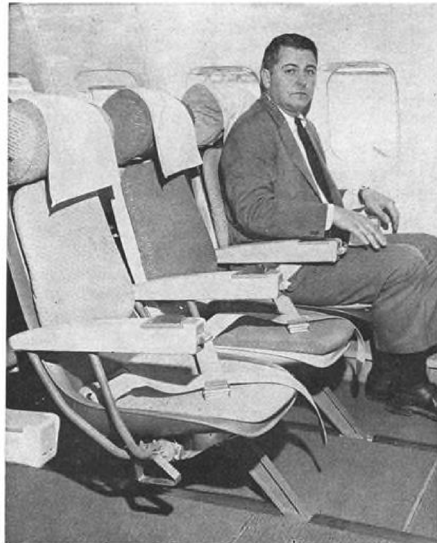
MASON SEATS , ordered by Continental Airlines and being evaluated by both American and TWA, have cushions glued to Mylar plastic shell and covered with removable seatcovers. The manufacturer claims maintenance savings of more than 50% over conventional seats are possible. Integral table is of plastic foam construction. Photo at left shows American's installation for inflight tests.
