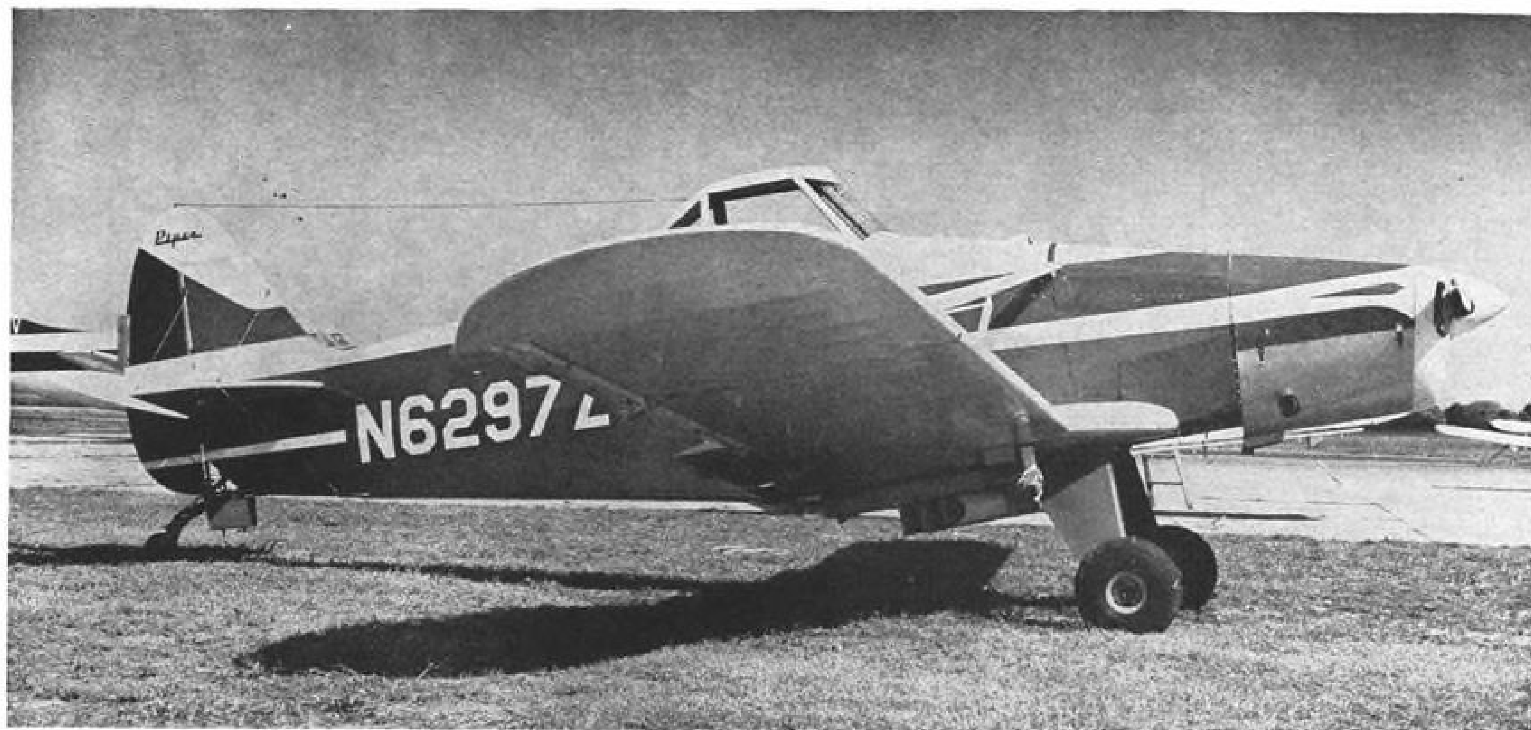
PAWNEE 235-HP. agricultural light plane retains 150-hp. model's basic structure except for some strengthening to handle 600-lb. increase in gross weight. Prototype shown is fitted with experimental engine cowling being tested to study cooling effects.
