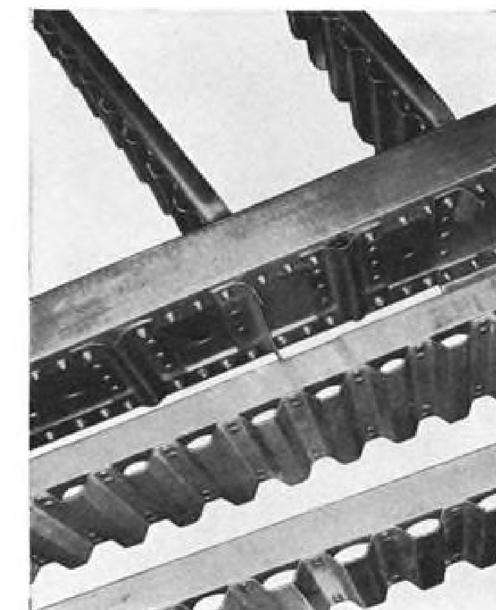
LEFT NOSE CONE splice joints are fastened with HS67 pins, type 431 stainless steel, heat treated to 125,000 psi minimum shear. The HS60M collars are R monel.
