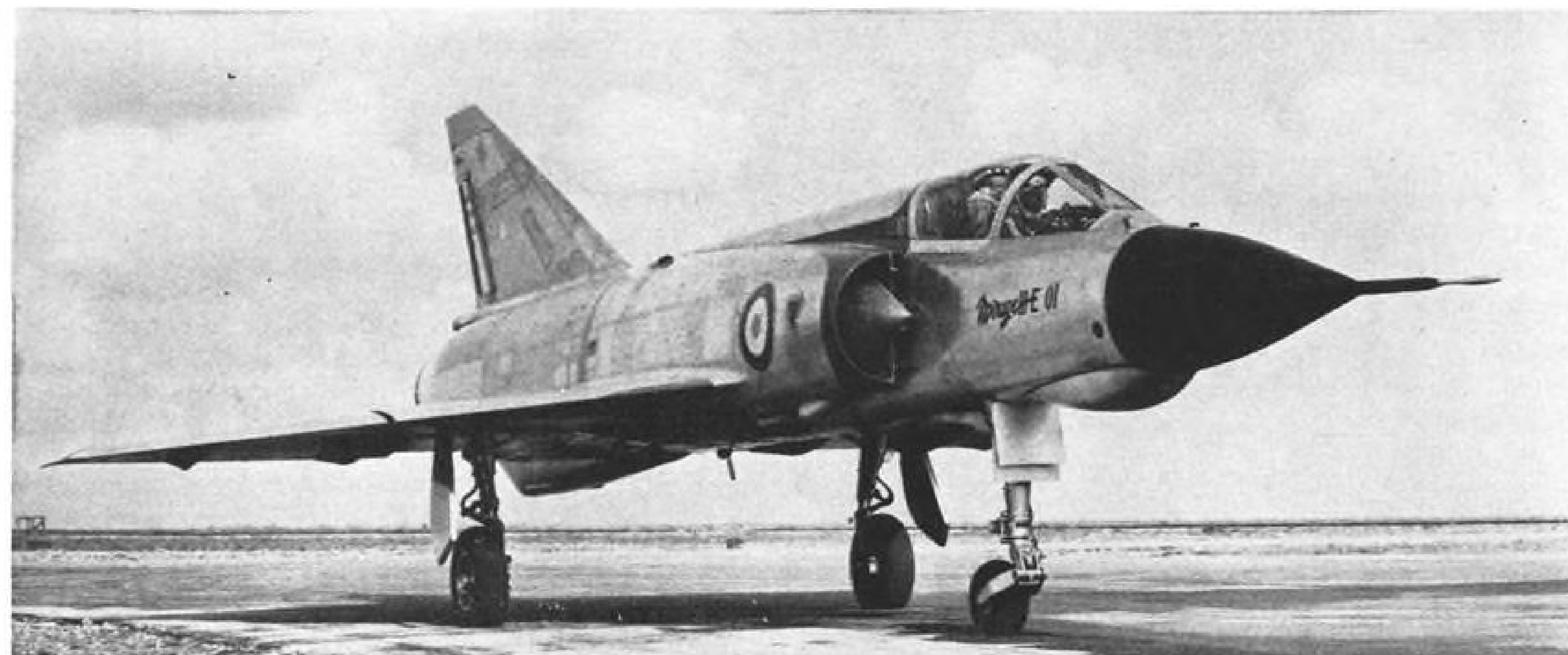
First photos show Dassault's Mirage 3-E. This French all-weather interceptor can also function as a ground-support aircraft, a capability lacking in the production Mirage 3-C. The Mirage 3-E has a cannon pod under the radar nose and a rocket pack under the tail for high-altitude interception. French air force plans to follow production of several hundred Mirage 3-Cs with the E version.
