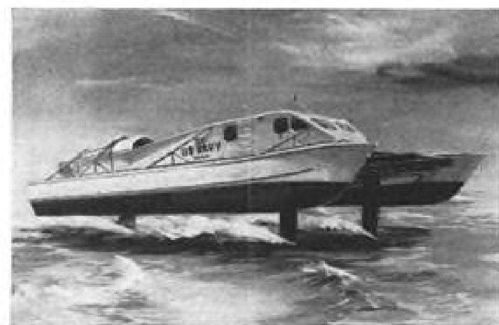
JET HYDROFOIL. Drawing shows jet-powered twin-hull test hydrofoil Boeing is designing and building for U.S. Navy. Hydrofoil will "fly" on under-water wings at 115 mph.
