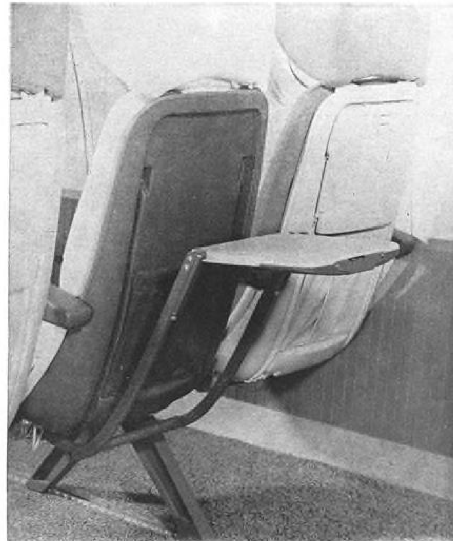
MASON SEATS , ordered by Continental Airlines and being evaluated by both American and TWA, have cushions glued to Mylar plastic shell and covered with removable seatcovers. The manufacturer claims maintenance savings of more than 50% over conventional seats are possible. Integral table is of plastic foam construction. Photo at left shows American's installation for inflight tests.
