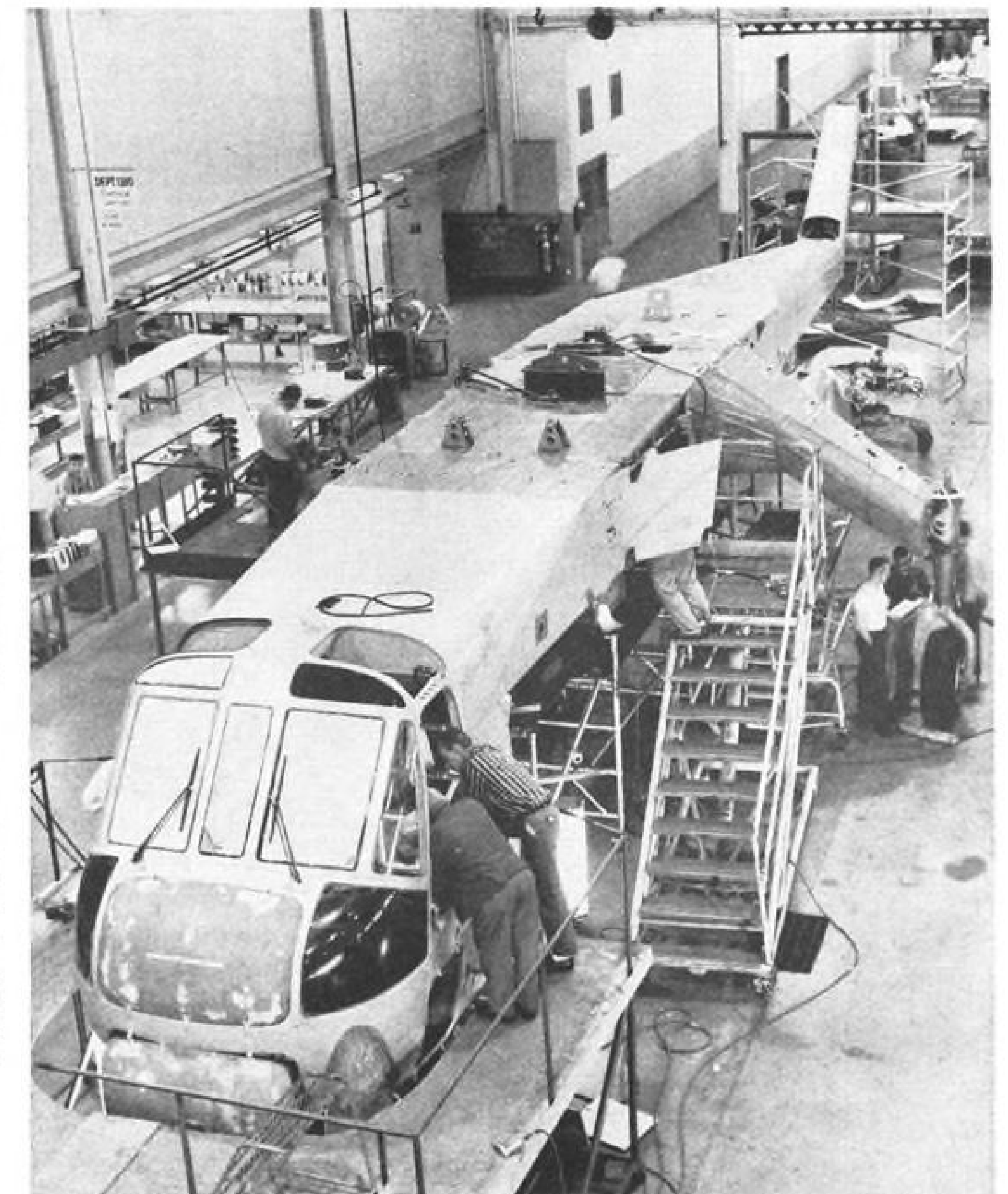
TRANSMISSION BOX (above) for S-64 is biggest built by Sikorsky so far, will handle more than 8,000 shp. through two input stub shafts. Smaller shaft ends could be connected to auxiliary propulsion system on stub wings. Below, Sikorsky mechanics complete installation of system and airframe components.
