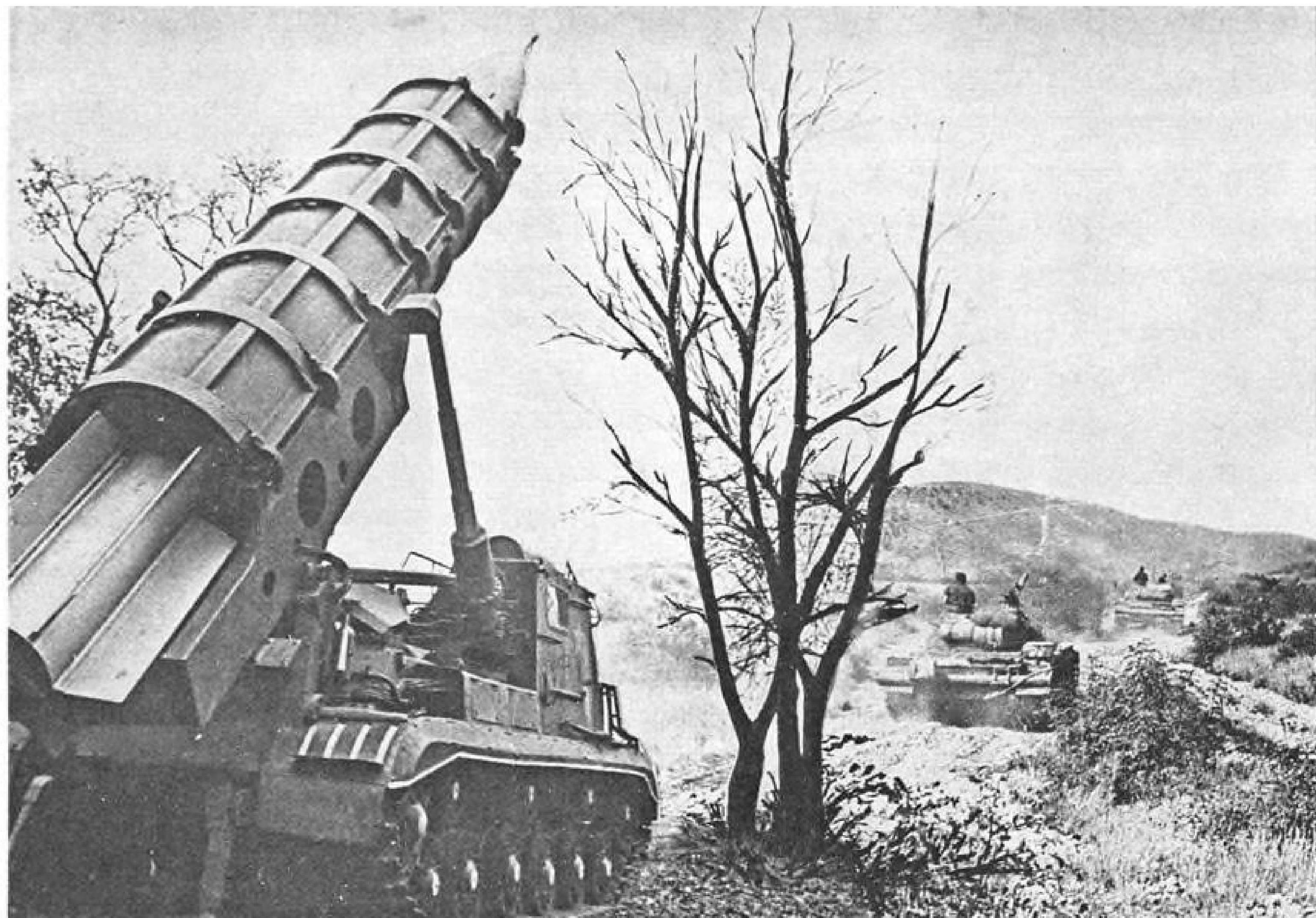
Russian unguided tactical missile, shown in firing position aboard armored carrier, has 35-mi. range. Background of picture has been heavily retouched to the immediate right of the tracked vehicle and in vicinity of tree. Missile has seven solid propellant rocket motors, fixed fins, conventional warhead. It is transported and launched from cylindrical container on vehicle with an independent power supply.
