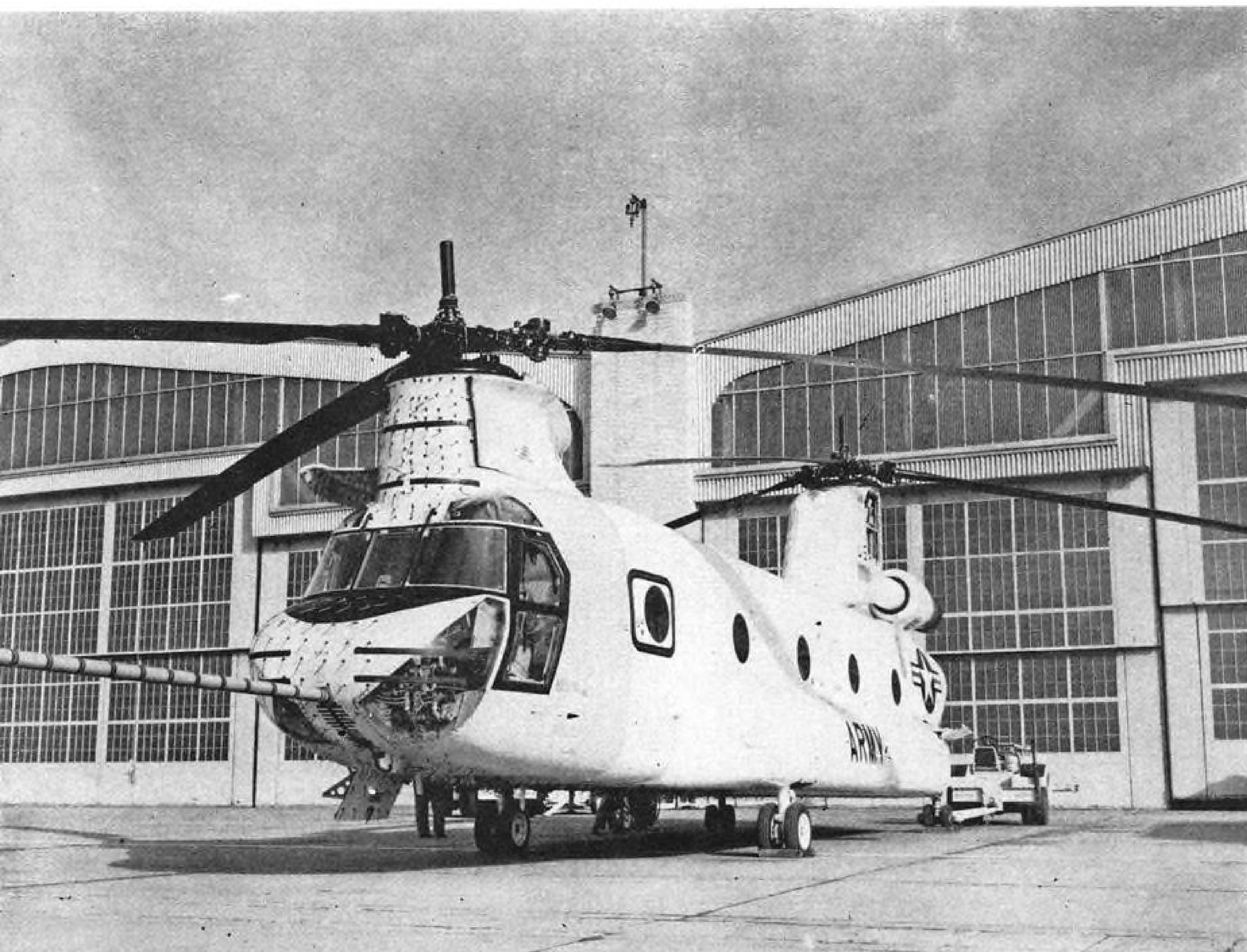
Second Vertol HC-1B Chinook helicopter for the U. S. Army carries more than 3,000 lb. of flight test instrumentation.
