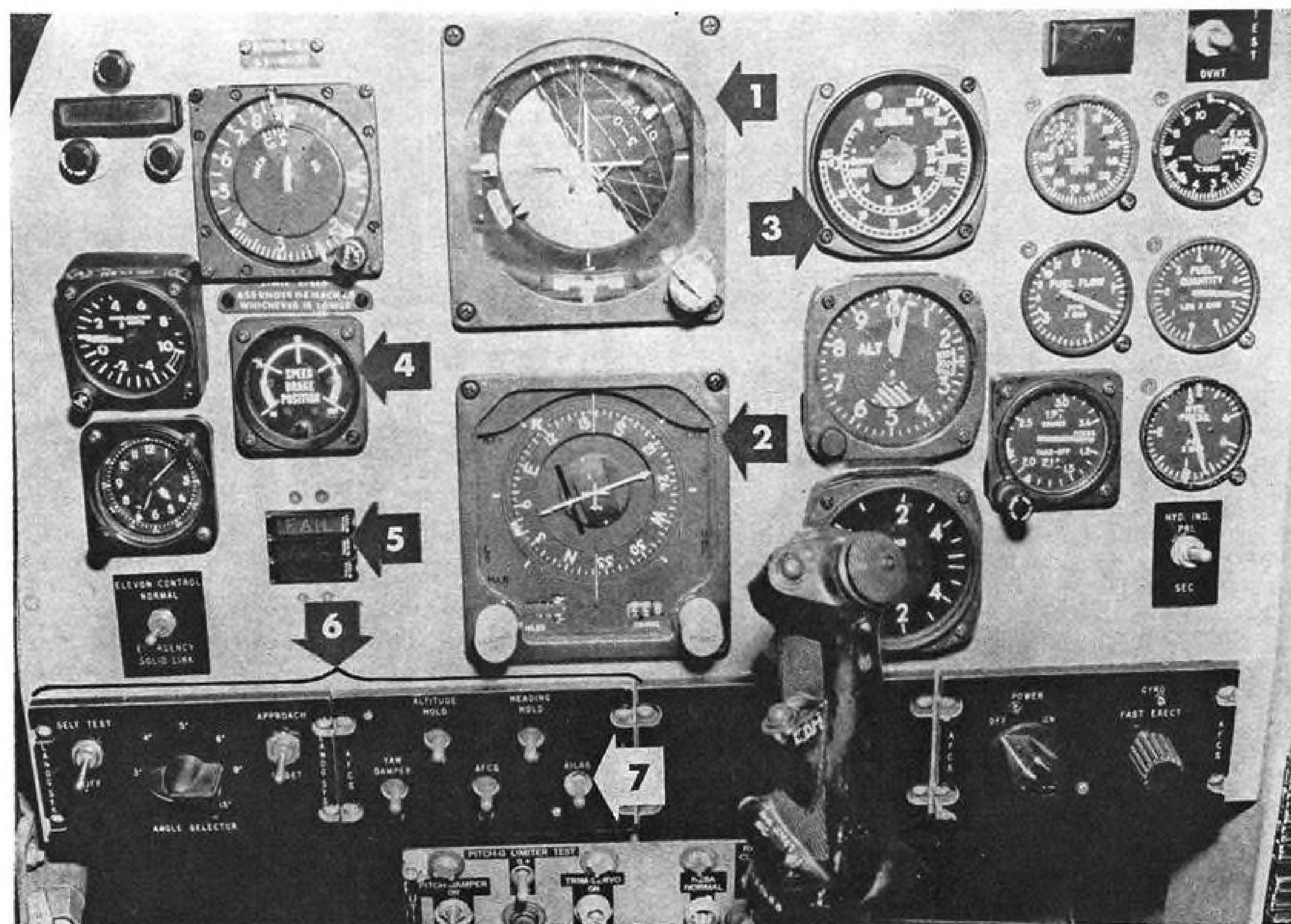
COCKPIT INSTRUMENTATION for the Autonetics APN-114 system in the TF-102A includes the following: (1) Attitude director indicator (ADI); (2) Horizontal situation indicator (HSI); (3) Radar altimeter and sinking rate meter; (4) Speed brake position indicator; (5) Function lights (top to bottom), Fail, Flare, Decrab; (6) Control panel. Once the localizer beam is captured the pilot turns on the Automatic Instrument Landing Approach System (AILAS) switch (7) and the system does the rest.
