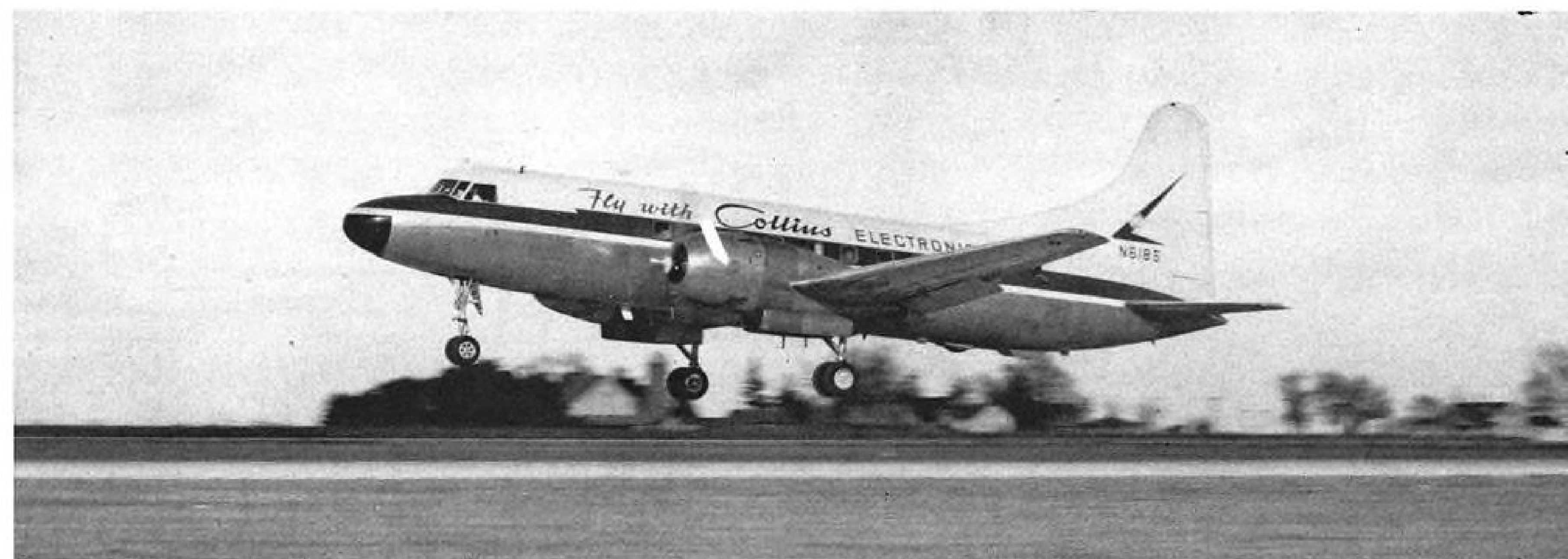
COLLINS CONVAIRE 240 is being used to evaluate new flight director instruments and improvements in autopilot, such as glide slope extension and control wheel steering, as part of company program to enhance low-approach capability of flight control equipment. New flight director system will be announced soon.
