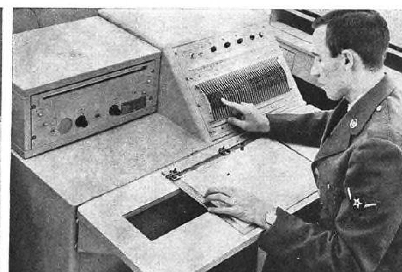
CLOSED CIRCUIT TELEVISION MONITOR in Westover AFB command post provides data for control officers. Seven monitors are located about the installation. Operator's console, right, allows AN/FMQ-5 Automatic Weather Station operators to manually inject data into processing sequence. Other information is received from automatic sensors.
