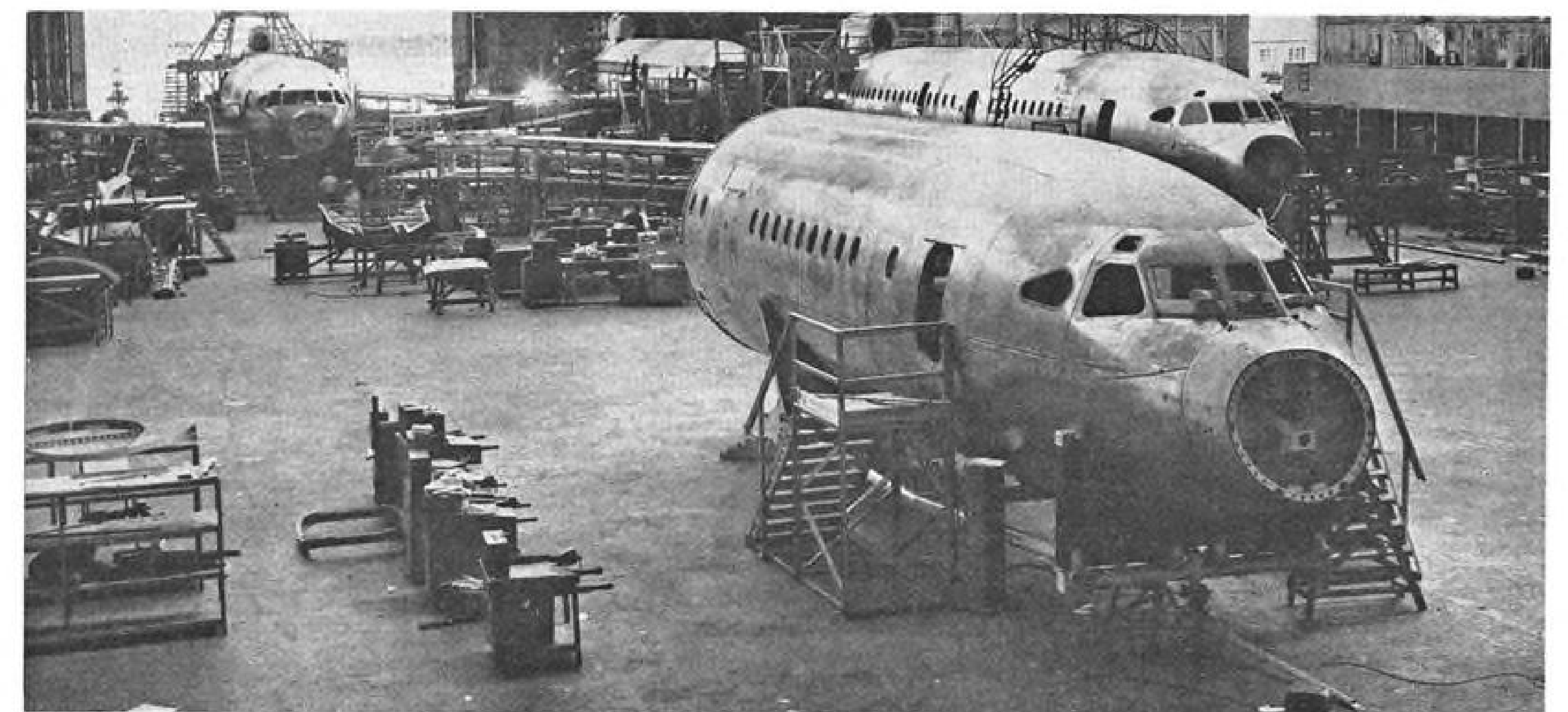
Four Tridents, the initial batch of British European Airways' order of 24, are shown in construction at de Havilland's Hatfield, England, plant. The short- to medium-range aircraft's gross weight is 107,000 lb.; maximum speed is 606 mph. (Mach .875).
