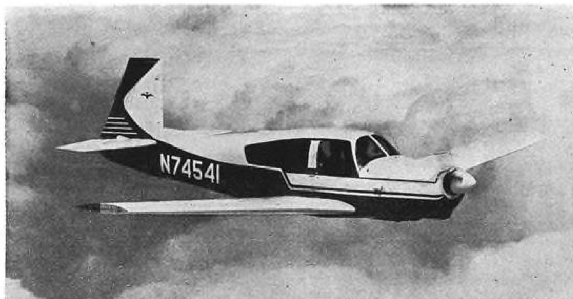
MARK 21C has low-drag, laminar-flow wing and cleaned up frontal area to increase speed without increasing power requirements. Entire tail cone is mounted on bearing and swivels when trim control wheel is moved. The aircraft has all spaces between stationary surfaces and movable control surfaces sealed.
