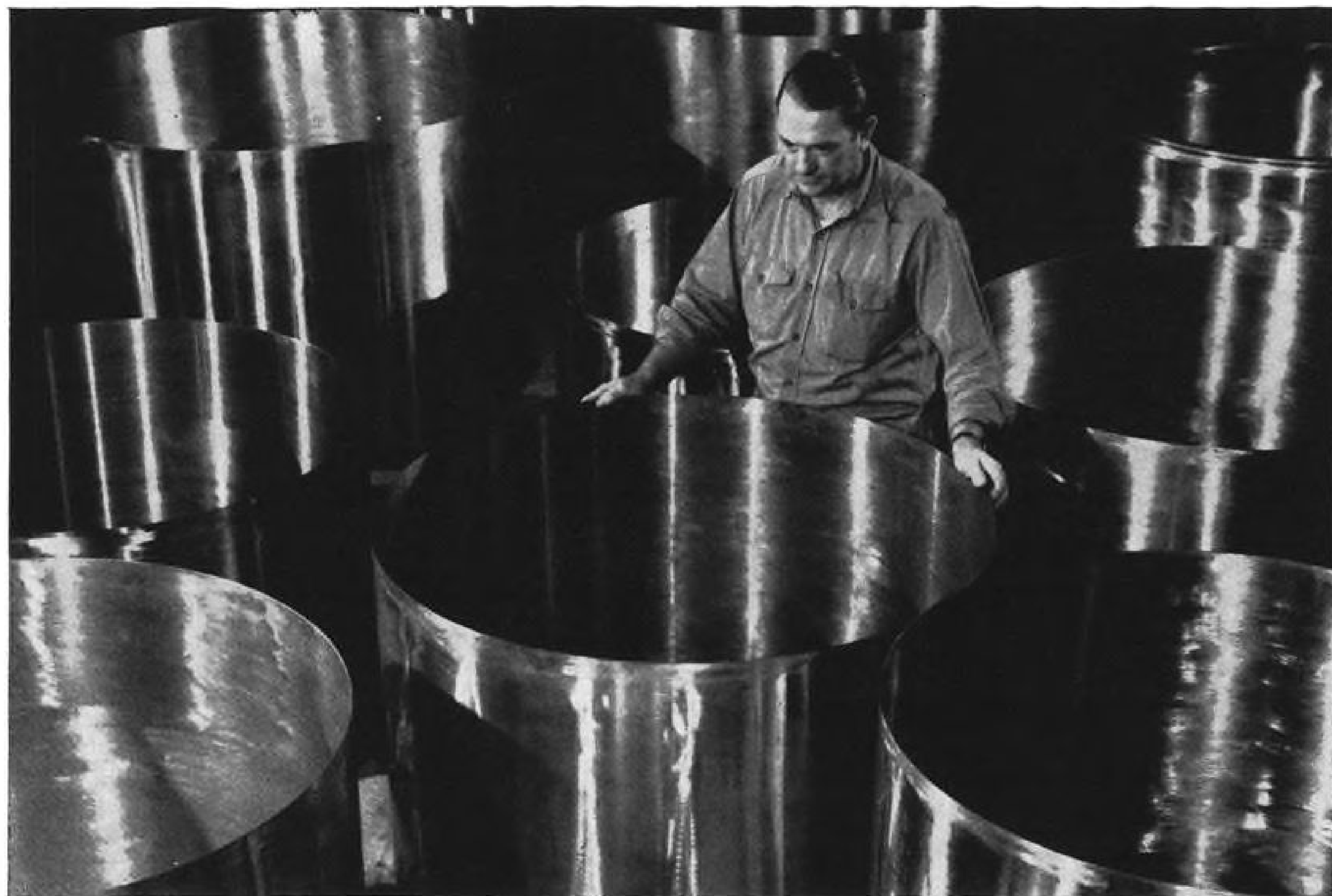
Titanium roll-forged parts prior to welding into body-sections of Minuteman casings at Lycoming Division of the Avco Corporation.
