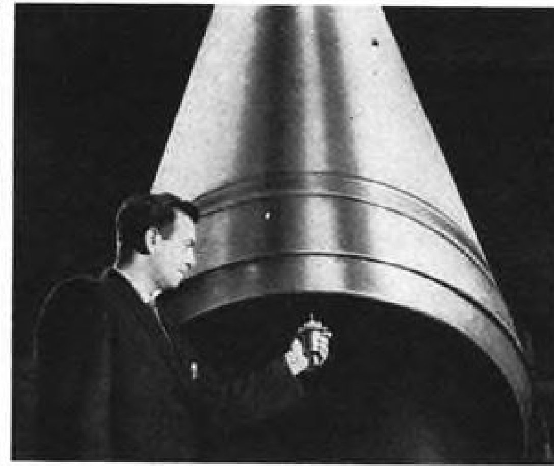
The scope of Wright Aeronautical activity in the missile and space propulsion field is illustrated in this comparison of a miniature-sized variable thrust rocket engine (in engineer's hand) and a huge 21-foot long rocket motor case fabricated for the Minuteman missile program.
