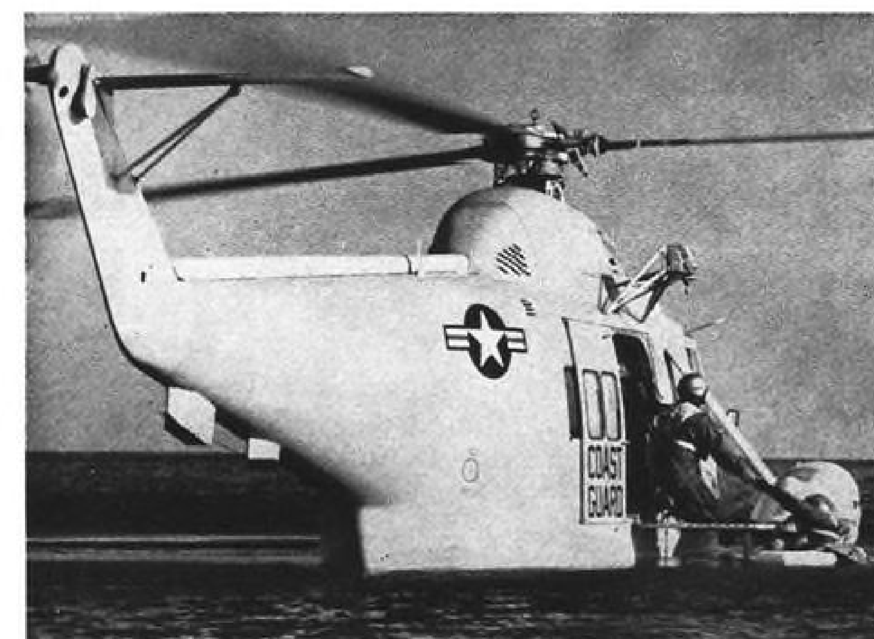
Rescue platform folds up, over and down to form deck extension of S-62. Crew chief can rapidly pull victim aboard.
