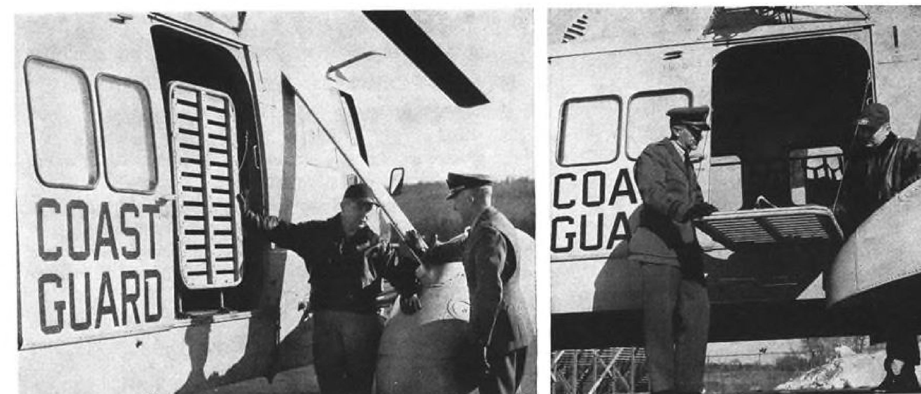
Rescue platform is being modified to fit flush with interior decking. Sikorsky originally developed the idea to meet Swiss requirements.
