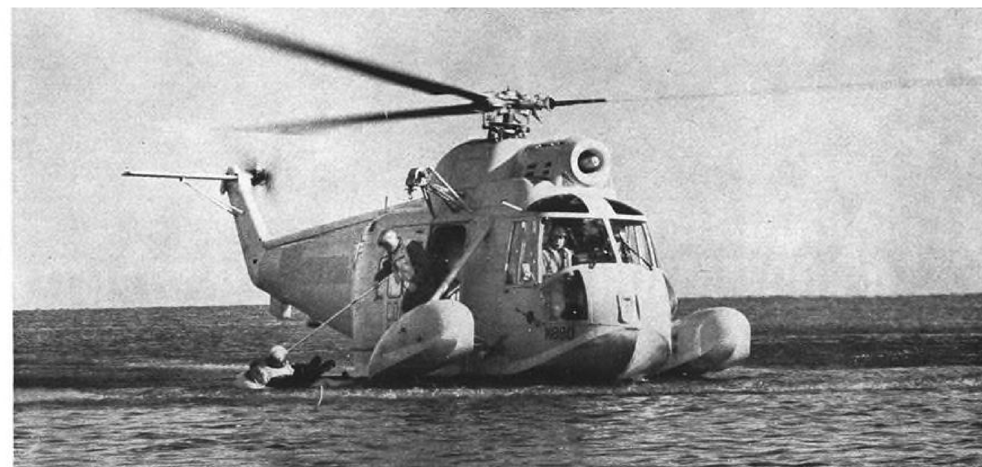
Sikorsky S-62 (HU2S-1) turbine-powered helicopter selected by Coast Guard is amphibious and has operated from 8-10 ft. seas. A company-funded project, it is powered by a General Electric T58-8 gas turbine engine.
