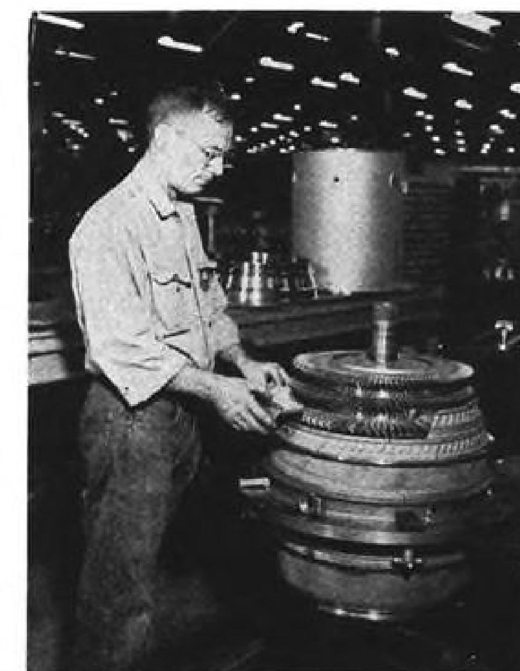
STATOR VANES are being installed on third-stage turbine wheel on Allison's turboprop assembly floor. As of last month, a total of 1,052 Model 501 engines, including the inventory of spares, was in service with Electras and Convair 340 and 440 transports with domestic and foreign airlines, corporations and individuals. Total breaks down into 798 in domestic airline service, 202 with foreign airlines plus an additional 52 in Convairs.
