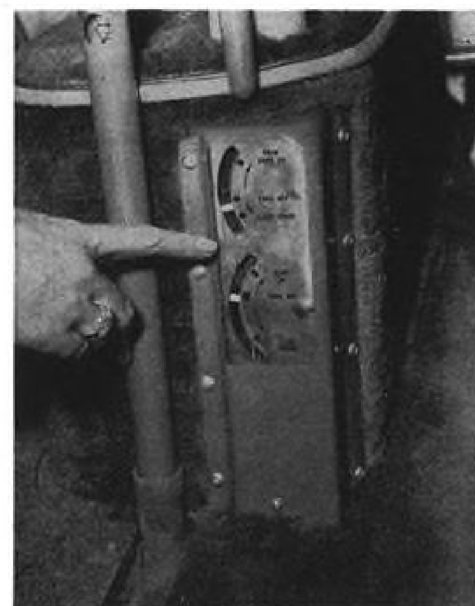
TRIM AND FLAP indicators have been added to the cockpit and are located on the nosewheel well covering. Gear retraction lever is at left and flap pump handle is above indicators.
