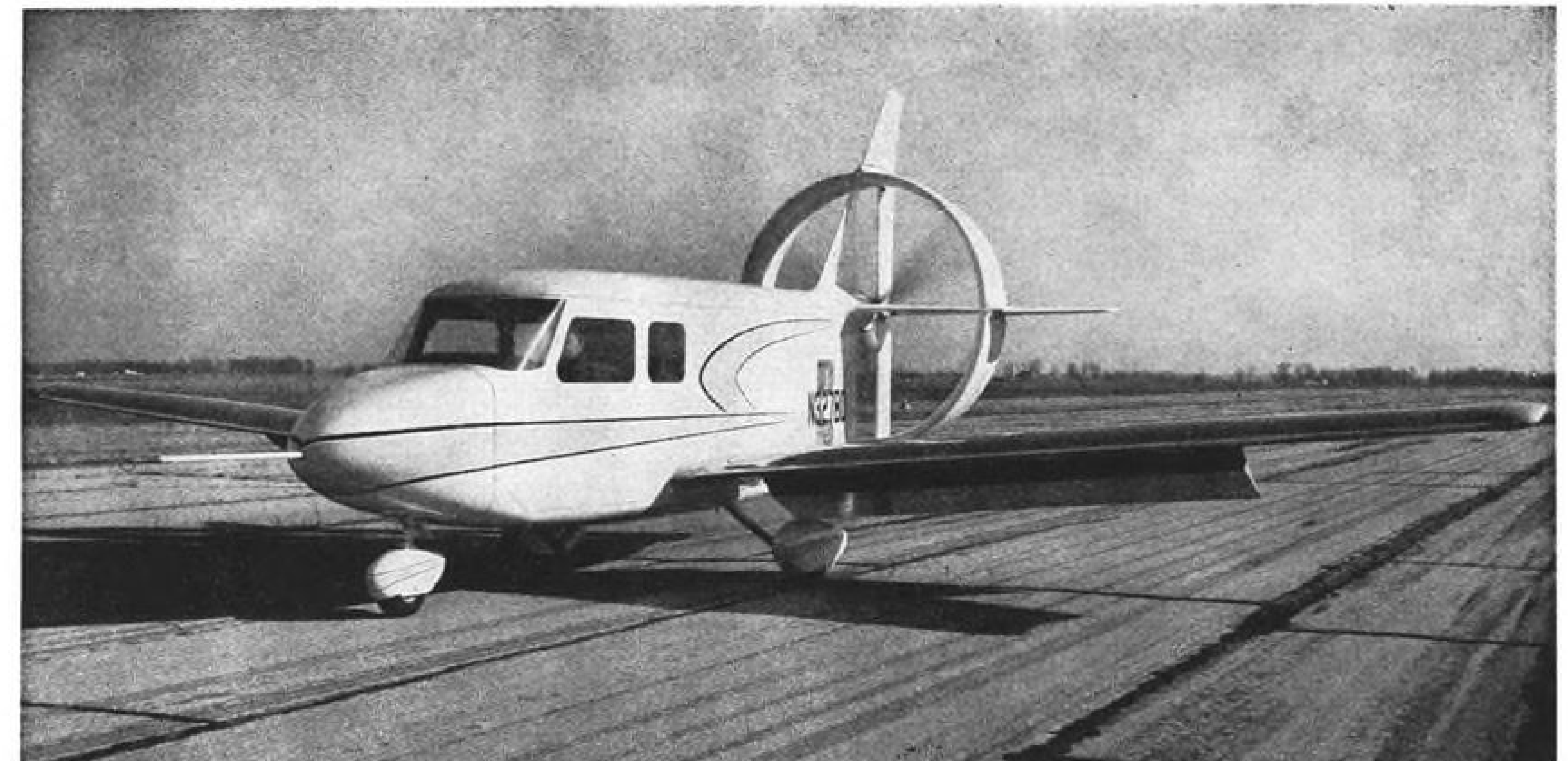
BEDE AIRCRAFT XBD-2 prototype uses twin piston engines to drive a single propeller and to power its boundary-layer control system.
