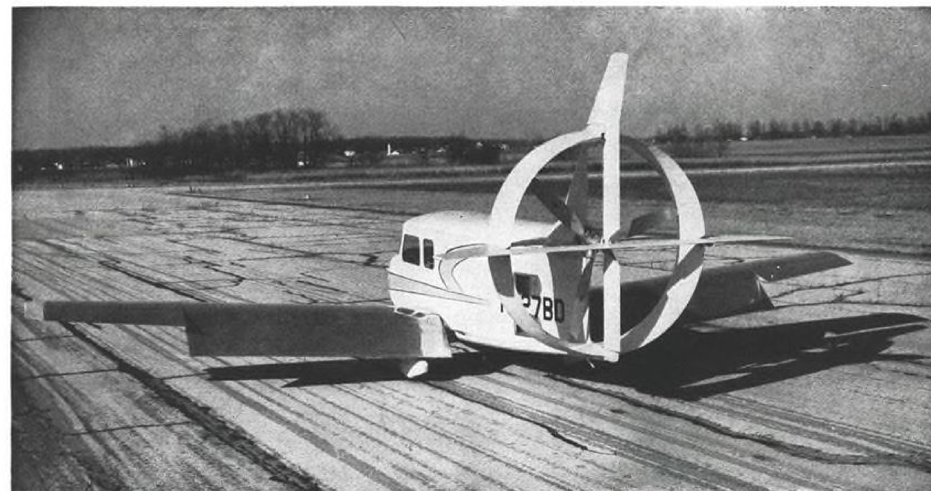
PUSHER PROPELLER SHROUD increases static thrust and efficiency. Ring is formed of unidirectional glass fiber cloth.
