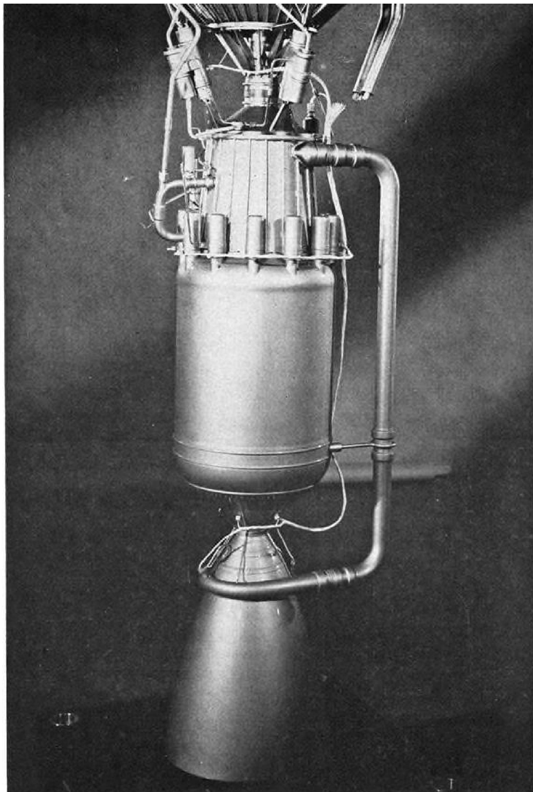
CYLINDRICAL REACTOR CHAMBER of the Nerva nuclear rocket engine (smooth center section) is shown in artist's conception above. Hook-shaped flame deflector duct in chamber in the Nerva test stand's reinforced concrete substructure is shown in model below.
