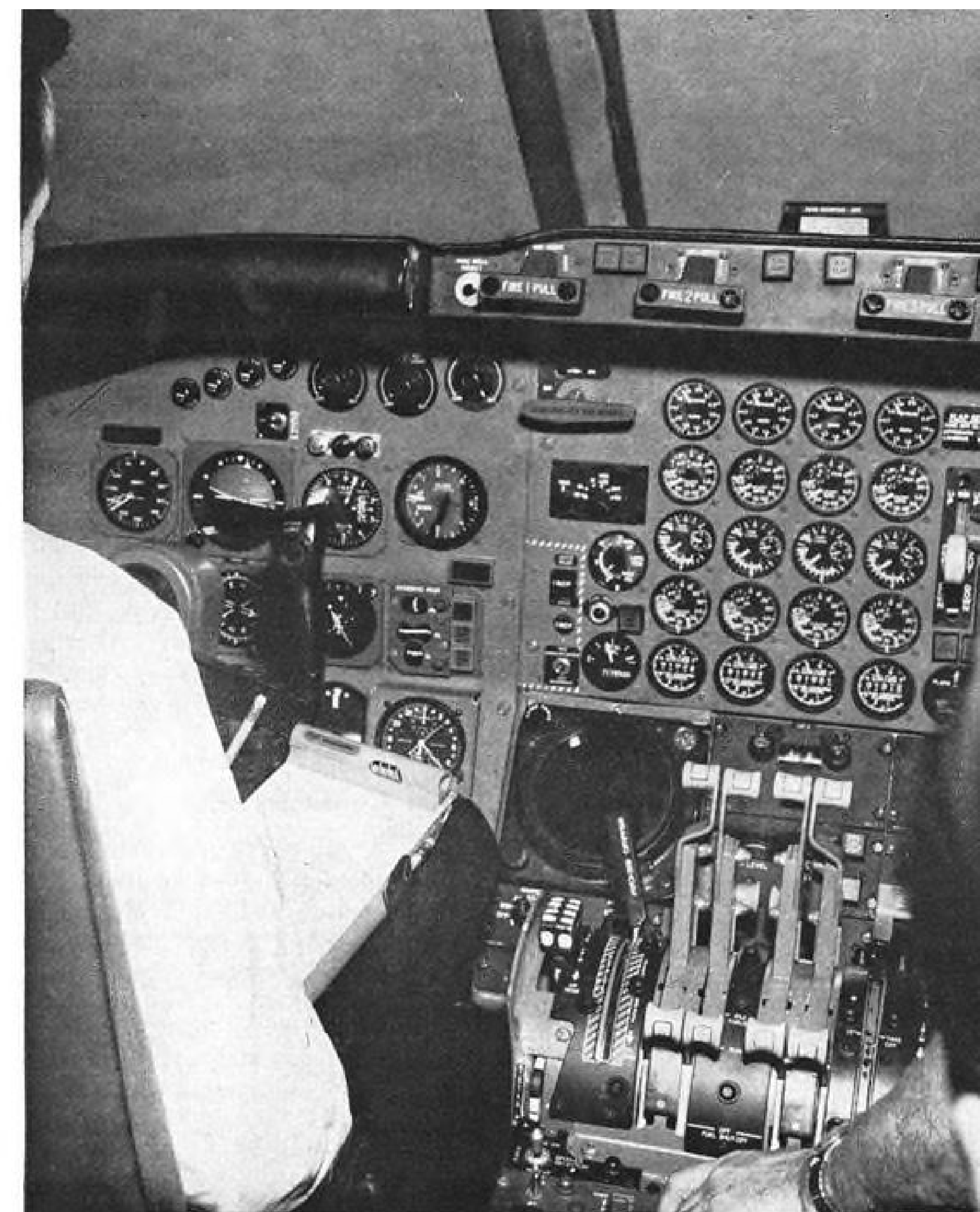
INSTRUMENT PANEL of the 990 has 20 major engine instruments grouped in the center panel. Gages in rows are, top to bottom, exhaust pressure ratio (EPR), fan rpm., exhaust gas temperature (EGT), engine rpm. and fuel flow in kilograms per hour.
