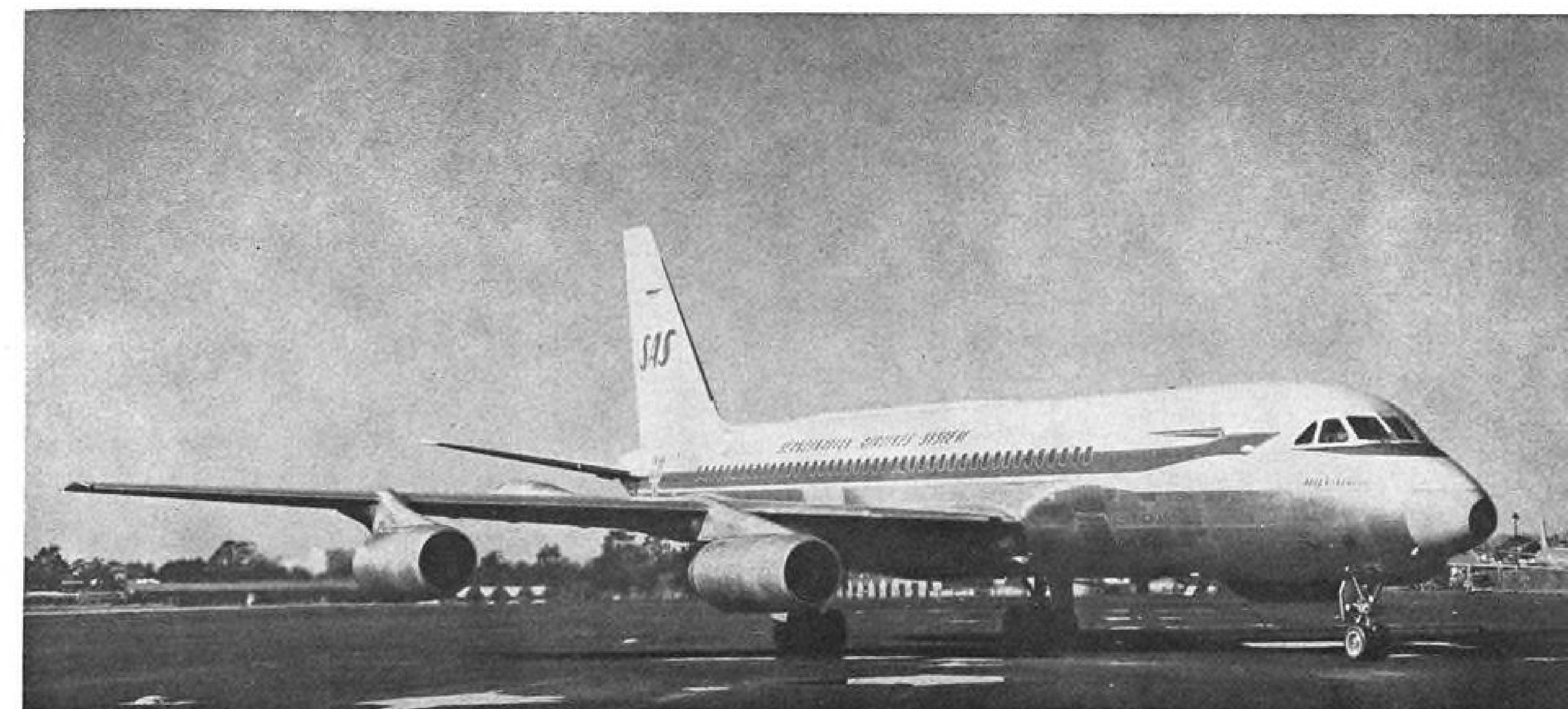
CONVAIR 990, shown here in Scandinavian Airlines System markings, is one of seven ordered by Swissair, two of which will be leased to SAS. Drag reduction program will include fairings on the aft portion of the engine nacelles and a smoother leading edge on the wing.
