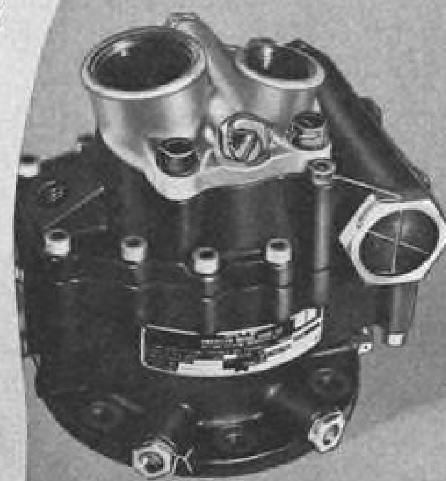
The Atchley servovalves can operate with contaminants as large as 200 microns without malfunction.
