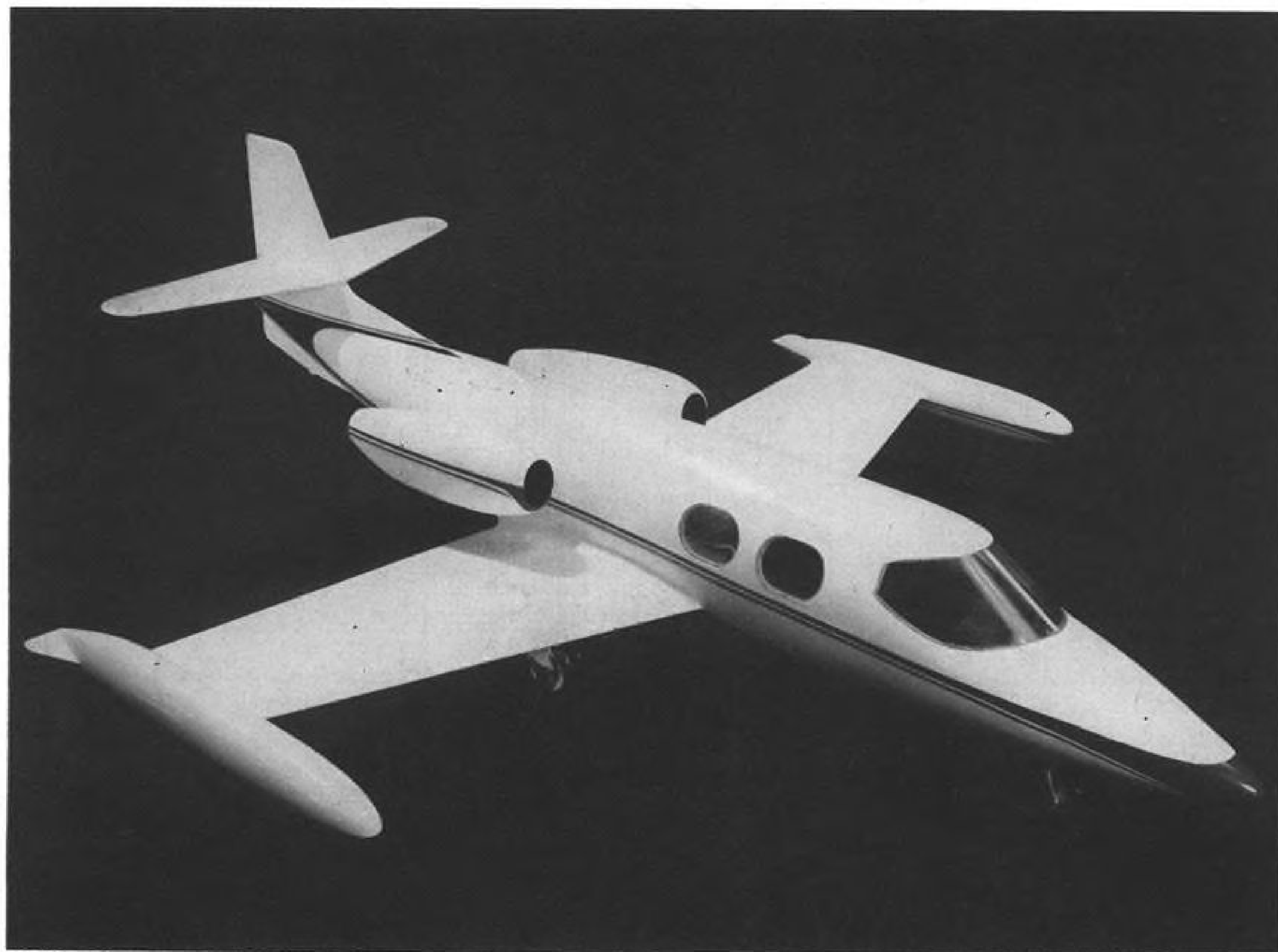
FINAL CONFIGURATION of SAAC 23 six-to-eight place executive jet is shown in model form. Design changes from original specifications include conventional fixed horizontal tail rather than movable surface, plus addition of 23 in. to the fuselage length.
