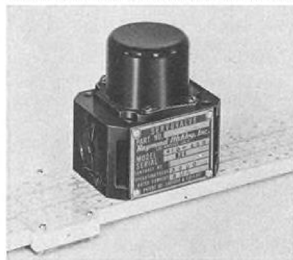
The Atchley servovalves can operate with contaminants as large as 200 microns without malfunction.
