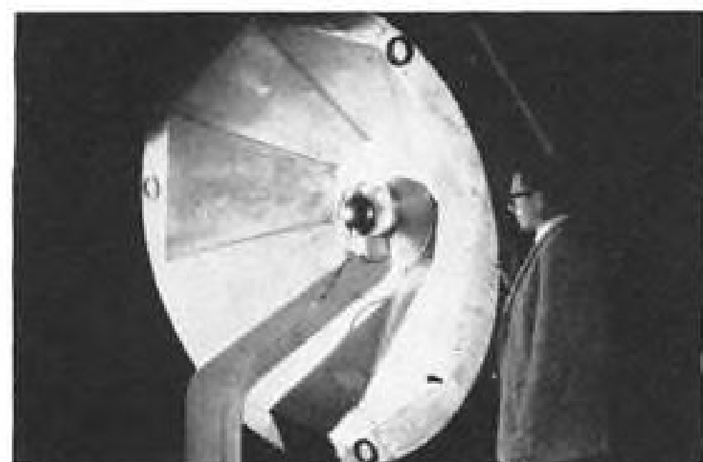
SPACE VEHICLE control systems are tested at Boeing with this satellite attitude control simulator. Optical sensor system controls attitude through reference to light-source simulating starlight. Other Boeing space research involves propulsion, guidance, space vehicles and systems.
