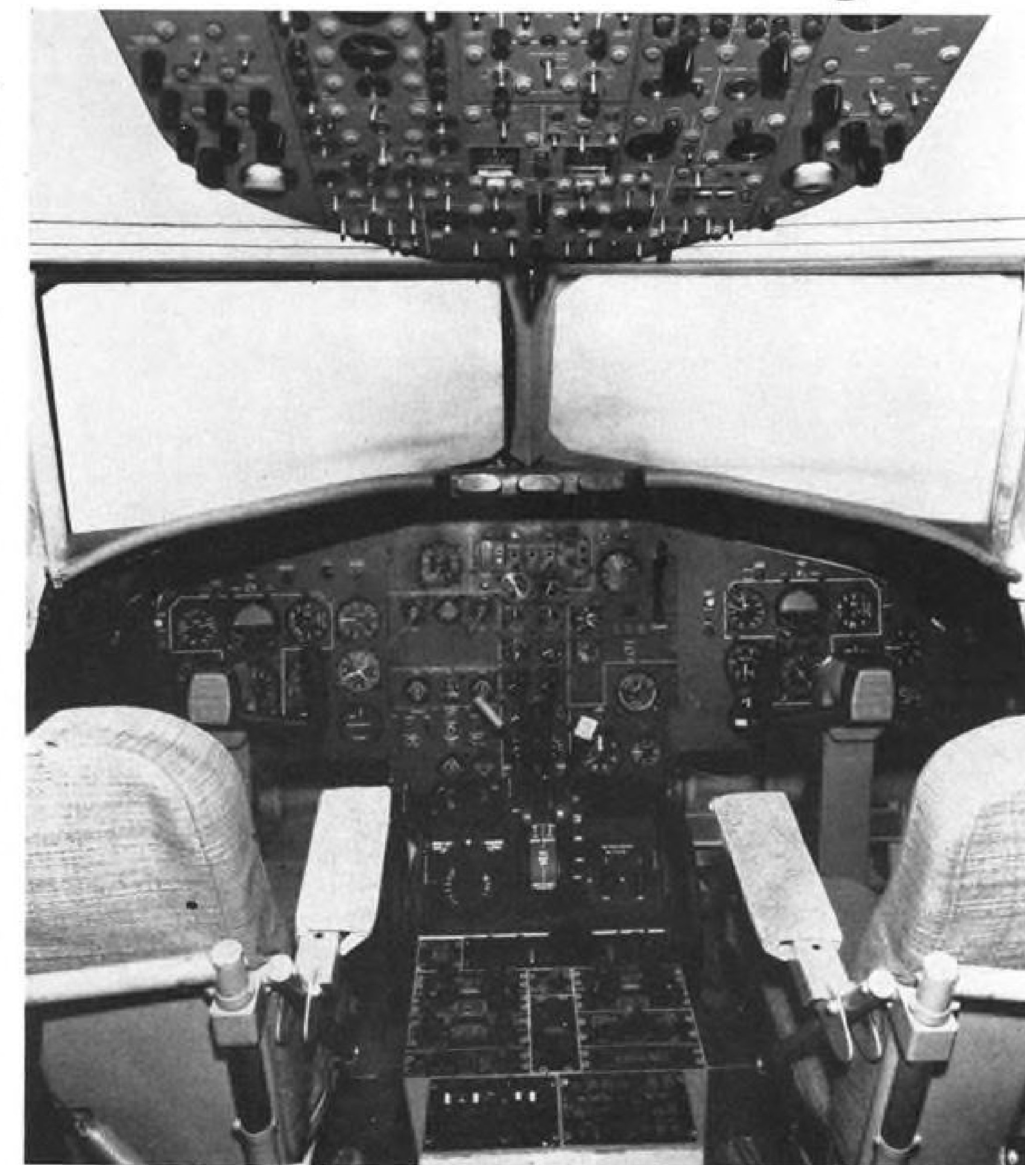
COCKPIT MOCKUP of BAC 111 at Hurn is based on Braniff Airways specifications for two pilot operation. Engine instruments are centered, with flight gages in left and right T outlines. White lighting is used.
