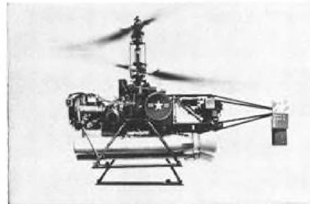
DASH is U. S. Navy's Drone Anti-Submarine Helicopter, designed to operate by remote control from a destroyer. Shown here on unmanned test flight, DASH, designed and built by Gyrodyne Company of America, is powered by a 270-hp Boeing T50 gas turbine engine. Boeing gas turbines, designed for reliability and easy maintenance, are used in land, sea and air applications.
