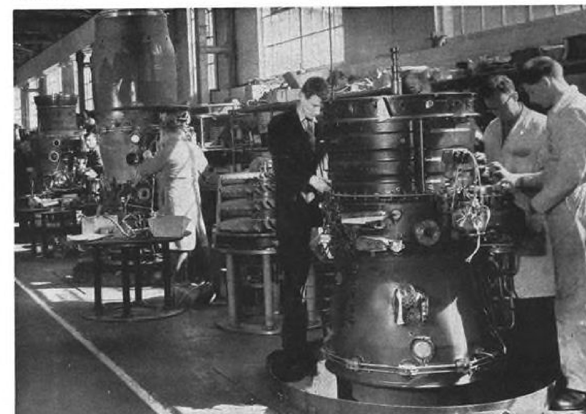
ROLLS-ROYCE SPEY bypass jet engine for BAC 111, de Havilland Trident and Blackburn Buccaneer naval strike fighter is built at the Derby factory.
