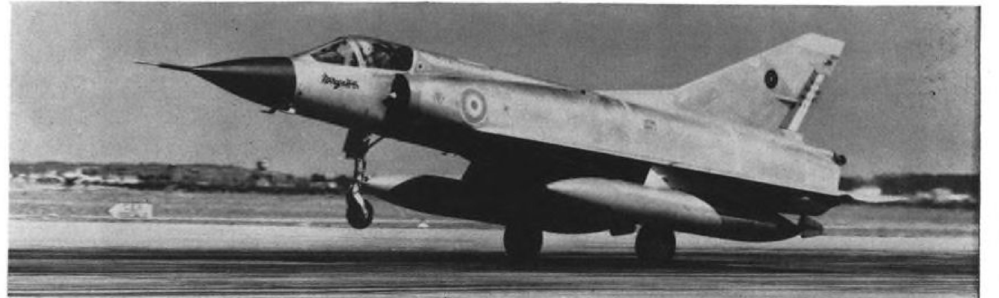
Mirage 3C is shown above with auxiliary fuel tanks slung under the wings. Below, USAF test pilot, one of three who evaluated the aircraft and its associated weapons systems deploys a cruciform arresting parachute immediately after touchdown.
