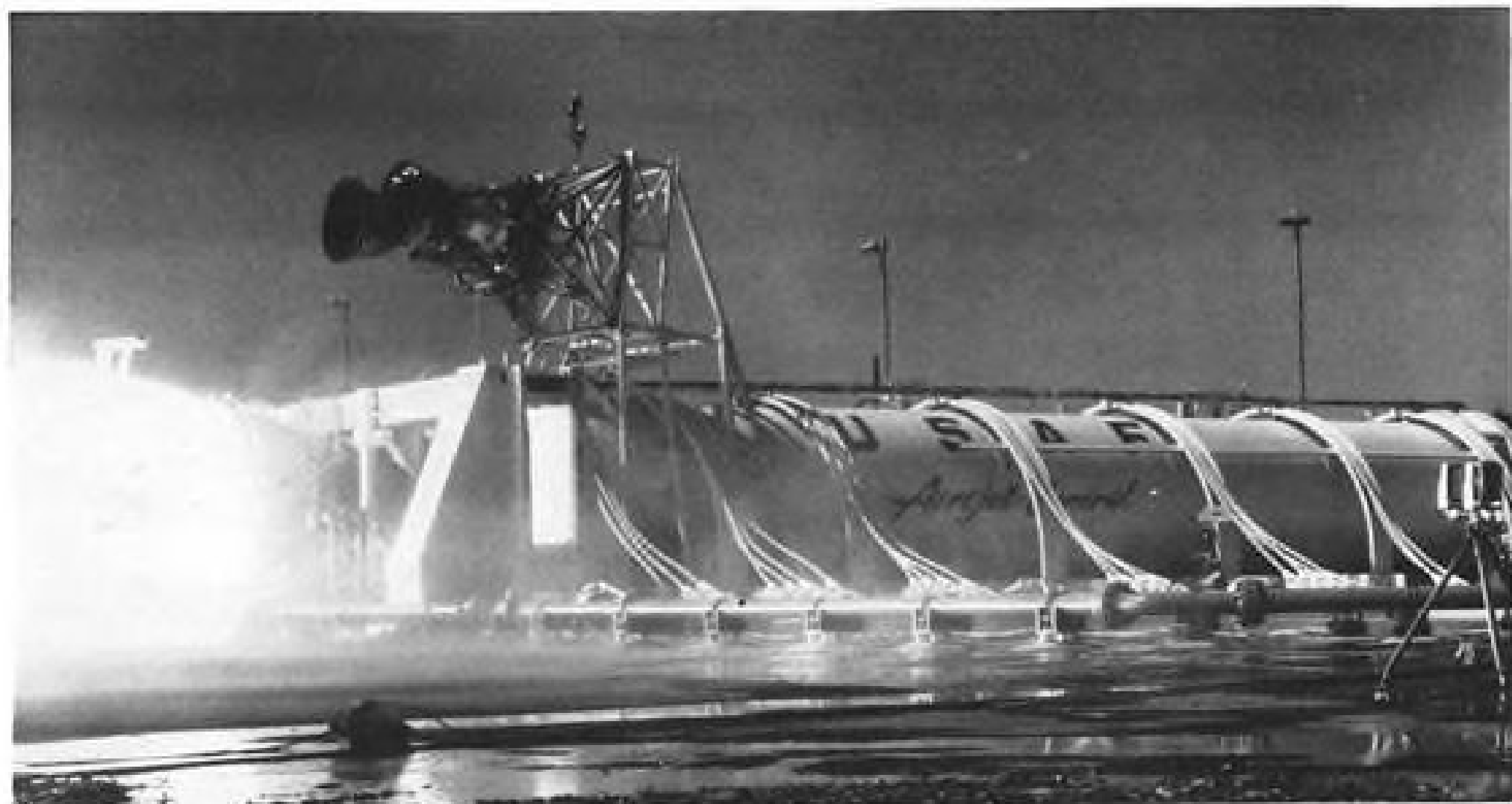
TITAN LIQUID PROPELLANT ENGINE was mounted near a large solid propellant engine for environmental tests during a recent firing of the solid motor by Aerojet-General Corp. at Sacramento, Calif. Solid engine developed 700,000 lb. thrust, but ruptured several seconds after photograph was taken. Titan engine nozzles were destroyed by the rupture which occurred when solid engine chamber pressure dropped after 45 sec. of scheduled 120-sec. firing. Total engine run was 71 sec. Titan engine environment tests are designed to show effect on the motor during future space flights with solid boosters.
