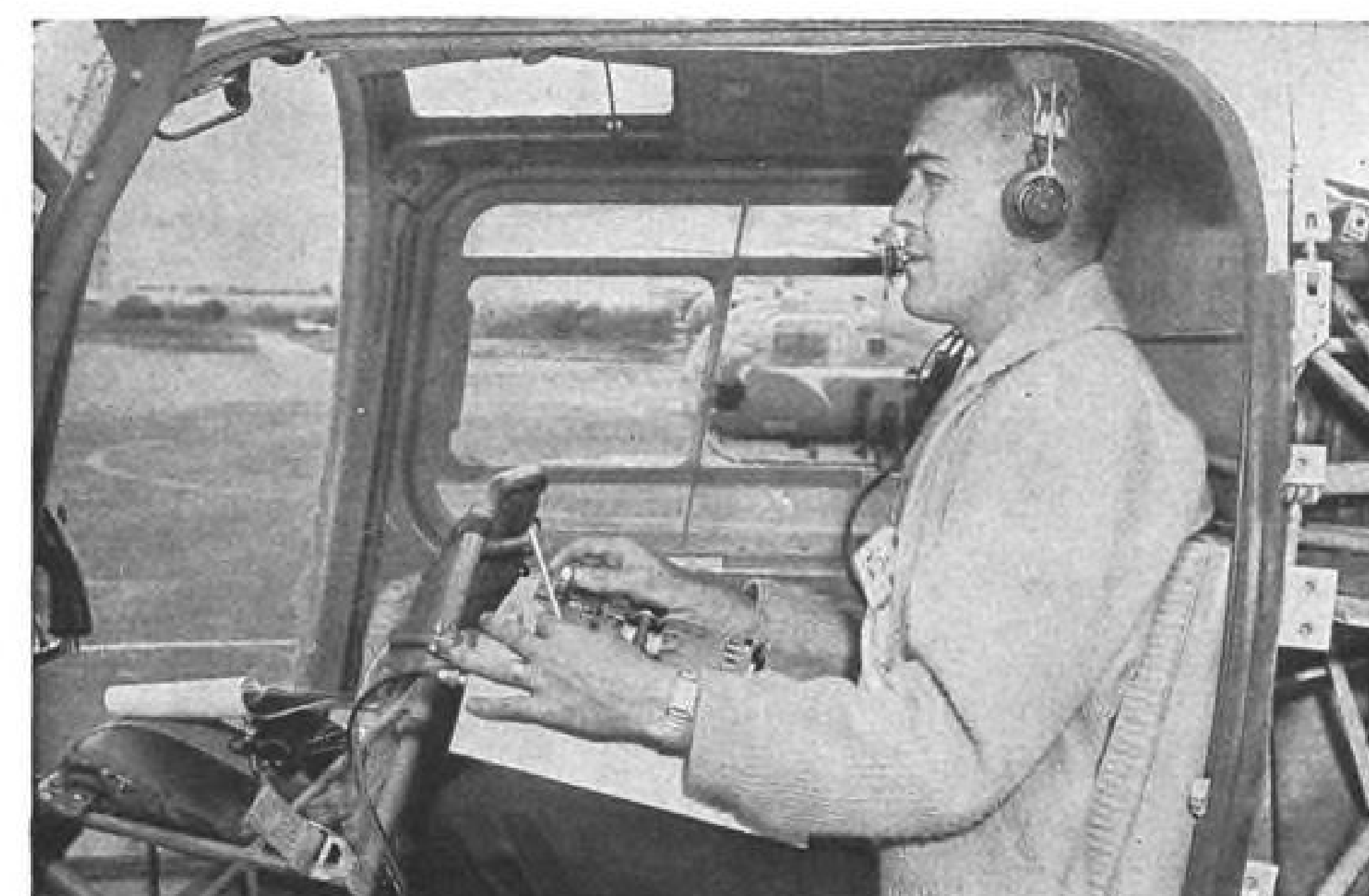
CONTROL PANEL 17 x 13 in. is held by non-pilot drone operator in cabin of 47J-2.
