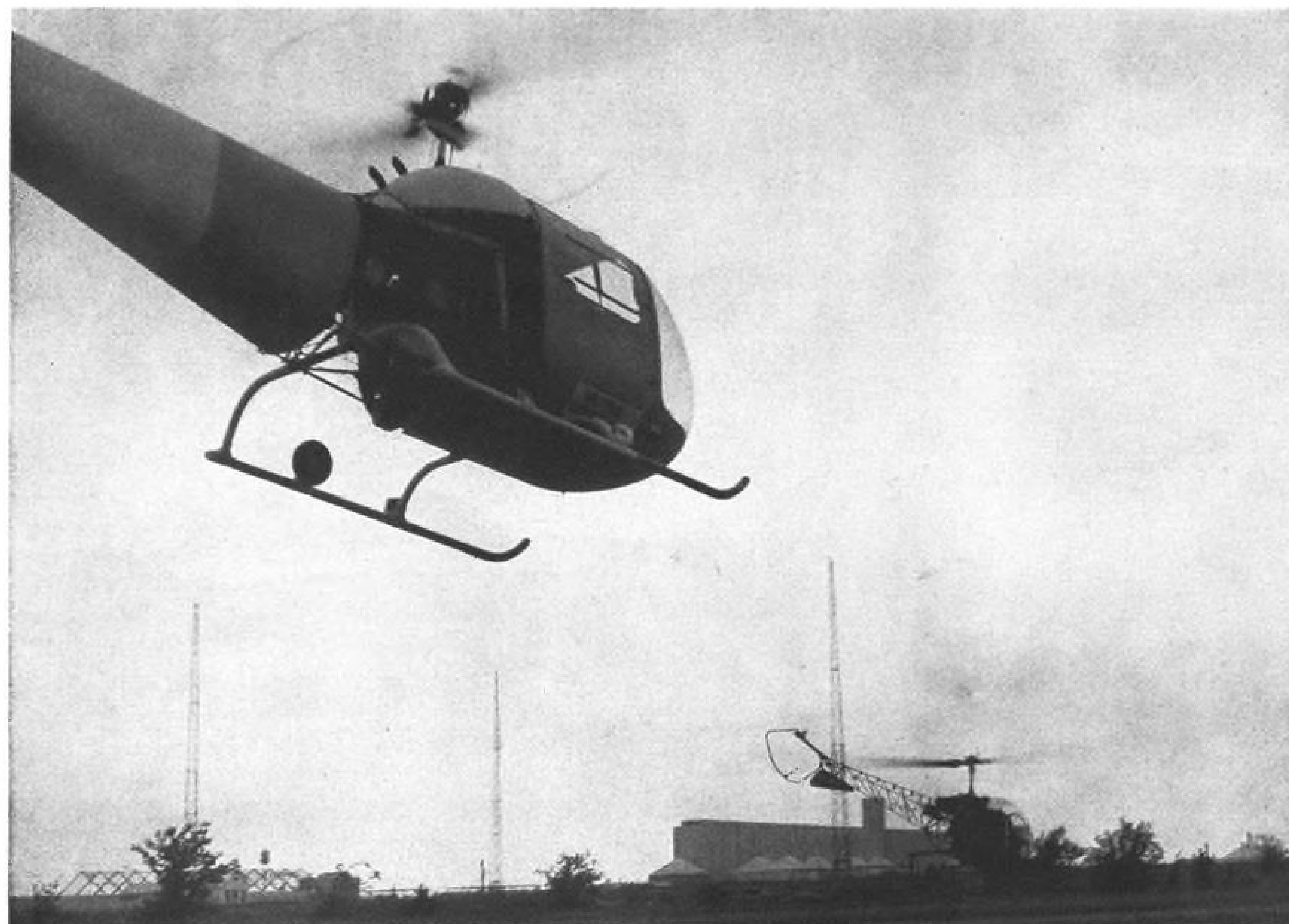
BELL 47J-2 MOTHER SHIP controls an Army H-13E drone in tests at Bell Helicopter's Ft. Worth, Tex., plant.
