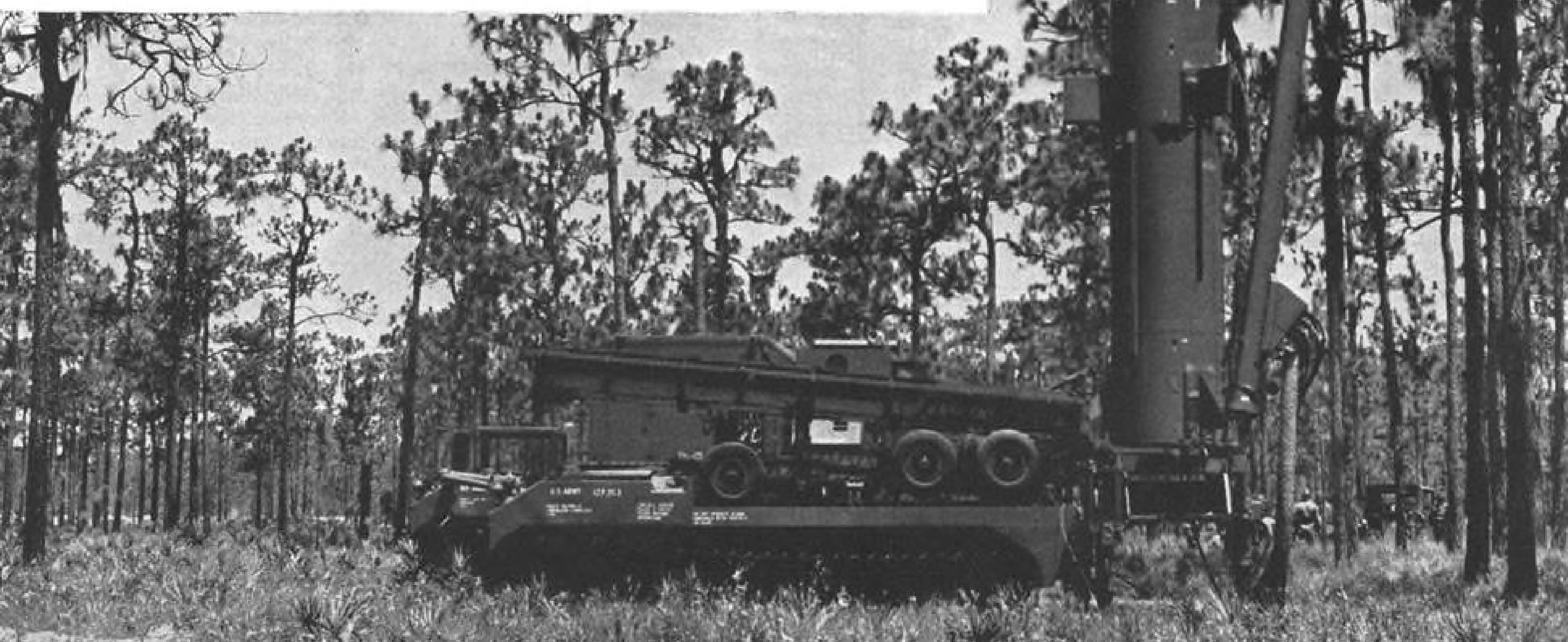
Army crew, above, mates warhead to missile, while other crewmen prepare missile for launch. Erection to firing position takes about one minute. Separation of umbilical mast signifies firing of missile. Operation took less than 15 min.
