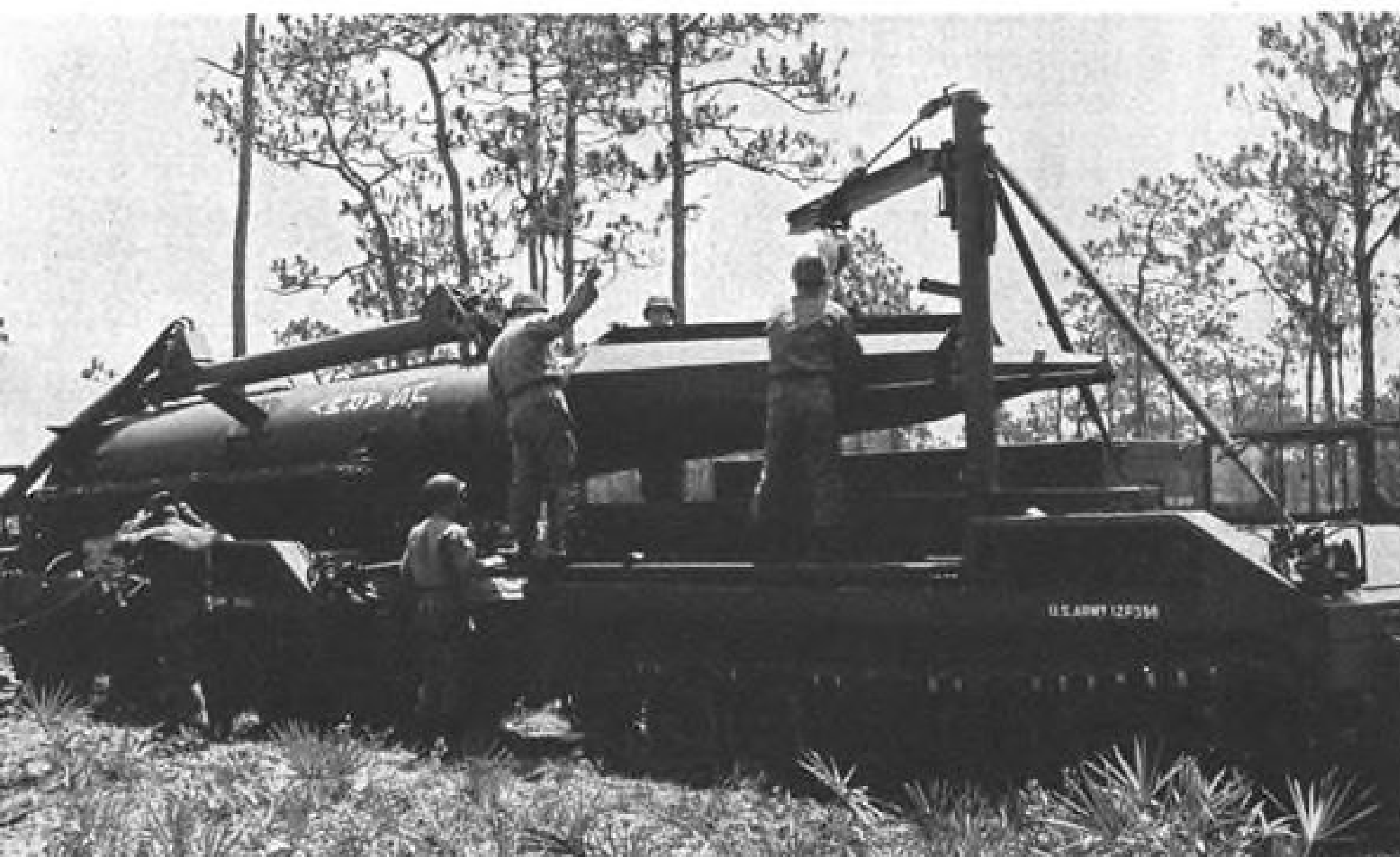
Army crew, above, mates warhead to missile, while other crewmen prepare missile for launch. Erection to firing position takes about one minute. Separation of umbilical mast signifies firing of missile. Operation took less than 15 min.
