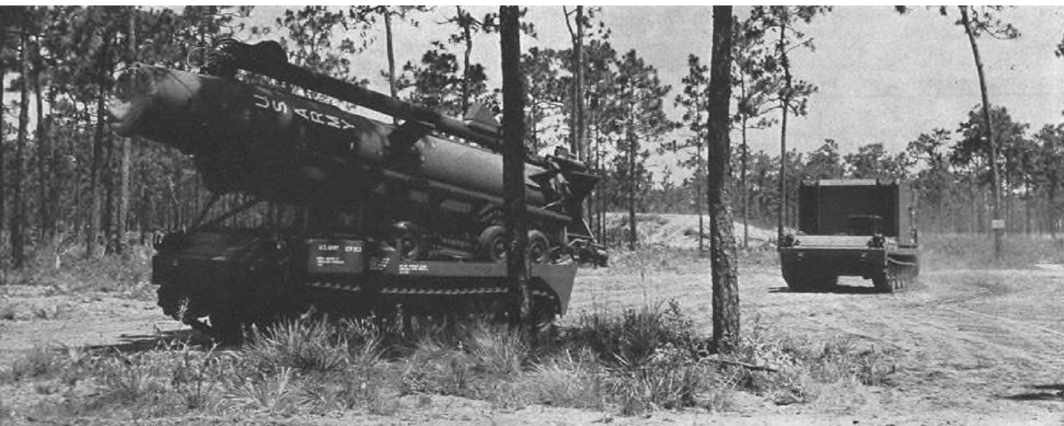
Pershing missile battery moves to pre-selected launch site during firing demonstration. Lead vehicle carries missile body on erector-launcher. Other vehicles carry the warhead and communications equipment. Demonstration took place at Orlando, Fla.
