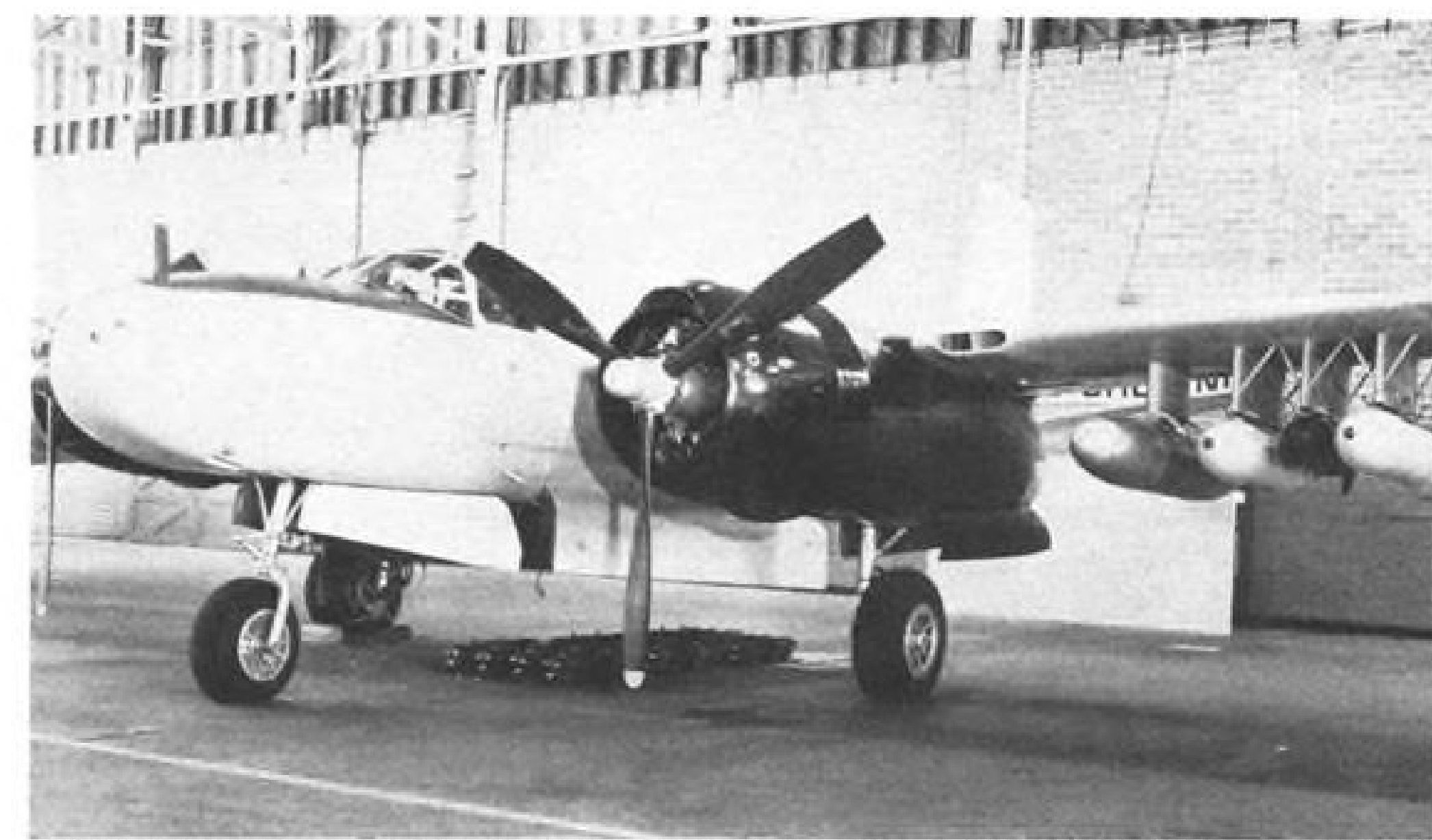
DOUGLAS B-26 , is equipped for special warfare with an M116A2 fire bomb; LAU-3A rocket launcher; 500 lb. general purpose bomb, and an LAU-3A fire bomb. On the hangar floor are M1A2 fragmentation bombs.
