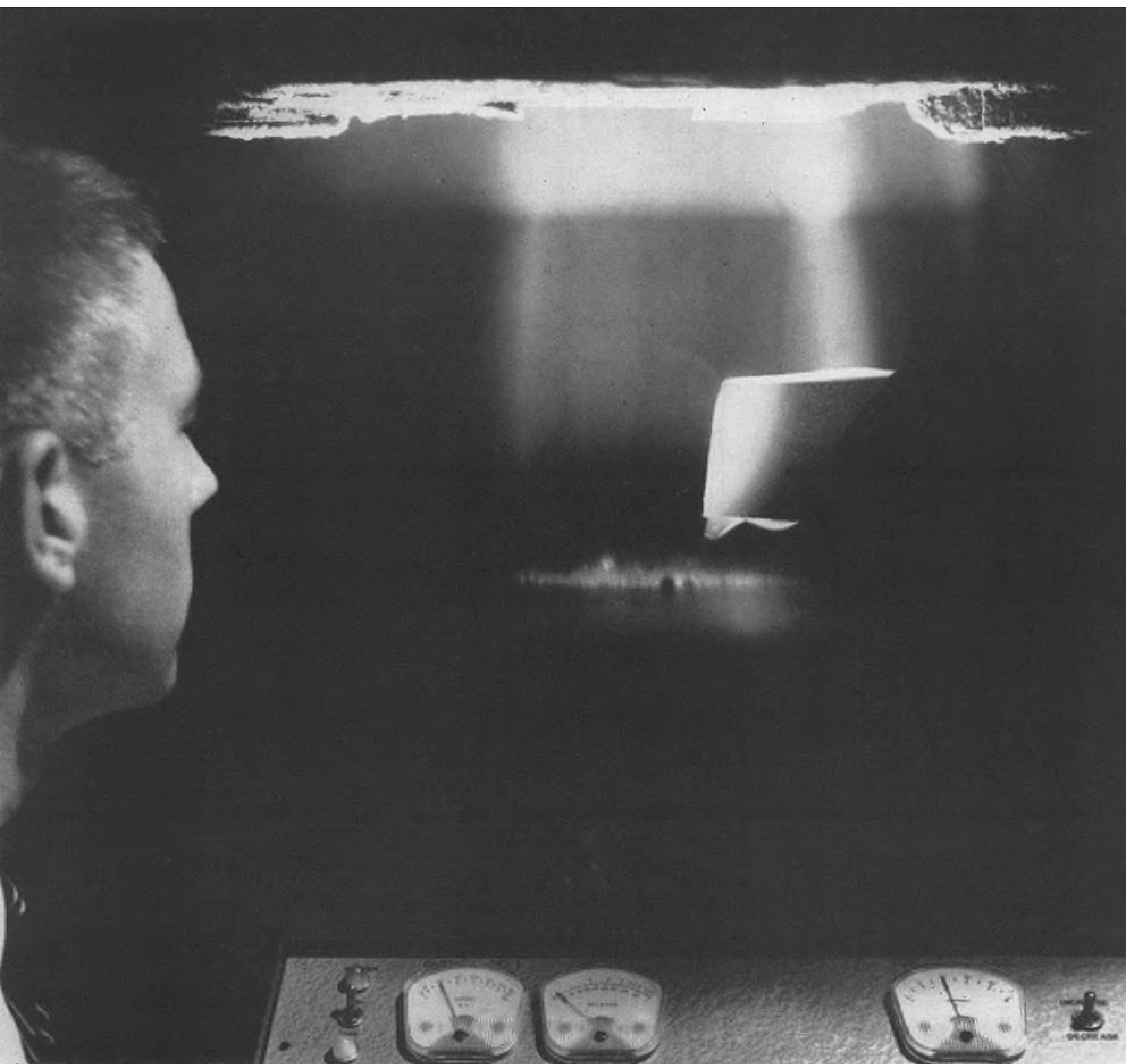
Melting a columbium alloy in Haynes Stellite's electron beam furnace.
