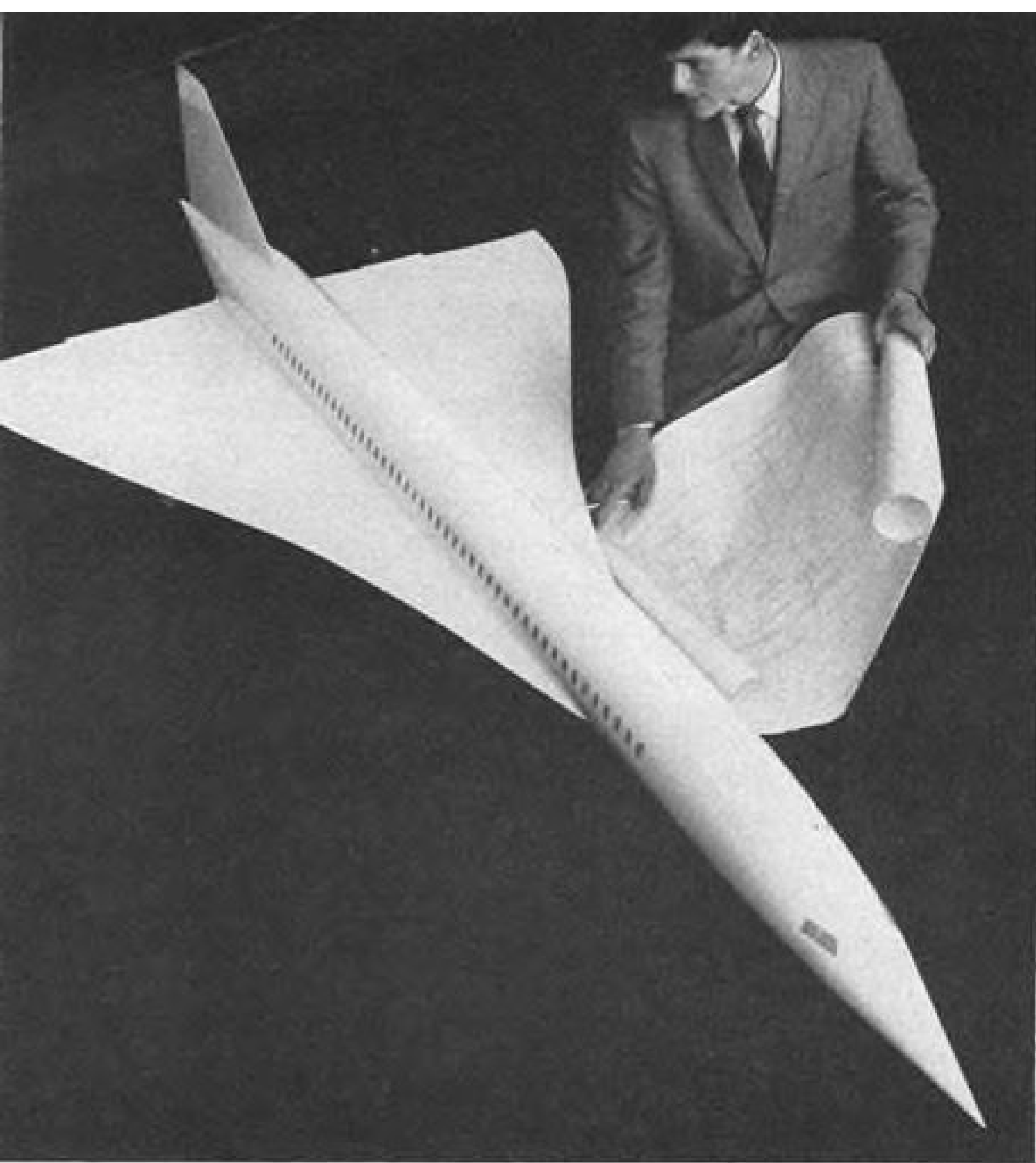
TOP VIEW of Mach 2.2 transport model, left, shows slight waisting aft of wing leading edge. Two versions are proposed, one for medium range and another for long ranges, such as London-Paris to New York. Note extensive tail area and squared exhaust outlets for four Olympus 593 engines, above. Variable geometry ramps are being designed by Snecma, which is responsible for about 40% of engine development, according to Sir Arnold Hall, Bristol Siddeley managing director.
