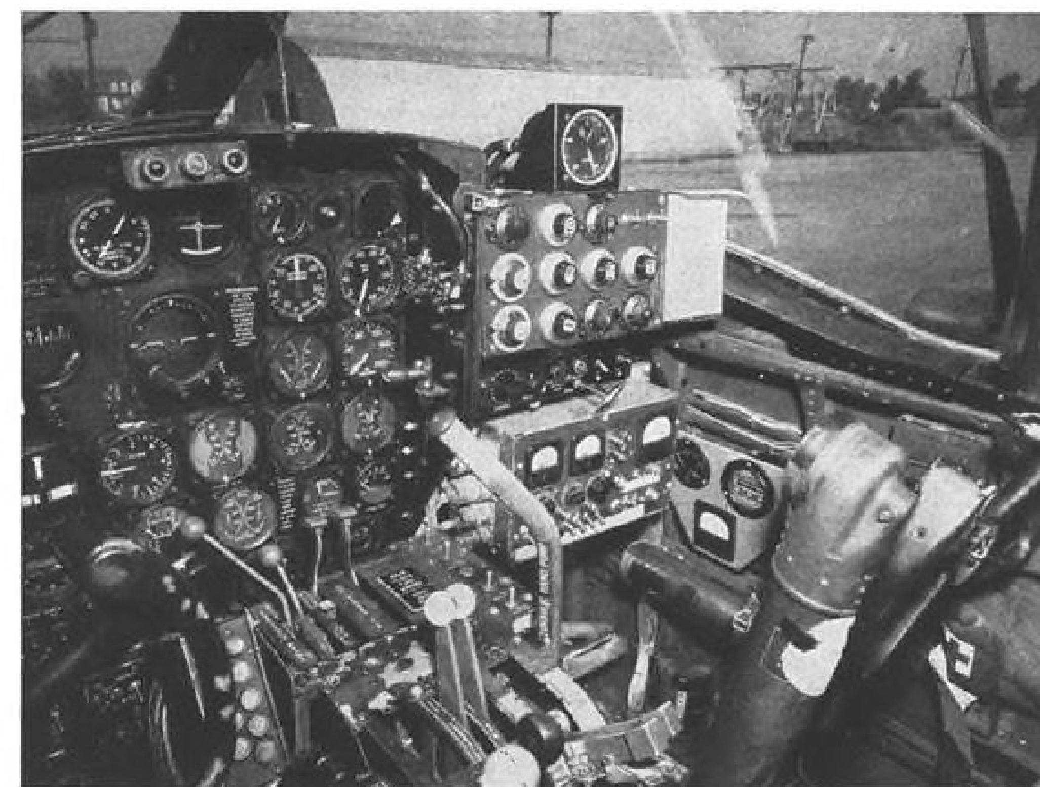
RHEOSTAT GAIN CONTROLS on panel forward of the right control column are used to vary the B-26's stability, stick forces and responsiveness.
