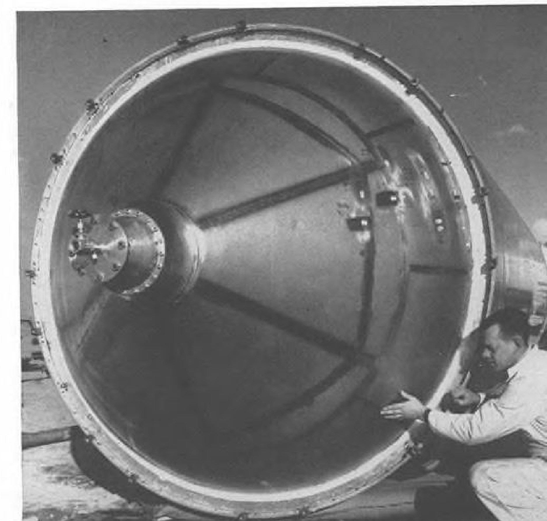
Largest titanium assembly ever made, the 7,000 gallon test vessel designed and produced by Beech Aircraft, measures 8 feet in diameter by 24 feet in length.
