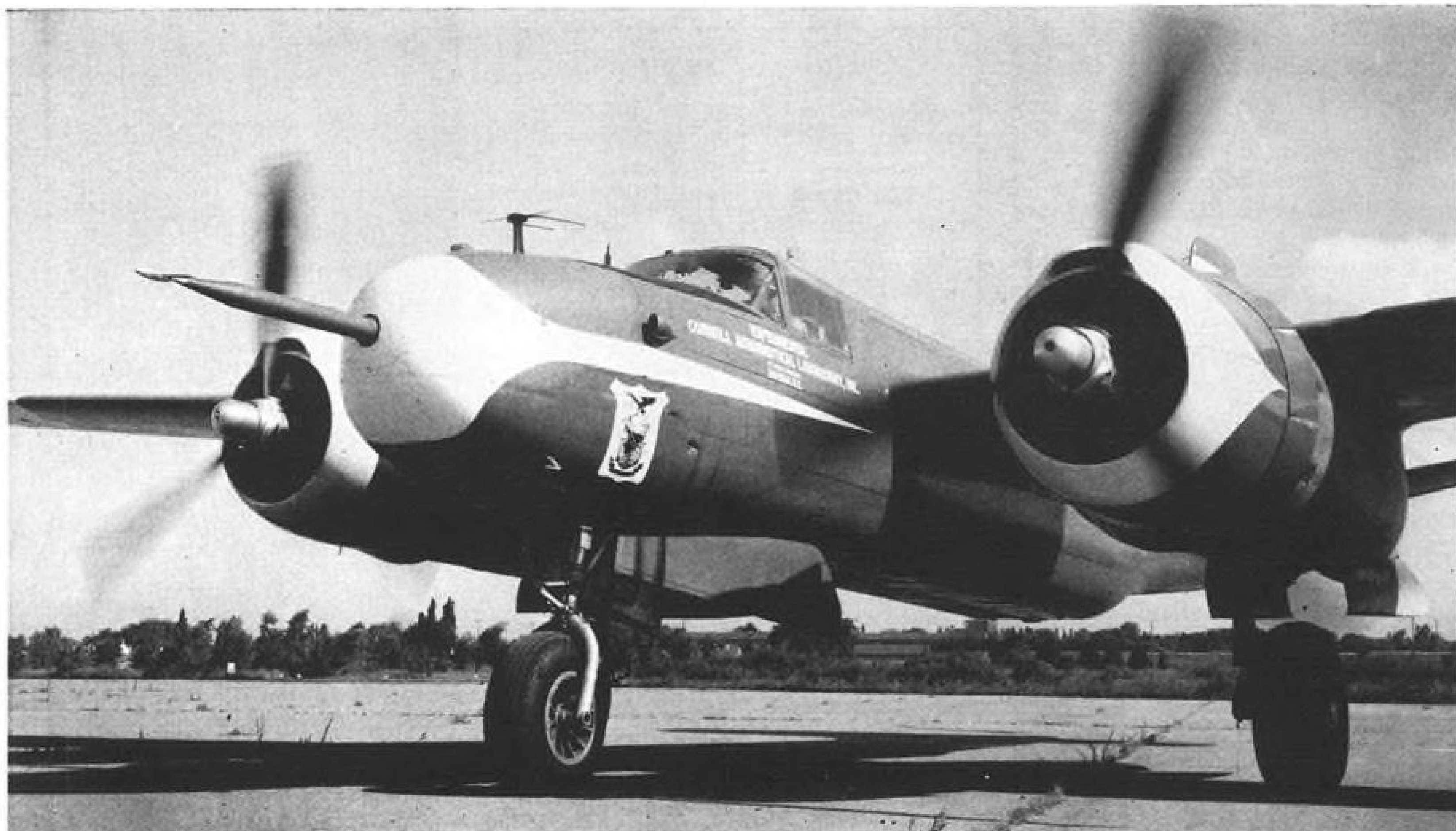
NAVY AND FEDERAL AVIATION AGENCY test pilots are flying Cornell Aeronautical Laboratory's variable stability Douglas B-26 under programs funded by the two services. During in-flight demonstrations, pilots learn to recognize and identify stability and control forces that, in combination, make an aircraft behave in its characteristic fashion. The probe extending from the nose of the aircraft is an angle of attack vein that is used for measuring angle of attack and rate of change.
