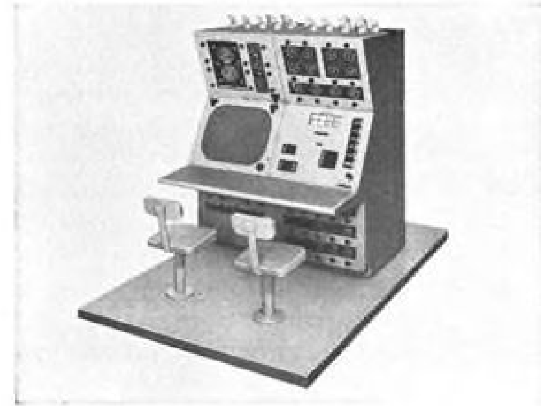
ASROC —The computer which directs firing of the Navy's antisubmarine rocket weapon system, a mainstay of U.S. defense. It is one of the latest of 11 major Librascope contributions to ASW dating from 1940. Many of the underwater fire control systems in the Navy's antisubmarine fleet today were designed and/or built by Librascope.
