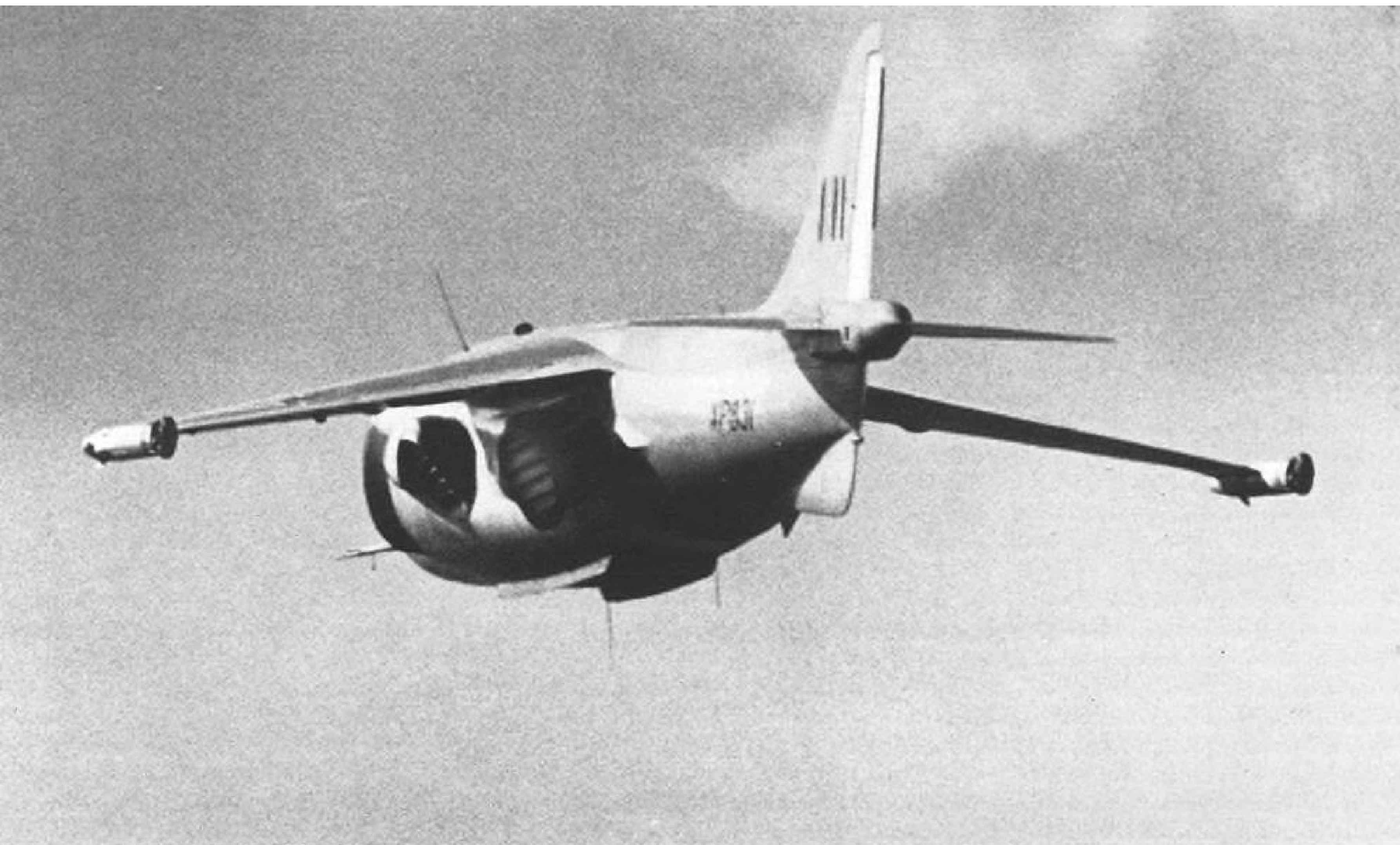
Swinging away and around after gear is fully retracted, P.1127 pilot begins swivelling the BS.53 nozzles back to the horizontal position for conventional flight and, moments later, a low-altitude high-subsonic pass over the field.
