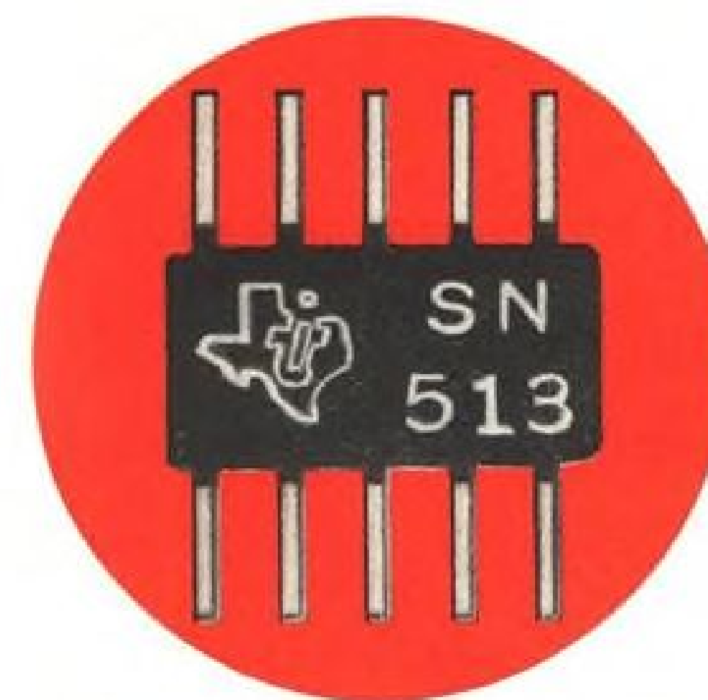
Completed SOLID CIRCUIT semiconductor network, enlarged 5½ times.
