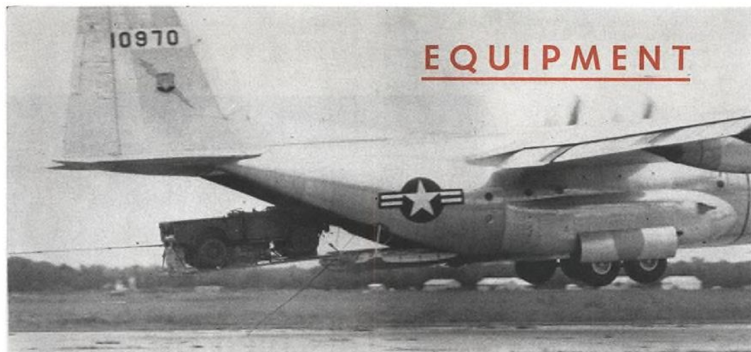
CARGO EXTRACTIONS were made with an Air Force C-130B on the ground and in the air using All American Engineering system.
