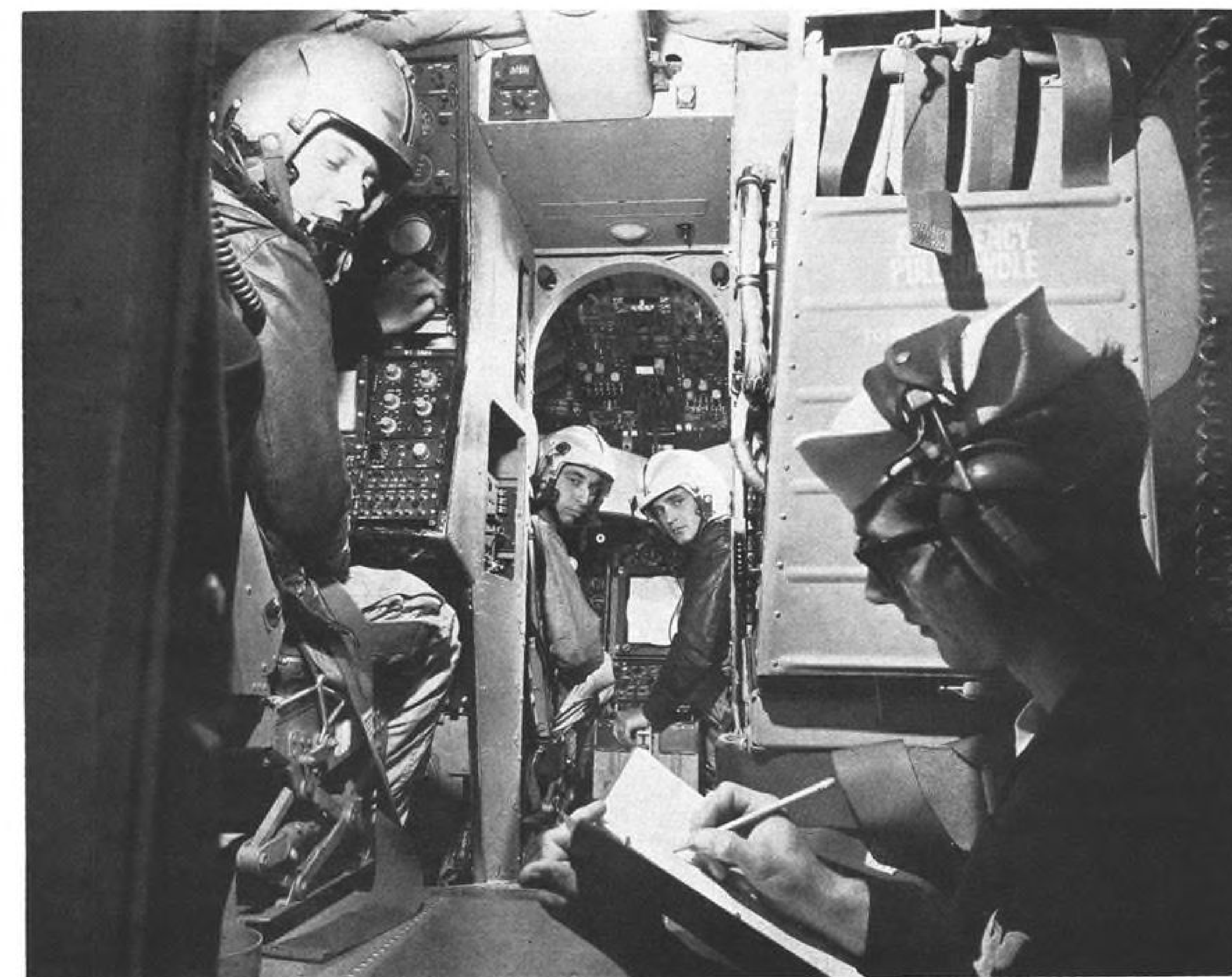
ACF ELECTRONICS 2F-66 ASW simulator contains an exact duplication of the cockpit and crew stations in the Grumman S2F-3. Radar/Magnetic Anomaly Detection gear operator at left is being critiqued by instructor at right during simulated problem.
