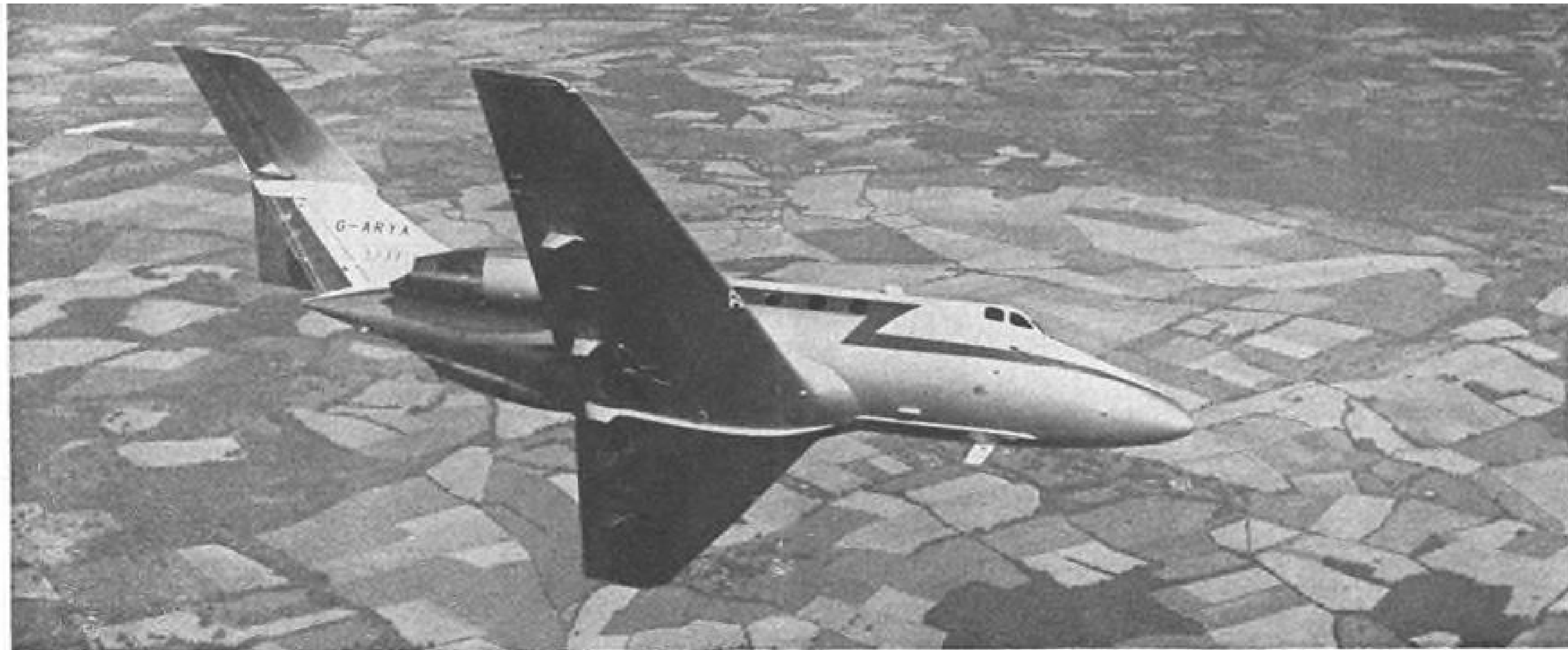
First production de Havilland DH-125 executive jet has lengthened wing and an increased tail area.
