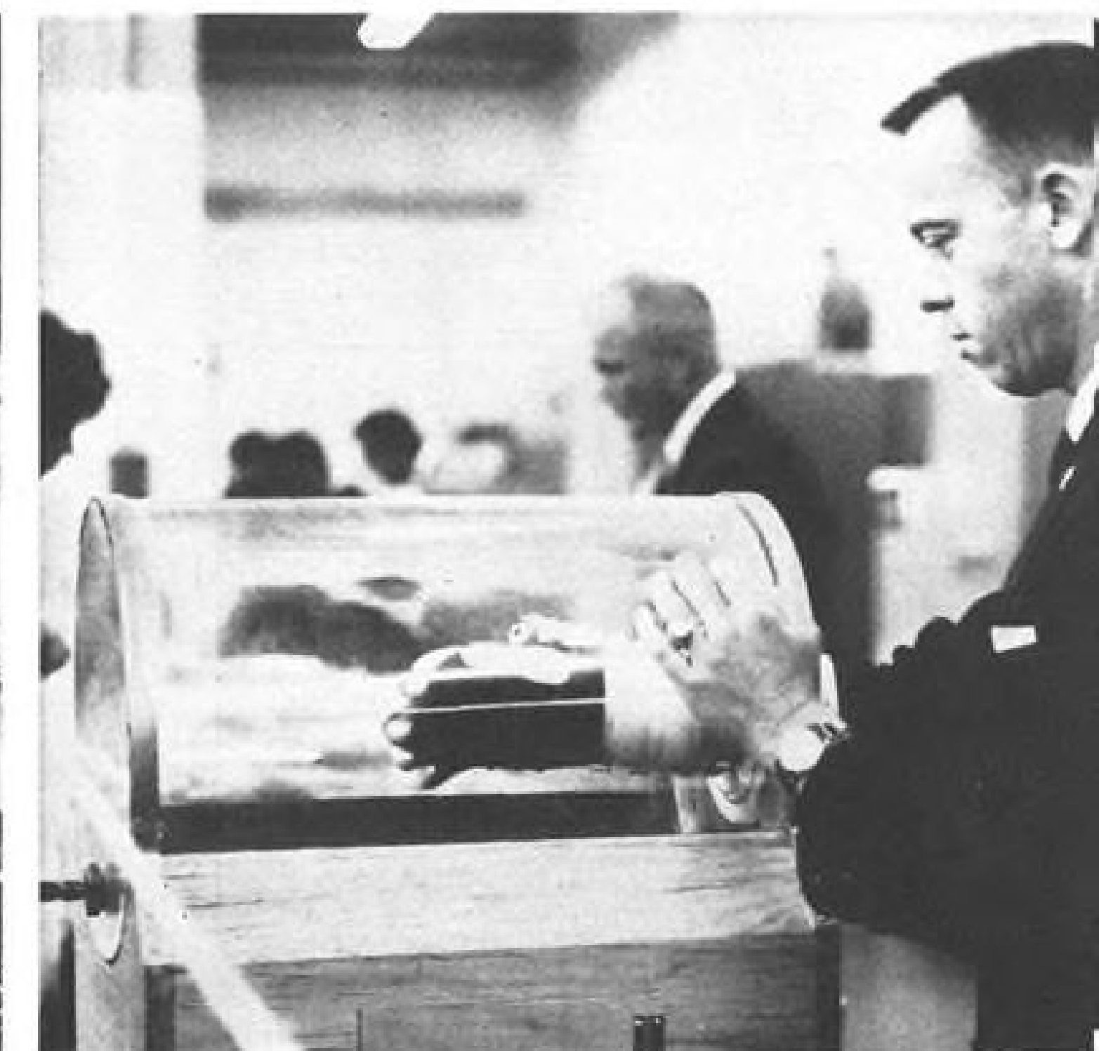
Half-scale model of Paraglider-Gemini configuration (left), in landing attitude was displayed. Adapter section of Gemini section is shown as it would be after jettisoning. Right, Astronaut Shepard demonstrates flexibility of Mercury pressure suit glove in vacuum chamber.
