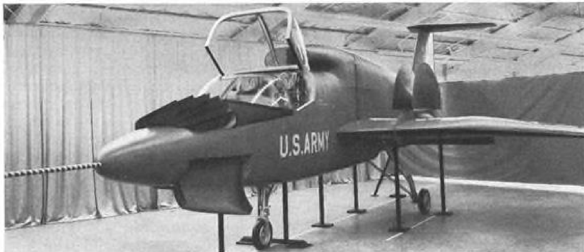
Mock-up of U.S. Army's VZ-11 lift-fan VTOL flight research aircraft shows vertical takeoff or landing configuration. Nose fan inlet louver doors, nose fan thrust modulation doors and lift-fan inlet closure doors are all in open position. At right,
