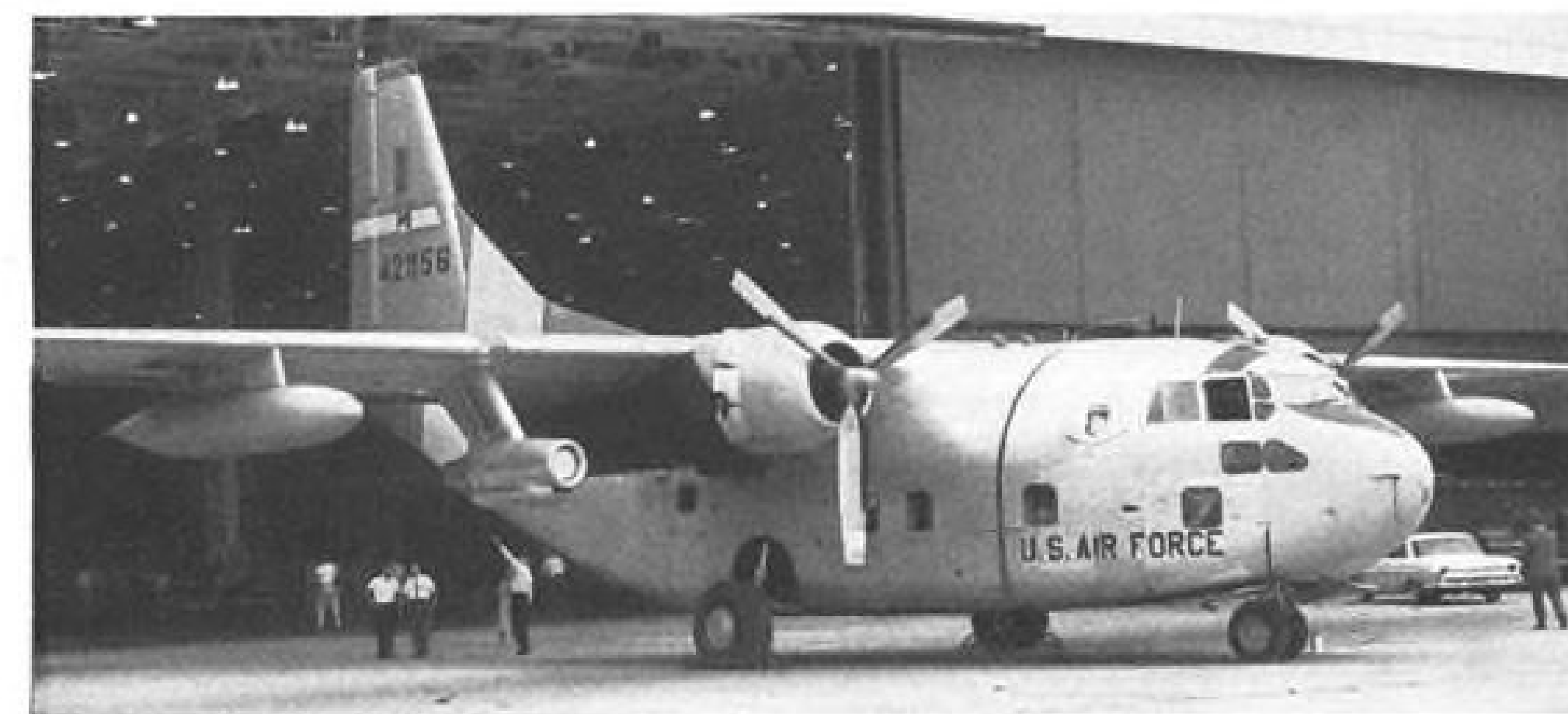
JET-BOOSTED, this C-123H was recently flight-tested with two General Electric CJ610 turbojets. Fairchild reports significant reductions in take-off and landing distances.
