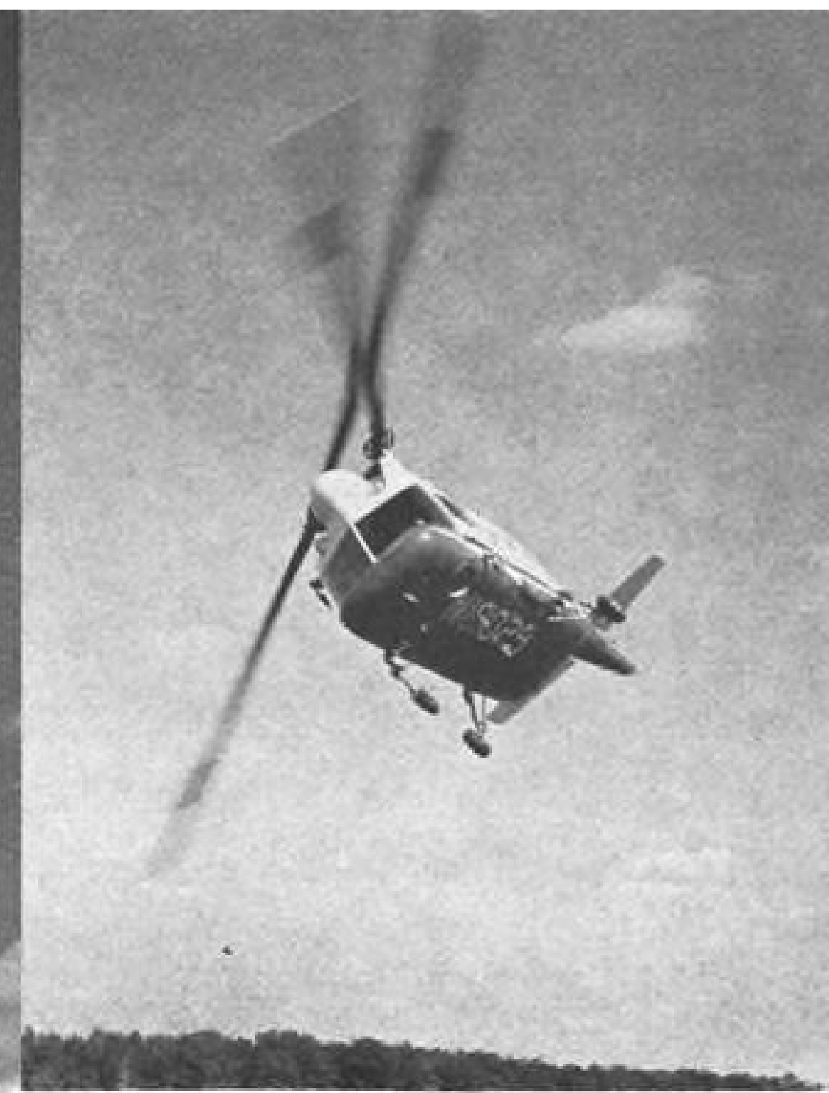
K-1125 DEMONSTRATES MANEUVERABILITY by making a tight turn at low-level. Right, redesigned cockpit has dual instrumentation for IFR flight and single twist-grip throttle on collective which controls both engines. Flat windshield also is designed for IFR work.
