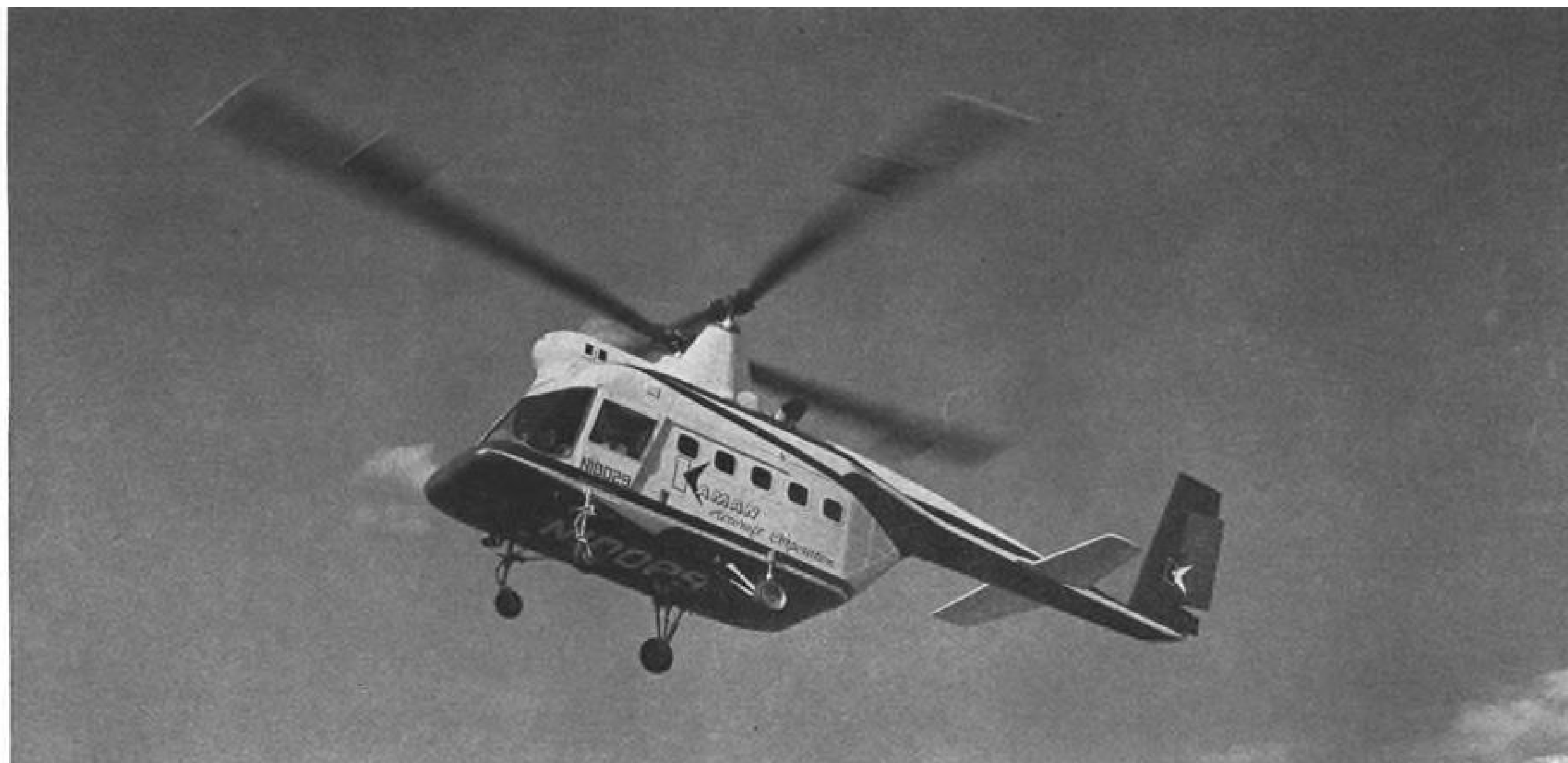
KAMAN K-1125 , growth version of the Air Force H-43B, is powered by twin Boeing YT-60-10 turbine engines and has a redesigned cockpit, enlarged cabin and single-boom empennage. Note large amount of rudder travel available.
