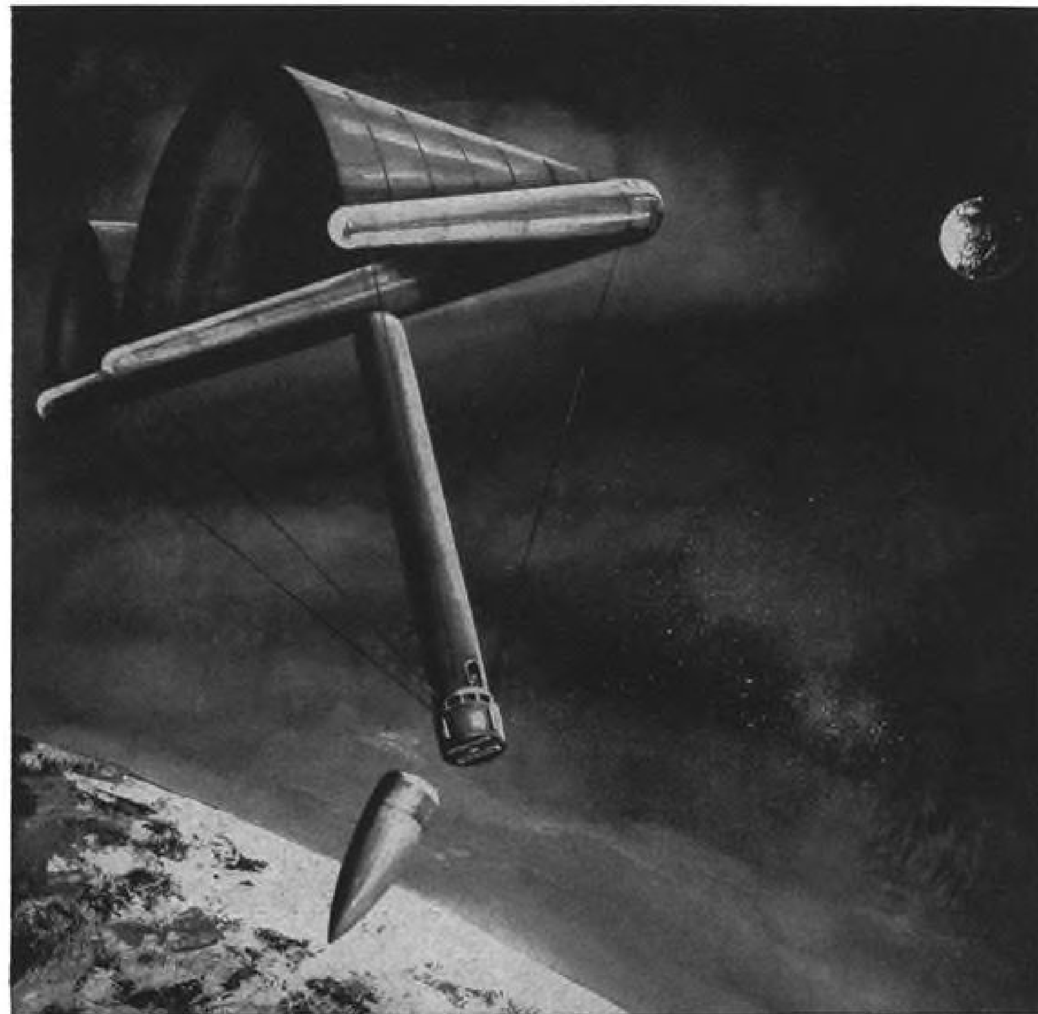
ARTIST'S VERSION of inflatable micrometeoroid paraglider (IMP), being developed by Space-General Corp. for NASA, shows nose cone containing power supplies, programmer, instrumentation, and telemetry being jettisoned just before paraglider begins re-entry. Sketch shows configuration of tubular structural members and sails, the latter being covered, top and bottom, with the micrometeoroid sensors.
